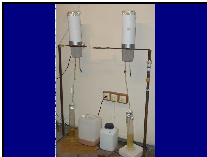
Figure A.1. Experimental set-up of LBRs under mesophilic conditions
