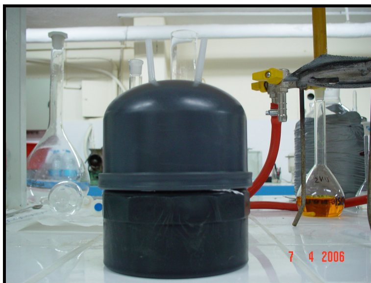
Figure B.2. Leachate collection component of LBRs design
