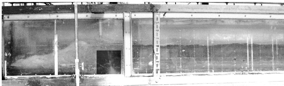
**Figure 4.6:** Steady jump [Reflection of the flasher is dimmed]
