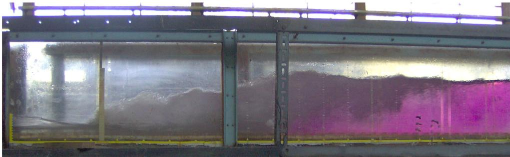
**Figure 4.1:** A view of steady jump ( $F_1=9.65$ ) [I]
