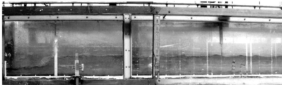
**Figure 4.4:** A view of jump for strip roughness with  $w/L=4$ ,  $w/Z=6$ ,  $F_0=5.08$ ,  $F_1=3.28$
