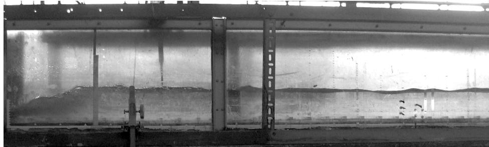
**Figure 4.5:** A view of jump over a strip roughness of  $w/L=4$ ,  $w/Z=6$ ,  $F_0=5.08$ ,  $F_1=4.02$
