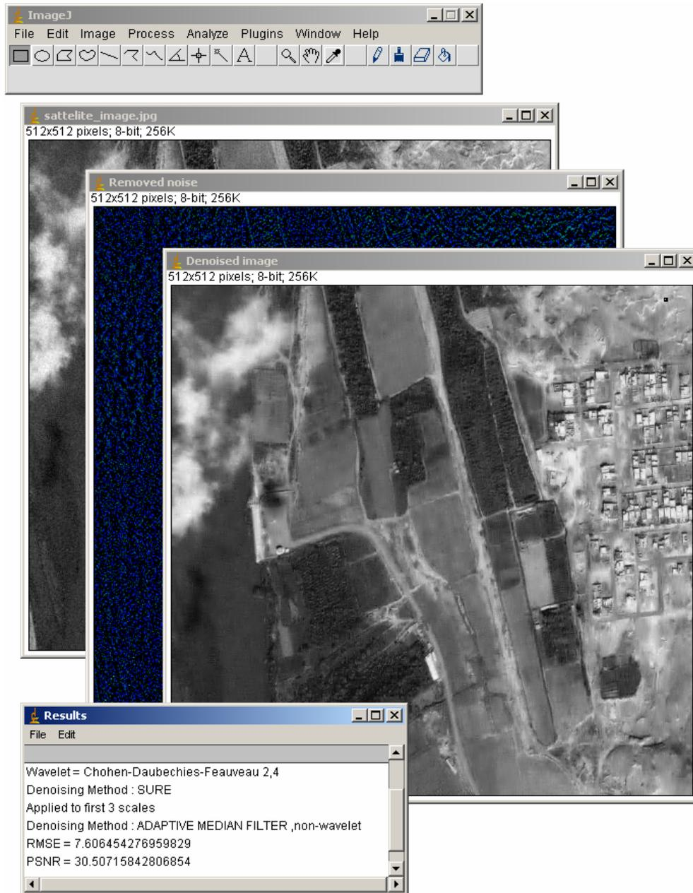
Figure 6-5 Result; noisy input image, removed noise, and denoised image with summary window
