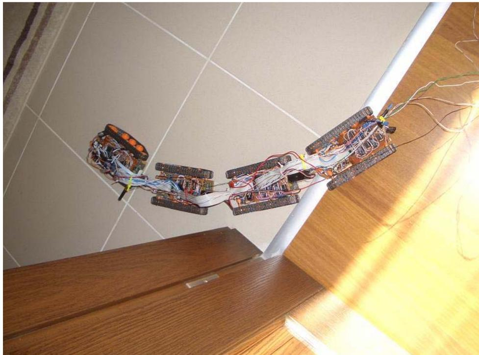
Figure 4.28. Accordion gait. The robot passes through the door way.
