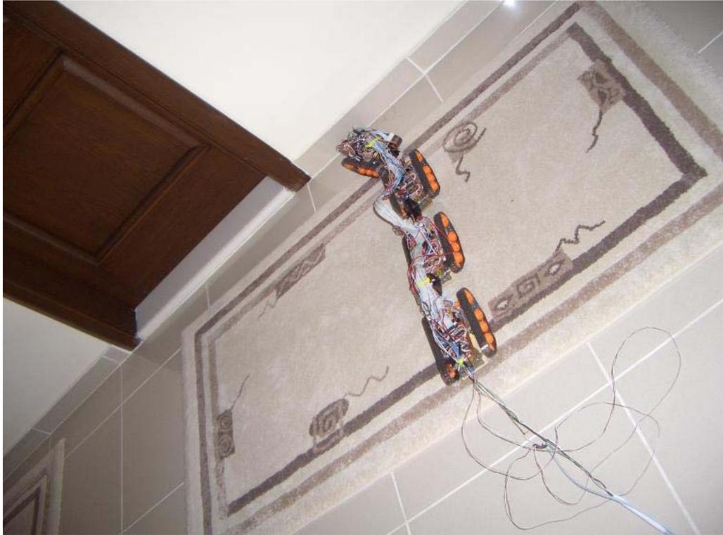
Figure 4.39. Lateral Undulation Gait with Obstacle Avoidance behavior. The robot crashes into the wall.
