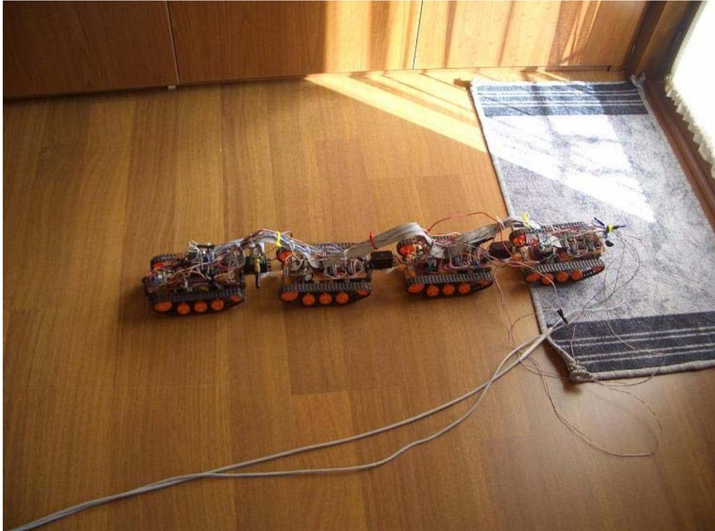
Figure 4.30. Lateral Undulation Gait without obstacle avoidance behavior.
