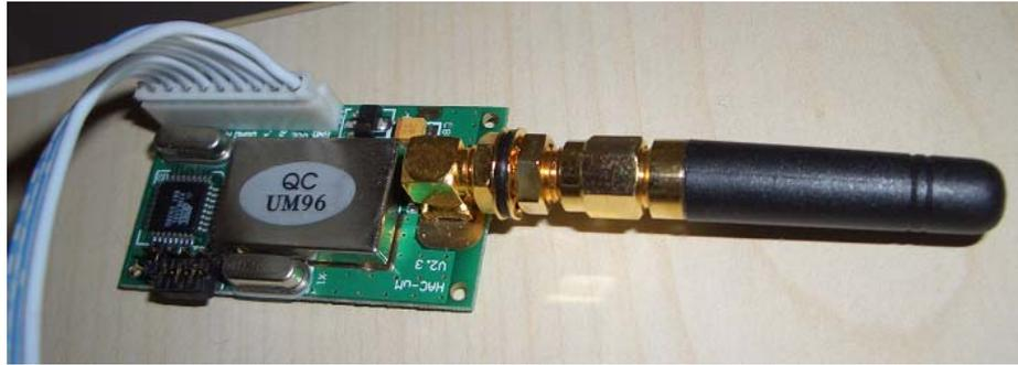
Figure 4.14. Half duplex RF modem.
