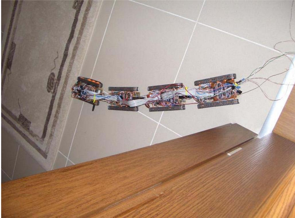
Figure 4.29. Accordion gait. The robot passes through the door way.
