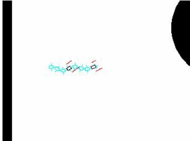
Figure 3.17. Sidewinding to left side. Segments having positive slope with respect to head position touch the ground.
