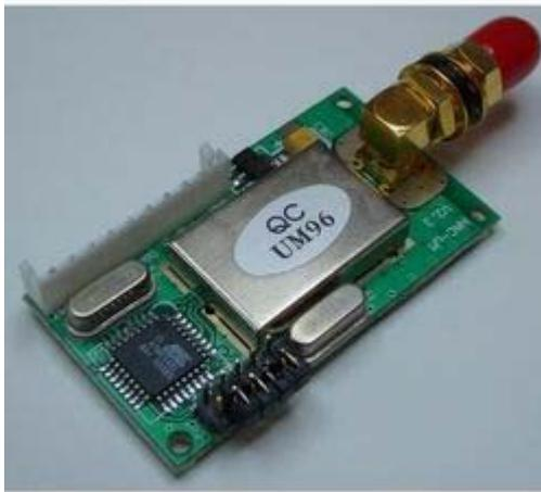
9600 baud half duplex serial connection.
