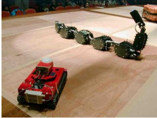
Figure 2.16. Kohga. CCD cameras are present in the tail and head. The tail and head joints are actively driven whereas the joints between the body segments are totally passive. But Kohga has sensors on passive joints to sense the body posture.
