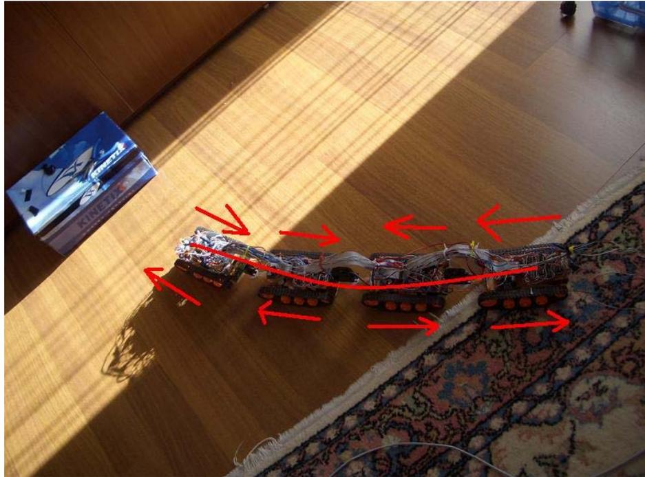
Figure 4.22. The steering of accordion gait. The joint servos are assisted by the palette motion indicated with red arrows.
