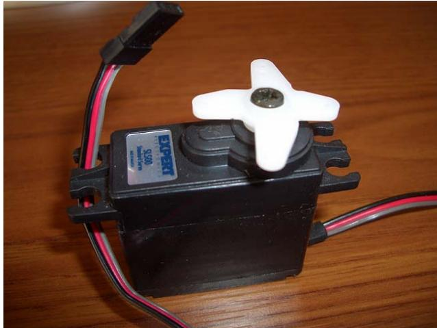
Figure 4.11. Servo used in joints.
