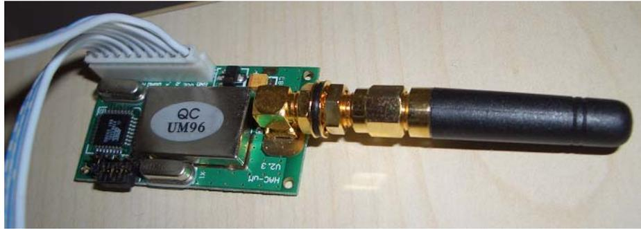
Figure 4.14. Half duplex RF modem.
