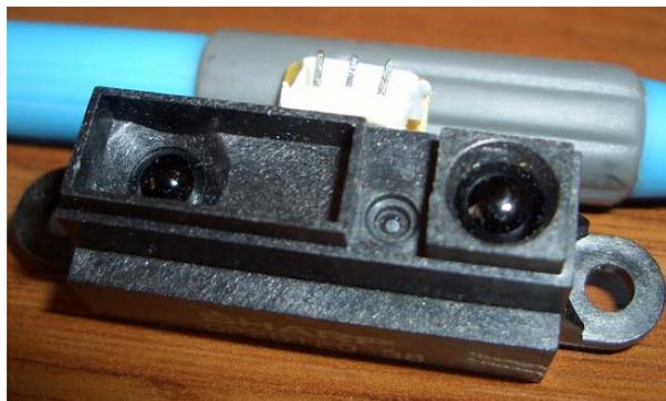
Figure 4.5. SHARP GP2D120 IR range sensor.
