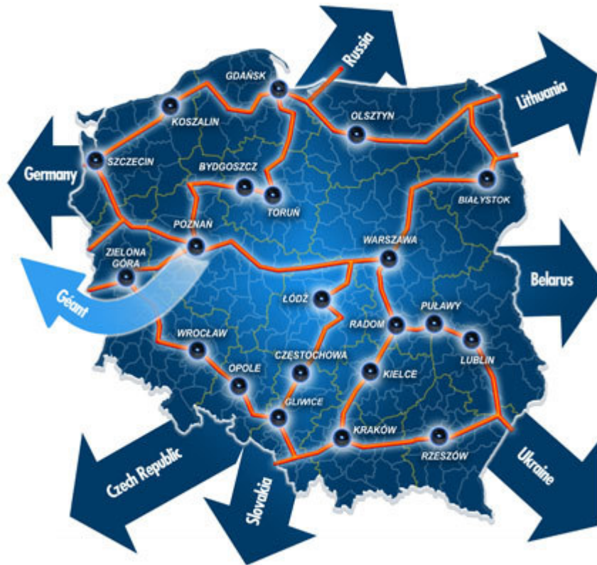
Figure 6: PIONEER fiber optic infrastructure ( http://www.pionier.gov.pl/network/index.htm , accessed Dec, 2006)
