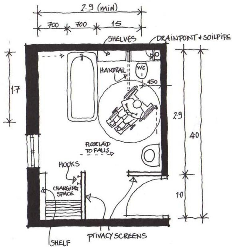
Figure B.16. Space data for an assisted bathroom.<sup>139</sup>
