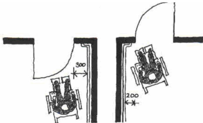
**Figure B.6. Negotiating door openings in a wheelchair.**<sup>129</sup>
