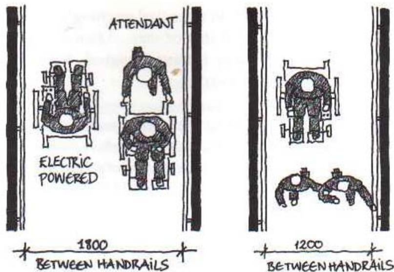
Figure B.1. Recommended widths of corridors for two-way and one-way traffic.<sup>124</sup>
