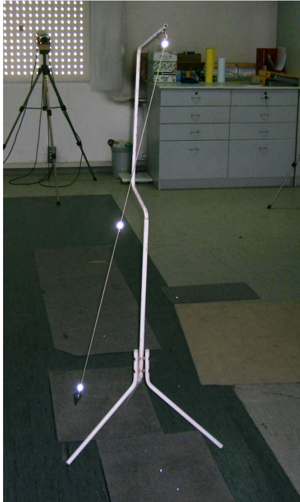
Figure 4.3 Pendulum assembly used to test the accuracy of the systems
