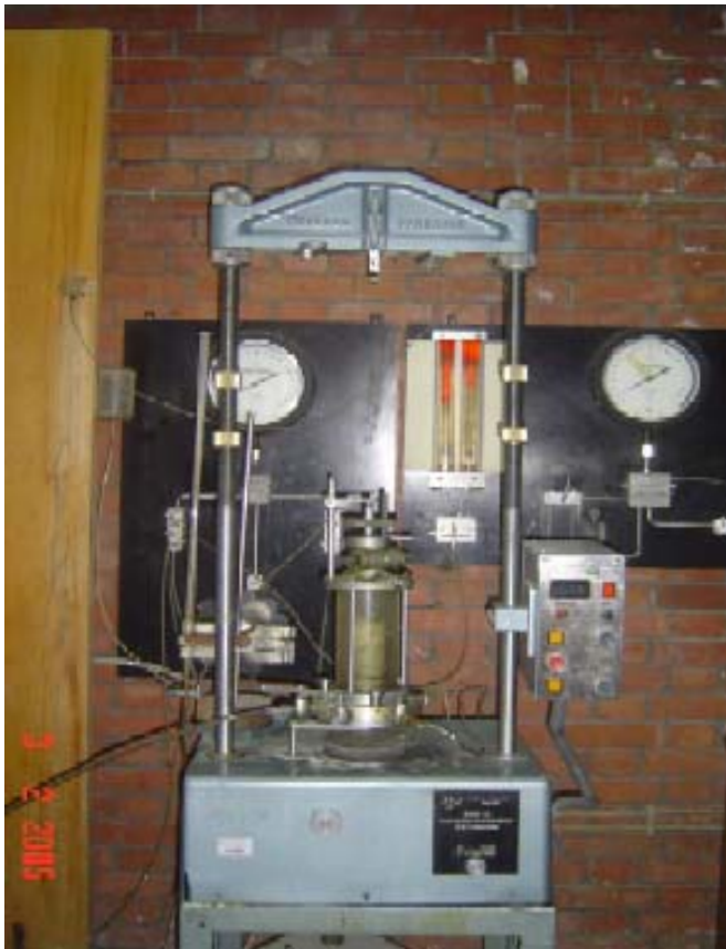
Figure 3.2 Saturated hydraulic conductivity test set up
