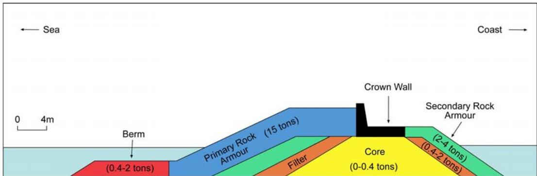
Figure 3.3 Primary breakwater cross-section of the Hisarönü ship shelter (after Çıkrıkçı, 2004)
