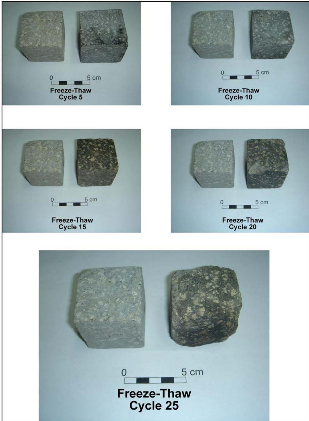
Figure 4.14 Physical appearances of the Çömlekçikuyu andesite during the freeze-thaw test. The sample on the left side of the photographs indicates a fresh reference sample.
