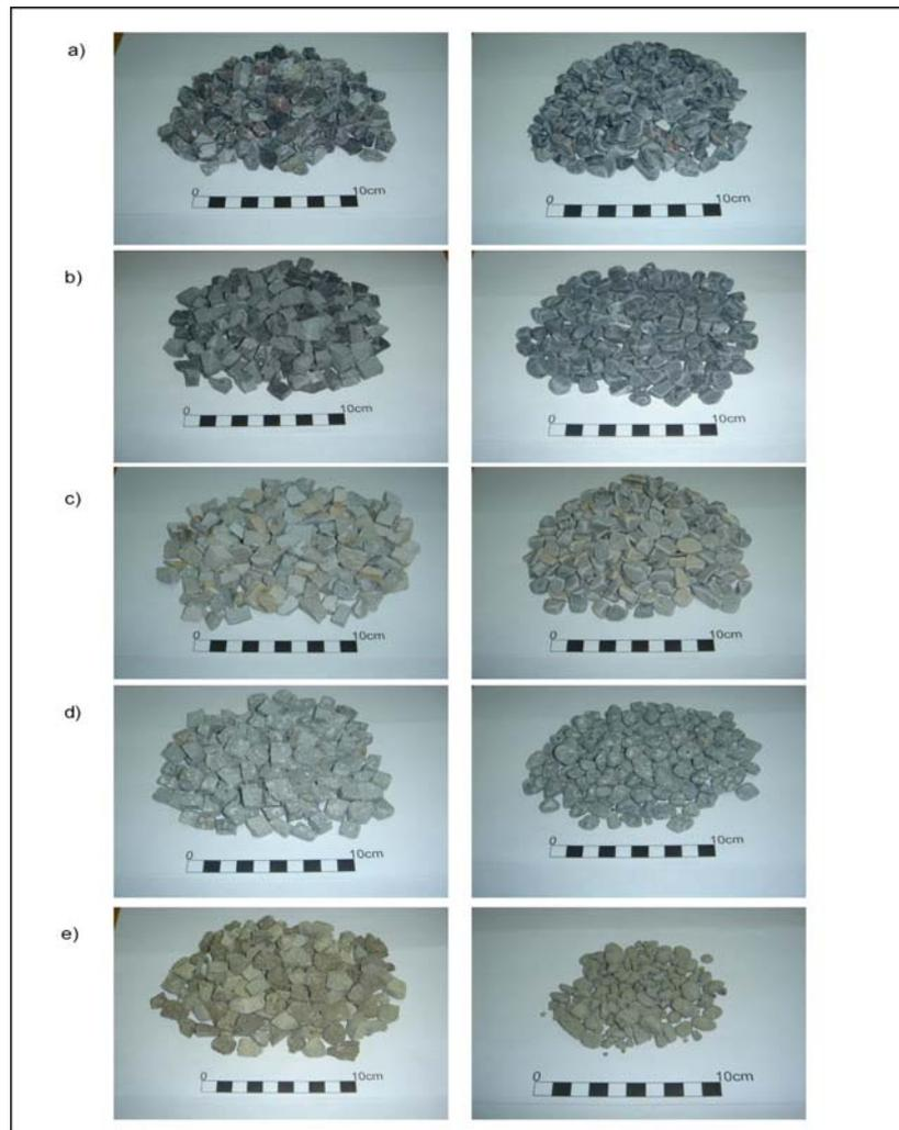
Figure 4.9 Physical changes of the samples after the micro-deval test. Fresh samples are given on the left. (a: Kavakdere limestone, b: Kavukkavlağı limestone, c: Tarlaağzı limestone, d: Çömlekçikuyu andesite, e: Kıran sandstone)
