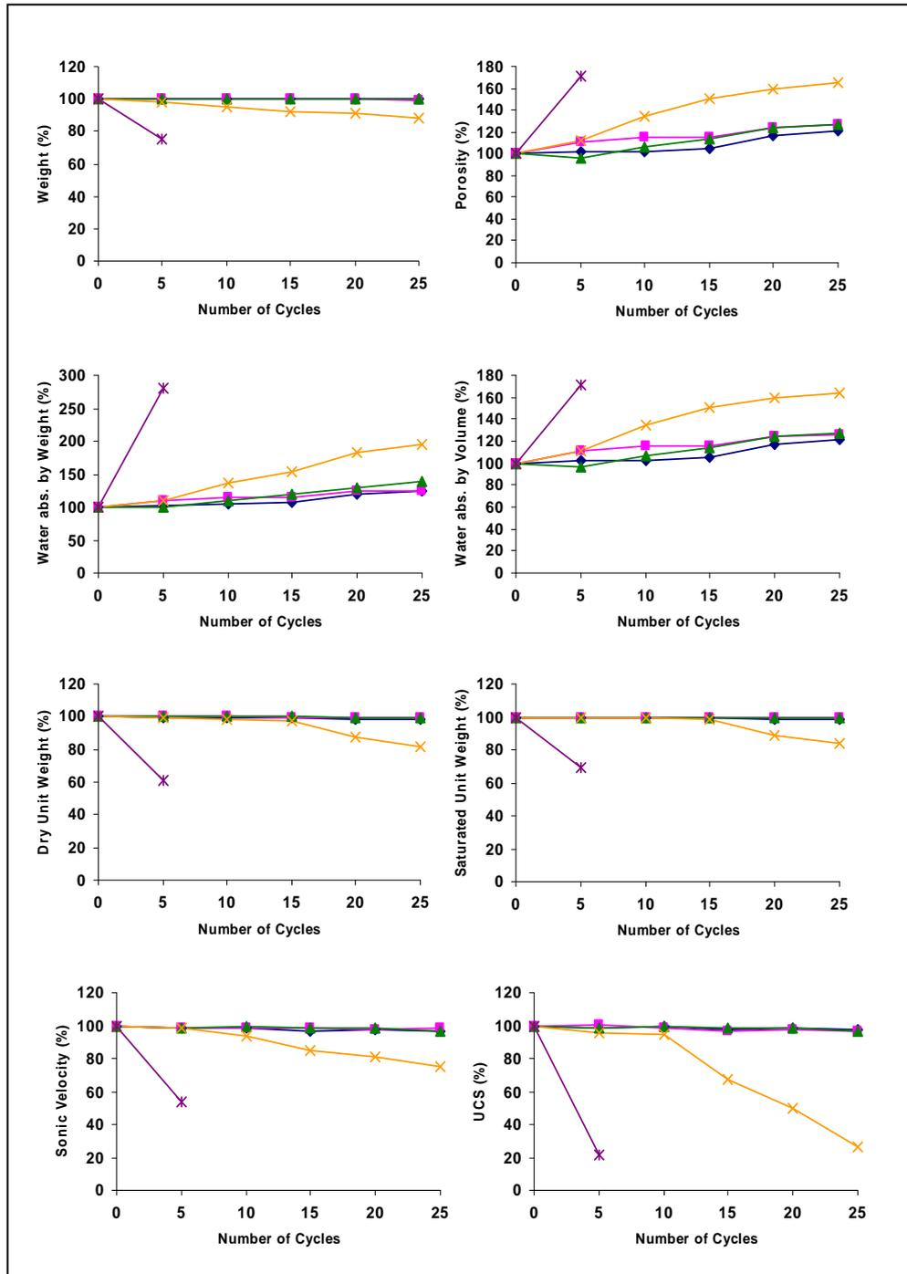
Figure 4.22 Variation of the physico-mechanical properties of the samples after magnesium sulphate soundness test (green line indicates the Kavakdere limestone, pink line indicates the Kavukkavlağı limestone, blue line indicates the Tarlaağı limestone, orange line indicates the Çömlekçikuyu andesite, and purple line indicates the Kıran sandstone)
