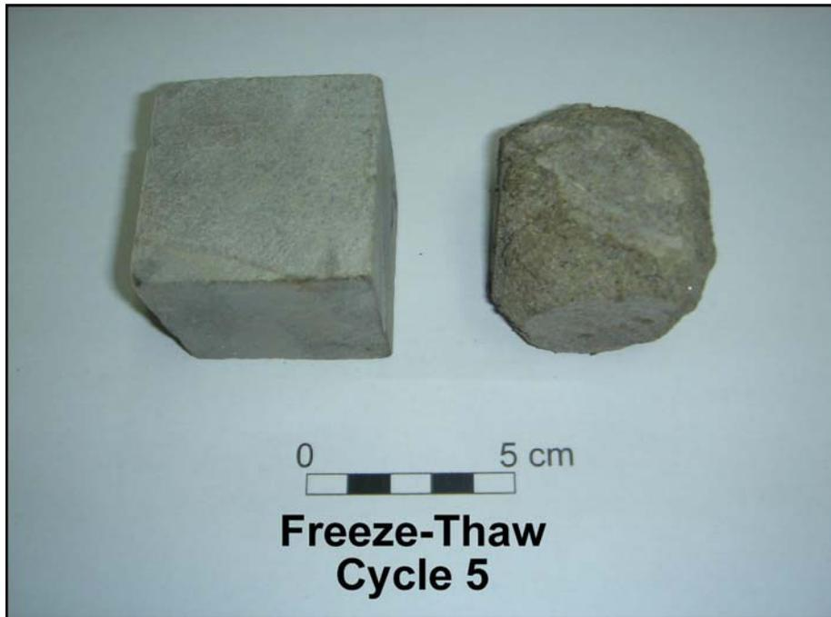
Figure 4.15 Physical appearance of the Kiran sandstone during the freeze-thaw test. The sample on the left side of the photographs indicates a fresh reference sample
