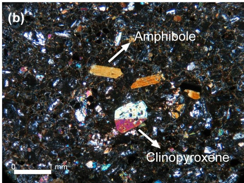
Figure 2.8 Photomicrographs of the Kiran sandstone (a) plane polarized light (PPL) x5, (b) cross polarized light (CPL) x5
