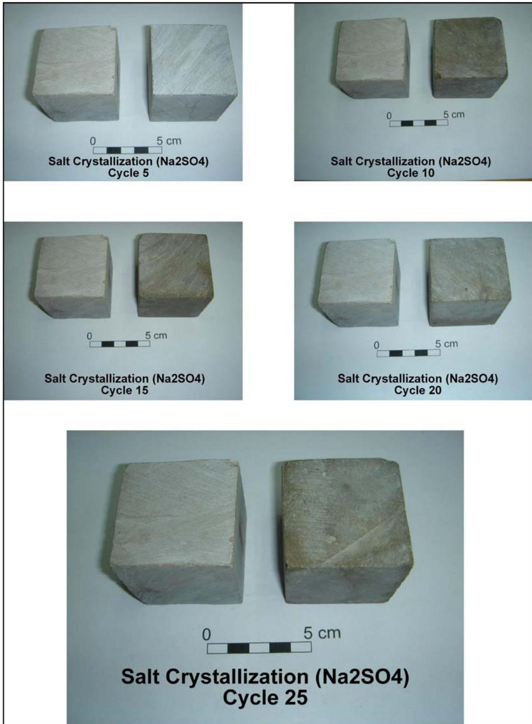
Figure 4.31 Physical appearances of the Tarlaağzı limestone during the sodium sulphate soundness test. The sample on the left side of the photographs indicates a fresh reference sample
