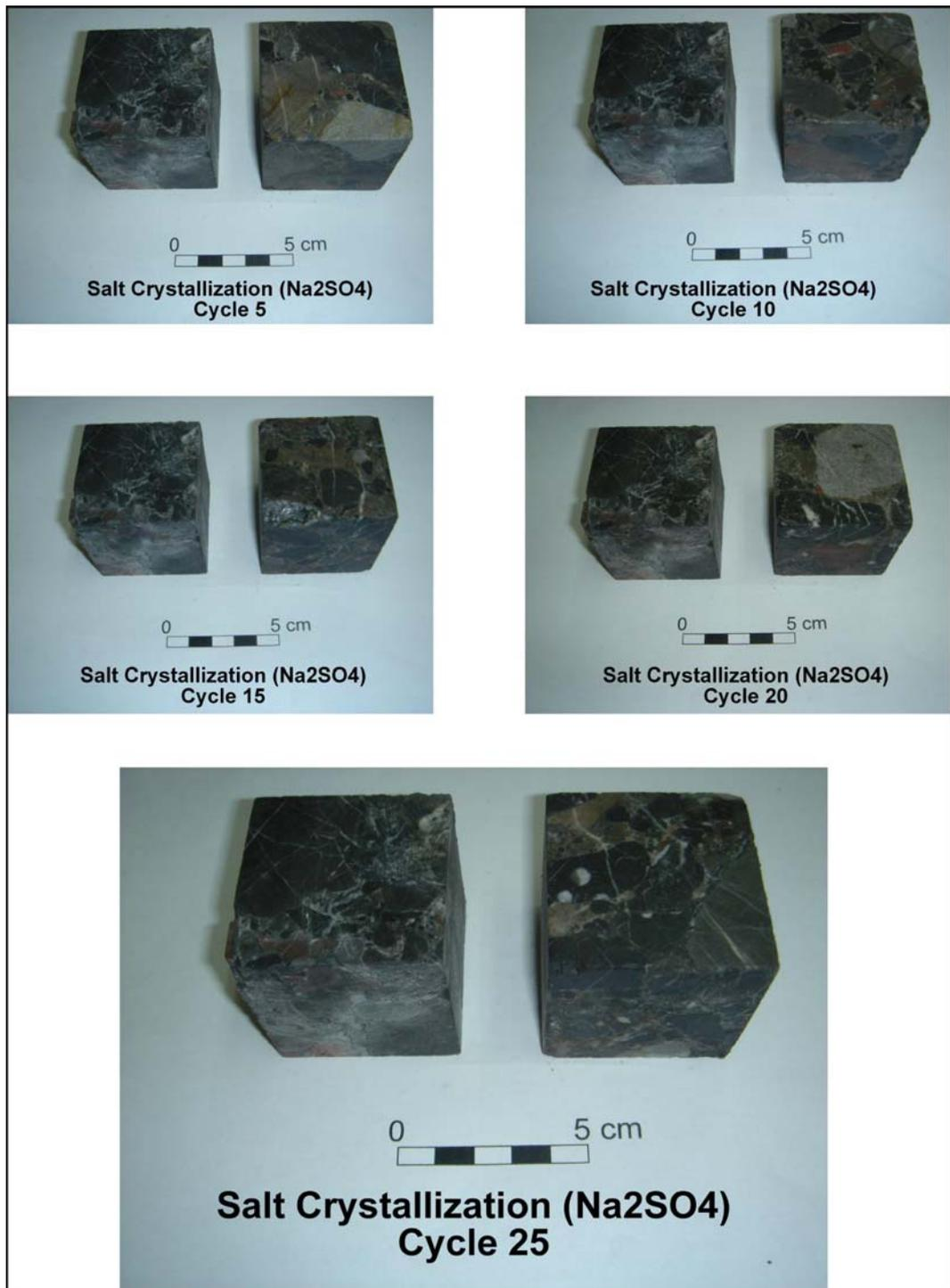
Figure 4.29 Physical appearances of the Kavakdere limestone during the sodium sulphate soundness test. The sample on the left side of the photographs indicates a fresh reference sample
