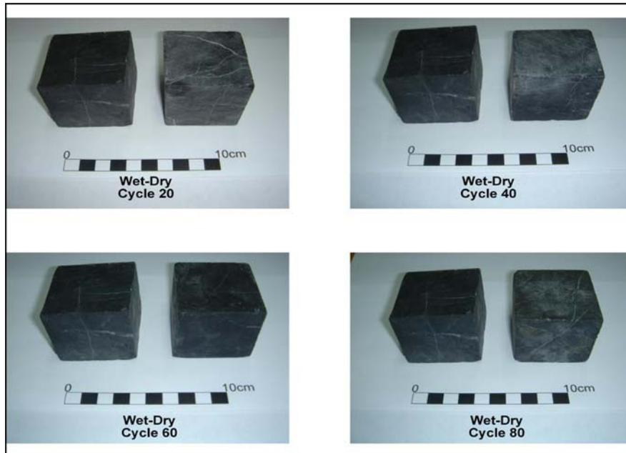
Figure 4.18 Physical appearances of the Kavukkavlağı limestone during the wetting-drying test. The sample on the left side of the photographs indicates a fresh reference sample
