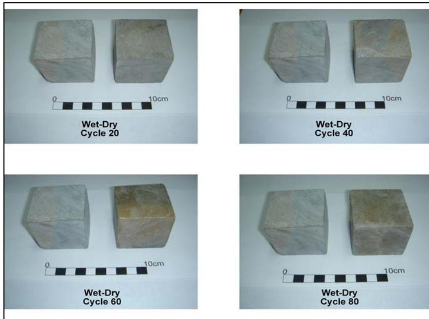
Figure 4.19 Physical appearances of the Tarlaağzı limestone during the wetting-drying test. The sample on the left side of the photographs indicates a fresh reference sample
