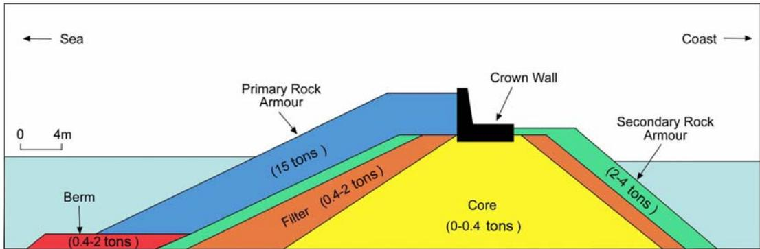
Figure 3.2 Primary breakwater cross-section of the Tarlağzı ship shelter (after Bağcı, 1995)
