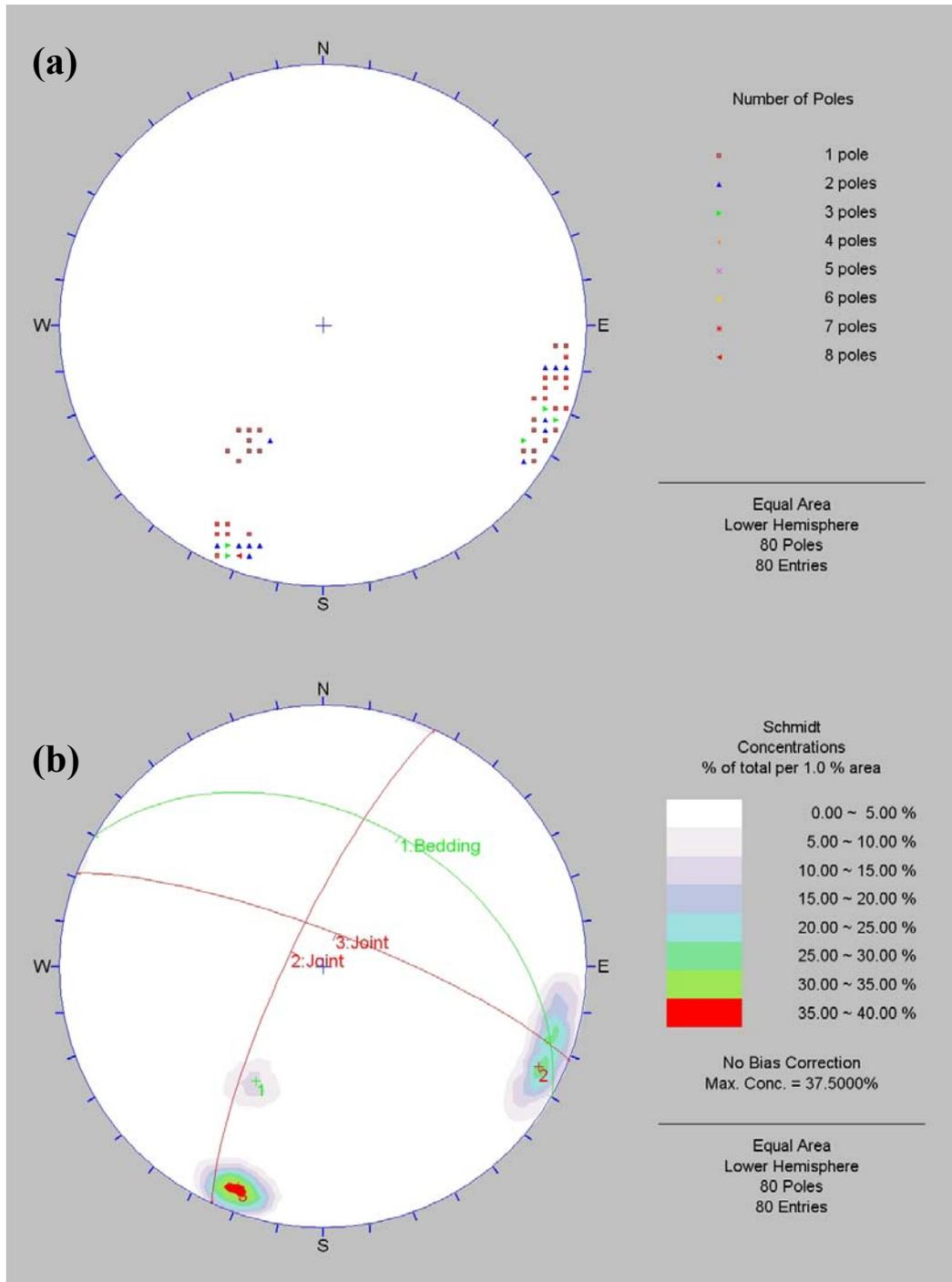
Figure 4.39 Pole plot (a) and contour plot (b) of the discontinuities in the Kavakdere quarry
