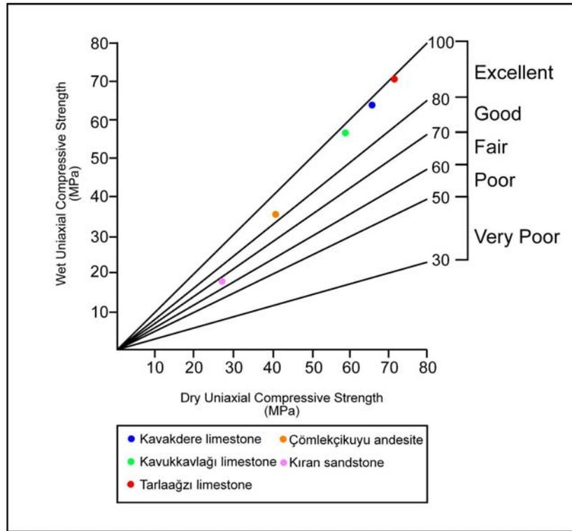
Figure 5.1 Durability evaluations of the samples based on the wet-to-dry strength ratio (after Winkler, 1986).
