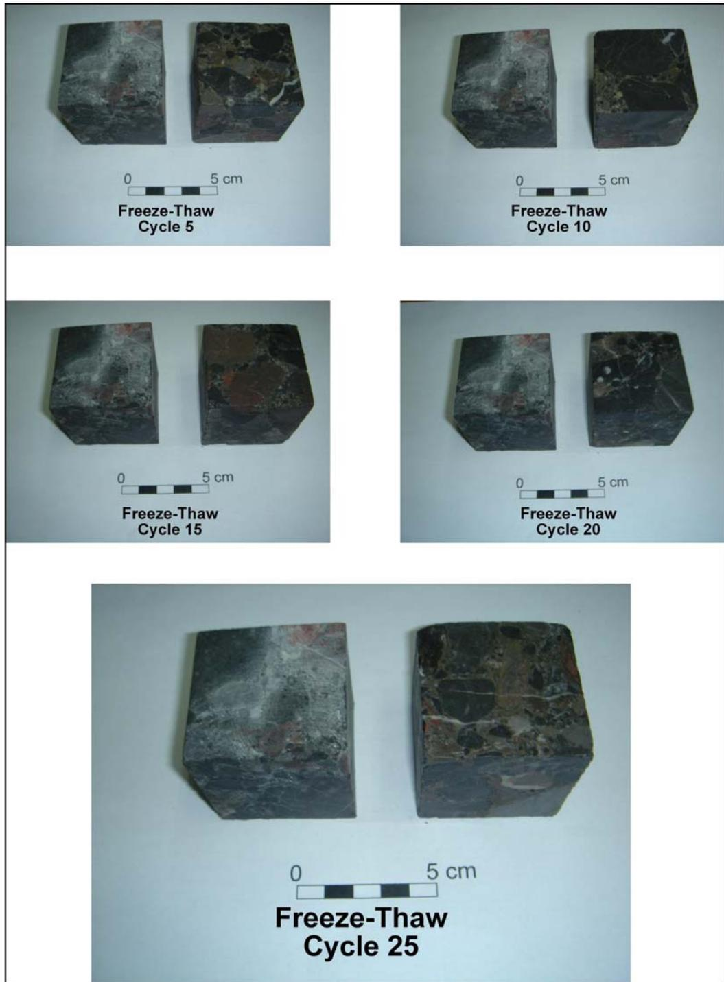
Figure 4.11 Physical appearances of the Kavakdere limestone during the freeze-thaw test. The sample on the left side of the photographs indicates a fresh reference sample.
