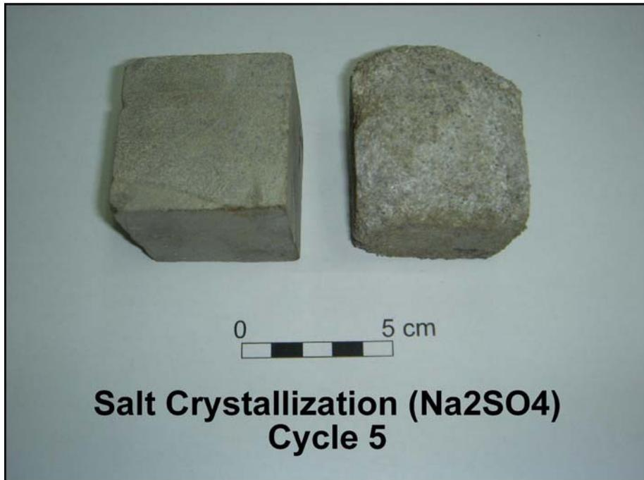
Figure 4.33 Physical appearance of the Kiran sandstone during the sodium sulphate soundness test. The sample on the left side of the photographs indicates a fresh reference sample
