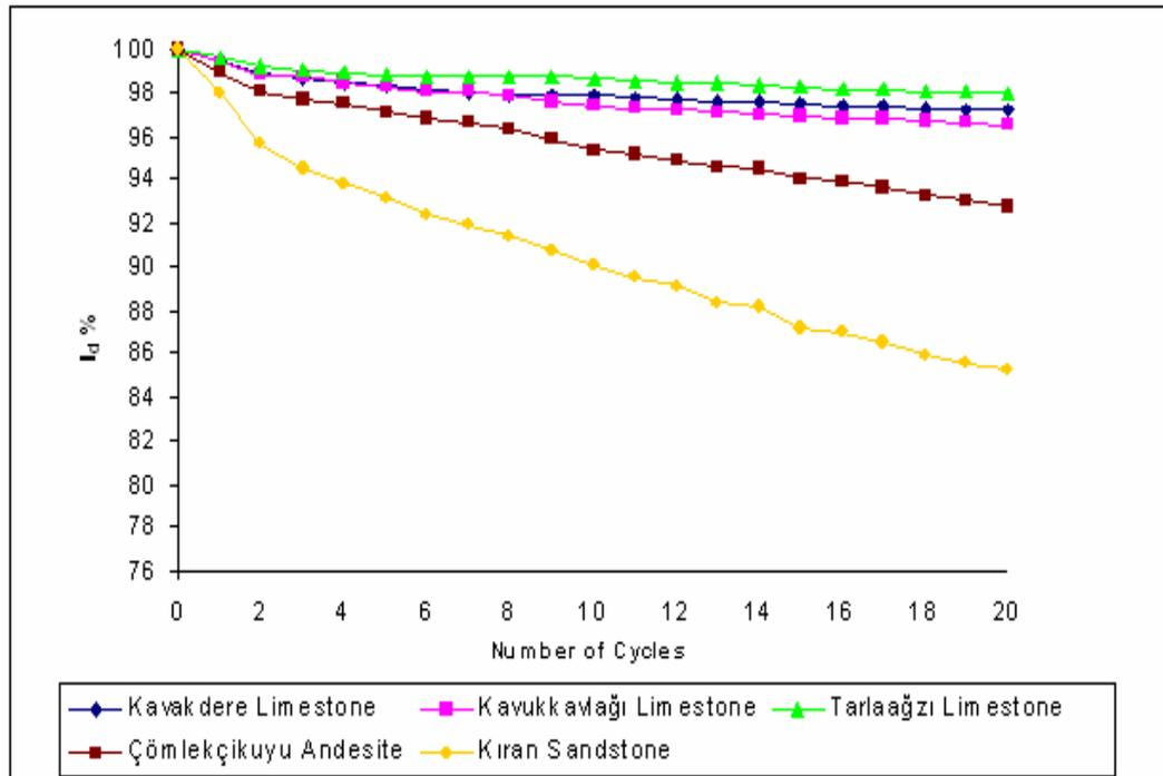
Figure 4.8 The variation of slake durability indexes of the samples for 20 test cycles.
