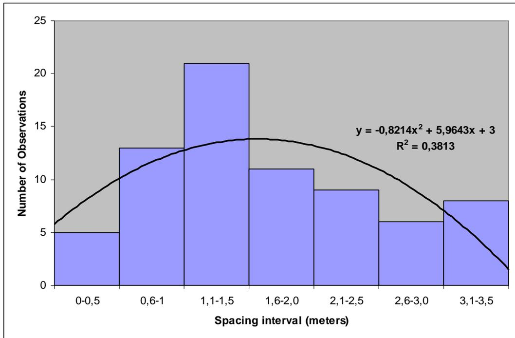
Figure 4.44 Distributions of the joint spacing in the Kavakdere quarry
