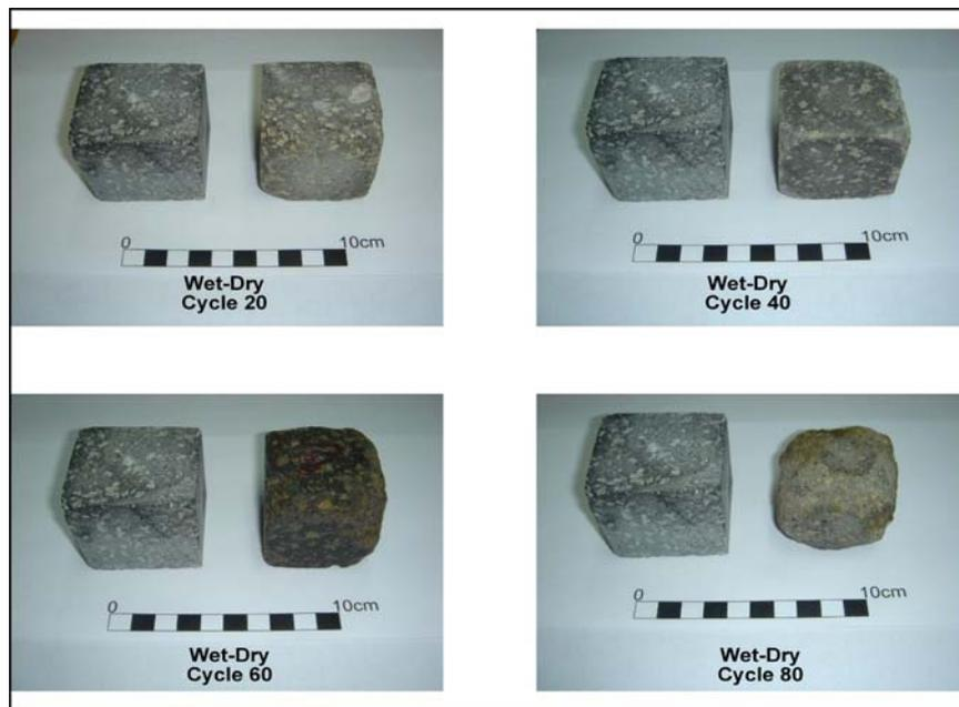
Figure 4.20 Physical appearances of the Çömlekçikuyu andesite during the wetting-drying test. The sample on the left side of the photographs indicates a fresh reference sample
