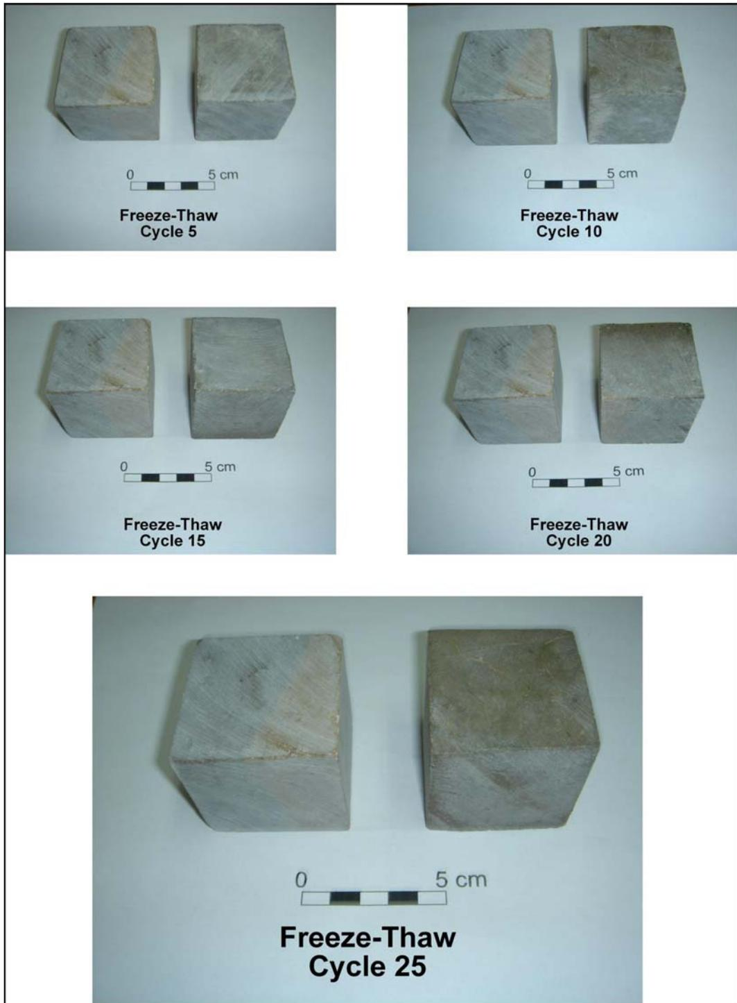
Figure 4.13 Physical appearances of the Tarlaağzı limestone during the freeze-thaw test. The sample on the left side of the photographs indicates a fresh reference sample.
