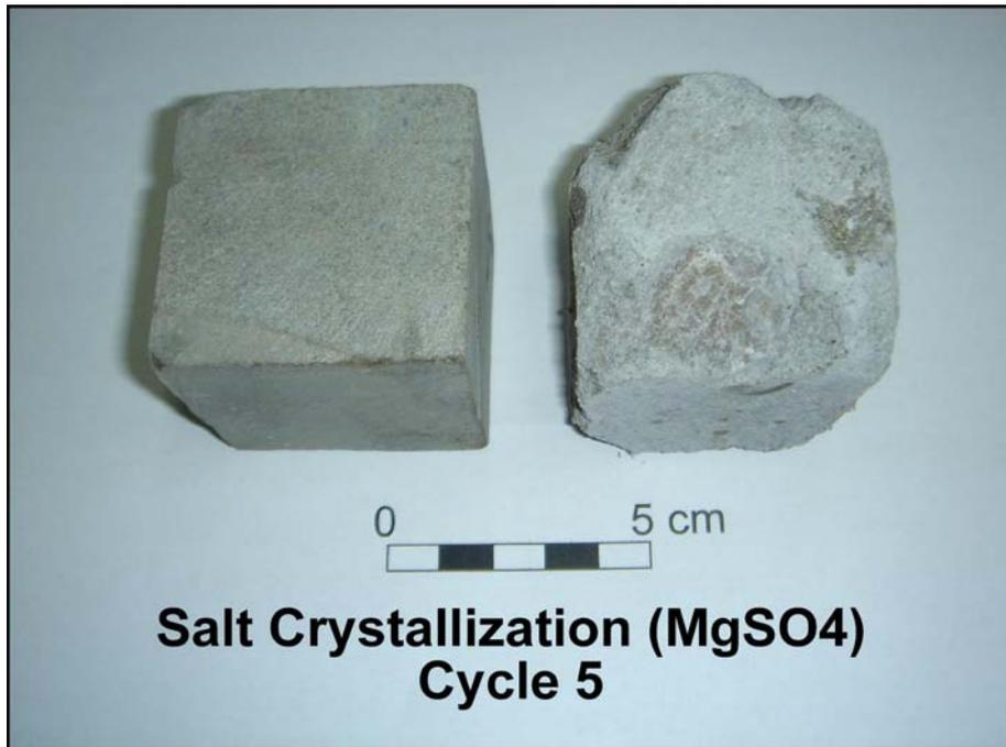
Figure 4.27 Physical appearance of the Kiran sandstone during the magnesium sulphate soundness test. The sample on the left side of the photographs indicates a fresh reference sample
