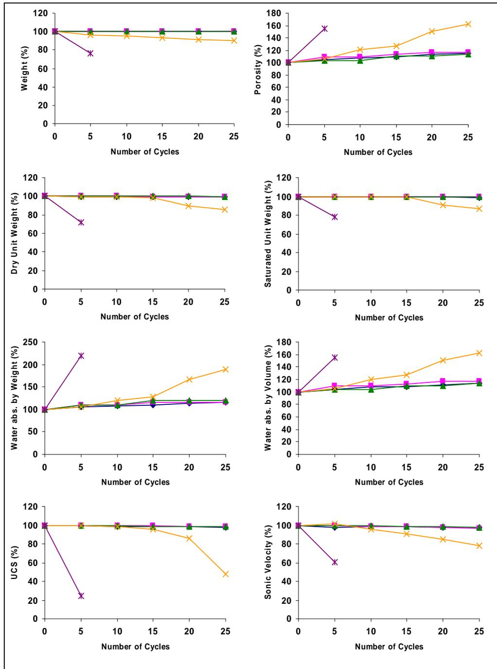
Figure 4.28 Variation of the physico-mechanical properties of the samples after sodium sulphate soundness test (green line indicates the Kavakdere limestone, pink line indicates the Kavukkavlağı limestone, blue line indicates the Tarlağı limestone, orange line indicates the Çömlekçikuyu andesite and purple line indicates the Kıran sandstone)
