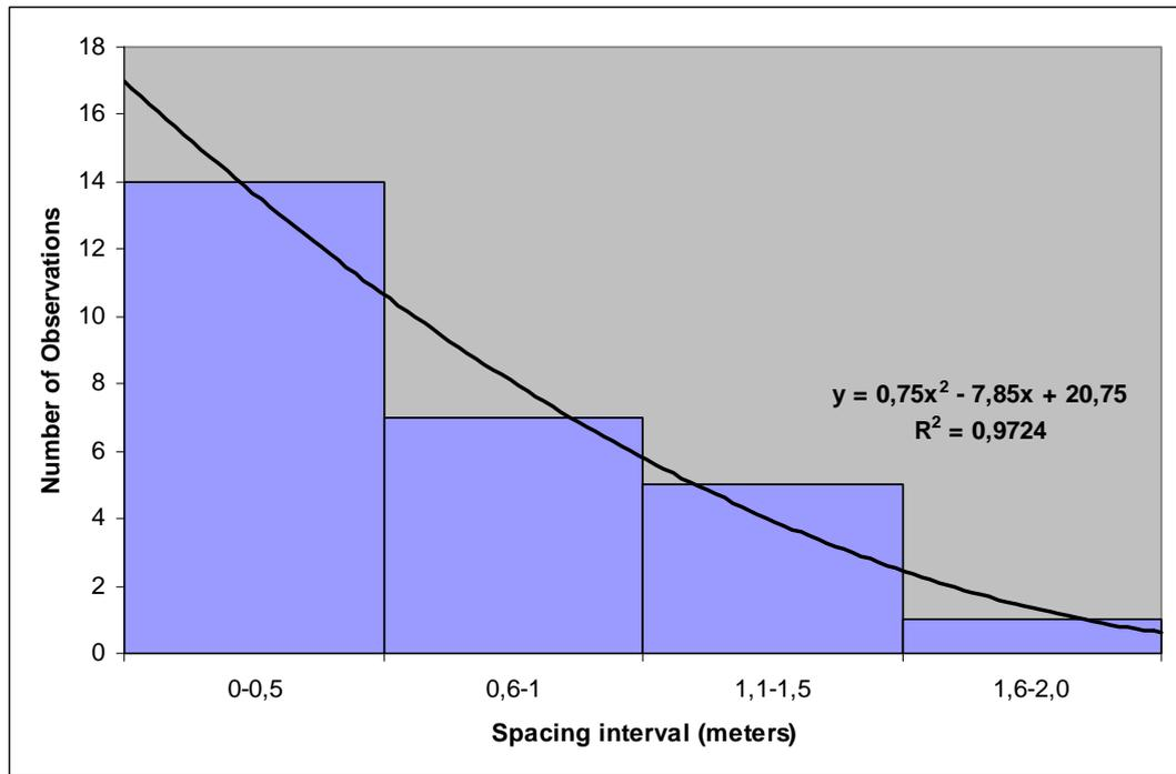
Figure 4.48 Distributions of the joint spacing in the Tarlaağzı quarry
