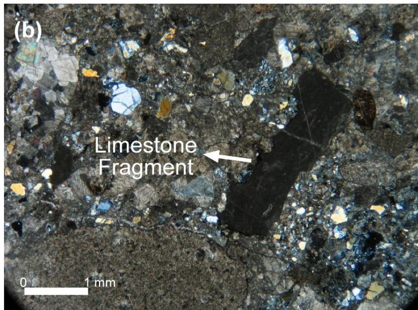
Figure 2.3 Photomicrographs of the Kavakdere limestone (a) plane polarized light (PPL) x5, (b) cross polarized light (CPL) x5
