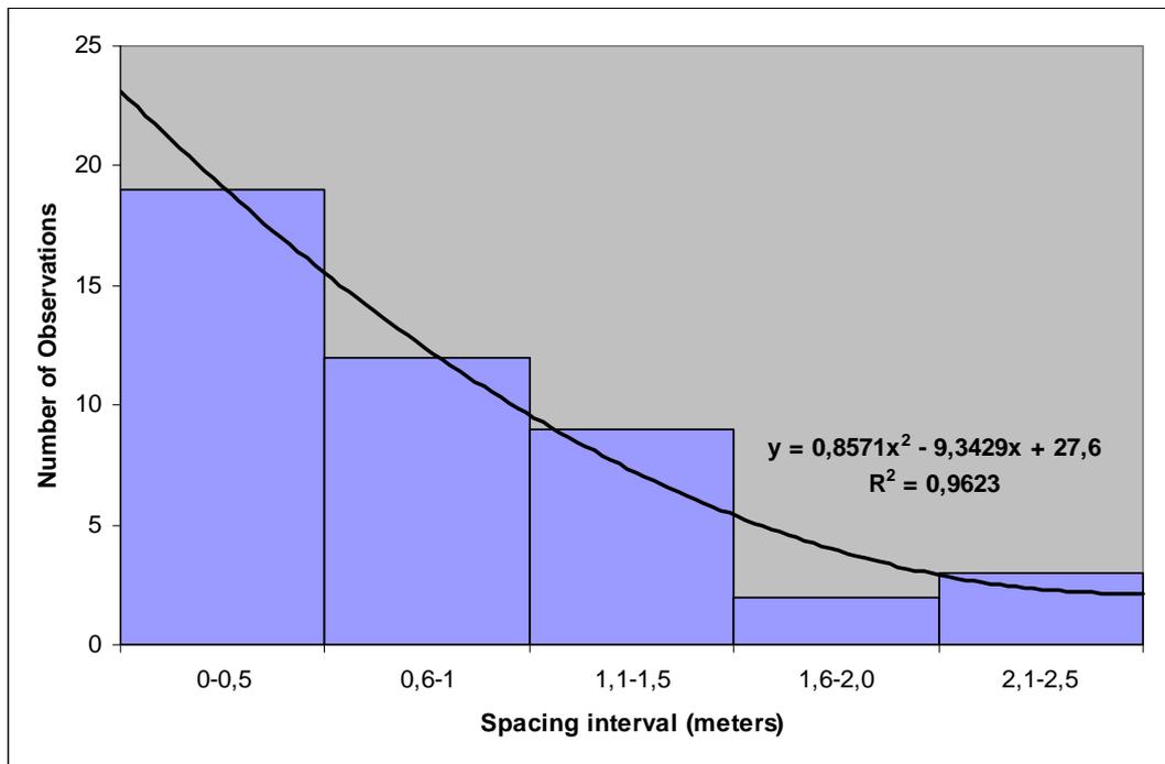
Figure 4.45 Distributions of the joint spacing in the Kavukkavlağı quarry
