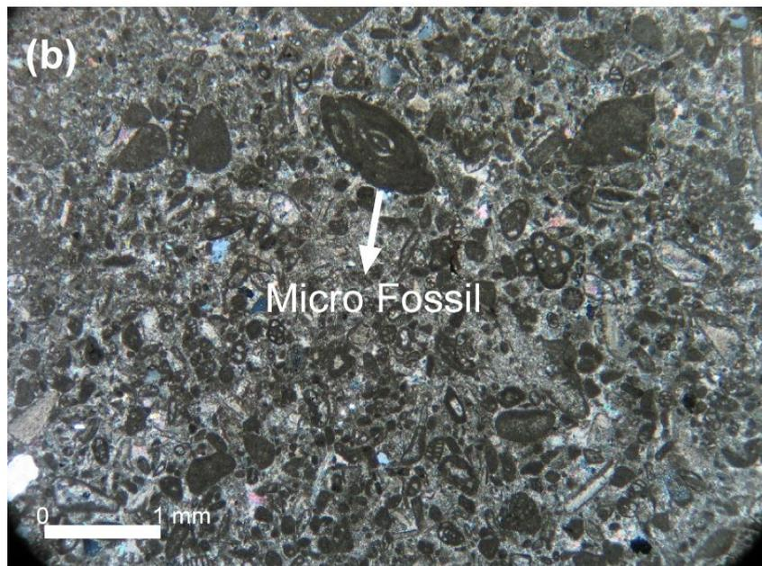
Figure 2.13 Photomicrographs of the Tarlaağzı limestone (a) plane polarized light (PPL) x5, (b) cross polarized light (CPL) x5
