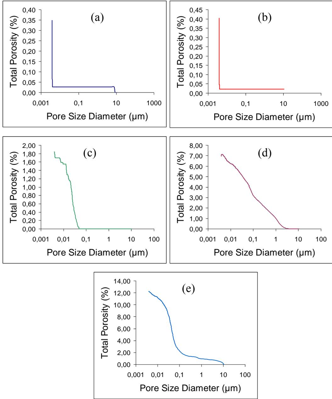
Figure 4.1 Cumulative intrusion curves of the samples (a) Kavakdere limestone (b) Kavukkavlağı limestone (c) Tarlaağı Limestone (d) Çömlekçikuyu andesite (e) Kıran sandstone
