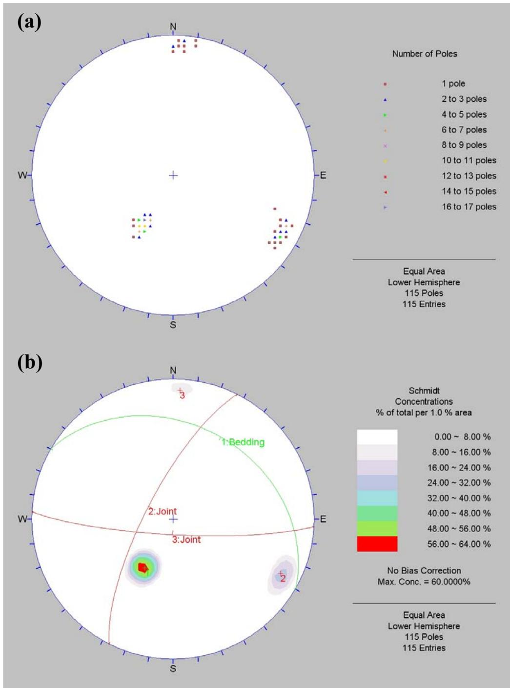
Figure 4.40 Pole plot (a) and contour plot (b) of the discontinuities in the Kavukkavlağı quarry
