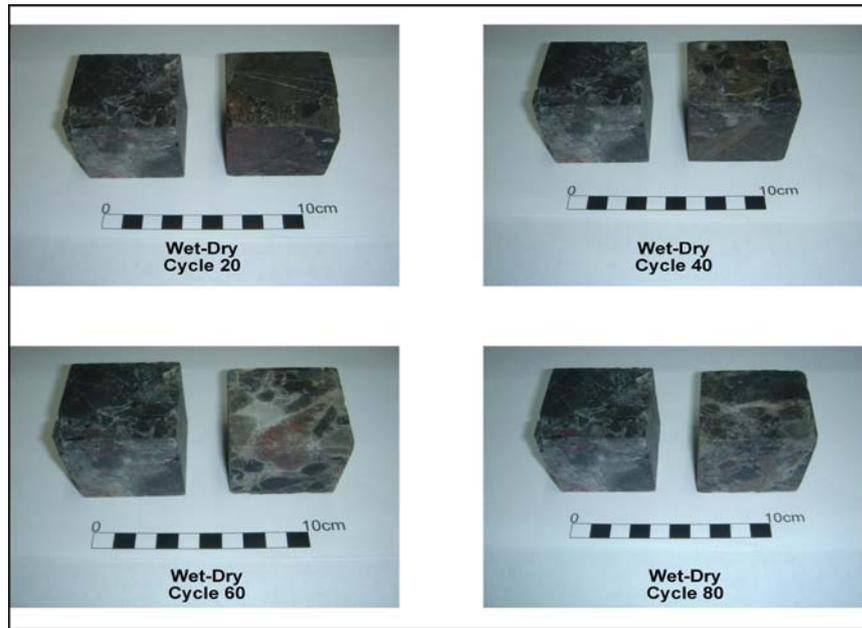
Figure 4.17 Physical appearances of the Kavakdere limestone during the wetting-drying test. The sample on the left side of the photographs indicates a fresh reference sample
