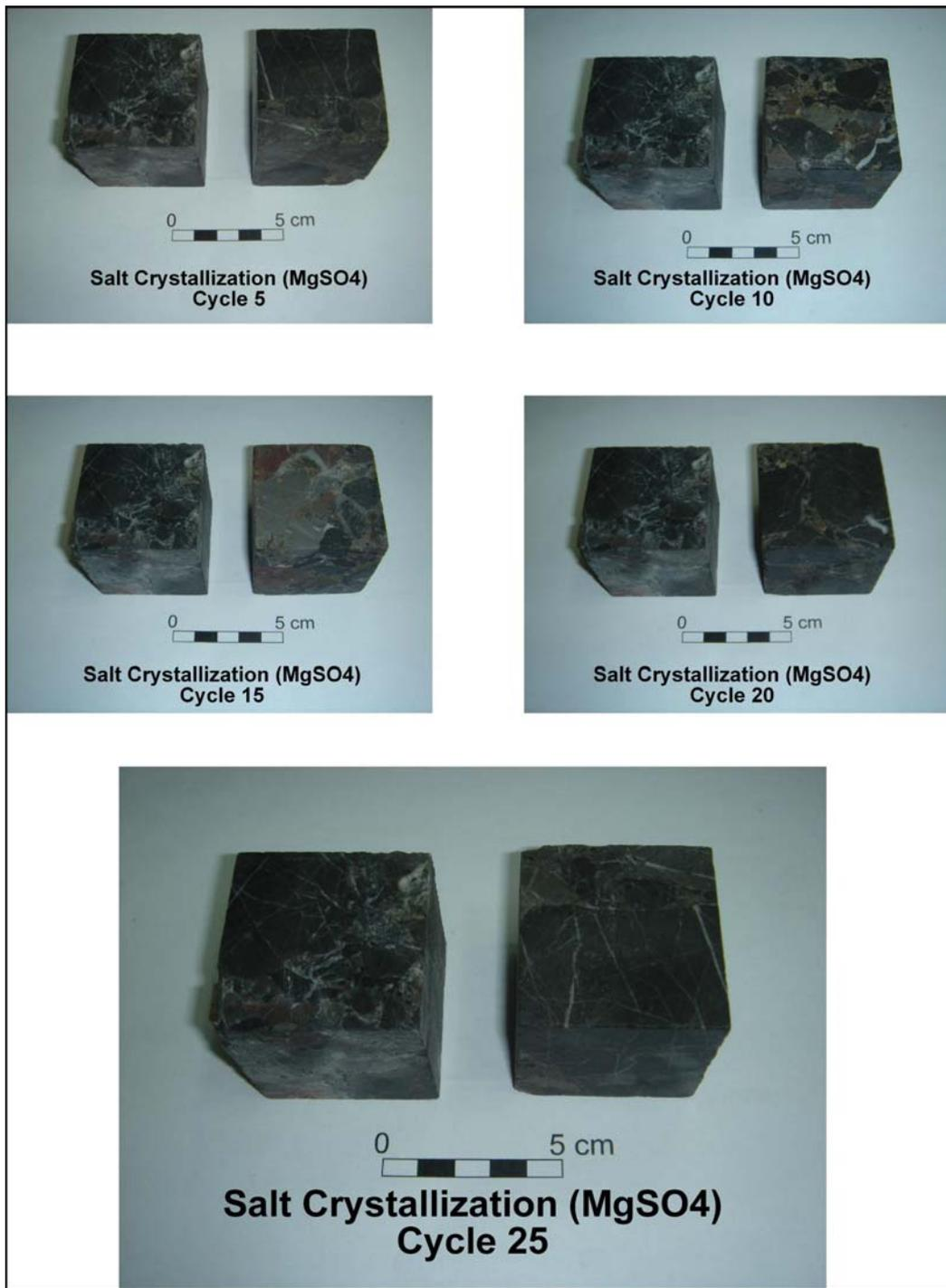
Figure 4.23 Physical appearances of the Kavakdere limestone during the magnesium sulphate soundness test. The sample on the left side of the photographs indicates a fresh reference sample
