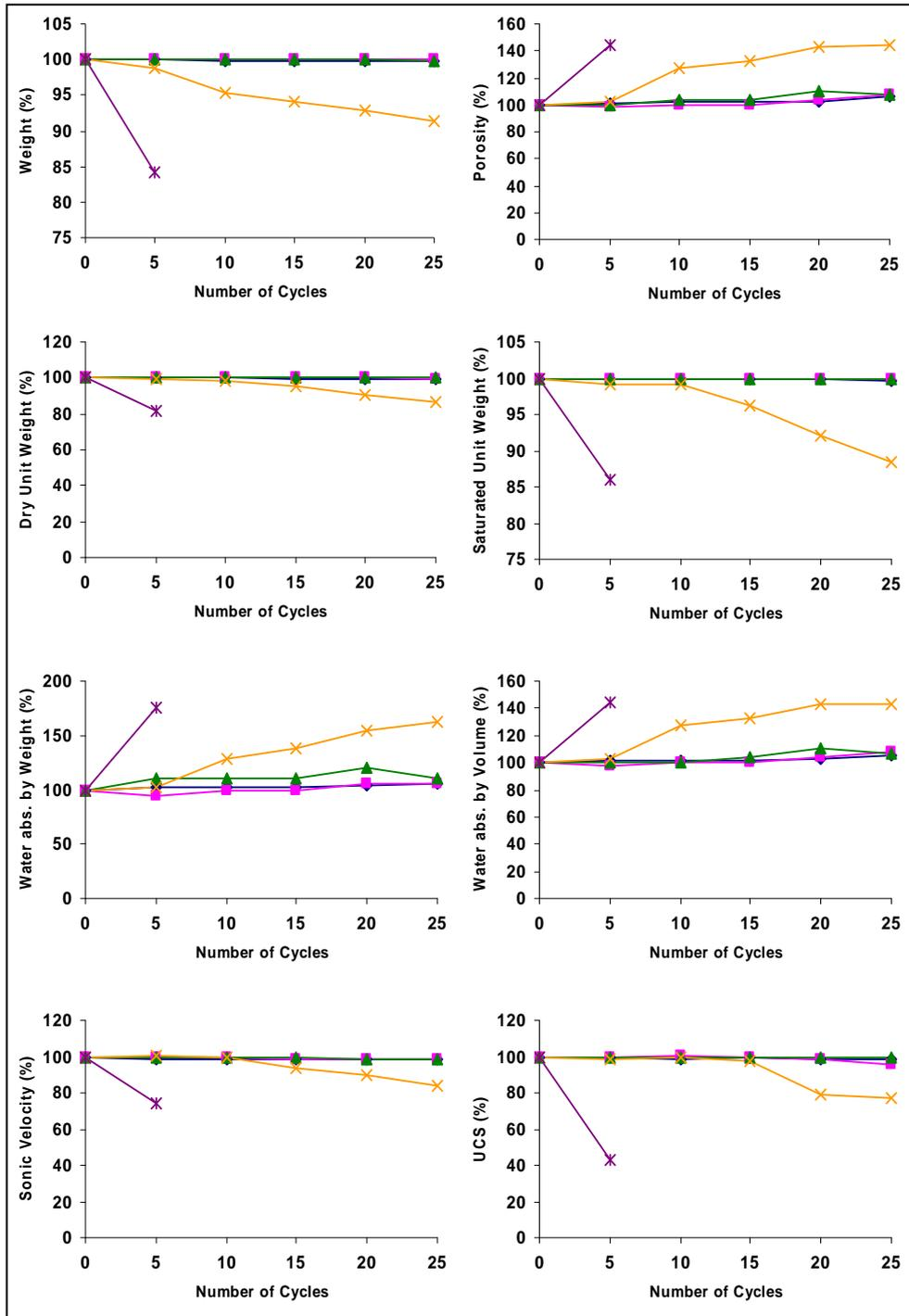
Figure 4.10 Variation of the physico-mechanical properties of the samples after freeze-thaw test (green line indicates the Kavakdere limestone, pink line indicates the Kavukkavlağı limestone, blue line indicates the Tarlağzı limestone, orange line indicates the Çömlekçikuyu andesite and purple line indicates the Kıran sandstone)
