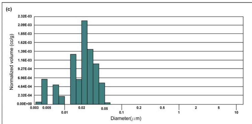
Figure 4.2 Pore size distributions of the samples (a) Kavakdere limestone (b) Kavukkavlağı limestone (c) Tarlaağı Limestone
