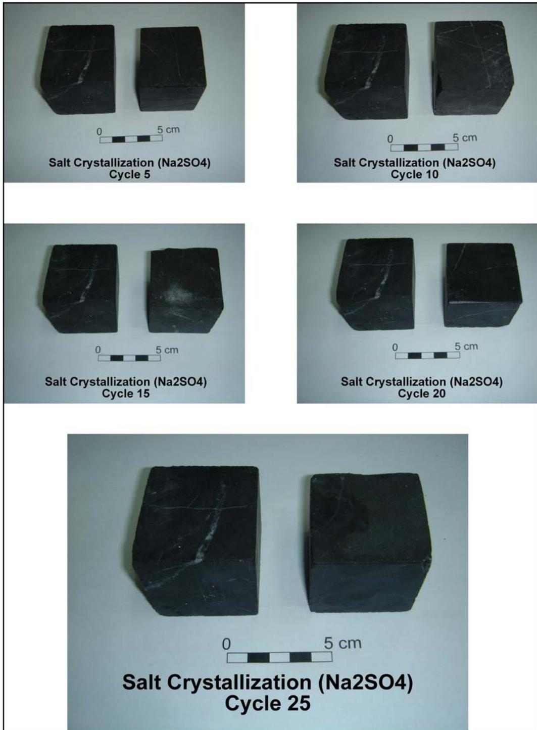
Figure 4.30 Physical appearances of the Kavukkavlađı limestone during the sodium sulphate soundness test. The sample on the left side of the photographs indicates a fresh reference sample
