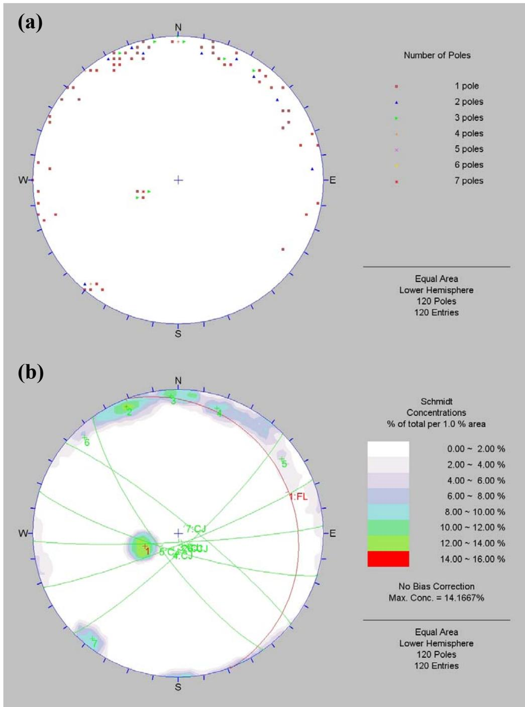
Figure 4.42 Pole plot (a) and contour plot (b) of the discontinuities in the Çömlekçikuyu quarry
