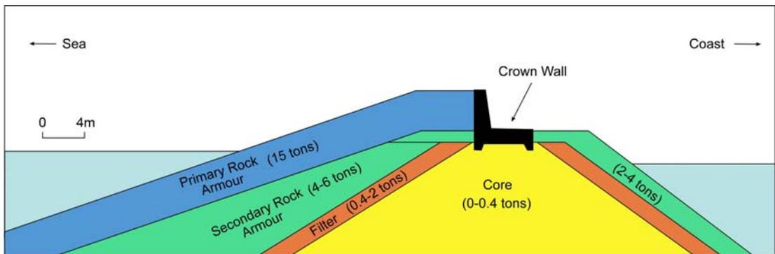
Figure 3.4 Primary breakwater cross-section of the Alaplı ship shelter (after İnan, 1995)
