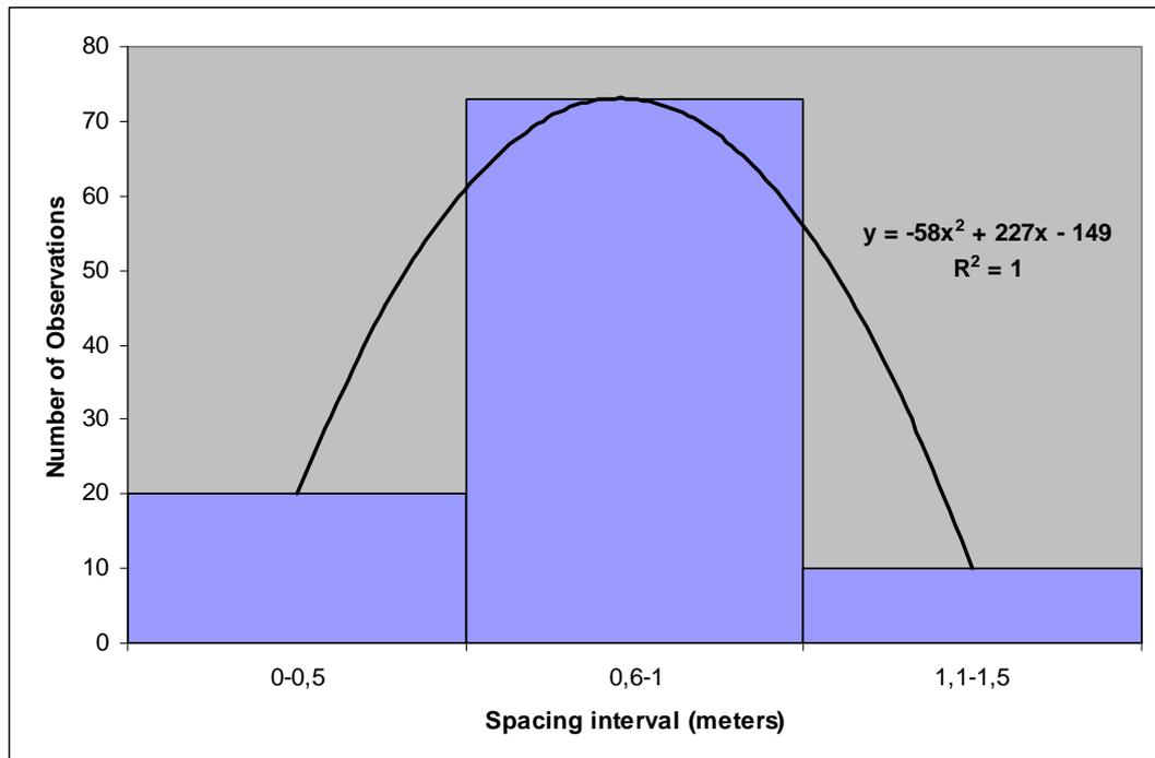
Figure 4.47 Distributions of the joint spacing in the Çömlekçikuyu quarry
