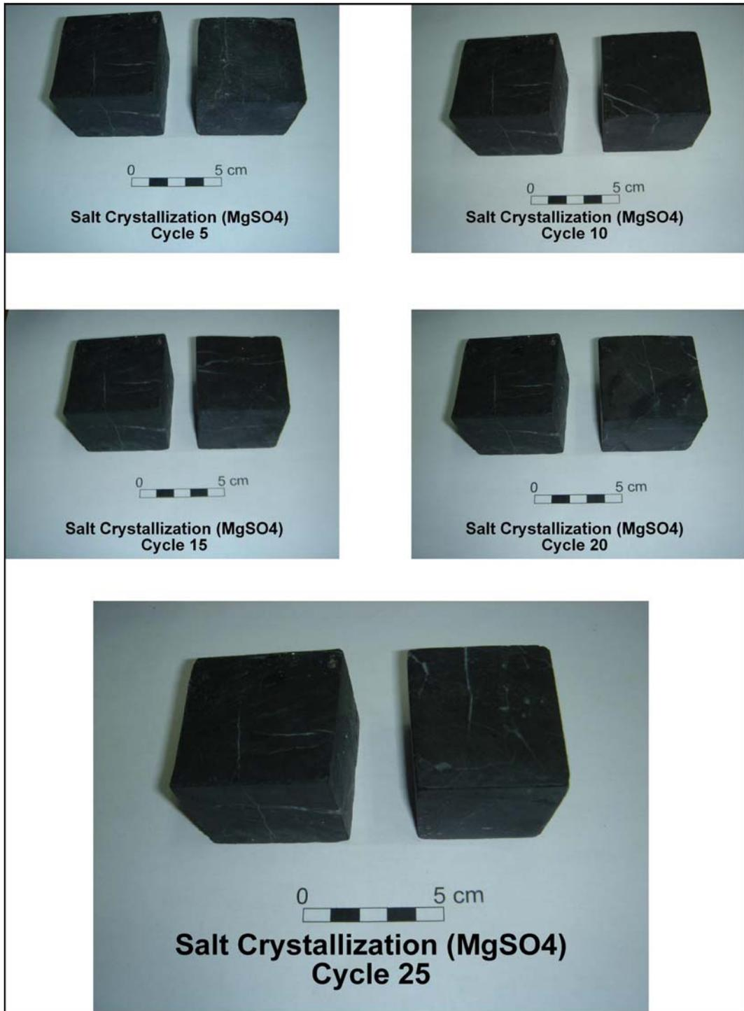
Figure 4.24 Physical appearances of the Kavukkavlađı limestone during the magnesium sulphate soundness test. The sample on the left side of the photographs indicates a fresh reference sample
