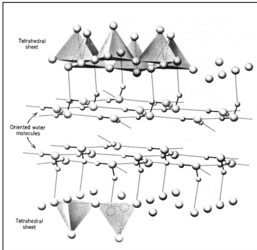
Figure 4.4 Diagrammatic sketch of the smectite group clay minerals, showing layers of water (after Grim, 1968)
