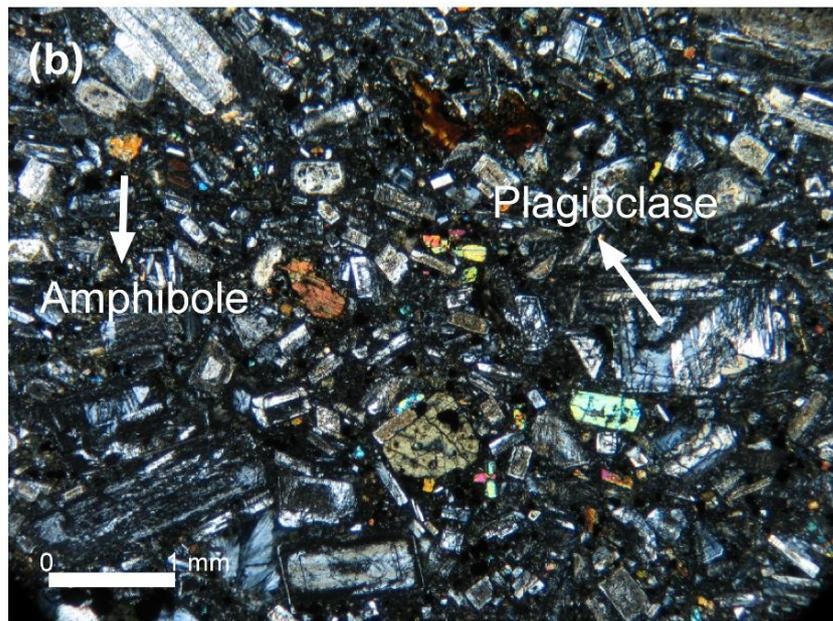
Figure 2.10 Photomicrographs of the Çömlekçikuyu andesite (a) plane polarized light (PPL) x5, (b) cross polarized light (CPL) x5
