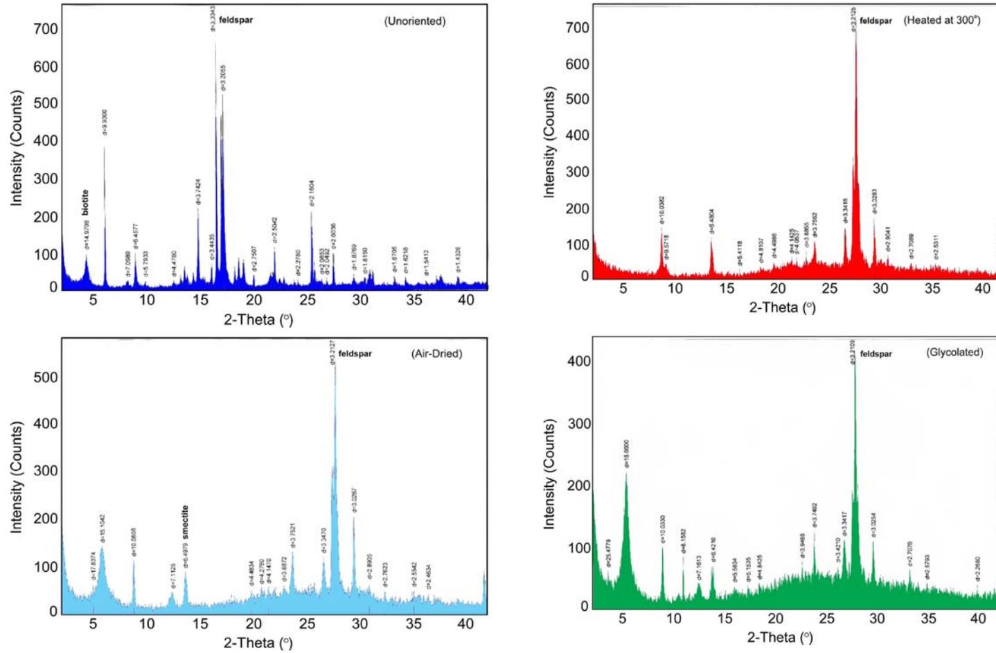
Figure 4.6 X Ray Diffraction patterns of the Çömlekçikuyu andesite
