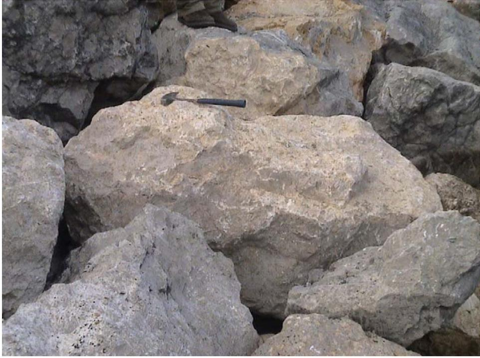
Figure 6.8 Tarlaağzı limestone after two years of service
