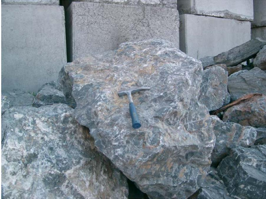
Figure 6.1 A close up view of the Kavakdere limestone used in the Alaplı breakwater
