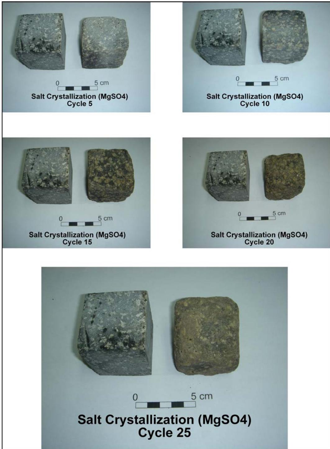
Figure 4.26 Physical appearances of the Çömlekçikuyu andesite during the magnesium sulphate soundness test. The sample on the left side of the photographs indicates a fresh reference sample
