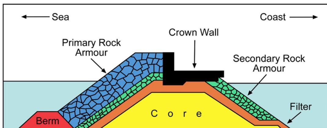
Figure 3.1 Typical cross-section of a conventional rubble mound breakwater (after Smith, 1999)
