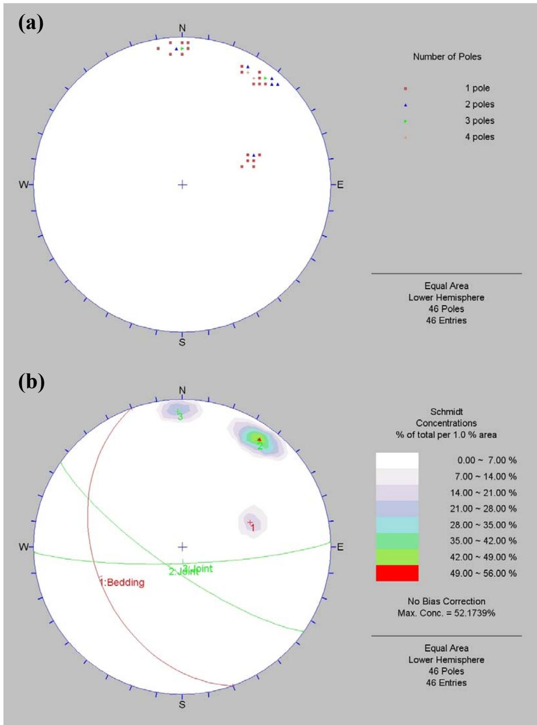
Figure 4.41 Pole plot (a) and contour plot (b) of the discontinuities in the Kiran District
