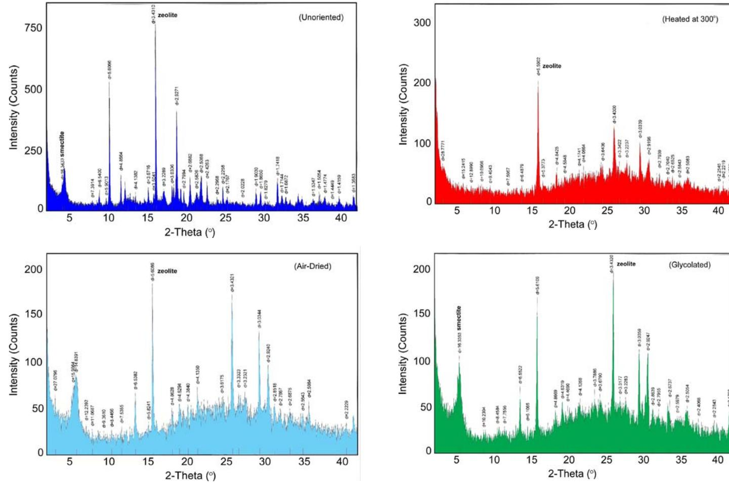
Figure 4.7 X Ray Diffraction patterns of the Kiran Sandstone
