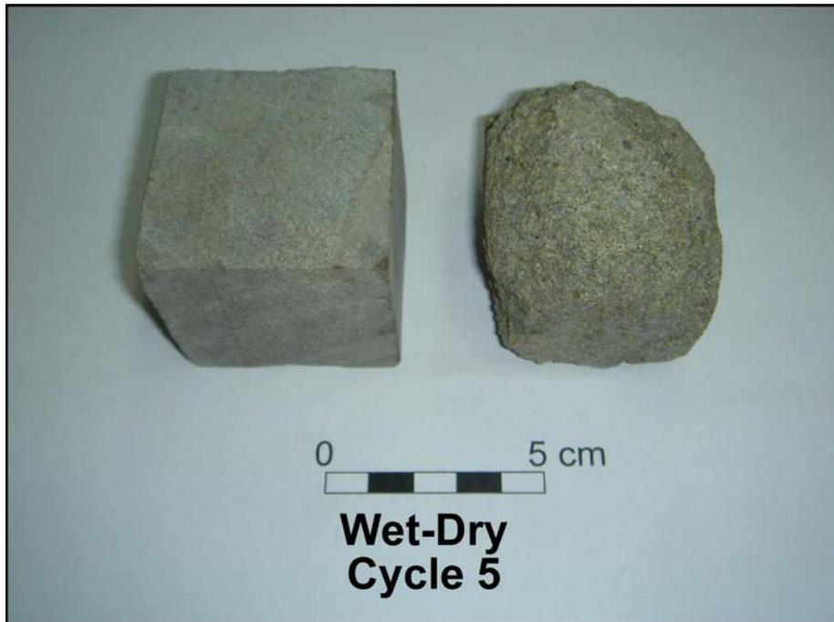
Figure 4.21 Physical appearance of the Kiran sandstone during the wetting-drying test. The sample on the left side of the photographs indicates a fresh reference sample
