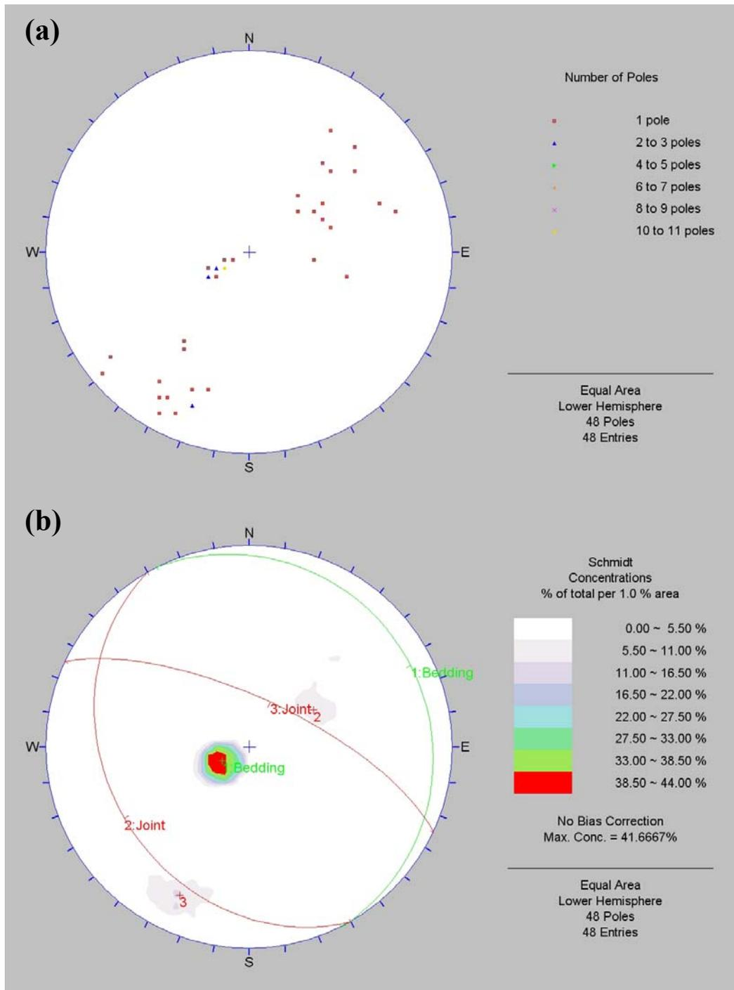
Figure 4.43 Pole plot (a) and contour plot (b) of the discontinuities in the Tarlaağzı quarry
