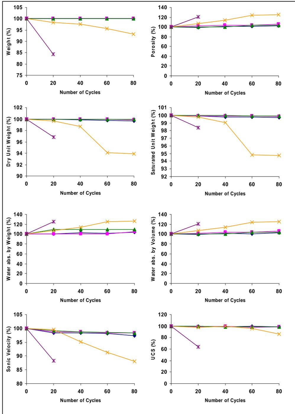
Figure 4.16 Variation of the physico-mechanical properties of the samples after wetting-drying test (green line indicates the Kavakdere limestone, pink line indicates the Kavukkavlağı limestone, blue line indicates the Tarlağzı limestone, orange line indicates the Çömlekçikuyu andesite, and purple line indicates the Kiran sandstone)
