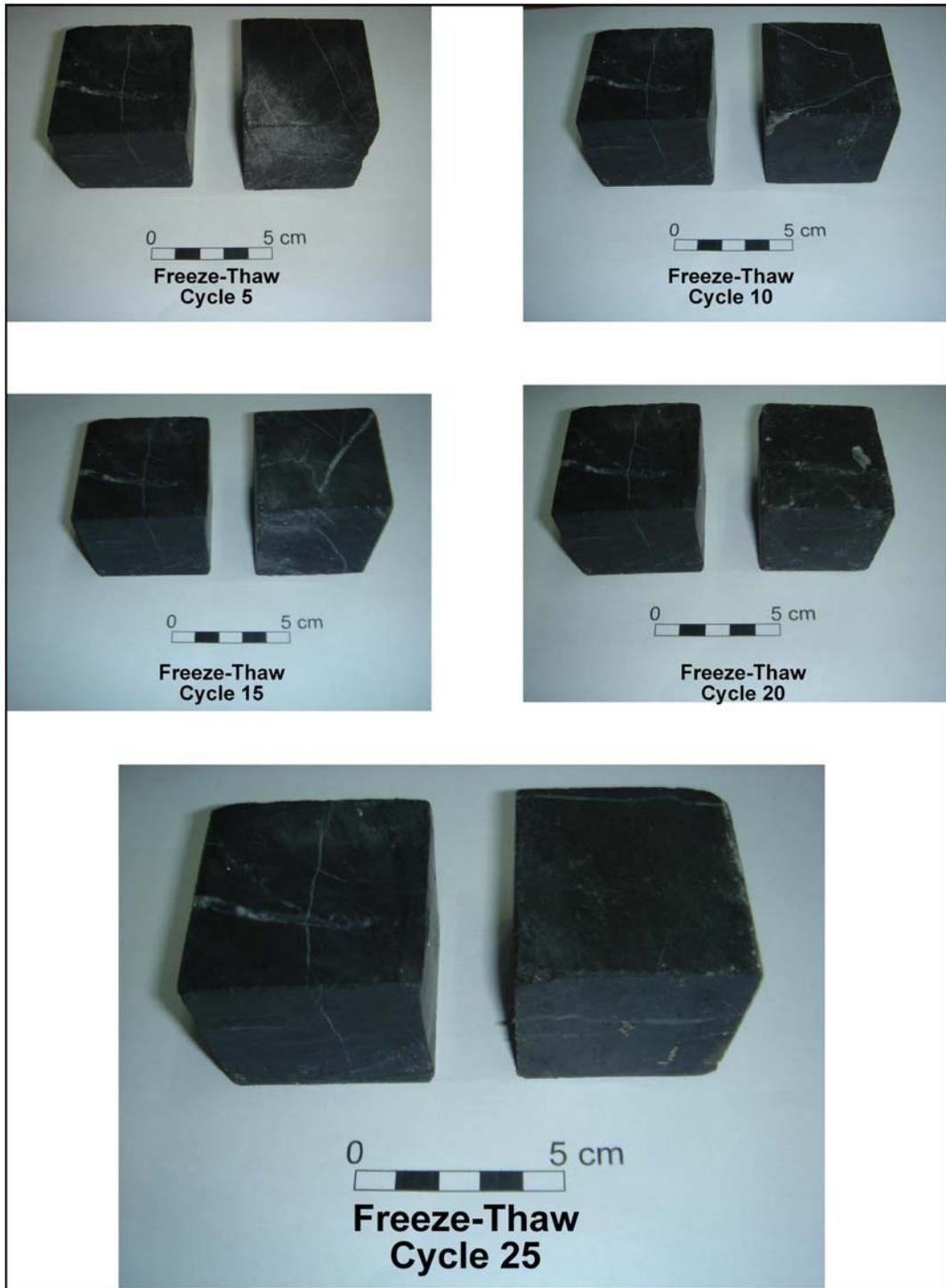
Figure 4.12 Physical appearances of the Kavukkavlağı limestone during the freeze-thaw test. The sample on the left side of the photographs indicates a fresh reference sample.
