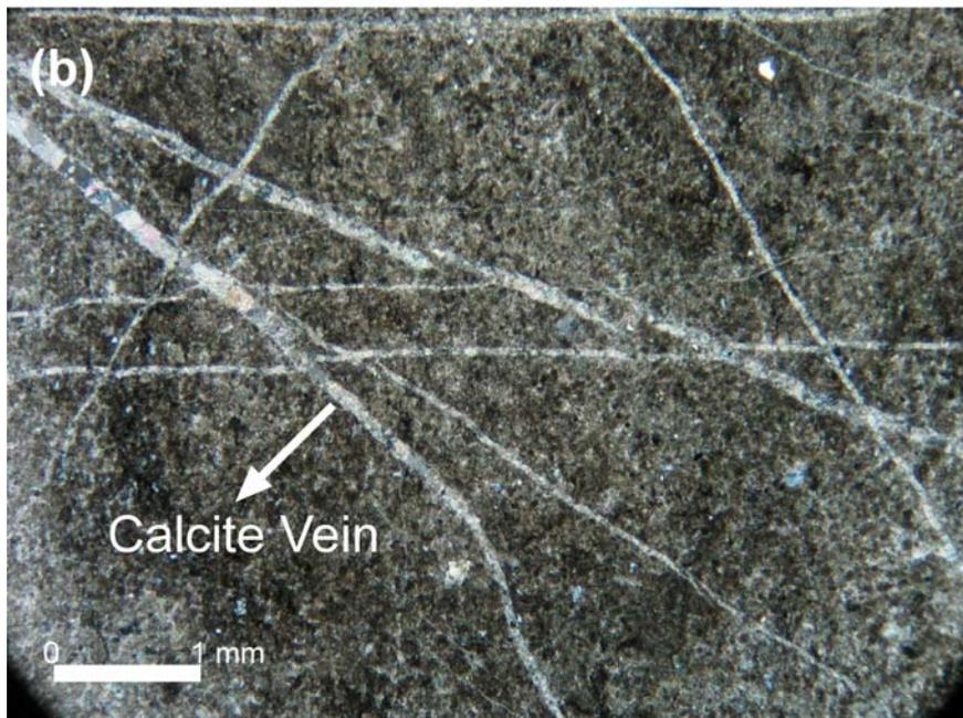
Figure 2.5 Photomicrographs of the Kavukkavlağı limestone (a) plane polarized light (PPL) x5, (b) cross polarized light (CPL) x5
