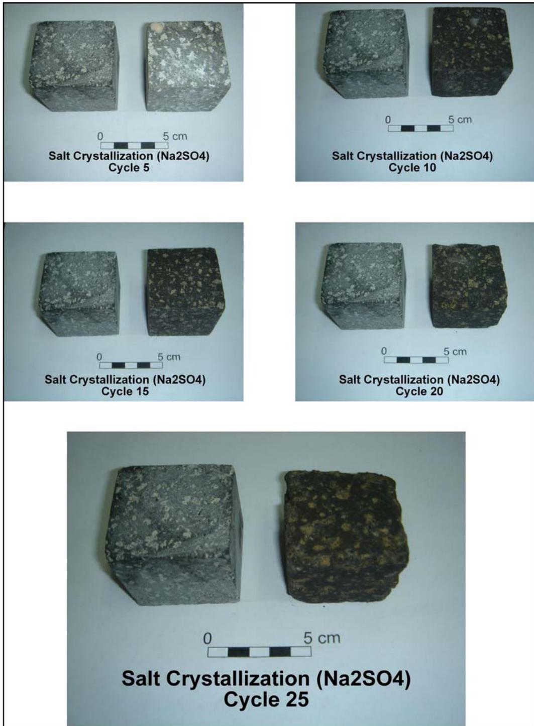
Figure 4.32 Physical appearances of the Çömlekçikuyu andesite during the sodium sulphate soundness test. The sample on the left side of the photographs indicates a fresh reference sample
