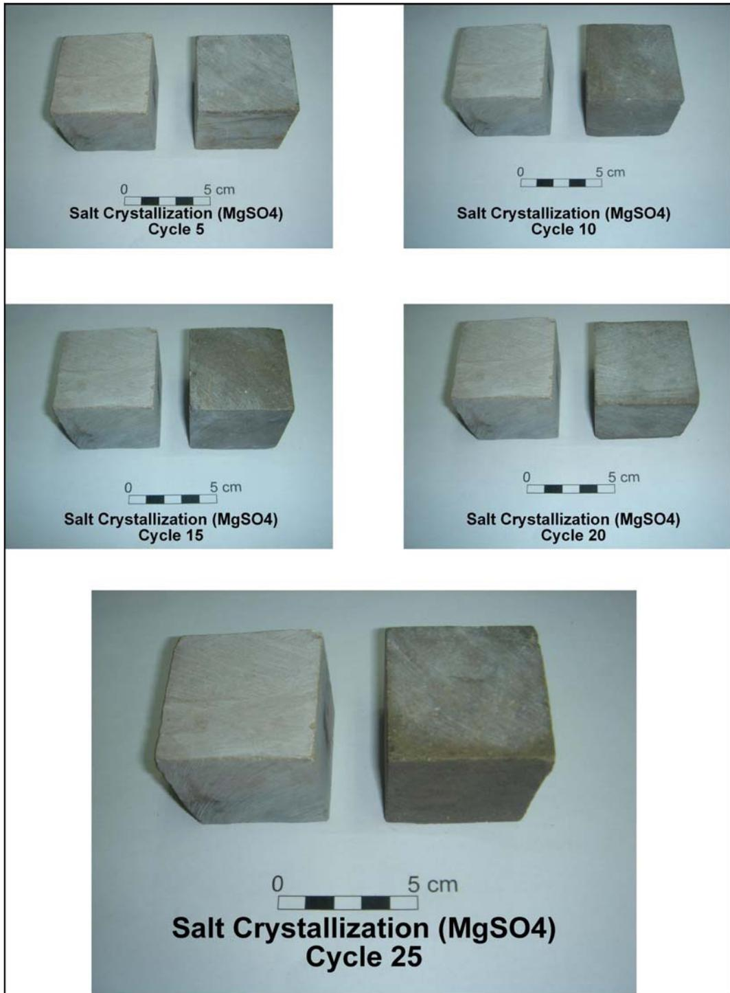
Figure 4.25 Physical appearances of the Tarlaağzı limestone during the magnesium sulphate soundness test. The sample on the left side of the photographs indicates a fresh reference sample
