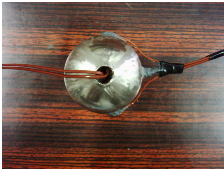
Figure 4.18 Shpere used in the Free&Forced Condensation Experiments After Silver Welding and Polishing
