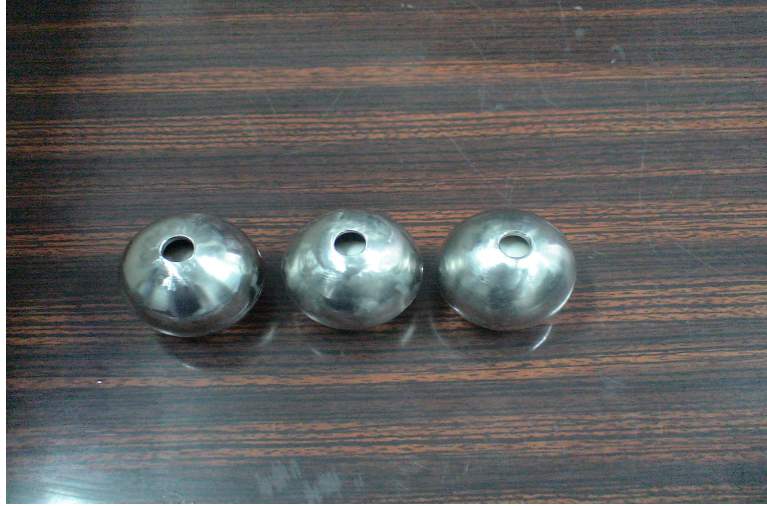
Figure 4.14 First Type of Spheres After Bonding and Polishing
