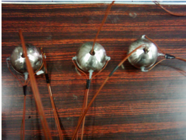
Figure 4.19 Second Type of Spheres with Thermocouples
