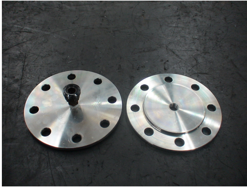
Figure 4.12 View of the Upper (left) and Lower (right) Caps.
