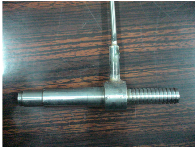
Figure 4.24 The View of the Tight Fit Type of Pipe.
