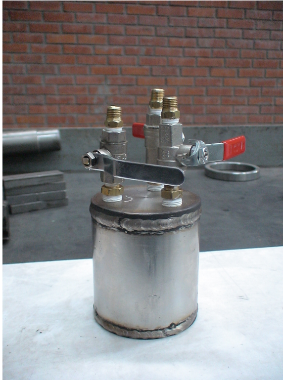
Figure 4.28 View of the Cooling Water Distributer Apparatus.
