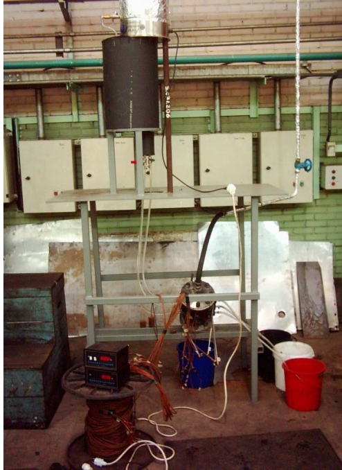
Figure 4.2 General View of the Free Condensation Experimental Setup
