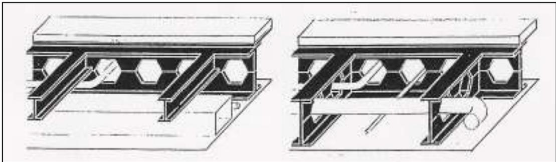
**Figure 2.10.** Unimpeded routing of services
