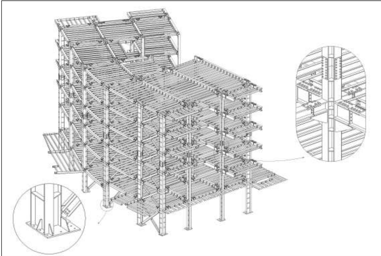
**Figure 4.20.** 3D drawings showing the structural system prepared by Rona Mühendislik for the TESKOMB building
