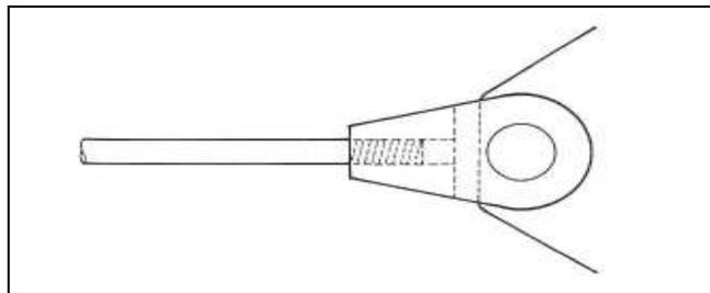
**Figure 2.22.** Pin joint connection for bar
