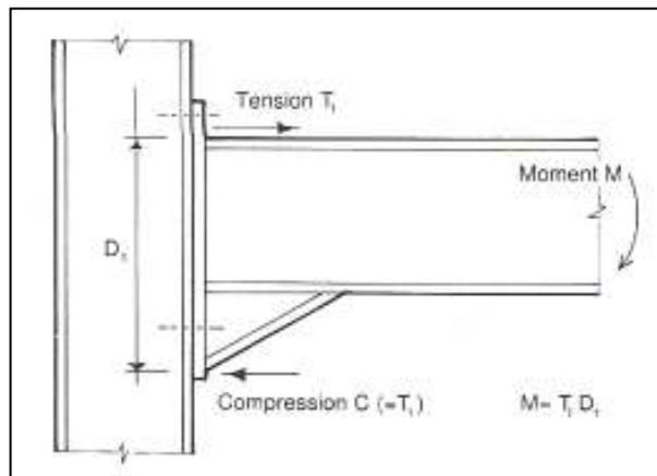
**Figure 2.18.** Beam-to-column moment connection using a gusset
