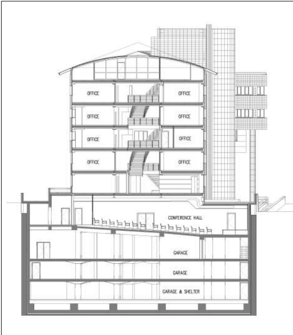
**Figure 4.3.** Section BB of TESKOMB Building
