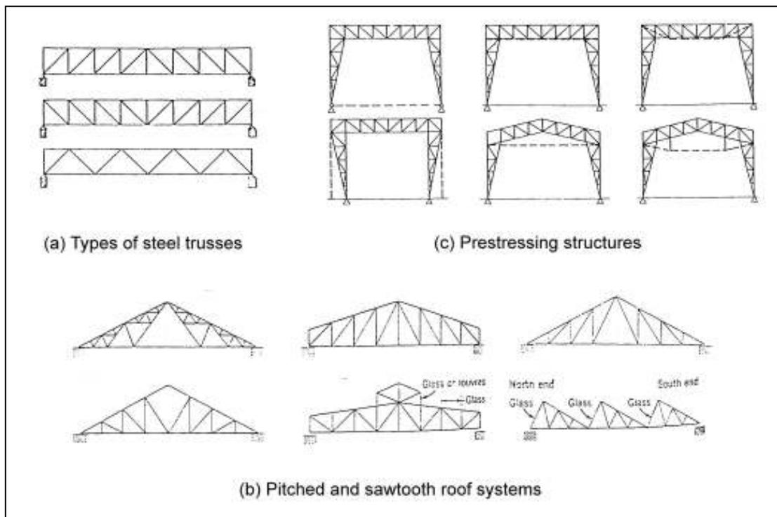
**Figure 2.24.** Structural systems for single-storey structures
