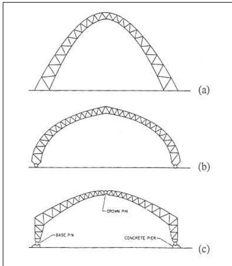
**Figure 2.25.** Typical steel arches; (a) hinged arch, (b) two-hinged arch and (c) three-hinged arch (Source: Watson, 1986)
