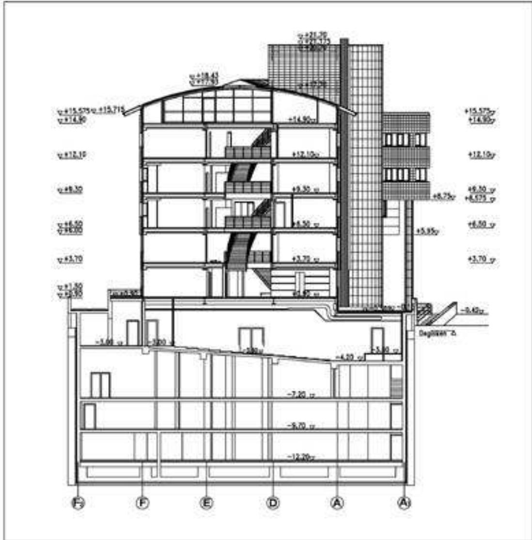
**Figure A.2.** Section BB of TESKOMB Building
