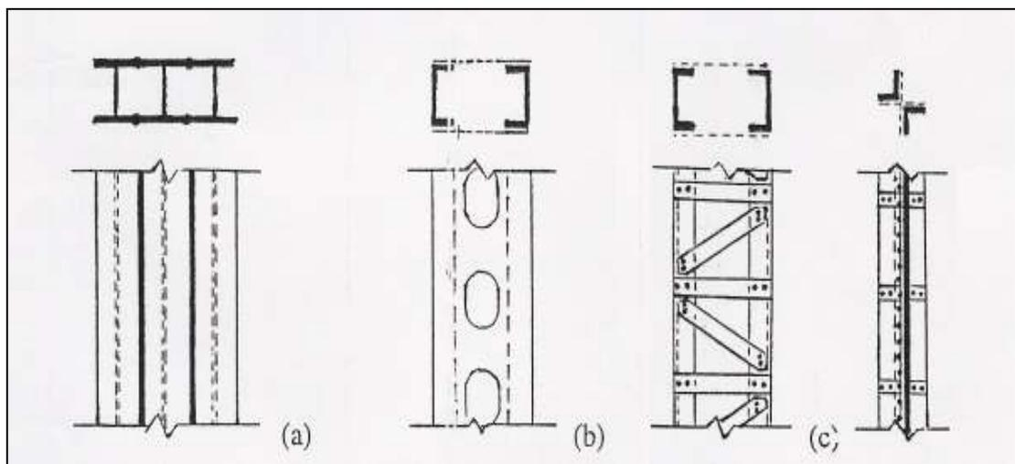
**Figure 2.5.** Built-up columns; (a) solid wall column, (b) solid wall column with perforated cover plates and (c) open type column (Source: Keyder, 1993)
