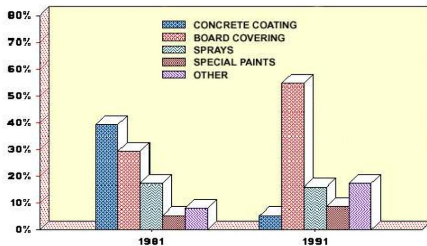
**Figure 2.42.** Fire proofing methods used for steel framed structures in England
