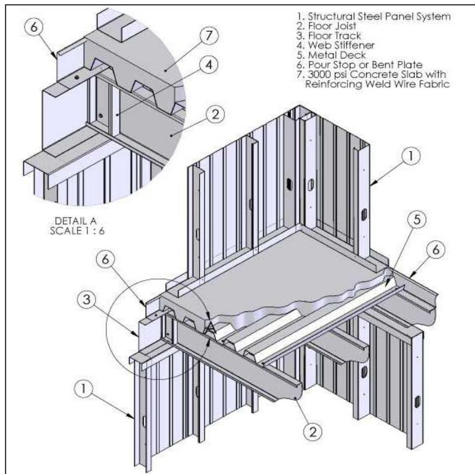
**Figure 2.9.** Steel deck floor system
