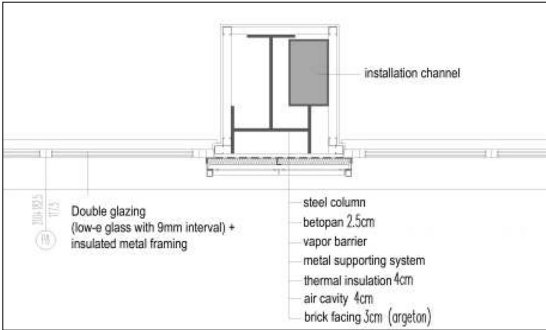
**Figure 4.23.** A detail showing the installation channel adjacent to the steel column
