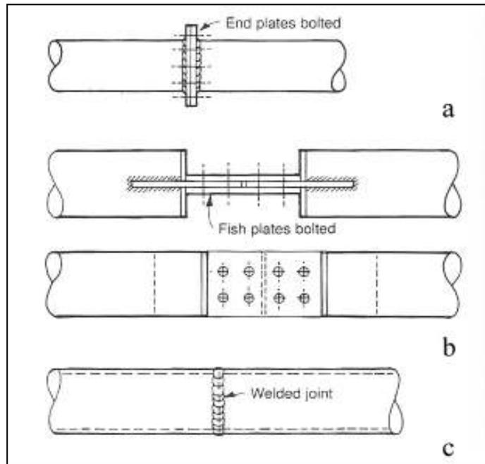
**Figure 2.23.** Tube-to-tube splice.
