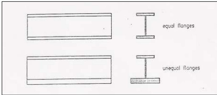
**Figure 2.8.** Fabricated plate girders (Source: Berklin, 1994)
