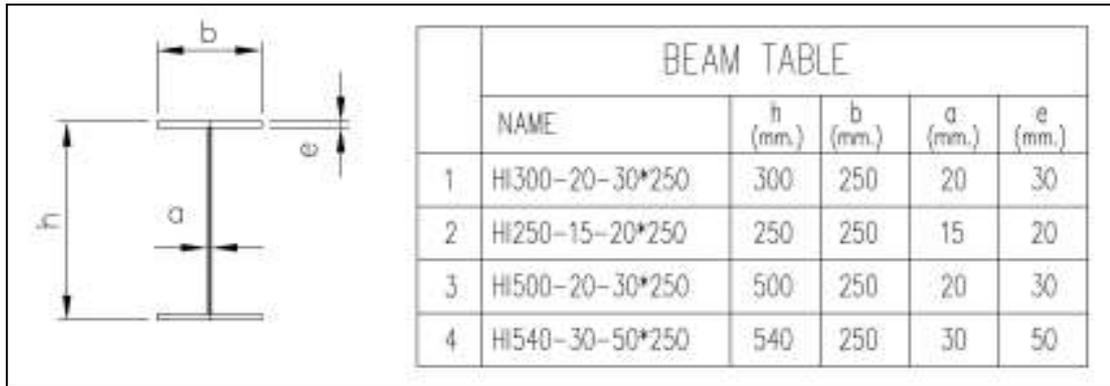
**Figure 4.6.** Beam sections and the various dimensions, used in the structure
