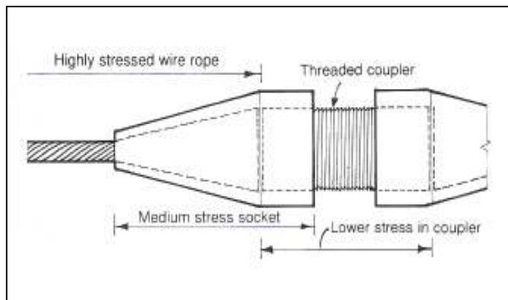
**Figure 2.20.** Threaded coupling for wire rope sockets
