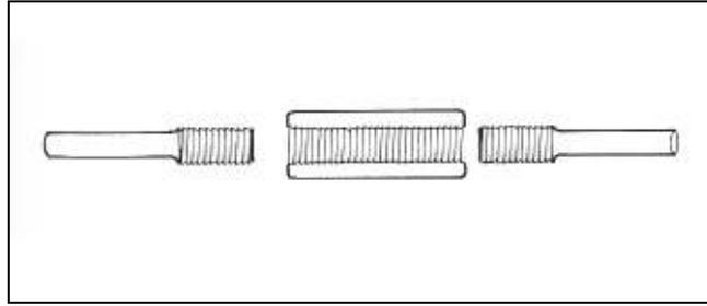
**Figure 2.21.** Threaded coupling for bars
