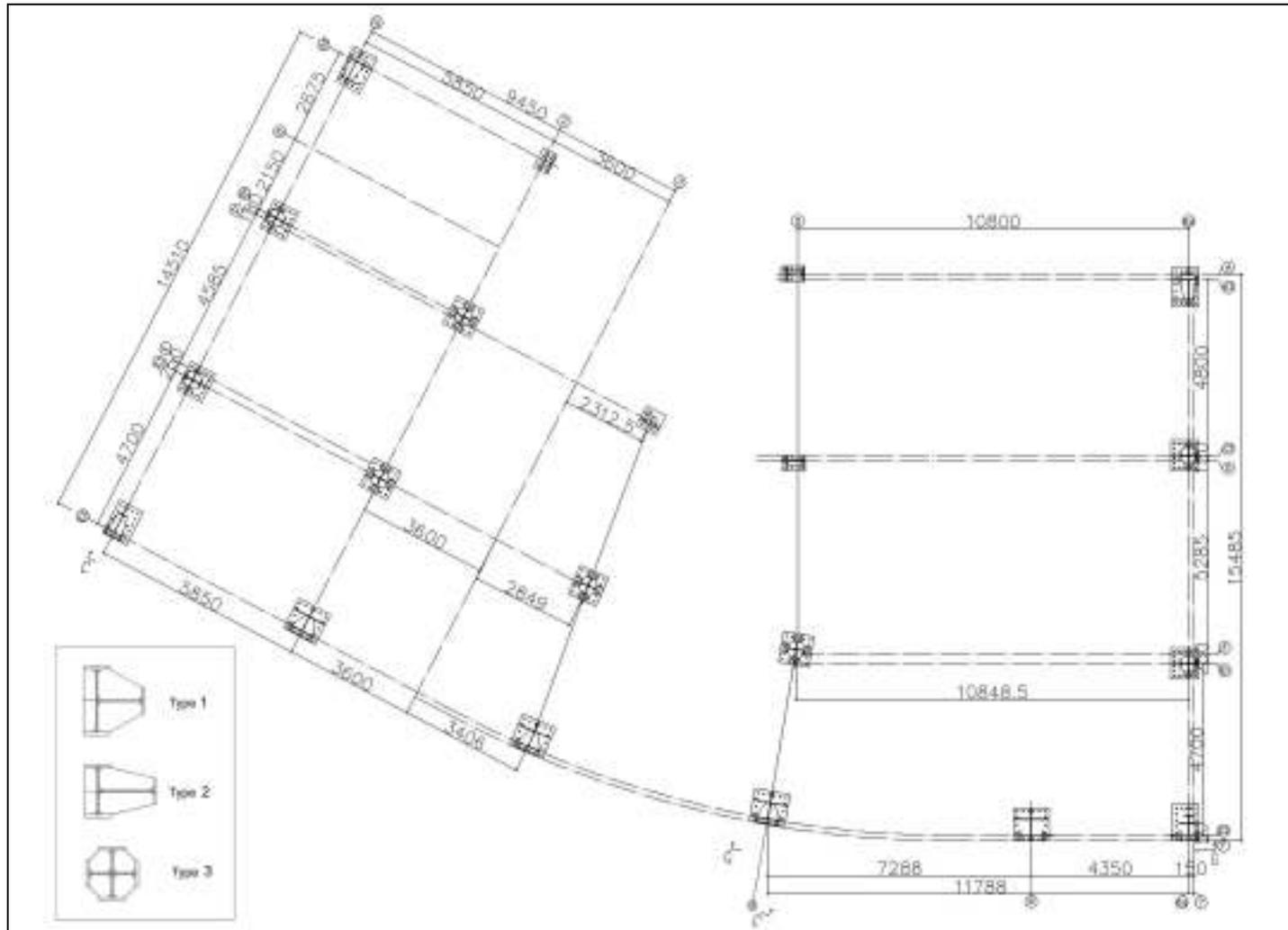
**Figure 4.4.** Structural plan showing location and sizes of columns and beams (Source: Rona Mühendislik)
