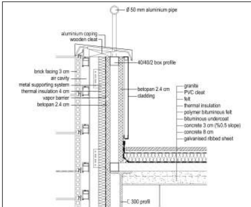
**Figure 4.28.** A detail drawing of the terrace-roof and parapet wall
