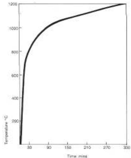
**Figure 2.41** Standard fire-curve (Source: Robinson, 1993)
