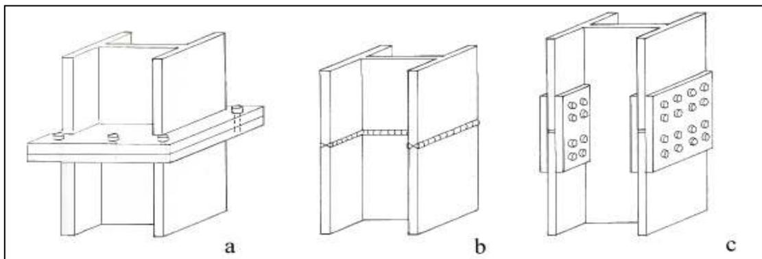
**Figure 2.14.** Direct compression in a column joint carried by (a) end plates, (b) on welds, and (c) on splice plates (Source: Schollar, 1993)
