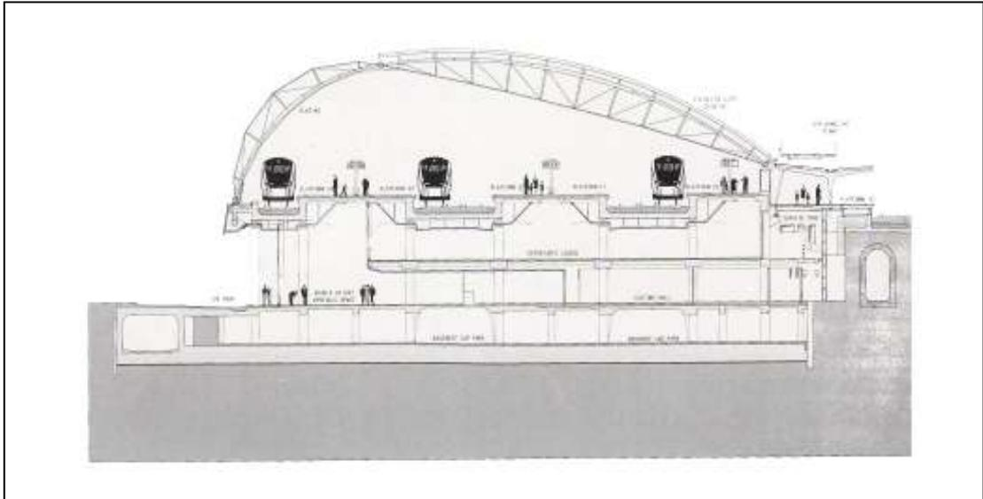
**Figure 2.26.** Cross-section of the Channel Tunnel Terminal Building in London, England (Source: Plank, 1993)
