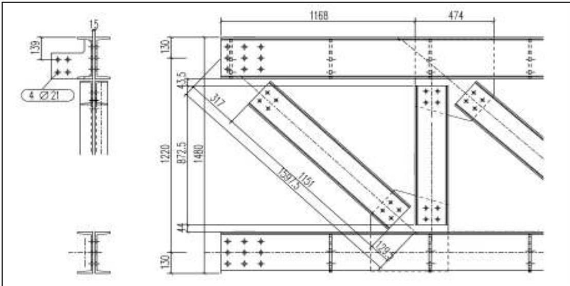
**Figure 4.10.** The section and elevation of the bracings used on the first floor
