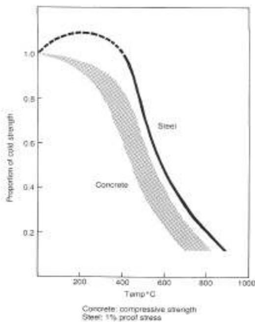
**Figure 2.40** Strength reduction at high temperatures (Source: Robinson, 1993)
