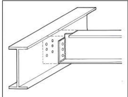
**Figure 2.16.** Beam-to-girder connection using a welded end plate
