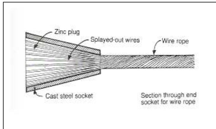
**Figure 2.19.** Diagram of splaying out of wire rope
