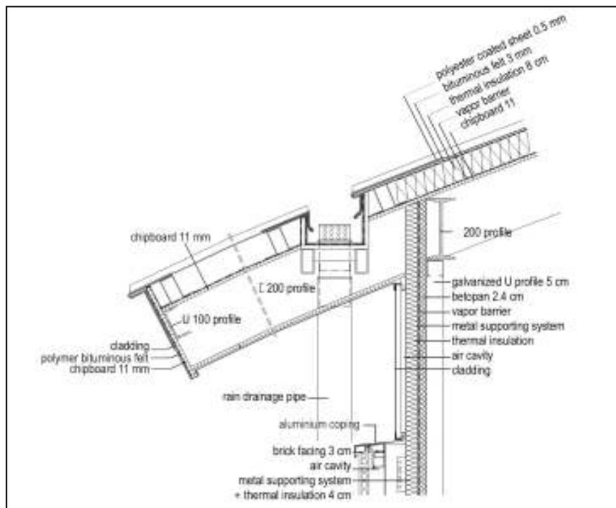
**Figure 4.30.** A point detail of the curved steel roof
