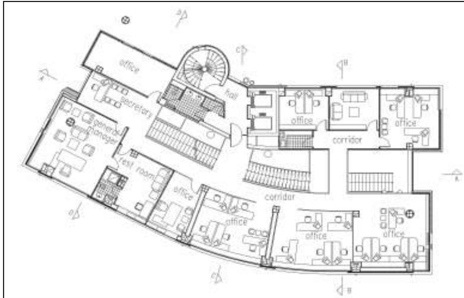
**Figure 3.7.** Second floor plan of TESKOMB Building
