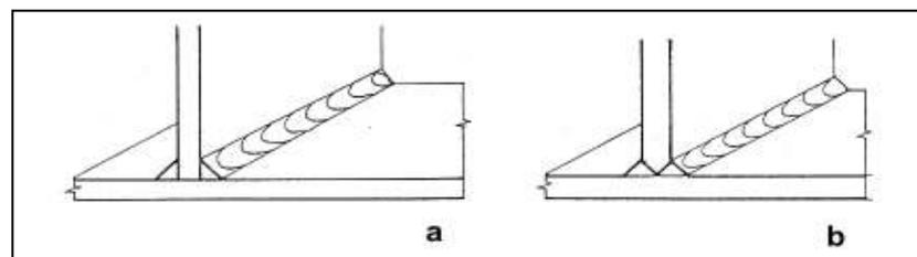
**Figure 2.13.** Typical welds: (a) Fillet weld and (b) butt weld
