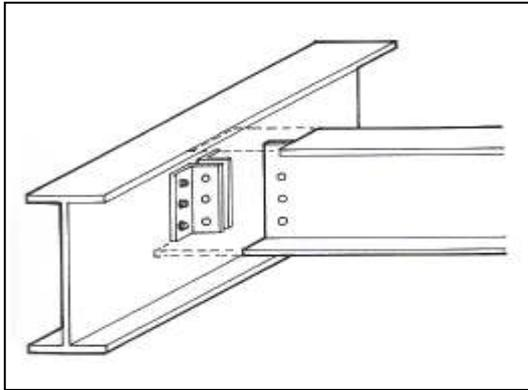
**Figure 2.15.** Beam-to-girder connection using web cleats
