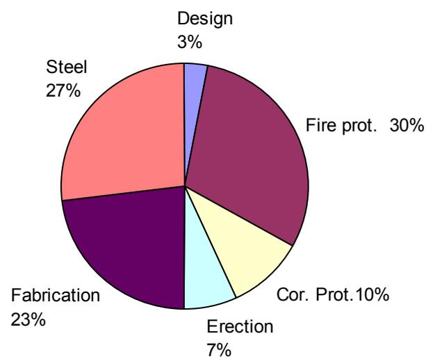
**Figure 2.38.** Pie chart showing cost breakdown for steel construction projects
