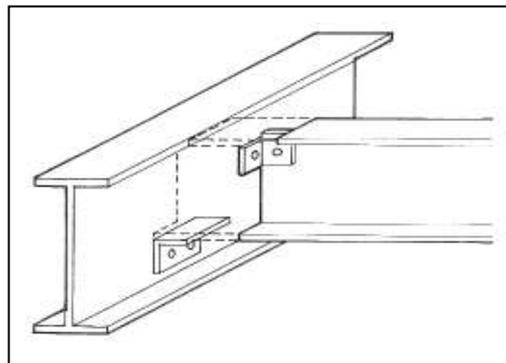
**Figure 2.17.** Beam-to-girder connection using seating and restraining cleats.
