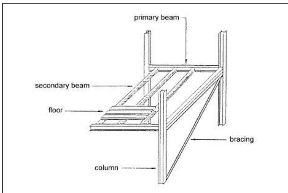
**Figure 2.4.** Typical components of a steel frame
