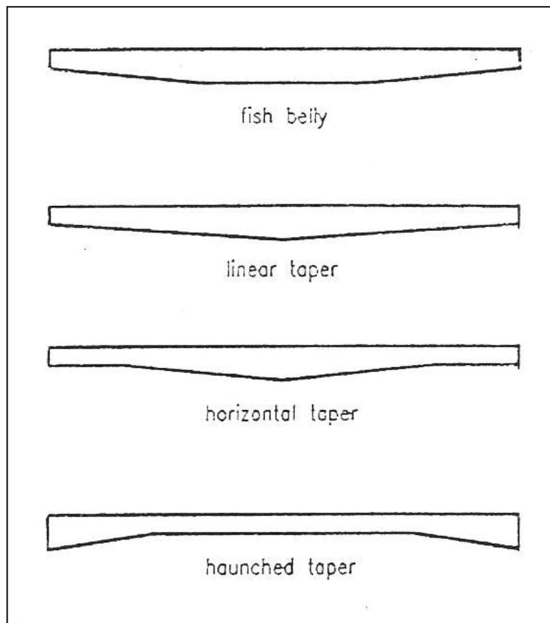
**Figure 2.7.** Tapered beams
