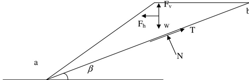
Figure 2.3 Forces acting on a sliding planar mass in Pseudostatic Method
