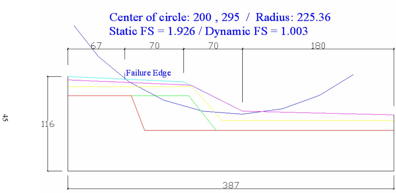
Figure 3.12 Cross section used in SLOPE analyses
