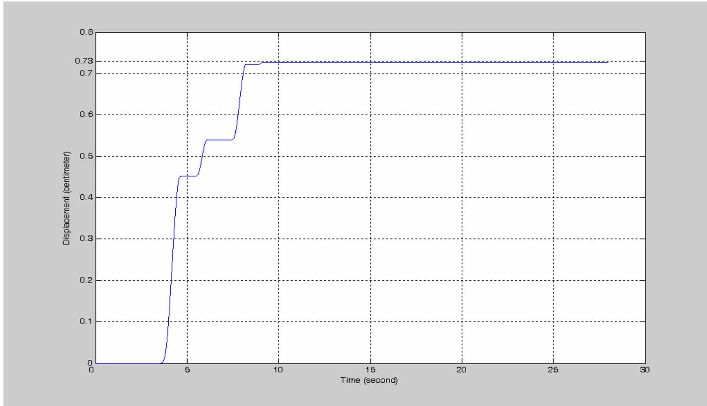
Figure 3.17 Displacement-time graph of the sliding mass (with N-S eq. data)
