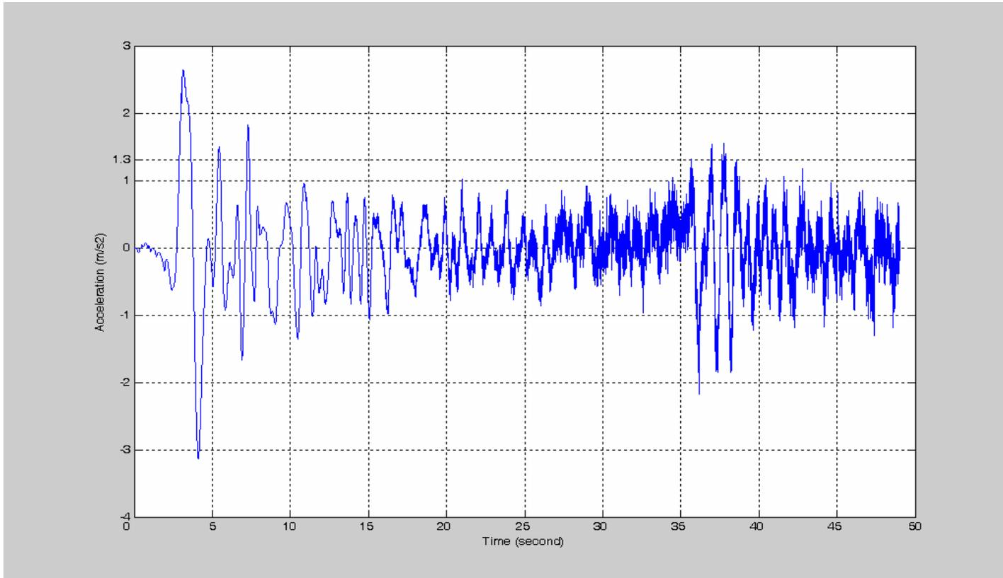
Figure 3.18 Acceleration-time graph of the sliding mass (with E-W eq. data)
