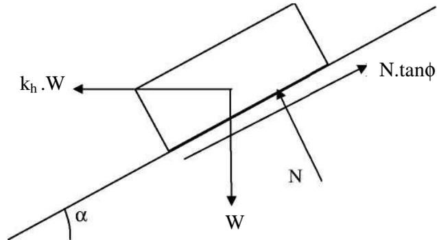
Figure 2.5 Forces acting on a sliding block
