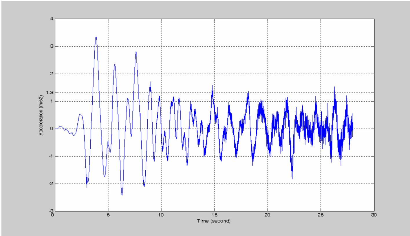
Figure 3.15 Acceleration-time graph of the sliding mass (with N-S eq. data)
