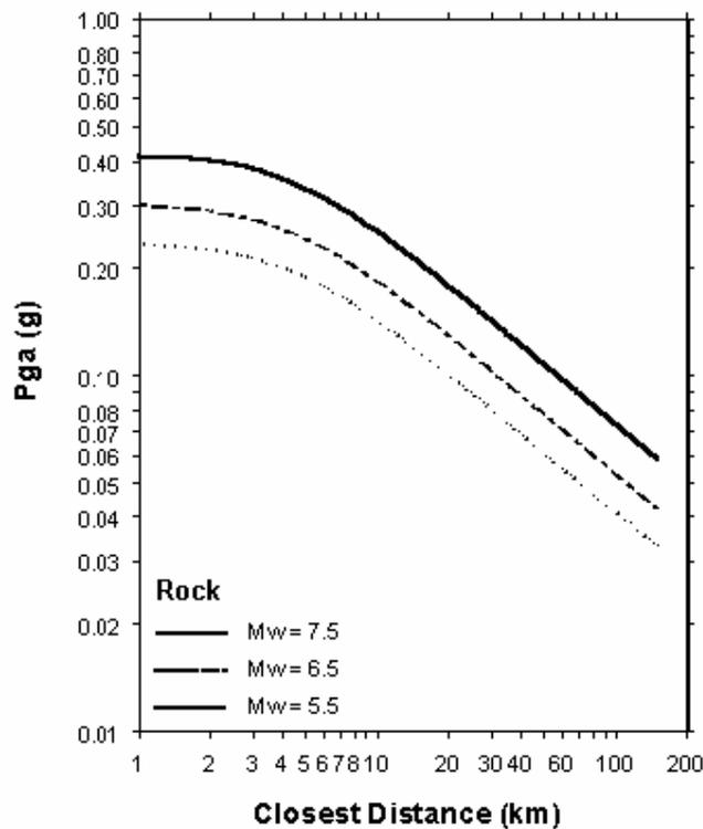
Figure 3.14 Curves of peak acceleration versus distance at rock sites (Gülkan & Kalkan, 2002)
