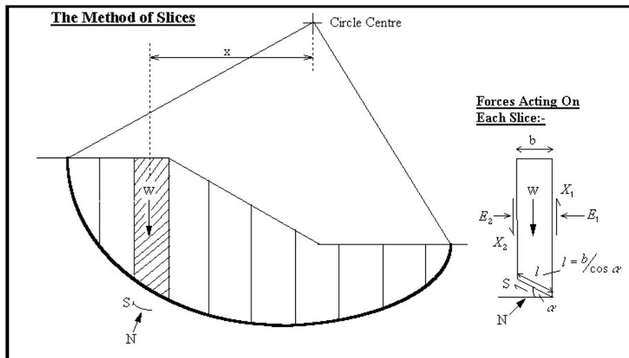
Figure 2.1 Forces acting on a slice in Method of Slices
