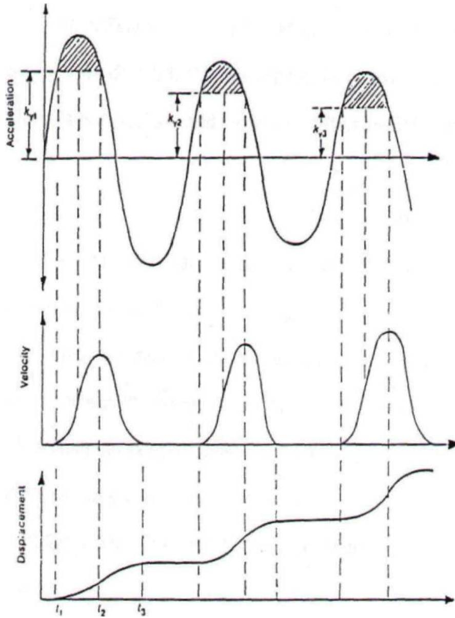
Figure 2.6 Twice integration of acceleration time-history to calculate displacements (Seed, H.B., 1979)
