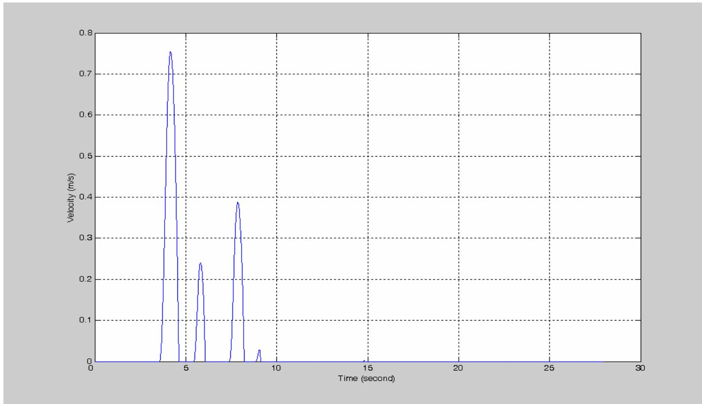
Figure 3.16 Velocity-time graph of the sliding mass (with N-S eq. data)
