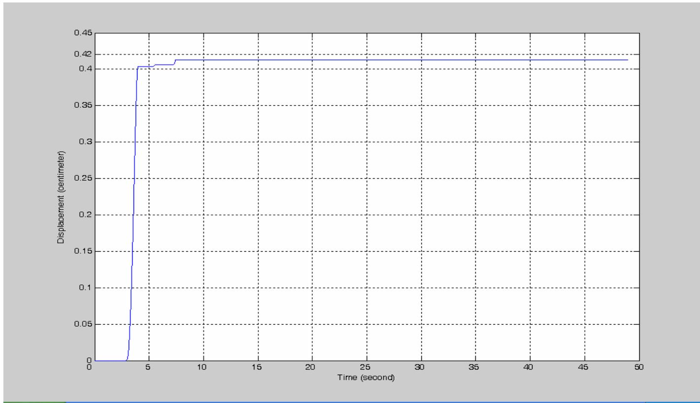
Figure 3.20 Displacement-time graph of the sliding mass (with E-W eq. data)
