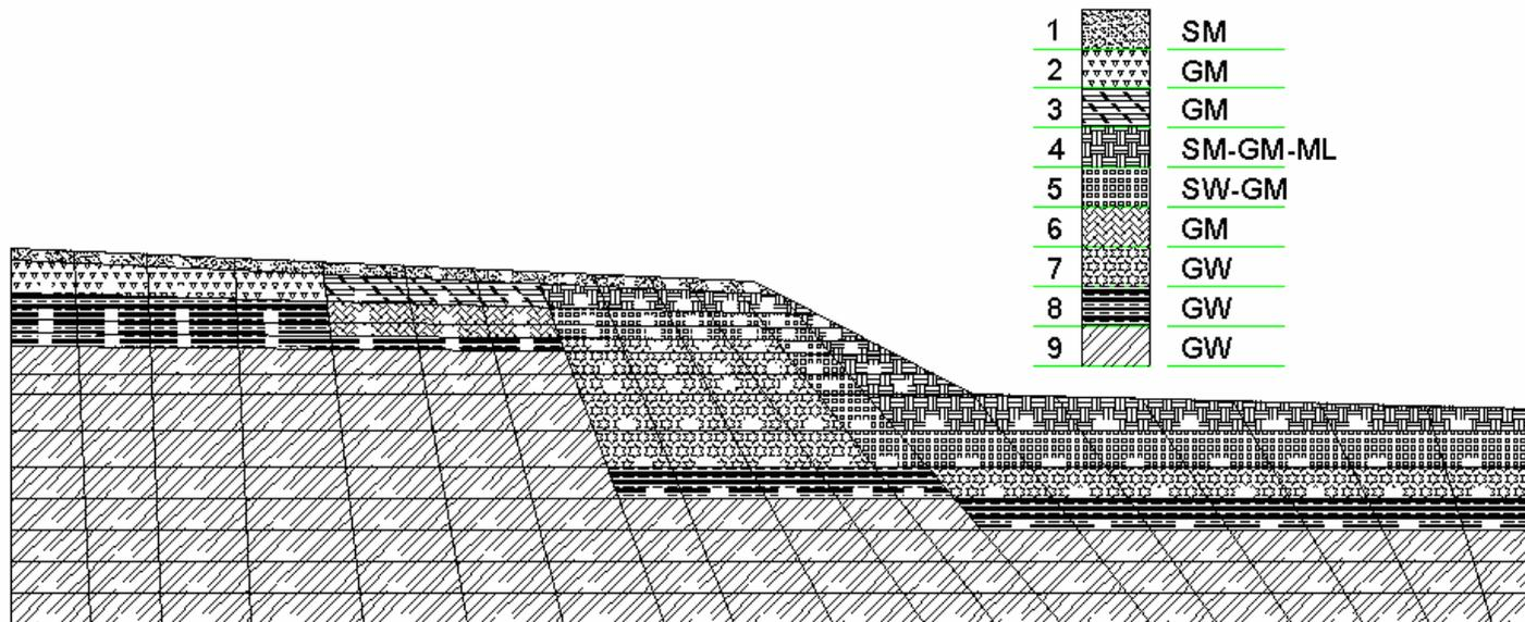
Figure 3.11 Cross section of the slope indicating the soil types
