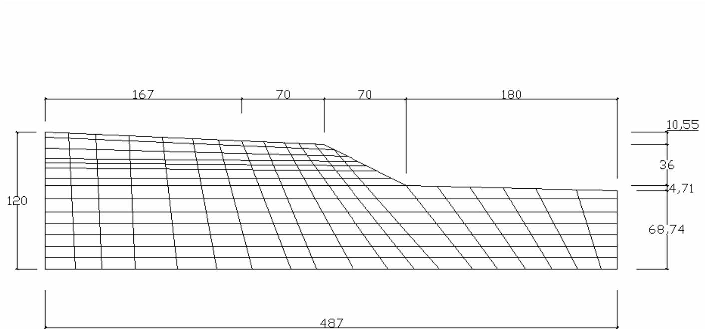
Figure 3.10 Mesh of cross section used in TELSTA and TELDYN analyses
