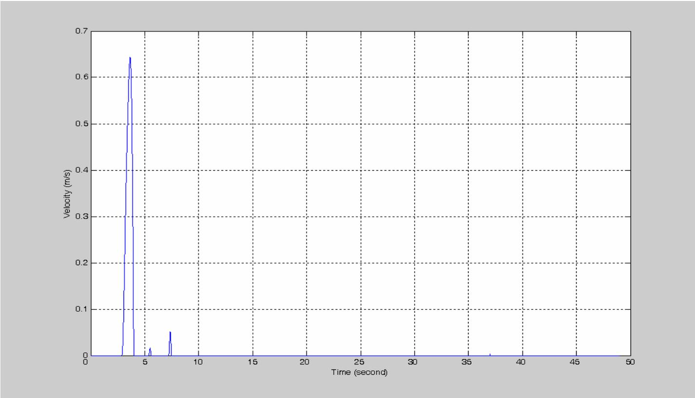
Figure 3.19 Velocity-time graph of the sliding mass (with E-W eq. data)
