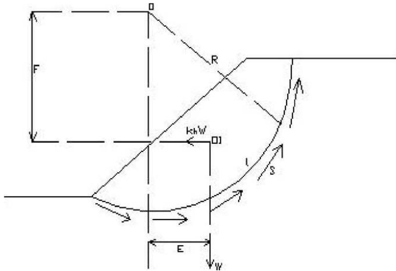
Figure 2.2 Forces acting on a sliding circular mass in Pseudo-static Method
