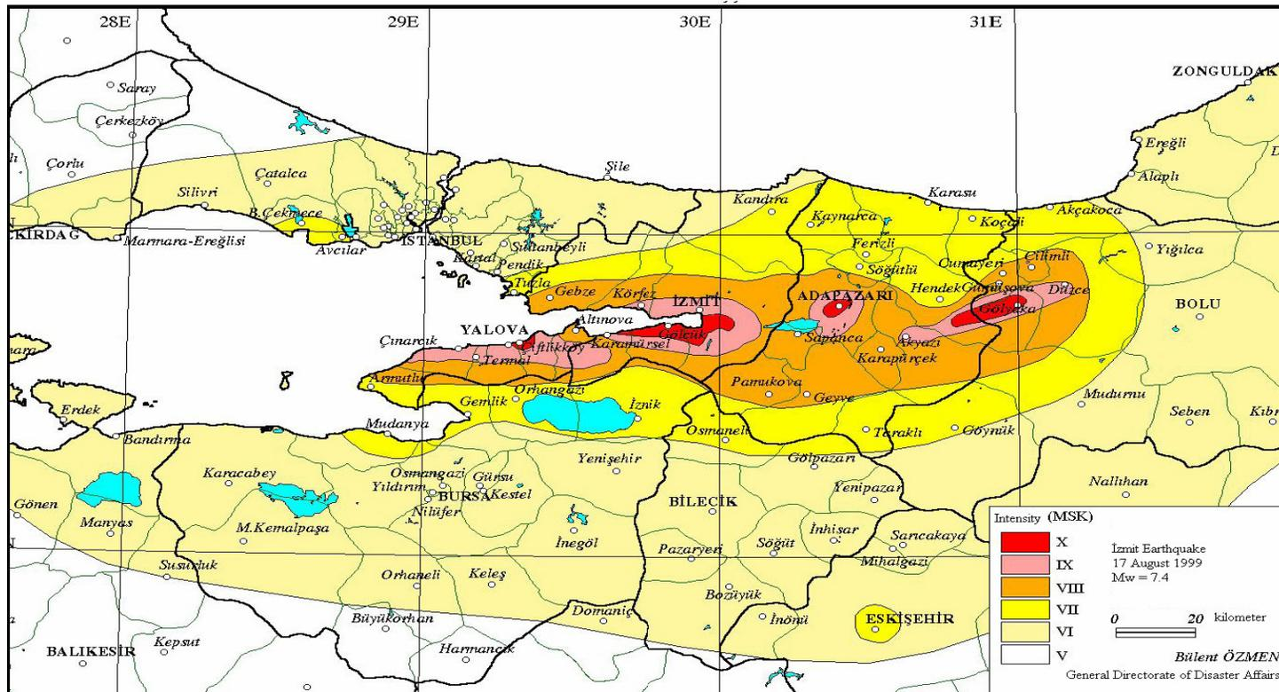
Figure 3.5 Isoseismal map of Kocaeli earthquake (Özmen, 2000.a)
