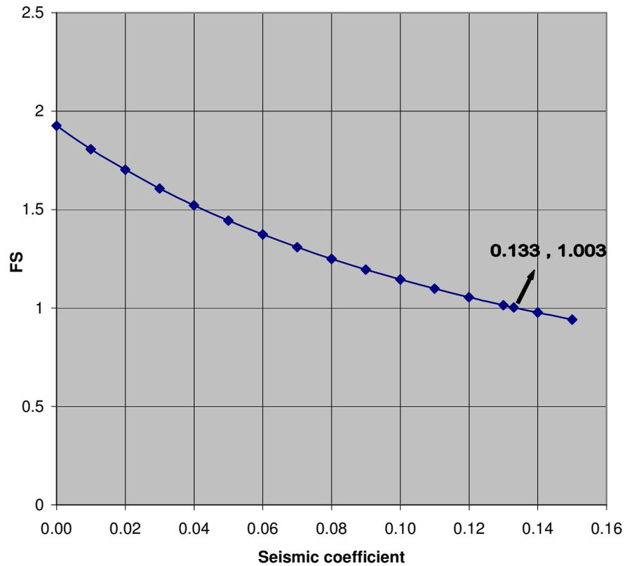
Figure 3.13 Sensitivity of FS to seismic coefficient
