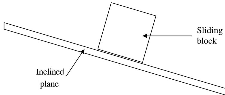
Figure 2.4 Sliding block resting on an inclined plane
