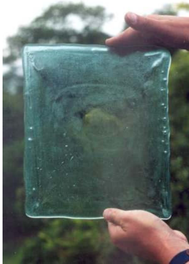
Figure 6: Window glass made by using ancient Roman casting techniques (Discovery Channel, Meet the Ancestors )
