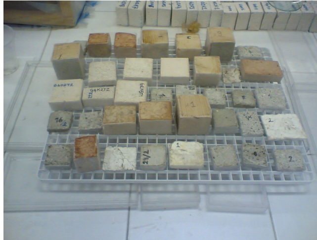
Figure 3.05. AAC, AAC plaster, historical infill and masonry fired brick, and historical lime based interior and exterior plaster samples left for drying at 20°C and 40±5 % relative humidity.
