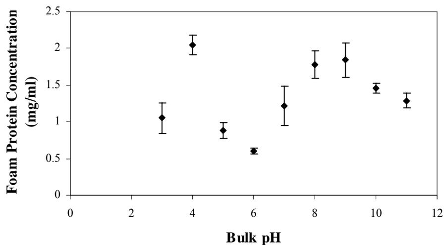
**Figure 3.16** Change of foam protein concentration with respect to bulk solution pH (initial protein concentration: 0.504 mg/ml, changed within a range of 0.399-0.570 mg/ml after pH adjustment; total foaming time: 30 min, temperature: 20-25°C). The points are average of duplicate experiments.
