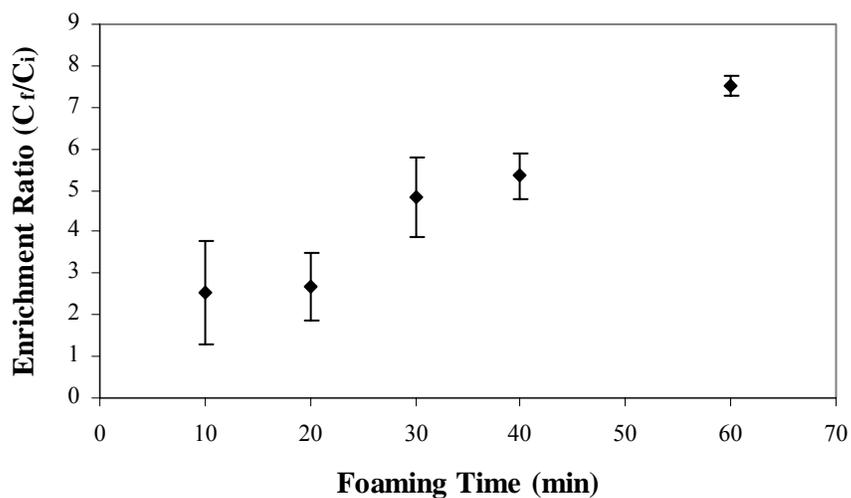
**Figure 3.12** Effect of foaming time on enrichment ratio (at room temperature: 20-25 °C, air velocity:  $38.5 \pm 1$  cm<sup>3</sup>/min, feed solution concentration: 0.064 mg/ml, feed volume: 250 ml, foaming time: 10-60 min). The points are average of triplicate experiments.
