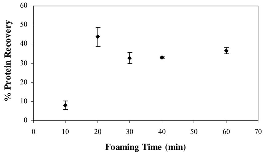
**Figure 3.14** Effect of foaming time on % protein recovery (at room temperature: 20-25 °C, air velocity:  $38.5 \pm 1 \text{ cm}^3/\text{min}$ , feed solution concentration: 0.064 mg/ml, feed volume: 250 ml, foaming time: 10-60 min). The points are average of triplicate experiments.
