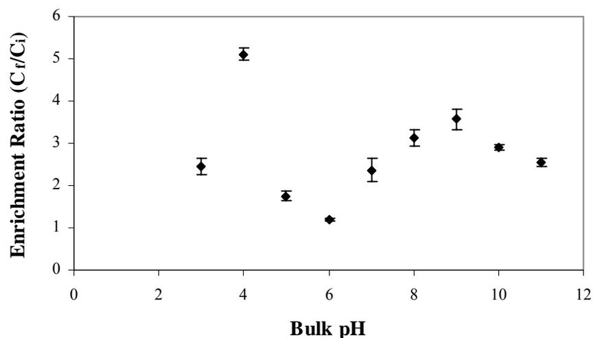
**Figure 3.17** Effect of bulk solution pH on enrichment ratio (initial protein concentration: 0.504 mg/ml, changed within a range of 0.399-0.570 mg/ml after pH adjustment; total foaming time: 30 min, temperature: 20-25°C). The points are average of duplicate experiments.
