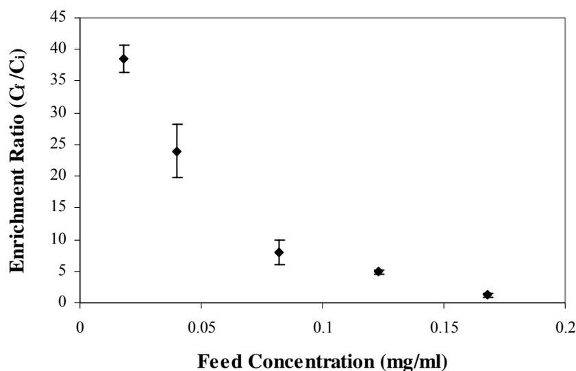
**Figure 3.2** Effect of feed protein concentration on enrichment ratio (at room temperature: 20-25 °C, air velocity:  $56 \pm 1$  cm<sup>3</sup>/min, feed volume: 200 ml, feed protein concentration: 0.018-0.168 mg/ml). The points are average of triplicate experiments.
