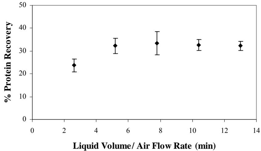
**Figure 3.11** Effect of liquid pool height on % protein recovery (at room temperature: 20-25 °C, air flow rate:  $38.5 \pm 1$  cm<sup>3</sup>/min, initial feed concentration: 0.031 mg/ml, feed volume: 100-500 ml with liquid pool height of 13-53.5 cm, foaming time: 1 h). The points are average of triplicate experiments.
