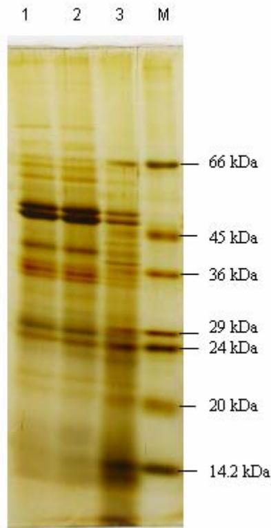
**Figure 3.19** SDS-PAGE analyses of spent yeast extract foam fractionation samples. The proteins on the gel were silver-stained. Molecular weight standard proteins are marked as “M” above the lane, lane 1: feed solution, lane 2: residual solution, lane 3: foam sample. Feed protein concentration: 0.147 mg/ml; residual solution protein concentration: 0.106 mg/ml; foam sample protein concentration: 0.328 mg/ml.
