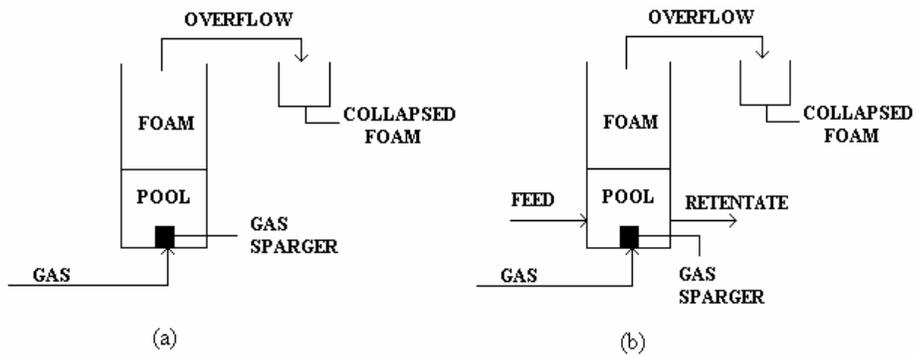
**Figure 1.5** Foam fractionation in the simple mode
