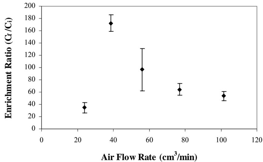
**Figure 3.6** Effect of air flow rate on enrichment ratio (at room temperature: 20-25 °C, air velocity: 24-101.5 cm<sup>3</sup>/min, feed solution concentration: 0.018 mg/ml, feed volume: 200 ml). The points are average of triplicate experiments.
