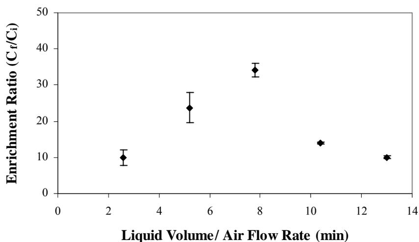
**Figure 3.9** Effect of liquid pool height on enrichment ratio (at room temperature: 20-25°C, air flow rate: 38.5±1 cm<sup>3</sup>/min, initial feed concentration: 0.031 mg/ml, feed volume: 100-500 ml with liquid pool height of 13-53.5 cm, foaming time: 1 h). The points are average of triplicate experiments.
