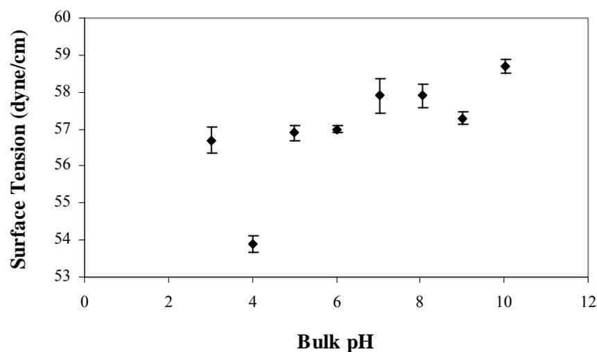
**Figure 3.15** Effect of pH on the surface tension of spent yeast extract solution. (initial protein concentration: 0.504 mg/ml, changed within a range of 0.399-0.570 mg/ml after pH adjustment. The points are average of duplicate experiments.
