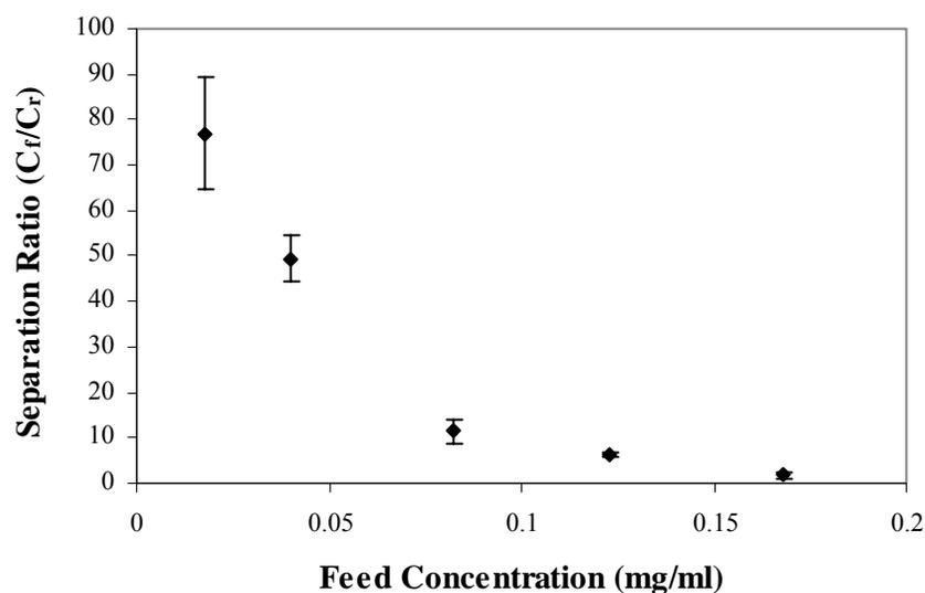
**Figure 3.4** Effect of feed protein concentration on separation ratio (at room temperature: 20-25 °C, air velocity:  $56 \pm 1$  cm<sup>3</sup>/min, feed volume: 200 ml, feed protein concentration: 0.018-0.168 mg/ml). The points are average of triplicate experiments.
