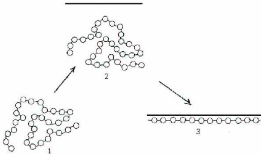
**Figure 1.7** Schematic illustration of protein molecules in the solution state (1), after diffusion to the subsurface region (2), and the reoriented molecules in the adsorbed state (Taken from Führling, 2004)
