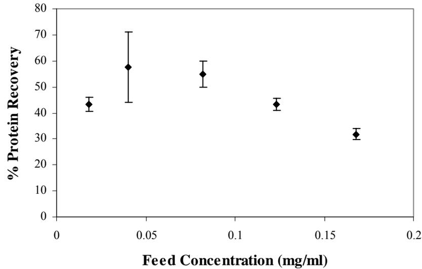
**Figure 3.5** Effect of feed protein concentration on percentage of total protein recovered as foam (at room temperature: 20-25 °C, air velocity:  $56 \pm 1$  cm<sup>3</sup>/min, feed volume: 200 ml, feed protein concentration: 0.018-0.168 mg/ml). The points are average of triplicate experiments.
