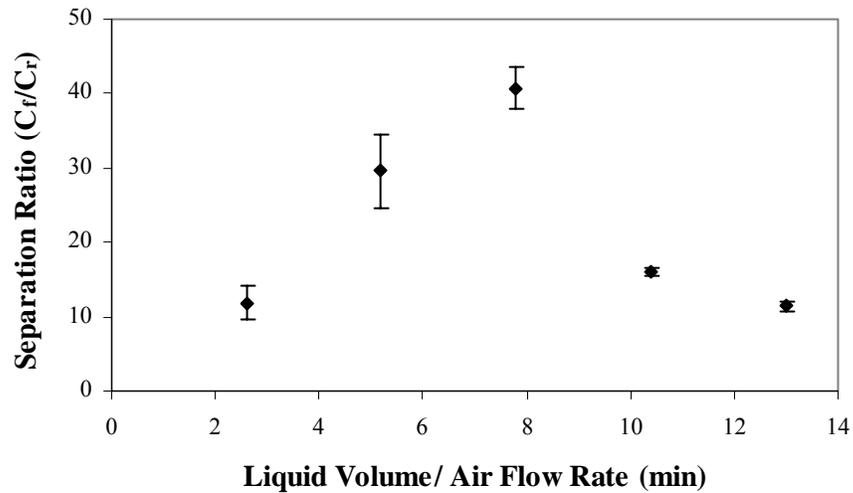
**Figure 3.10** Effect of liquid pool height on separation ratio (at room temperature: 20-25 °C, air flow rate:  $38.5 \pm 1$  cm<sup>3</sup>/min, initial feed concentration: 0.031 mg/ml, feed volume: 100-500 ml with liquid pool height of 13-53.5 cm, foaming time: 1 h). The points are average of triplicate experiments.
