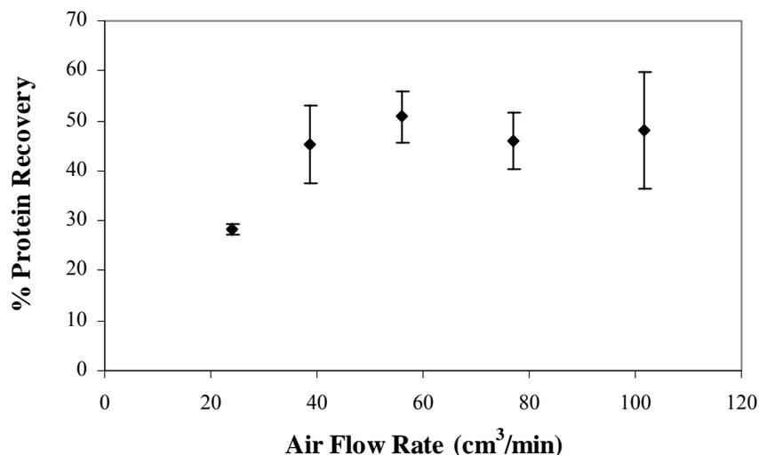
**Figure 3.8** Effect of air flow rate on percentage of total protein recovered in foam (at room temperature: 20-25°C, air velocity: 24-101.5 cm<sup>3</sup>/min, feed solution concentration: 0.018 mg/ml, feed volume: 200 ml). The points are average of triplicate experiments.
