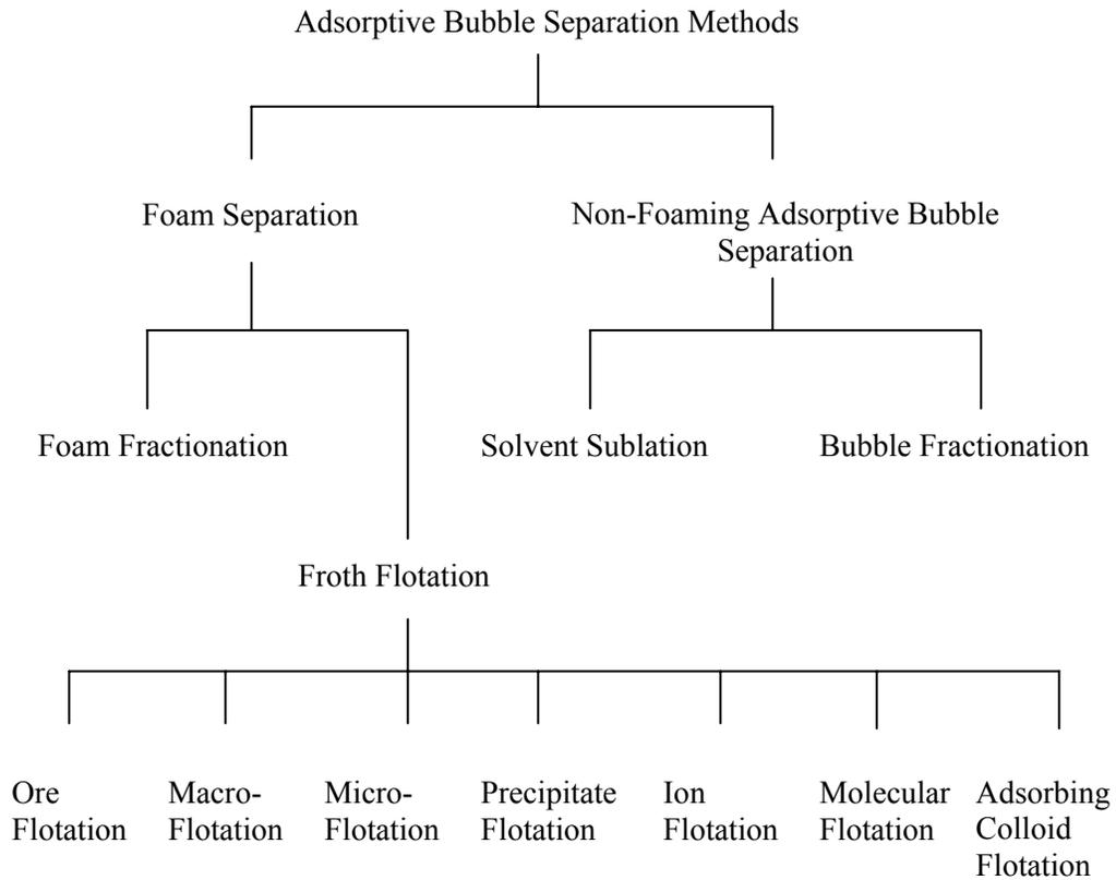
**Figure 1.1** Schematic classification of the adsorptive bubble separation techniques (Taken from Lemlich, 1972).
