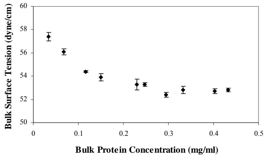
**Figure 3.1** Effect of protein concentration (0.03-0.43 mg/ml) on bulk surface tension of lactic acid broth (measured at 20°C). The points are average of triplicate measurements.
