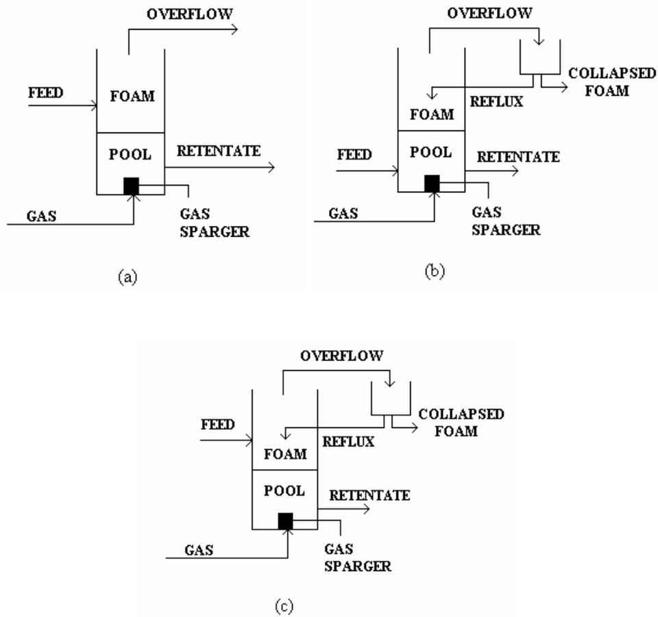
**Figure 1.6** Foam fractionation in continuous mode
