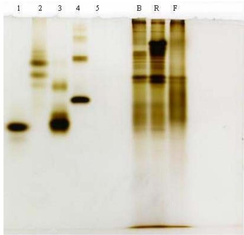
**Figure 3.20** Native-PAGE analysis of residual beer foam fractionation. Lanes 1-4 are molecular weight markers (1.  $\alpha$ -lactalbumin, 2. carbonic anhydrase, 3. chicken egg albumin, 4. BSA), B: residual beer feed solution, R: residual solution, F: Foam sample. Each sample contains 10  $\mu$ g of protein.
