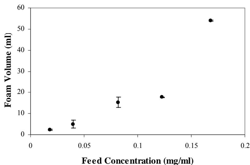
**Figure 3.3** Change in volume of the foam collected with respect to initial feed concentration (at room temperature: 20-25 °C, air velocity:  $56 \pm 1$  cm<sup>3</sup>/min, feed volume: 200 ml, feed protein concentration: 0.018-0.168 mg/ml). The points are average of triplicate experiments.
