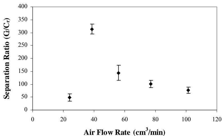
**Figure 3.7** Effect of air flow rate on separation ratio (at room temperature: 20-25 °C, air velocity: 24-101.5 cm<sup>3</sup>/min, feed solution concentration: 0.018 mg/ml, feed volume: 200 ml). The points are average of triplicate experiments.
