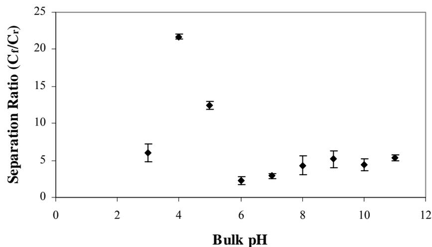
**Figure 3.18** Effect of bulk solution pH on separation ratio (initial protein concentration: 0.504 mg/ml, changed within a range of 0.399-0.570 mg/ml after pH adjustment; total foaming time: 30 min, temperature: 20-25°C). The points are average of duplicate experiments.
