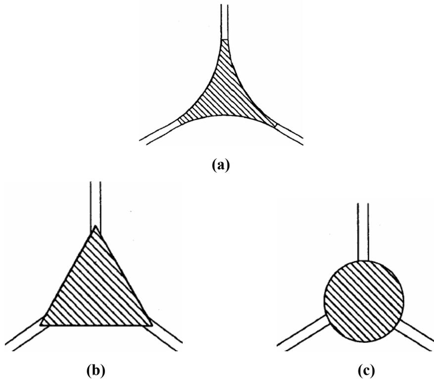
**Figure 1.4** Schematic diagram of different shapes of Plateau borders
