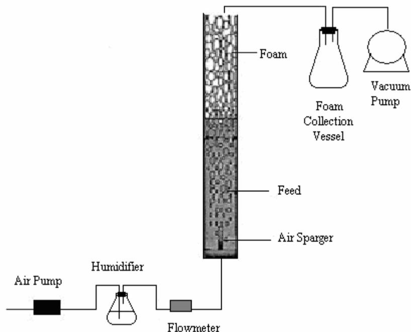
**Figure 2.1** Foam Fractionation Column
