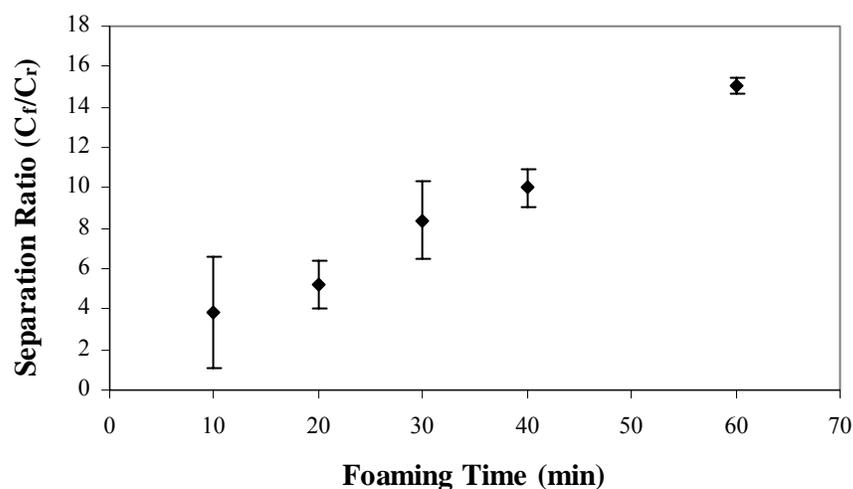
**Figure 3.13** Effect of foaming time on separation ratio (at room temperature: 20-25°C, air velocity:  $38.5 \pm 1$  cm<sup>3</sup>/min, feed solution concentration: 0.064 mg/ml, feed volume: 250 ml, foaming time: 10-60 min). The points are average of triplicate experiments.
