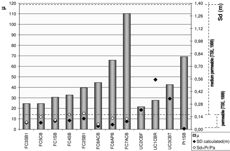
Figure 4.3  $\mu$  values of the samples, in relation to their  $S_D$  values when used with or without primer.
