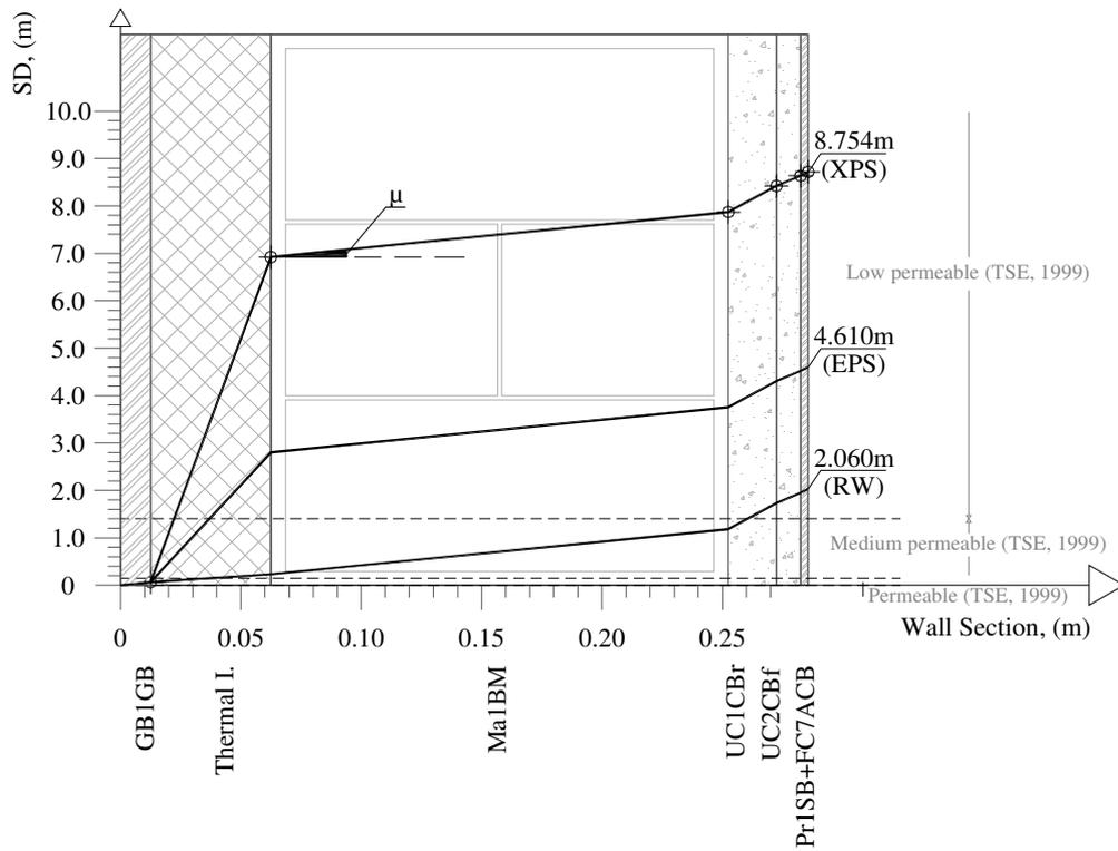
Figure 4.5. Total  $S_D$  values in an internally insulated wall section plastered with  $FC7ACB$ .
