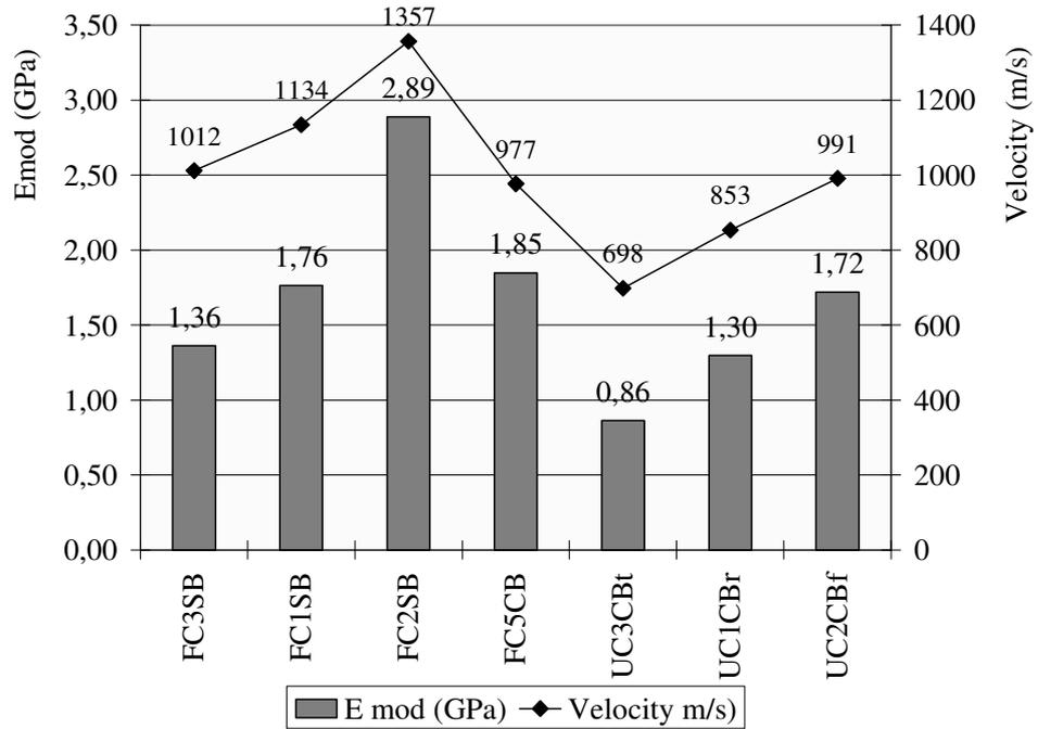
Figure 4.10.  $UPV$  and  $E_{mod}$  values for finish coats and undercoats.
