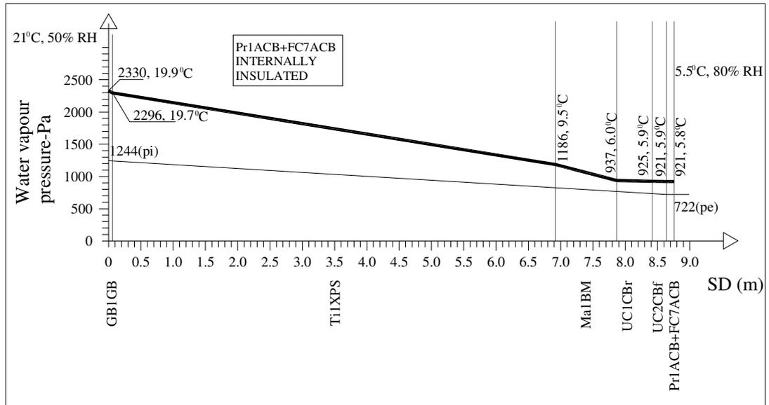
Figure 4.9. Partial ( $p_i$  and  $p_e$ ) and equilibrium ( $p_s$ ) water vapour pressure distribution for an internally insulated wall section coated by  $FC7ACB$ .
