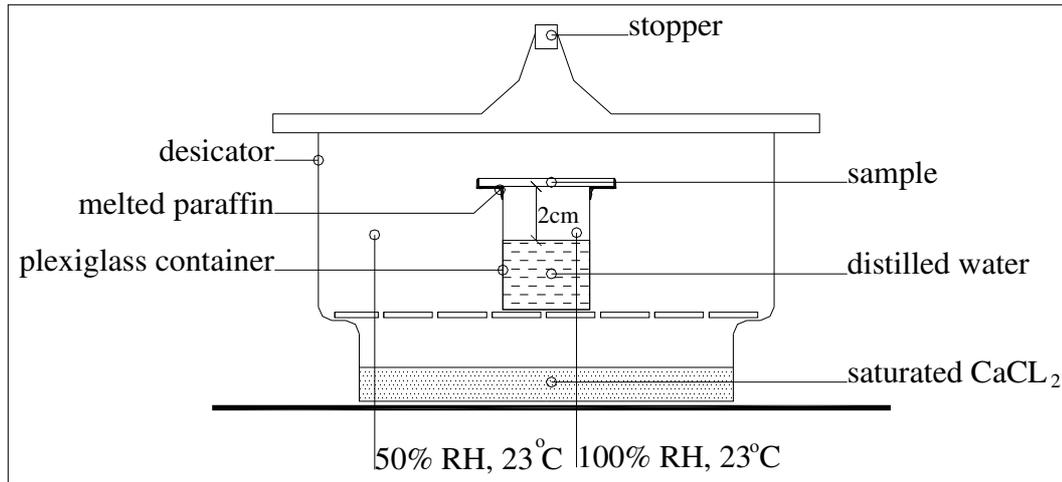
Figure 3.9. The experimental set-up for the analysis of water vapour permeability.
