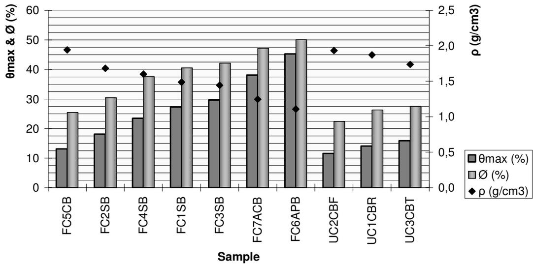
Figure 4.1 Bulk density ( $\rho$ ), porosity ( $\emptyset$ ) and water absorption capacity ( $\theta_{max}$ ) of the samples of finish and undercoats.
