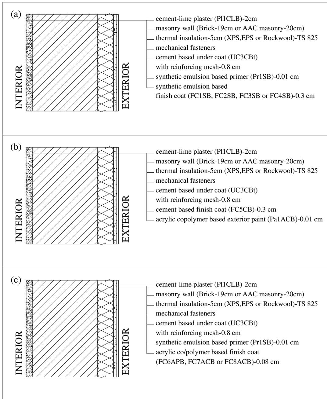
Figure 3.2. Externally insulated single leaf wall plastered with (a) synthetic emulsion-based exterior finish coat (*FC1SB*, *FC2SB*, *FC3SB* or *FC4SB*); (b) cement-based exterior finish coat (*FC5CB*); (c) acrylic polymer-based exterior finish coats (*FC6APB*, *FC7ACB* or *FC8ACB*) (<http://www.kaleterasit.com.tr>, 2006).
