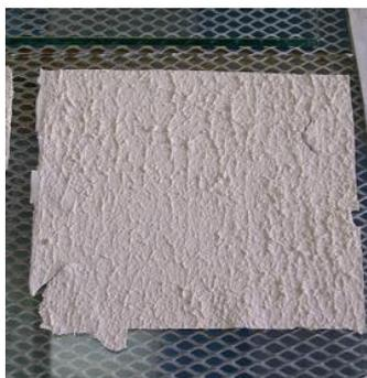
Figure 3.7 Sample of acrylic polymer-based finish coat, *FC6APB*, applied on primer.
