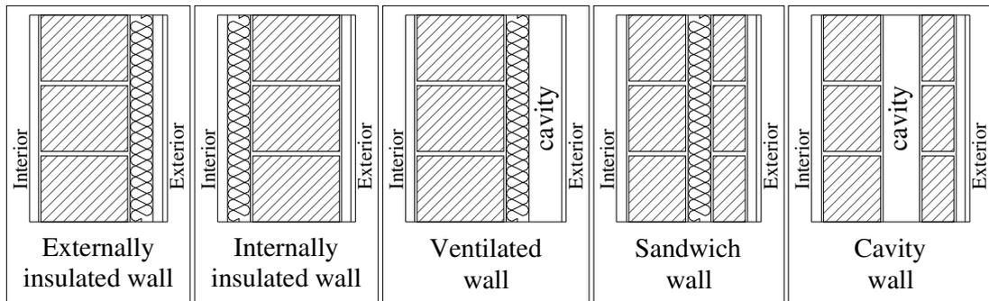
Figure 2.1 Types of external wall (<http://www.izocam.com.tr>, 2006).
