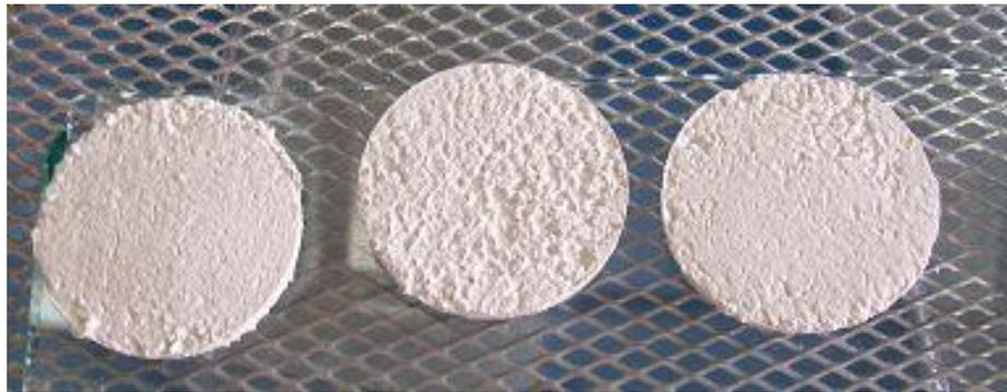
Figure 3.6 Samples of cement-based finish coat, *FC5CB*, after painting.
