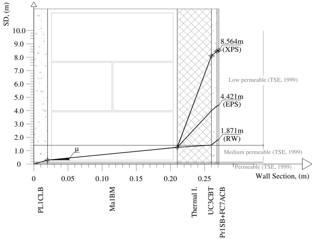
Figure 4.4. Total  $S_D$  values in an externally insulated wall section plastered with  $FC7ACB$ .
