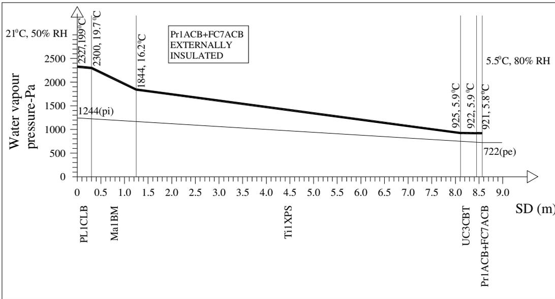
Figure 4.8. Partial ( $p_i$  and  $p_e$ ) and equilibrium ( $p_s$ ) water vapour pressure distribution for an externally insulated wall section coated by *FC7ACB*.
