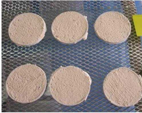
Figure 3.5 Samples of synthetic emulsion-based finish coats, *FC1SB*, with (at top) and without (at bottom) primer.
