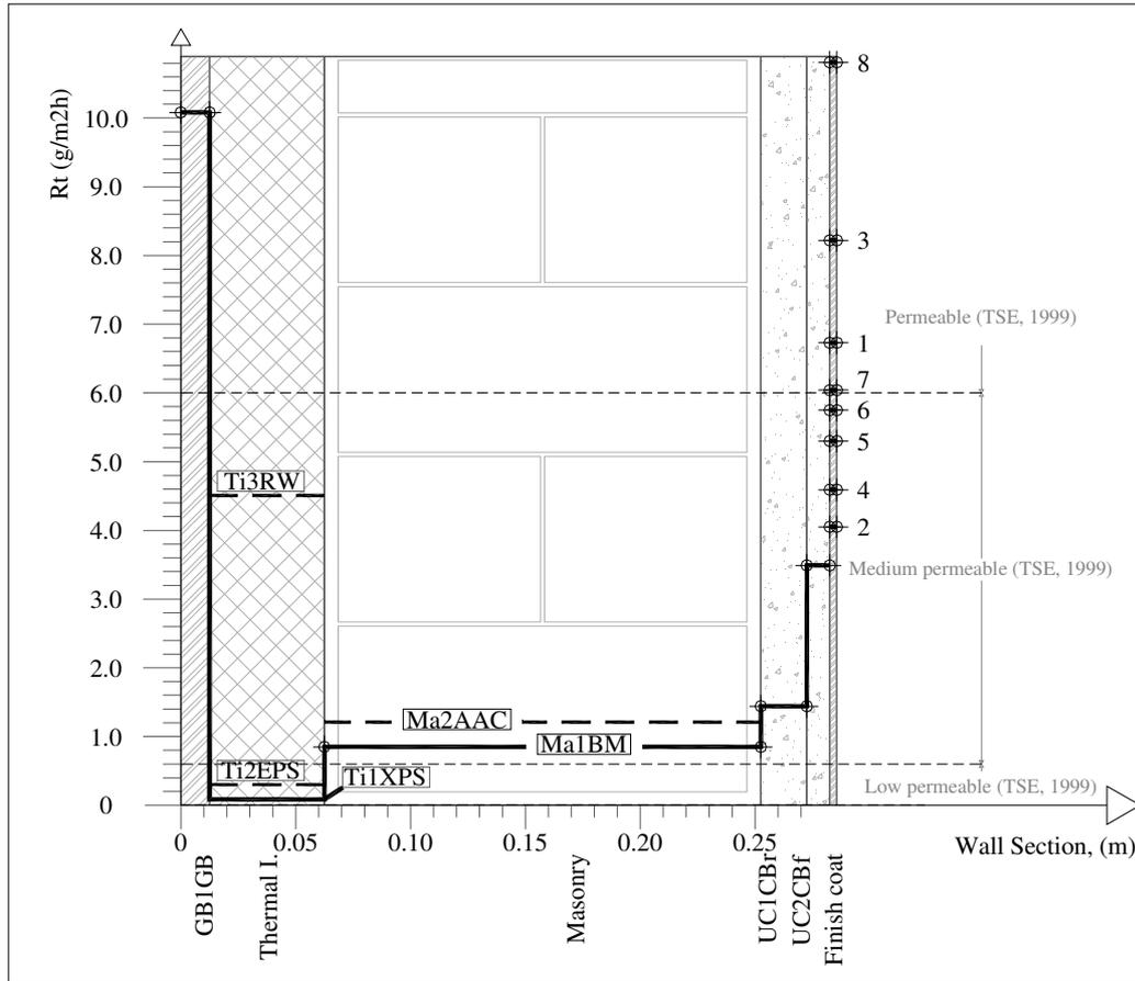
Figure 4.7. RT values for each layer of an internally insulated wall section. The numerical arrangement in the external face presented the sample number of finish coat, for example FC3SB is presented by 3.
