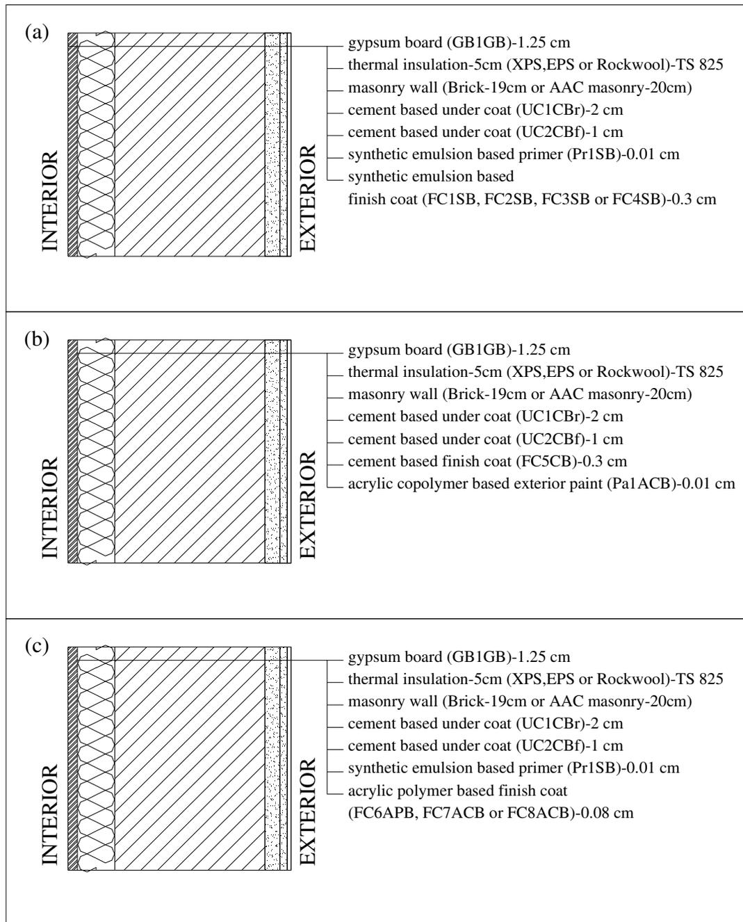
Figure 3.3. Internally insulated single leaf wall plastered with (a) synthetic emulsion-based exterior finish coat (*FC1SB*, *FC2SB*, *FC3SB* or *FC4SB*); (b) cement-based exterior finish coat (*FC5CB*); (c) acrylic polymer-based exterior finish coat (*FC6APB*, *FC7ACB* or *FC8ACB*) (<http://www.kaleterasit.com.tr>, 2006).
