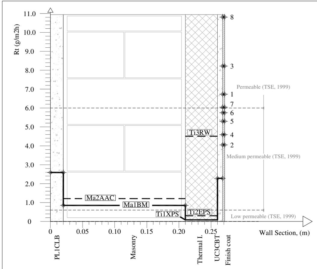
Figure 4.6.  $R_T$  values for each layer of an externally insulated wall section. The numerical arrangement in the external face presented the sample number of finish coat, for example  $FC3SB$  is presented by 3.
