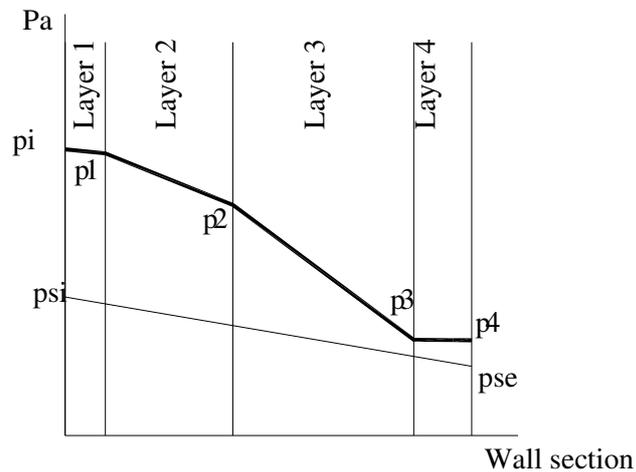
Figure 3.10. Partial and equilibrium water vapour pressure distribution in a wall where, there is no risk of condensation.
