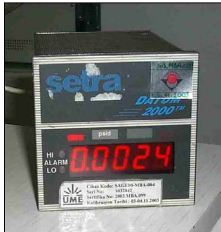
Figure 5 Pressure Transducer and Manometer
