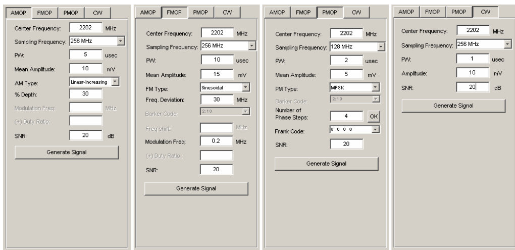
Figure B.3. Details of the Signal Generator.
