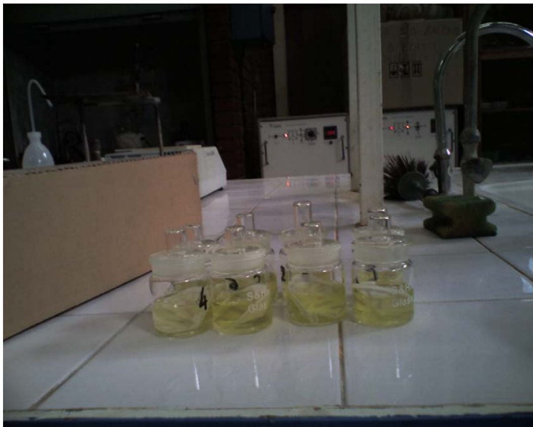
Figure 3.8: Filter papers immersed in %90 pure ethanol solution (notice the green color due to Chl-a extracted into the ethanol)
