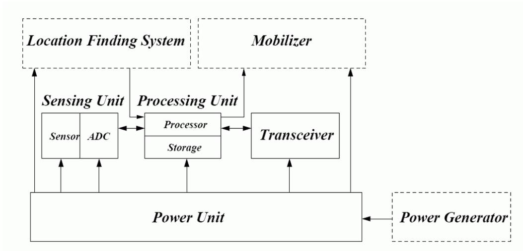
**Figure-3** Block diagram of a sensor node [1]
