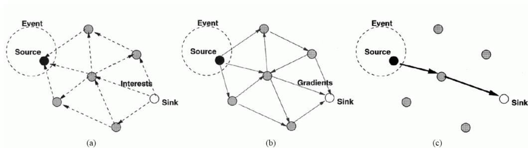
**Figure-7** Directed Diffusion - (a) Interest propagation. (b) Initial gradients setup. (c) Data delivery along reinforced path. [4]
