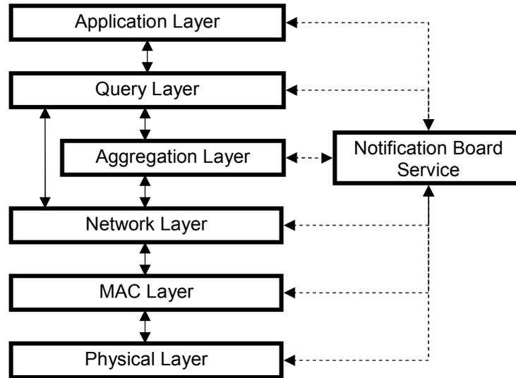
**Figure-1** The sensor network stack proposed in this thesis
