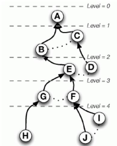
**Figure-6** TAG routing tree [3]
