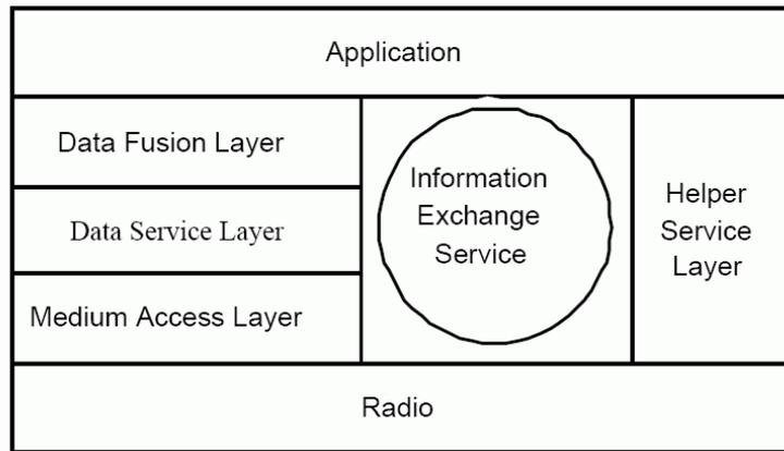
**Figure-5** SensorStack layers [8]
