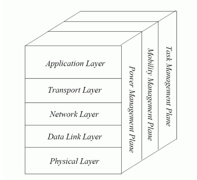
**Figure-4** Sensor network protocol stack of Akyildiz et.al.[1]
