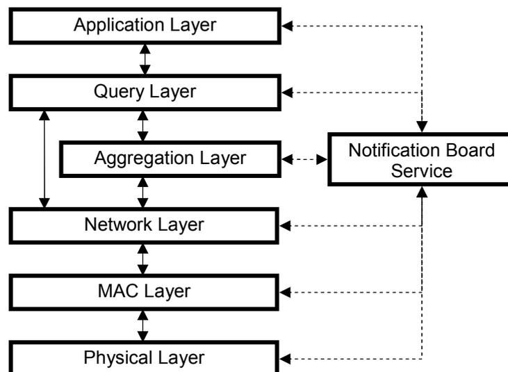
**Figure-11** The new sensor network protocol stack
