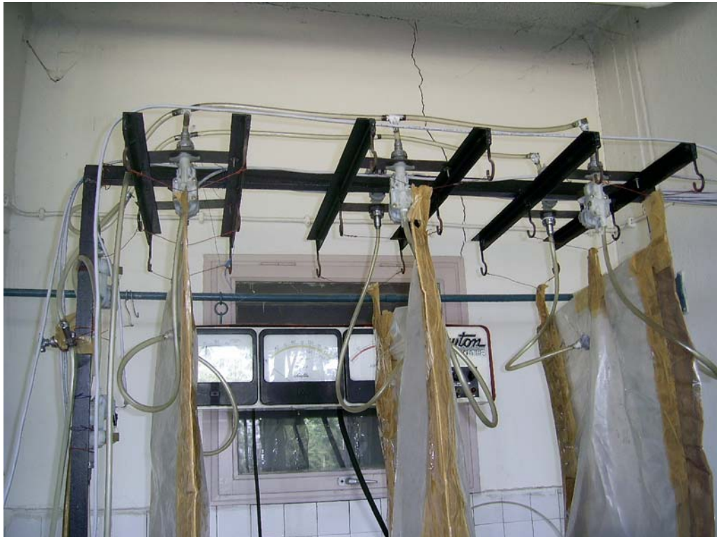
Figure 3.5.1: Nylon bags and solenoid valves on them
