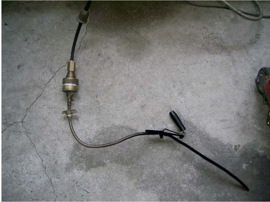
Figure 3.5.3: AVL gas analyzer's gaseous emissions measurement probe and filter holder on it.
