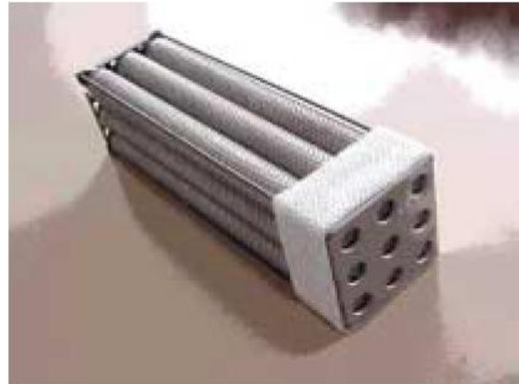
Figure 2.3.4.4.1: Knitted Fiber Filter (Mayer, 2003).
