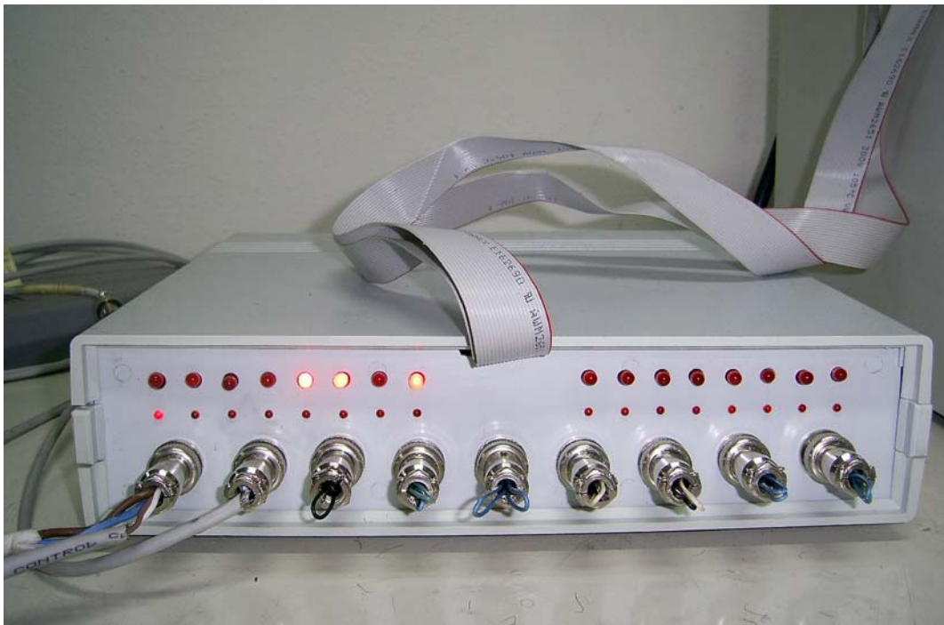
Figure 3.6.3: Front of the input-output control box.
