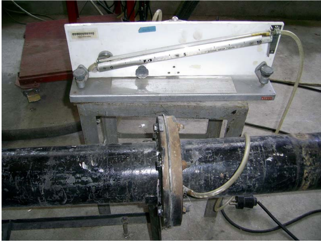
Figure 3.3.2: Manometer connected to orifice on dilution tunnel (DT).
