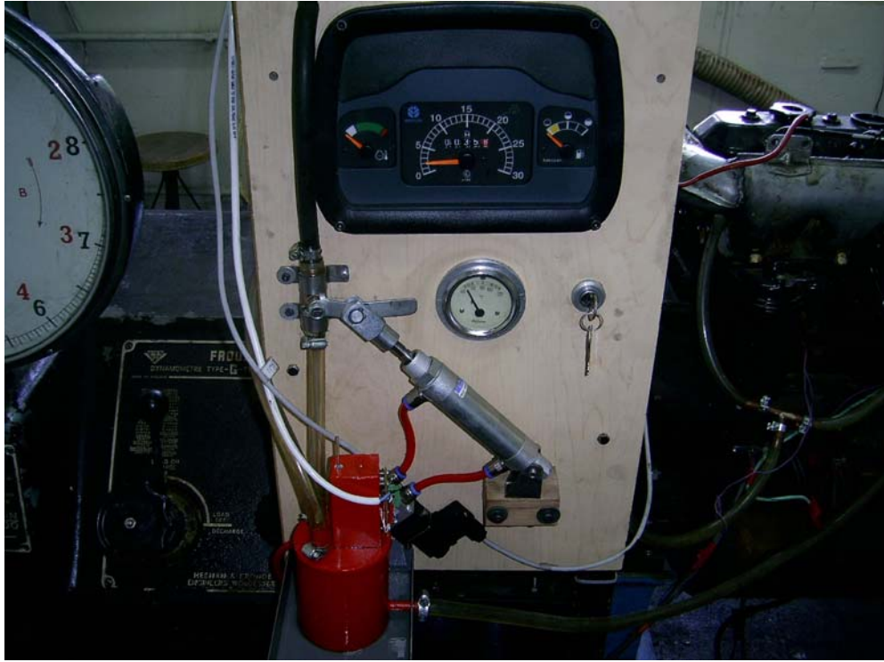
Figure 3.2.1: Control panel of the engine.
