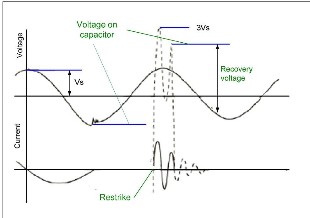
Figure 3.2 – Current and voltage relation at capacitive current interruption
