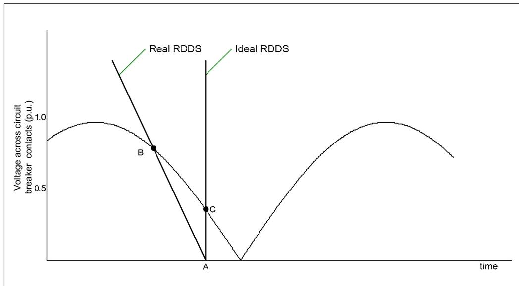
Figure 2.6 – RDDS characteristics of circuit breakers
