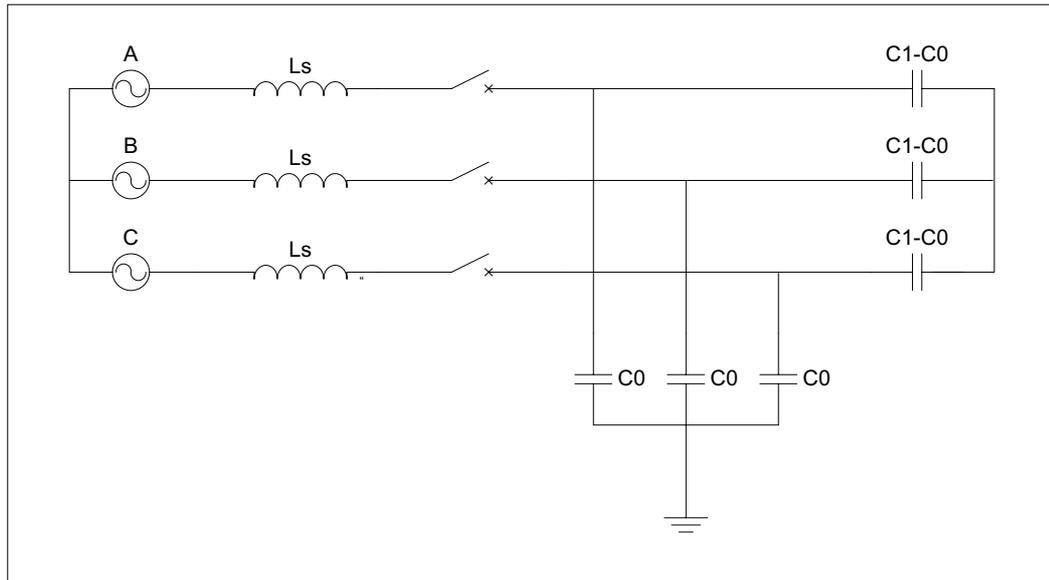
Figure 3.3 – Unloaded overhead line three phase representation
