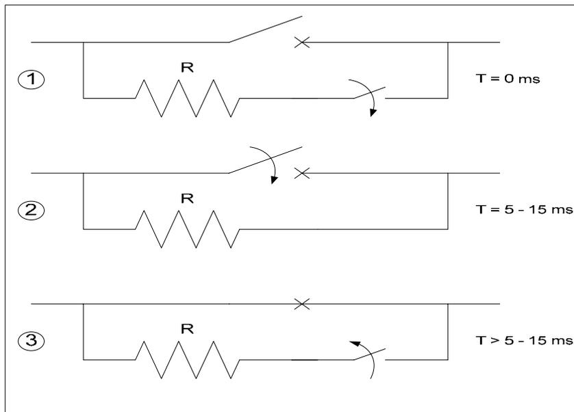
Figure 2.9 – Operation sequence of closing resistor
