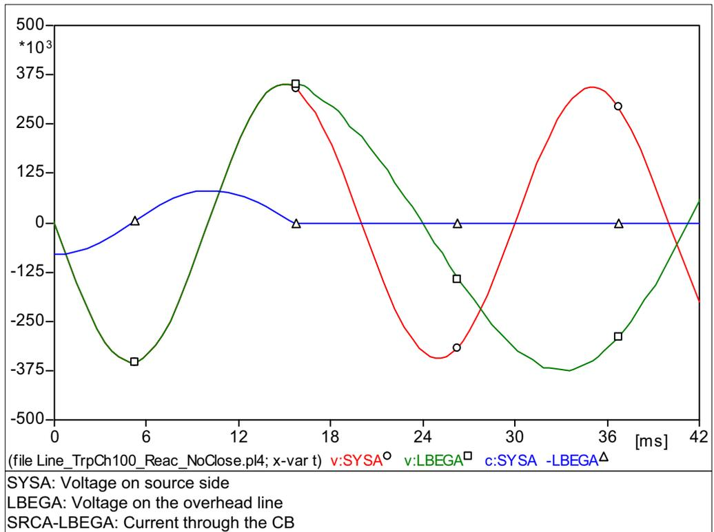
Figure 3.6 – Current and voltage relation in compensated overhead line
