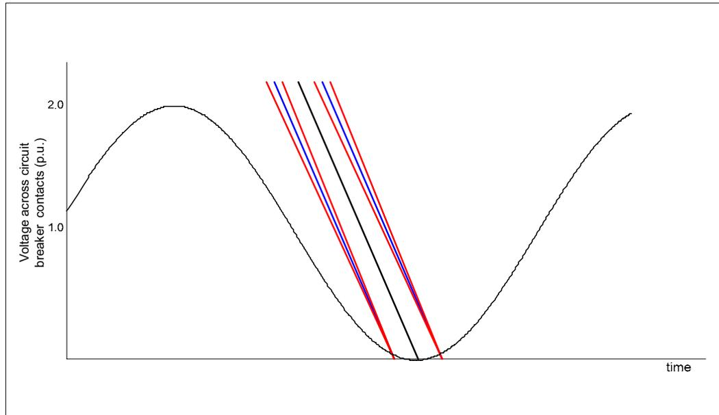
*Figure 4.8 – Target instant for non-compensated unloaded OHL with trapped charge of 1 p.u.*
