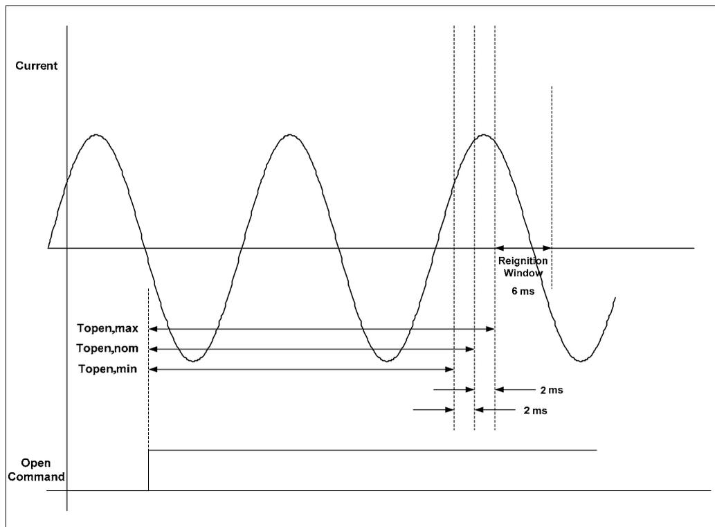
Figure 4.3 – Reignition window for controlled shunt reactor switching
