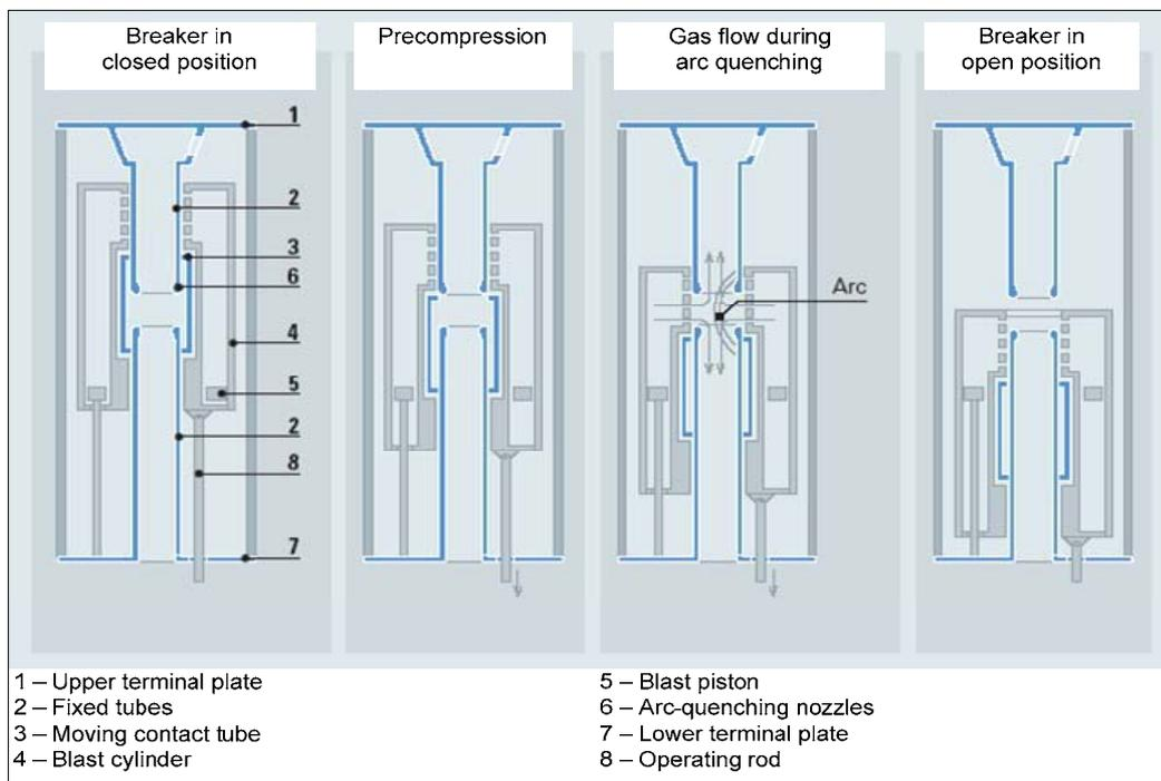
Figure 2.1 – Basic scheme of HV circuit breaker interrupter
