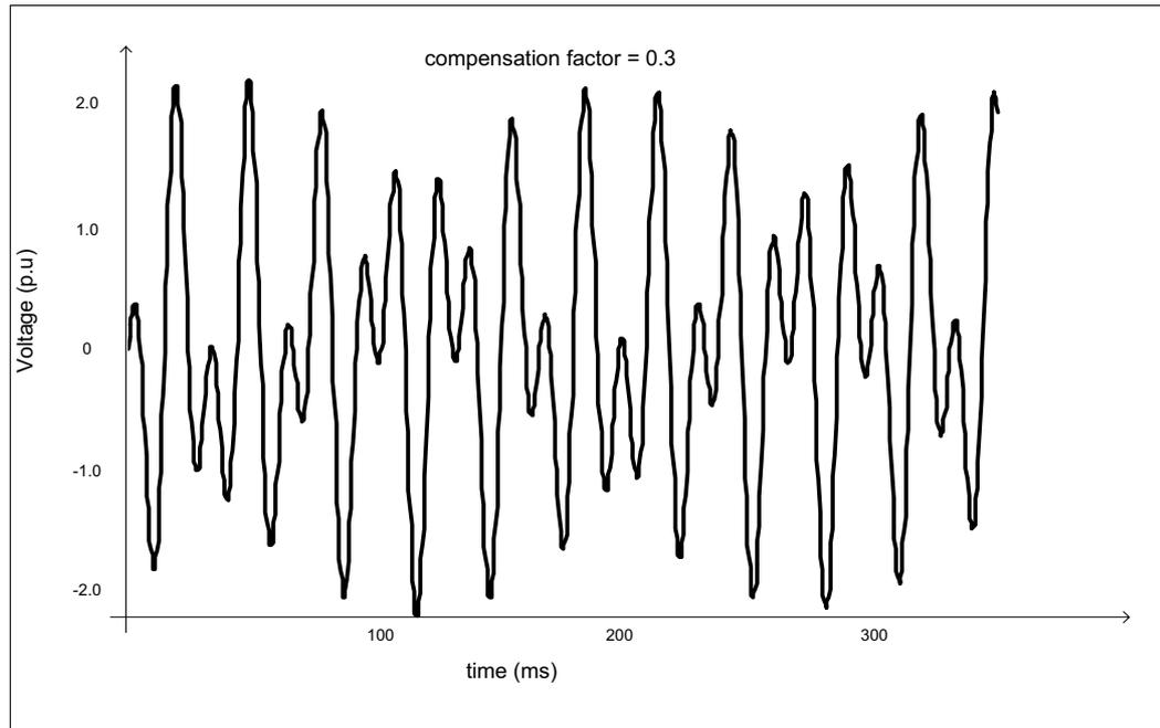
*Figure 4.10 – Voltage across circuit breaker for compensated line with trapped charge ( $k=0.3$ )*
