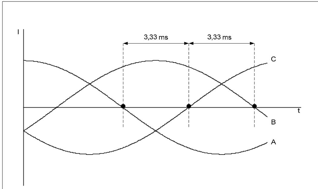
*Figure 4.4 – Sequence of current zero instants directly grounded shunt reactors*
