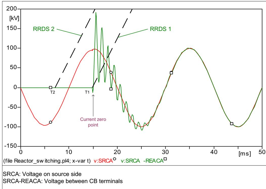
Figure 2.5 – Recovery voltage for inductive load case
