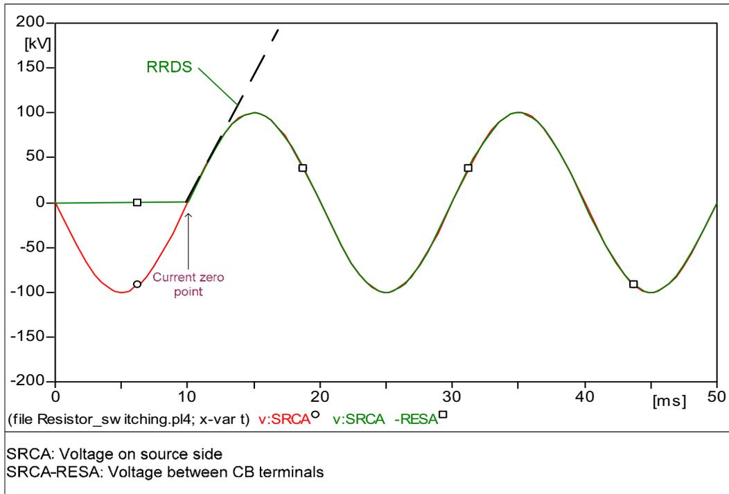
Figure 2.3 – Recovery voltage for resistive load case
