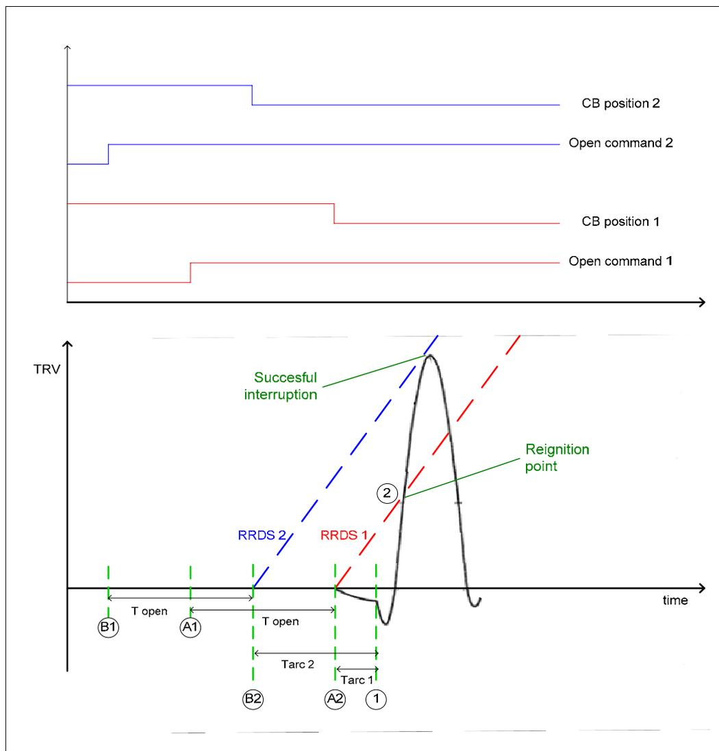
Figure 4.2 – Controlled switching example for shunt reactor opening
