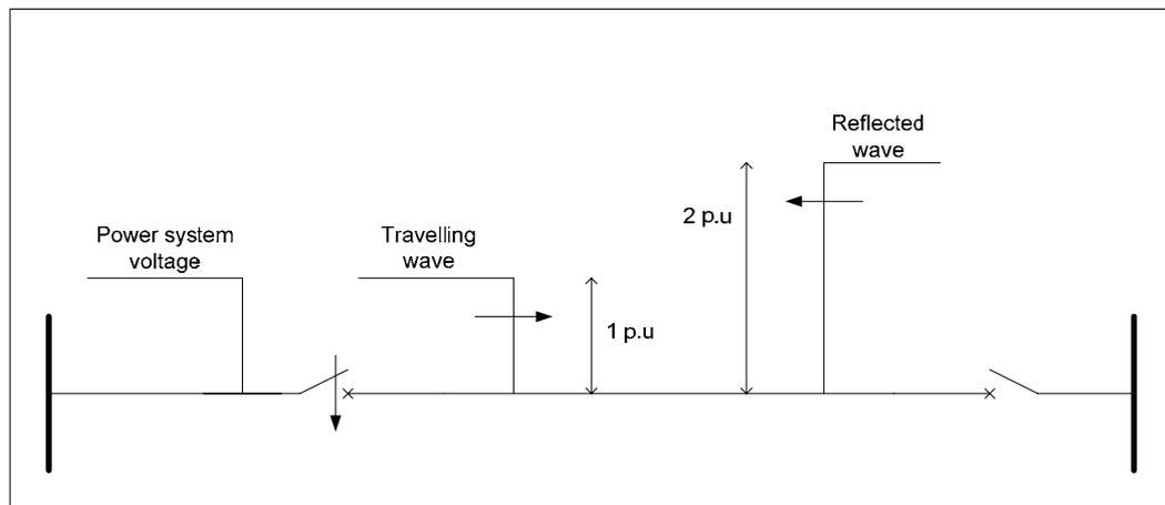
*Figure 3.8 – Travelling wave reflection from open line end*
