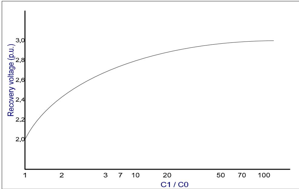
Figure 3.4 – Recovery voltage peak in the FPTC as a function of C1/C0
