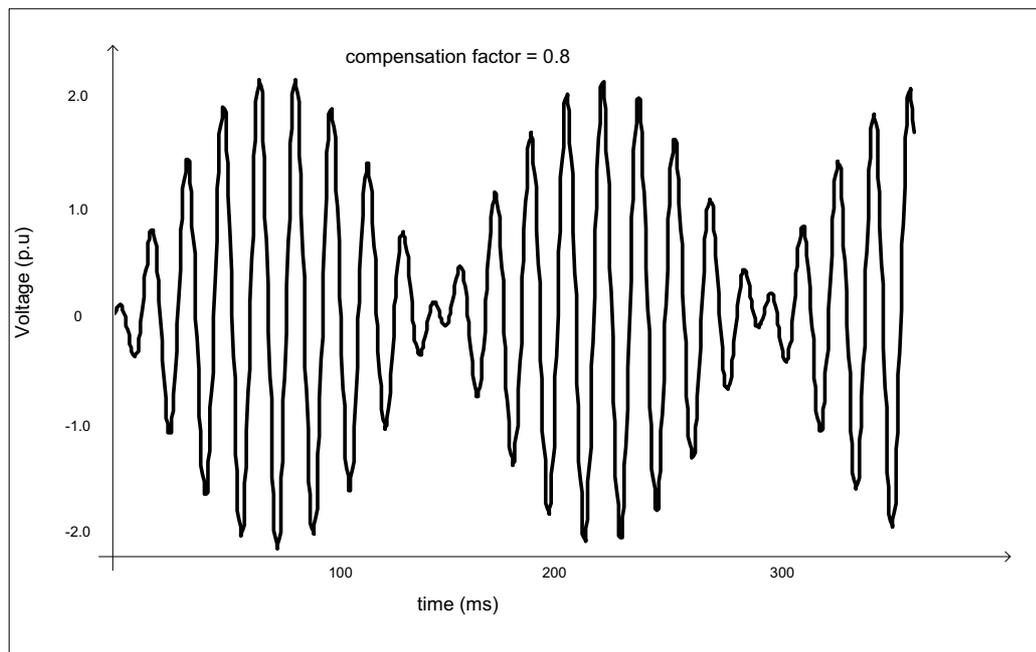
*Figure 4.9 – Voltage across circuit breaker for compensated line with trapped charge ( $k=0.8$ )*
