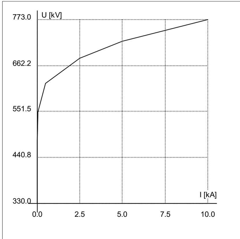
Figure A.4 – Surge arrester characteristics
