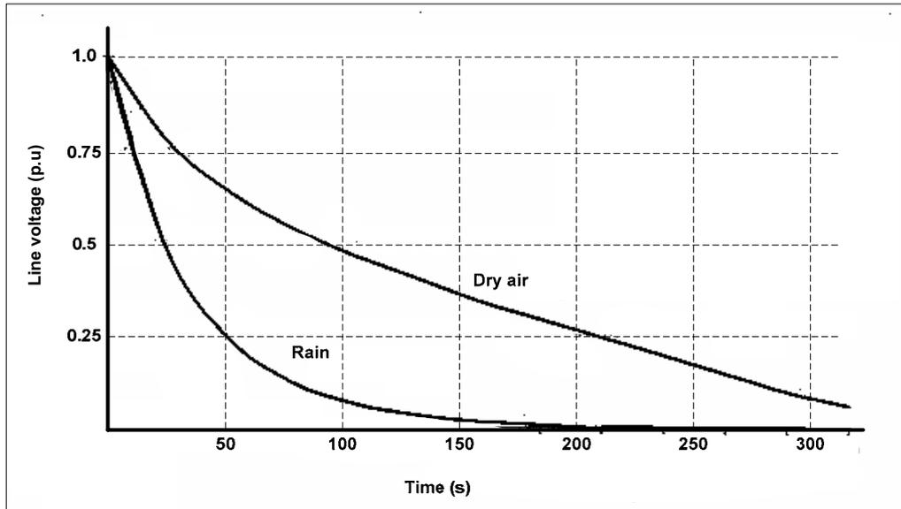
Figure 3.9 – Decay of trapped charge on an unloaded overhead line
