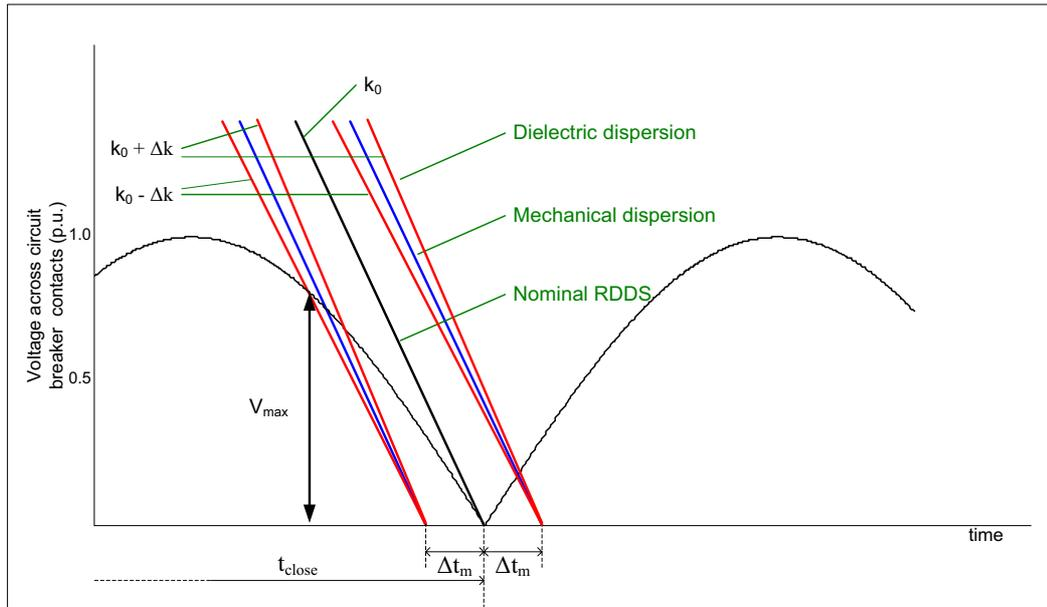
Figure 4.5 – Closing time variation in voltage zero target
