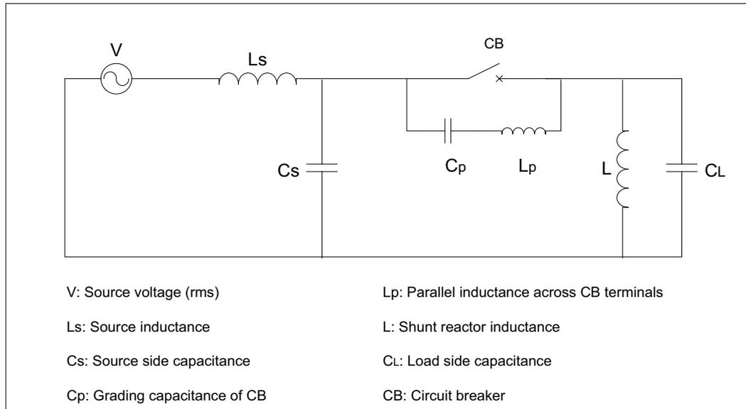
Figure 3.10 – Single phase equivalent circuit of inductive current interruption
