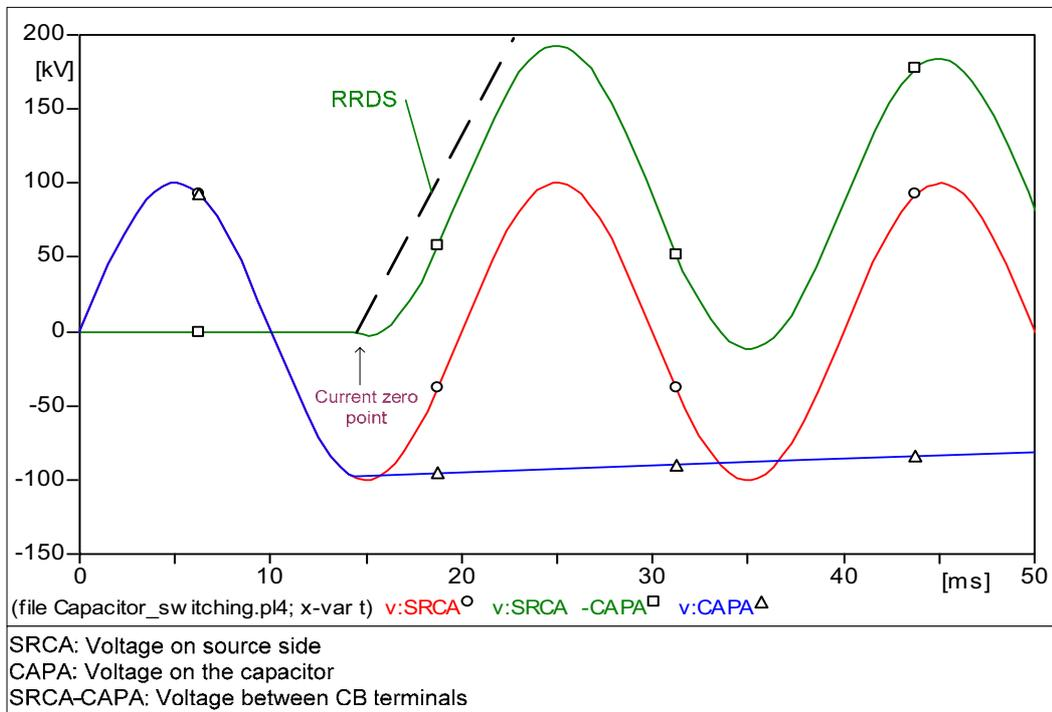
Figure 2.4 – Recovery voltage for capacitive load case
