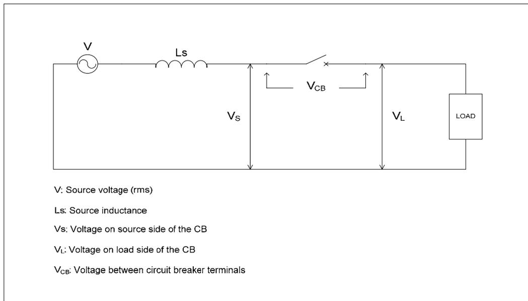
Figure 2.2 – Example circuit for recovery voltage on a circuit breaker
