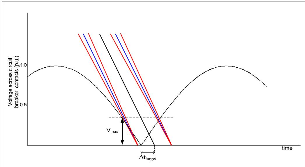
Figure 4.6 – Target shifting for minimum making voltage
