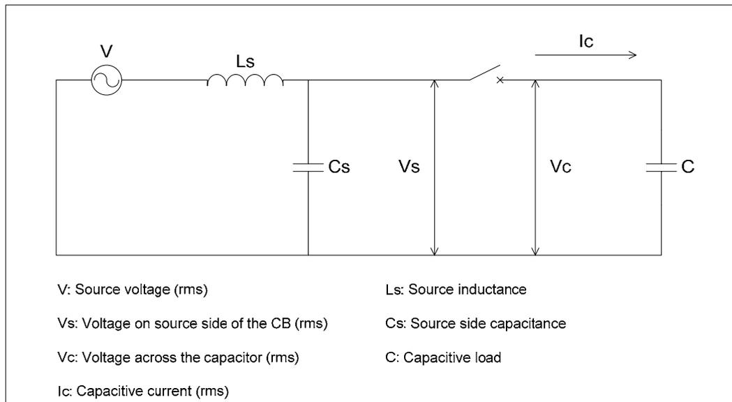
*Figure 3.1 – Single phase equivalent circuit of capacitive current switching*
