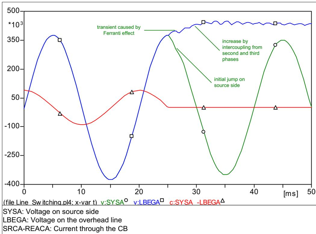
Figure 3.5 – Voltage and current waveforms after overhead line deenergising
