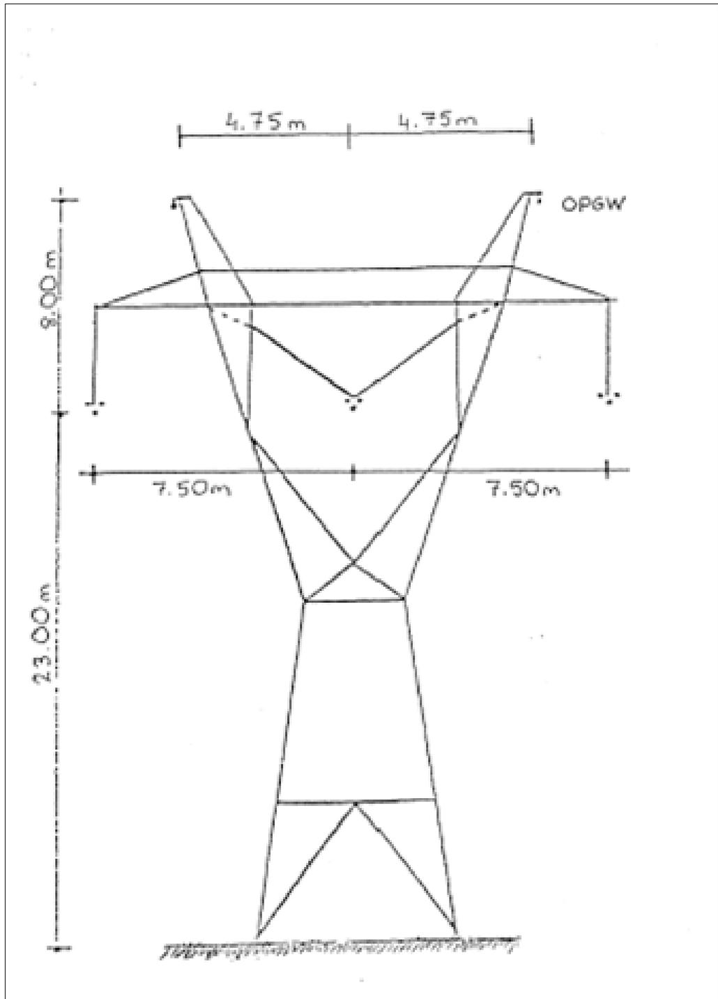
Figure A.1 – Overhead line tower data
