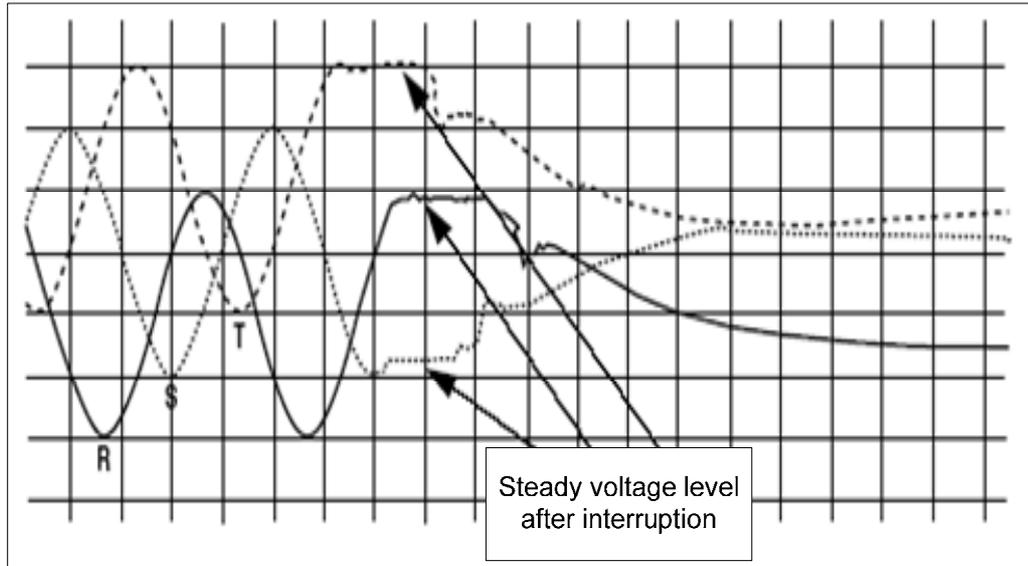
*Figure 4.7 – Voltage measurements from a CVT at opening of a healthy OHL*
