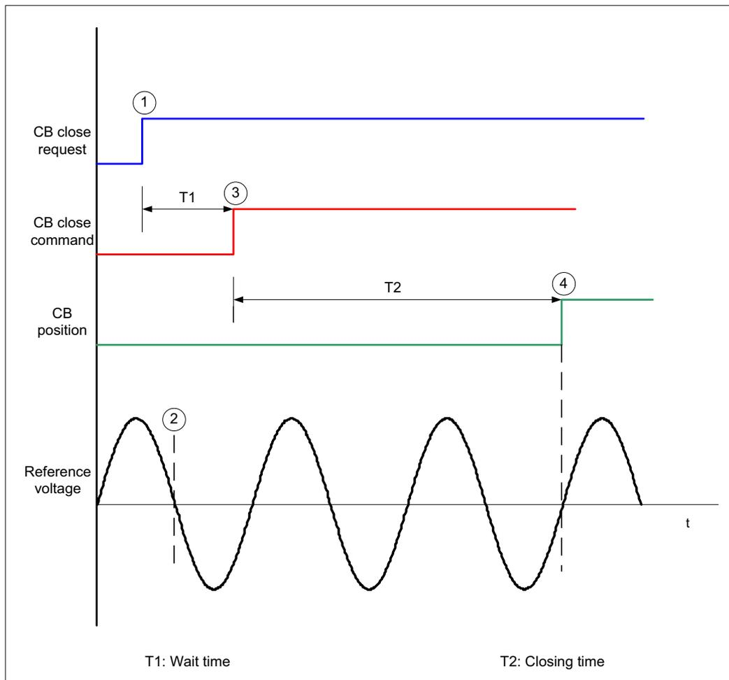
Figure 4.1 – Controlled switching example
