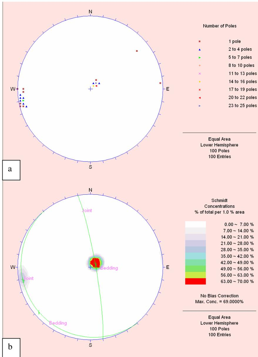
Figure 4.34 Pole plot (a) and contour plot (b) of the discontinuities in the Tirtar middle and lower level quarry.
