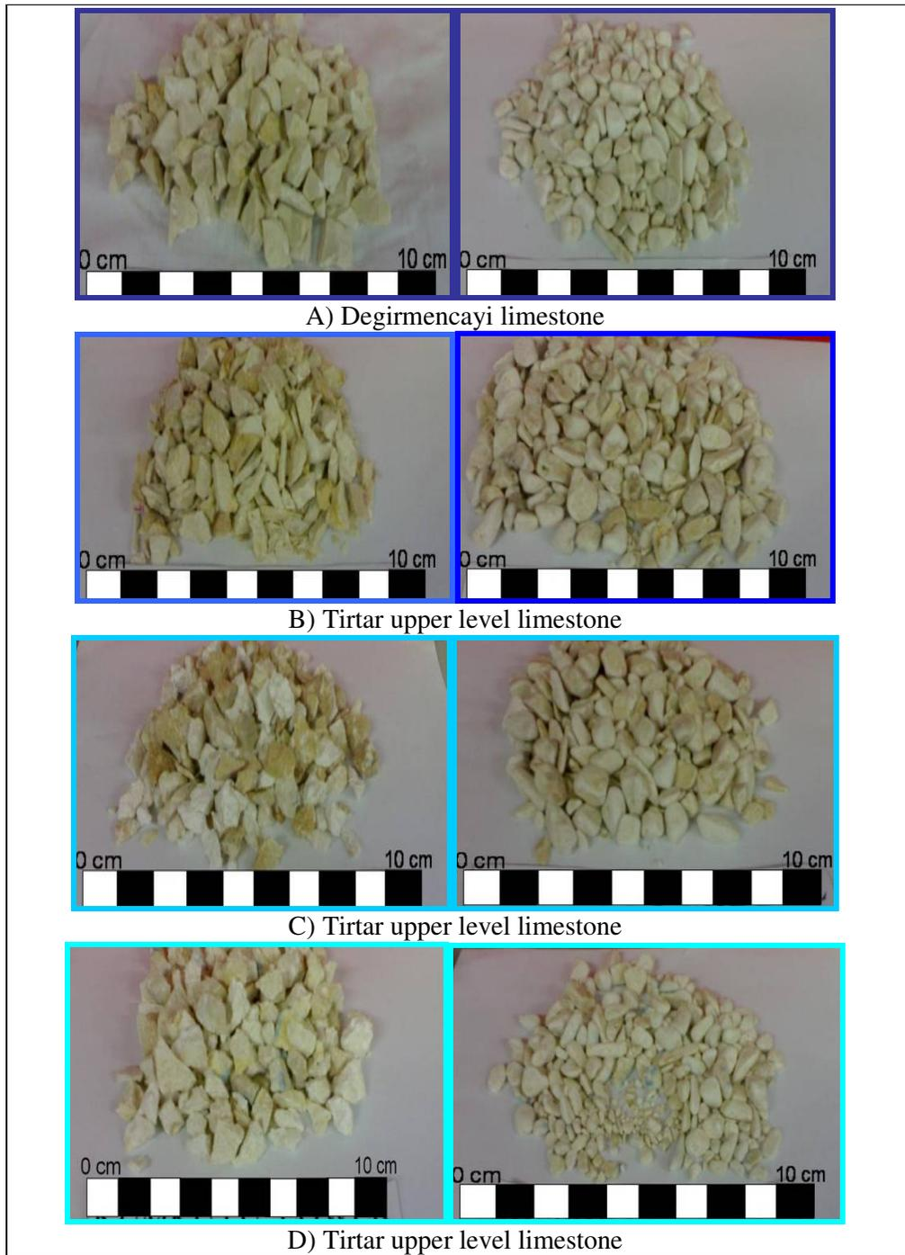
Figure 4.27 The physical appearance of limestones after Micro-Deval test. Fresh reference sample is placed at the left side of the photograph.
