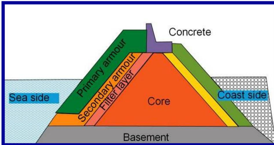
Figure 3.1 Simplified cross section of a rubble mound breakwater.
