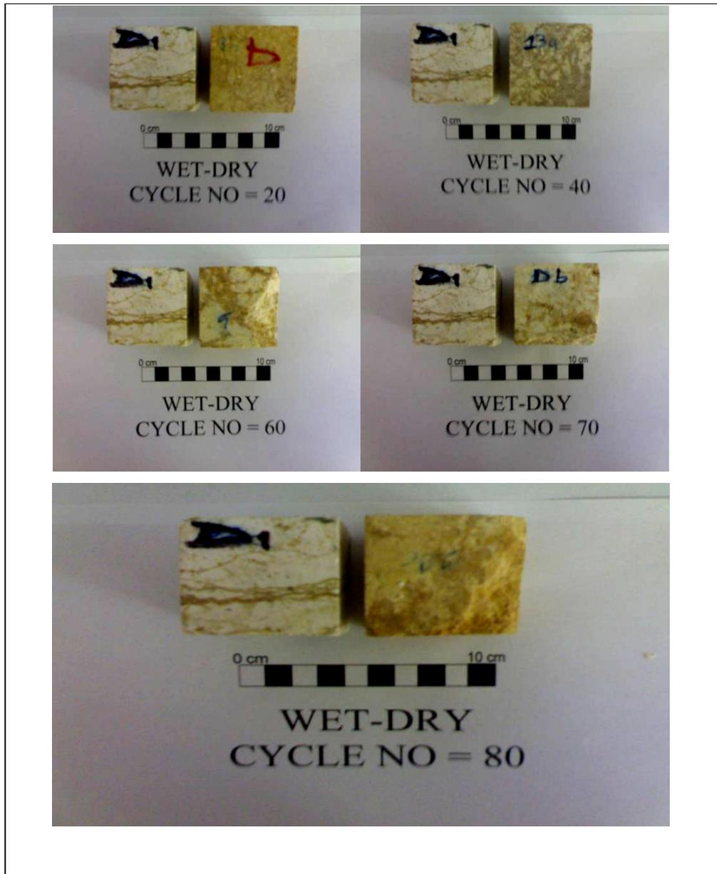
Figure 4.9 Physical appearance of the Tirtar middle level limestone subjected to 80 wetting-drying test cycles. The sample at the left side of the photograph is a fresh reference sample.
