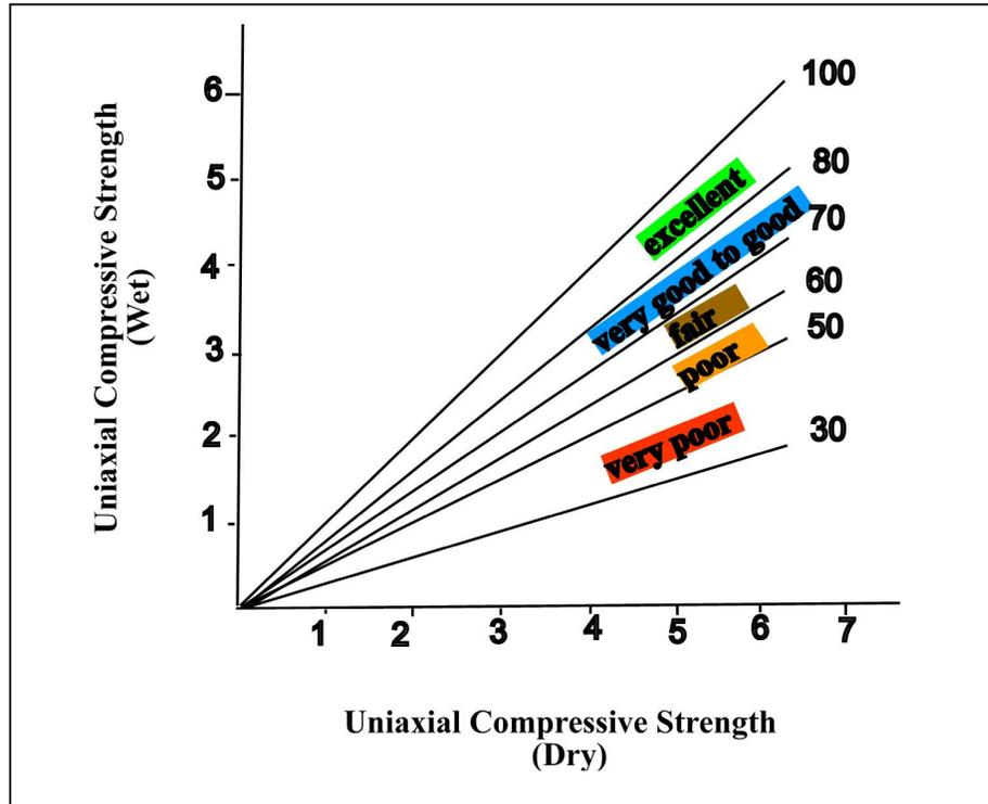
Figure 5.1 Durability evaluations of stone based on the wet-to-dry strength ratio (after Winkler, 1986).
