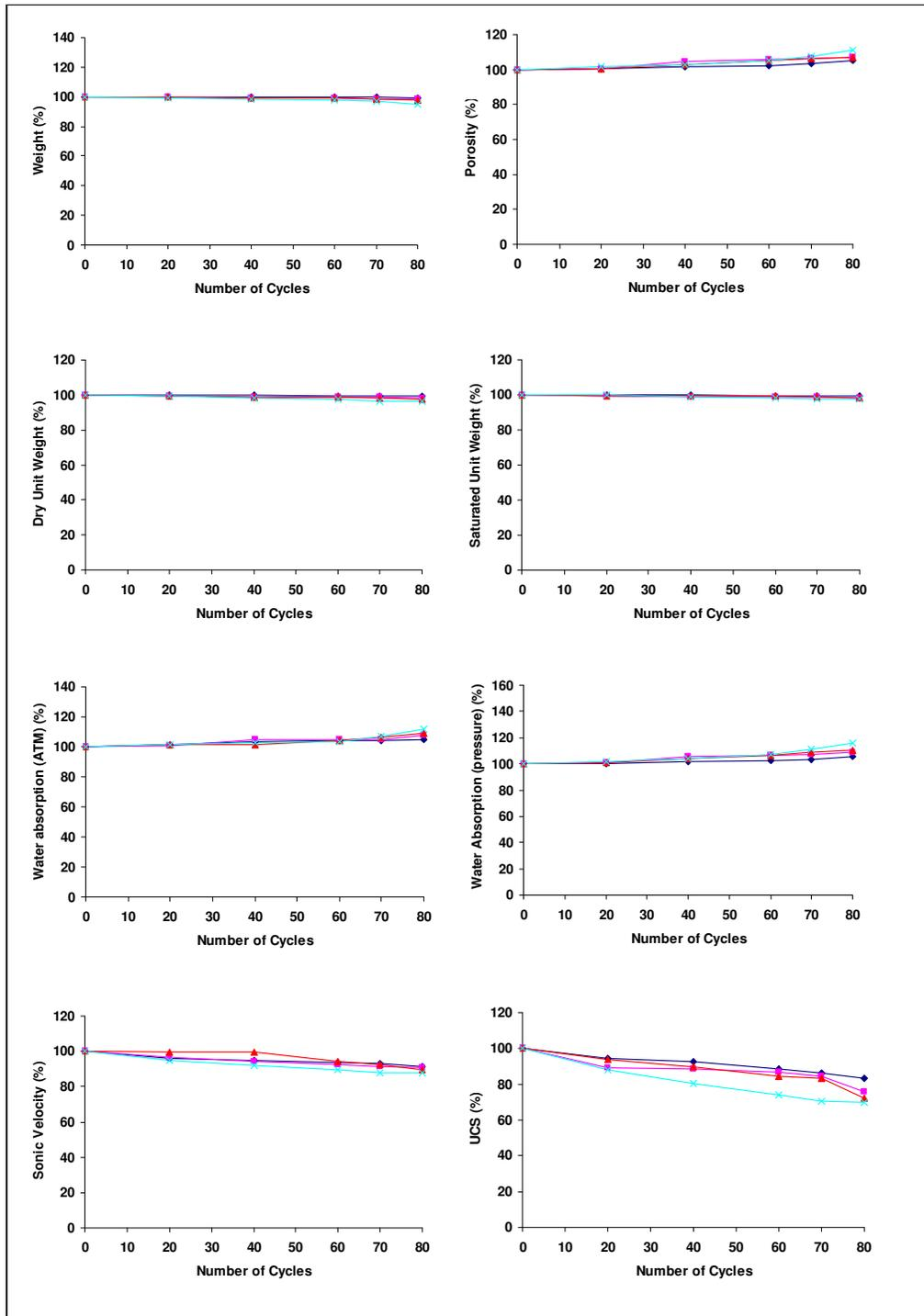
Figure 4.6 Variation of the physico-mechanical properties of the limestone after wetting-drying tests (blue line shows Değirmençayı limestone, pink line shows Tirtar upper level limestone, red line shows Tirtar middle level limestone, turquoise line shows Tirtar lower level limestone)
