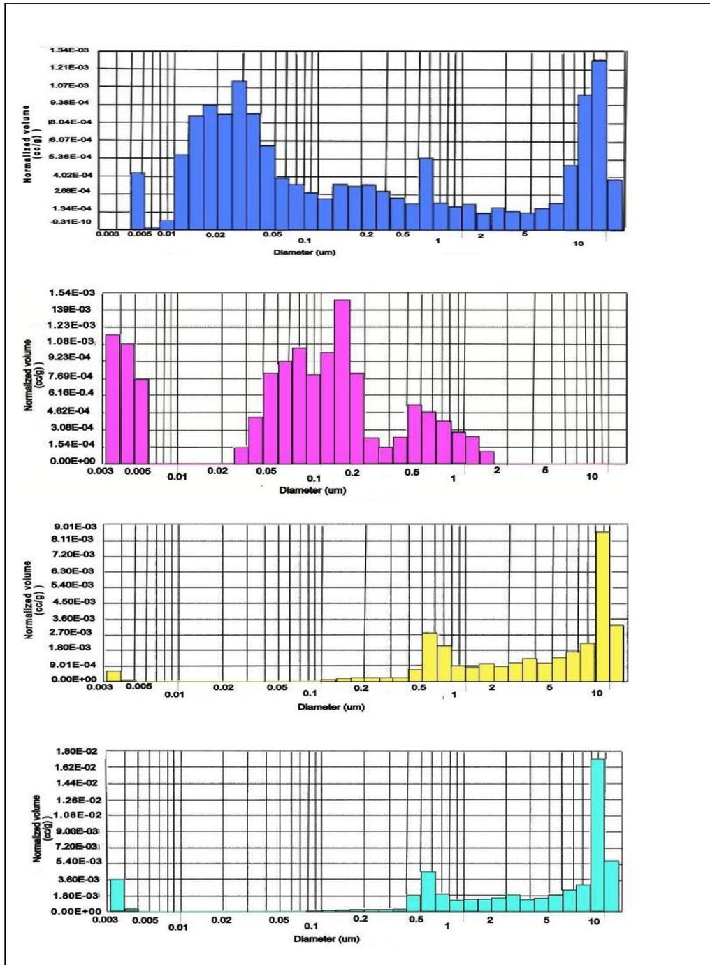
Figure 4.29 Pore size distributions of the four fresh limestone samples.
