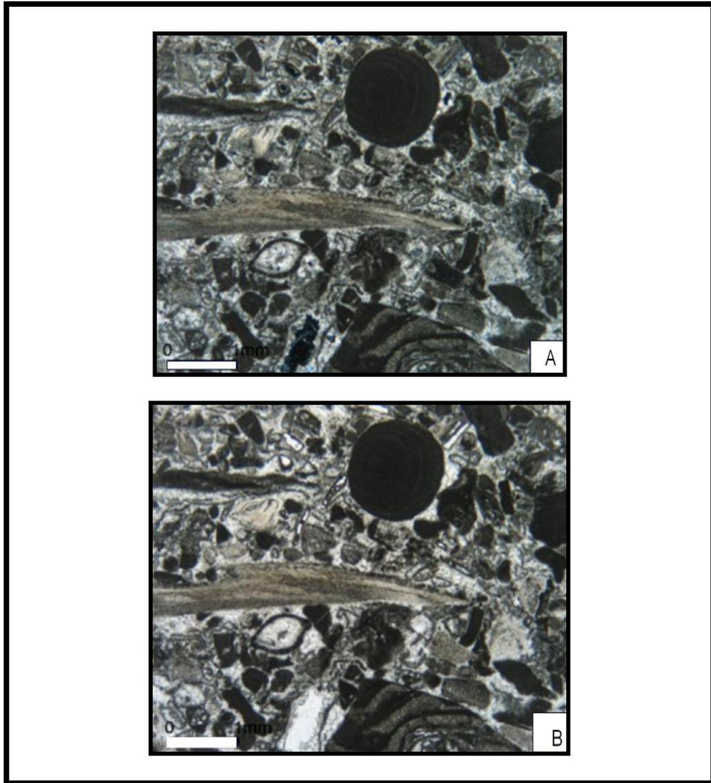
Figure 2.4 Photomicrographs of the Tirtar upper level limestone (A) Plain polarized light (PPL)x5, (B) Cross polarized light (CPL)x5
