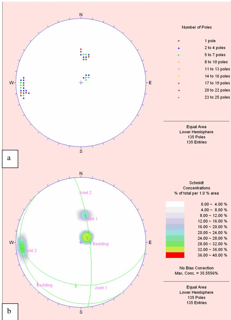
Figure 4.33 Pole plot (a) and contour plot (b) of the discontinuities in the Tirtar upper level quarry.
