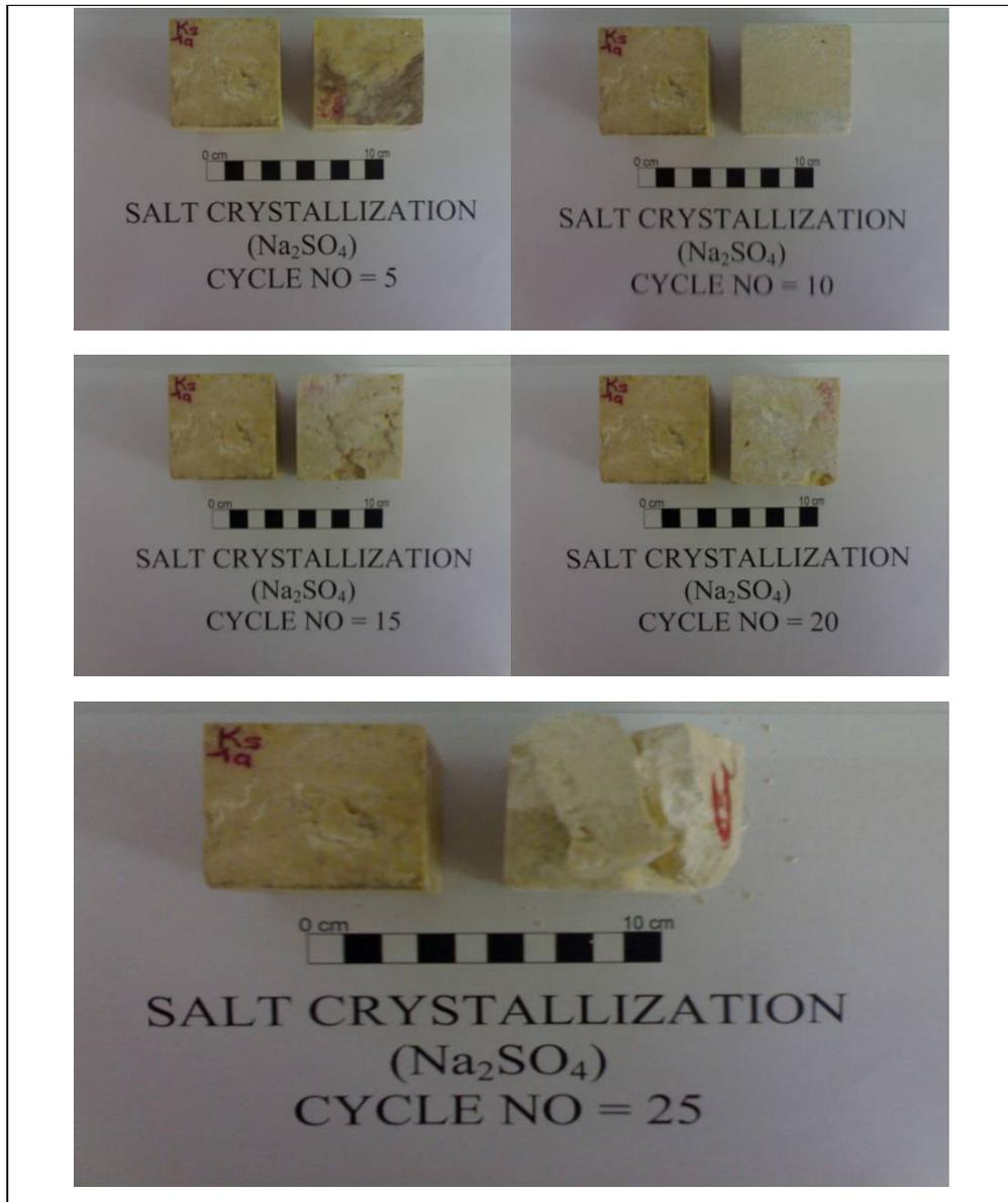
Figure 4.23 Physical appearance of the Tirtar upper level limestone subjected to 25 salt crystallization ( $\text{Na}_2\text{SO}_4$ ) test cycles. The sample at the left side of the photograph is a fresh reference sample.
