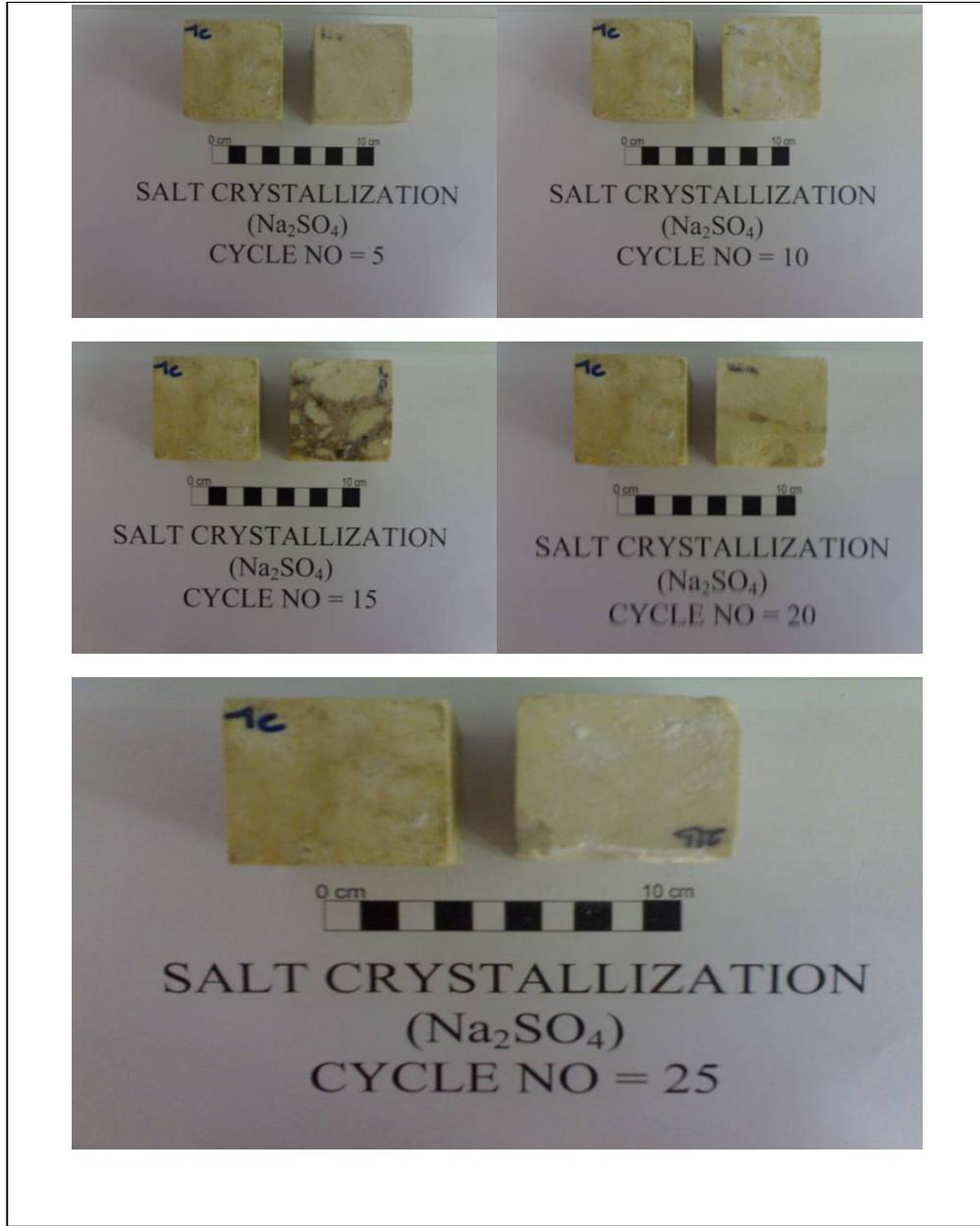
Figure 4.22 Physical appearance of the Değirmençayı limestone subjected to 25 salt crystallization ( $\text{Na}_2\text{SO}_4$ ) test cycles. The sample at the left side of the photograph is a fresh reference sample.
