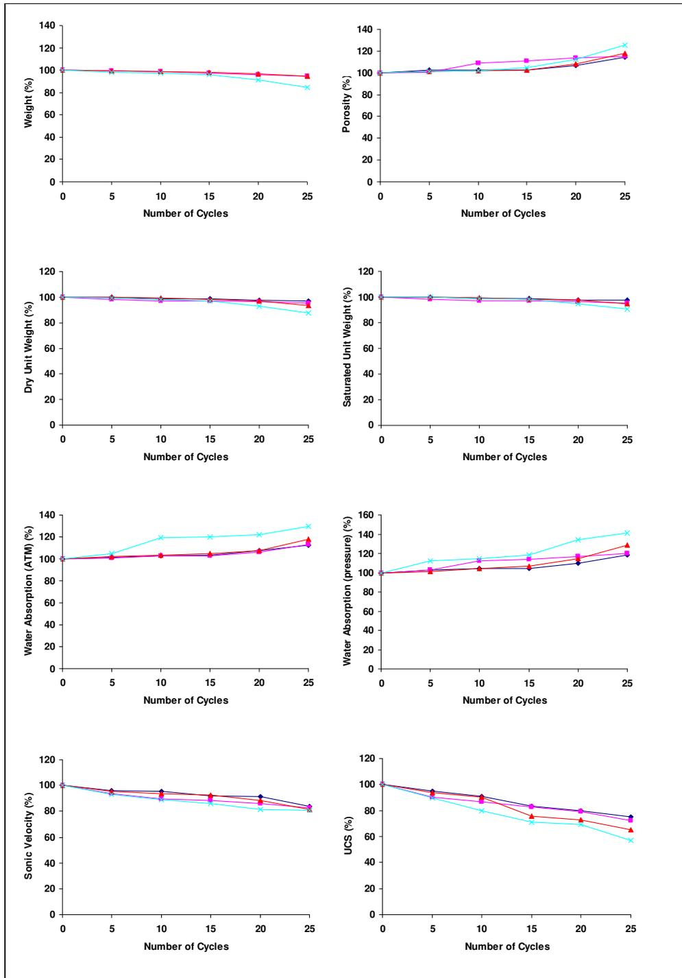
Figure 4.21 Variation of physico-mechanical properties of the limestones after  $\text{Na}_2\text{SO}_4$  salt crystallization tests (blu line shows Değirmençayı limestone, pink line shows Tirtar upper level limestone, red line shows Tirtar middle level limestone, turquoise line shows Tirtar lower level limestone).
