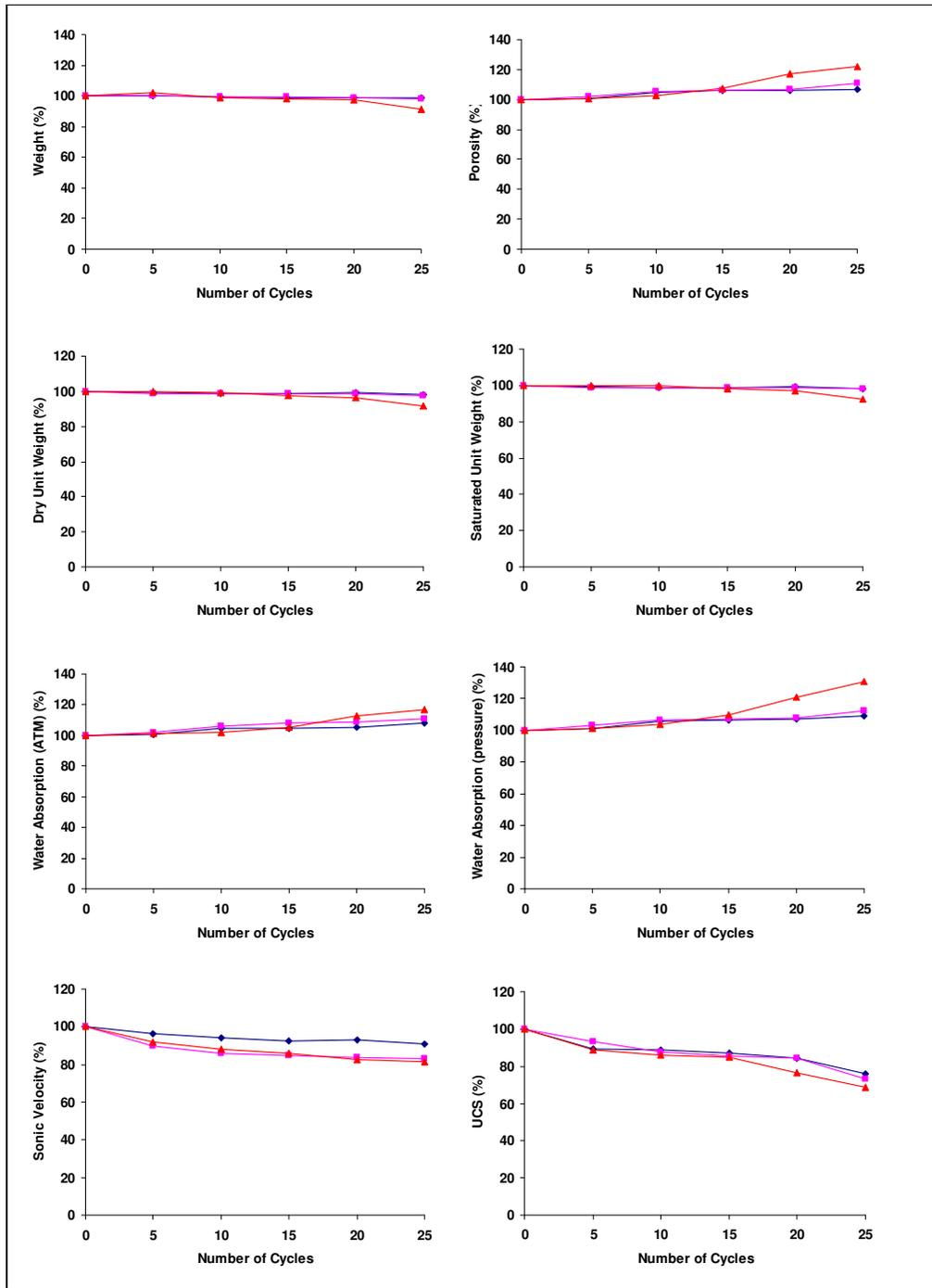
Figure 4.36 Effect of durability tests on the physical and mechanical properties of the Tirtar upper level limestone (blue line shows wet-dry; pink line shows freeze-thaw and the red line shows salt crystallization test).
