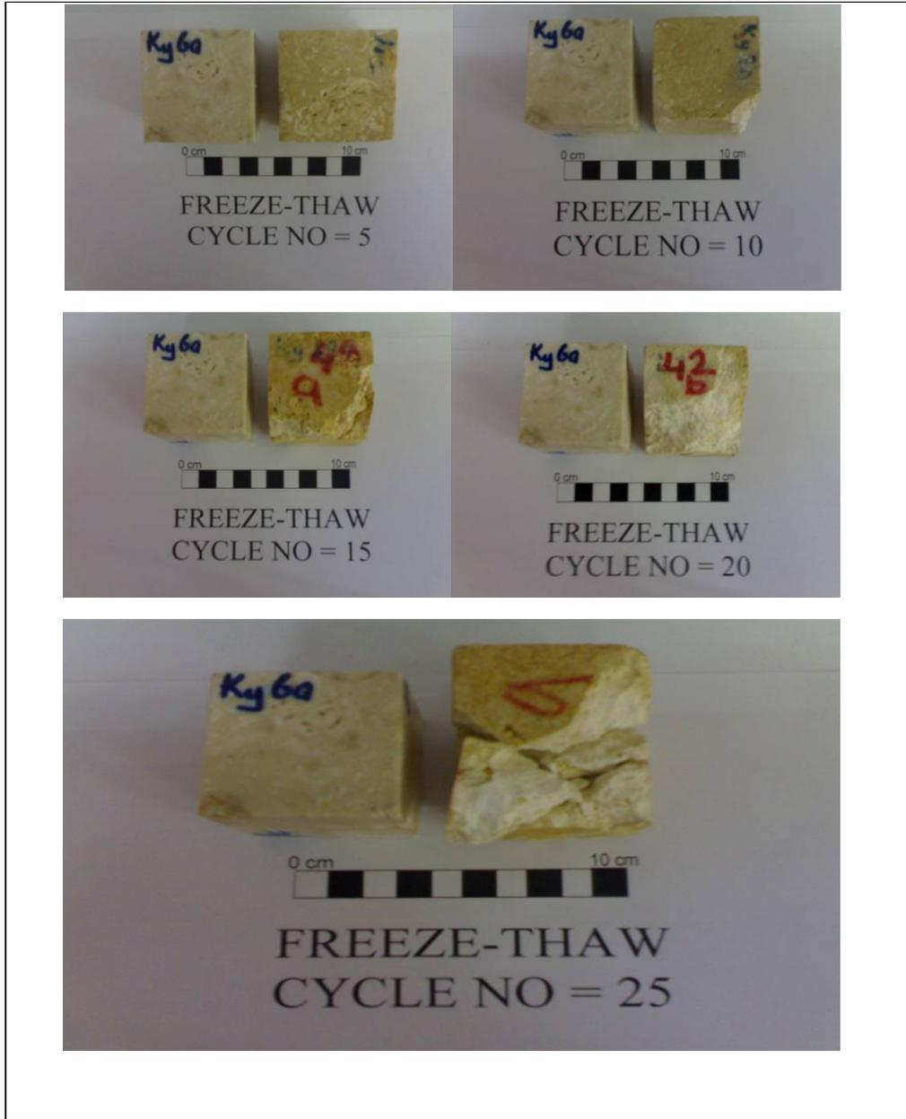
Figure 4.15 Physical appearance of the Tirtar lower level limestone subjected to 25 freezing-thawing test cycles. The sample at the left side of the photograph is a fresh reference sample.
