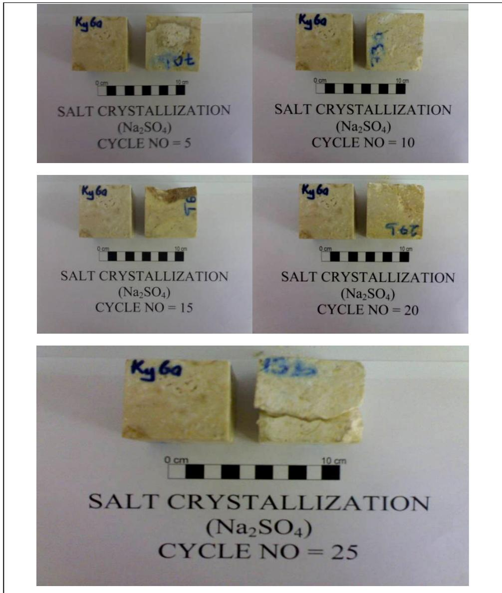
Figure 4.25 Physical appearance of the Tirtar lower level limestone subjected to 25 salt crystallization ( $\text{Na}_2\text{SO}_4$ ) test cycles. The sample at the left side of the photograph is a fresh reference sample.
