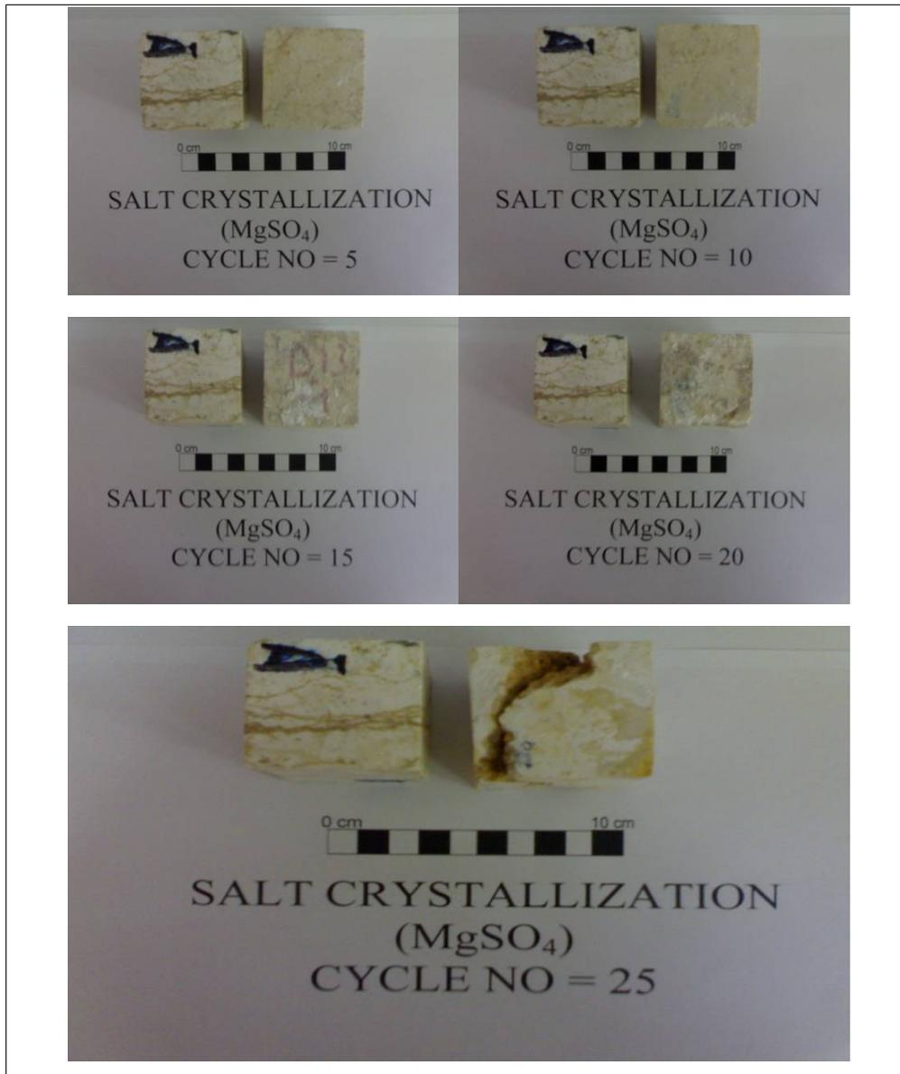
Figure 4.19 Physical appearance of the Tirtar middle level limestone subjected to 25 salt crystallization (MgSO<sub>4</sub>) test cycles. The sample at the left side of the photograph is a fresh reference sample.
