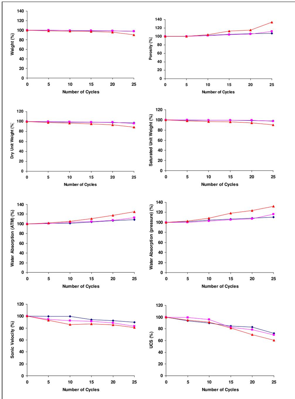
Figure 4.37 Effect of durability tests on the physical and mechanical properties of the Tirtar middle level limestone (blue line shows wet-dry; pink line shows freeze-thaw and the red line shows salt crystallization test).
