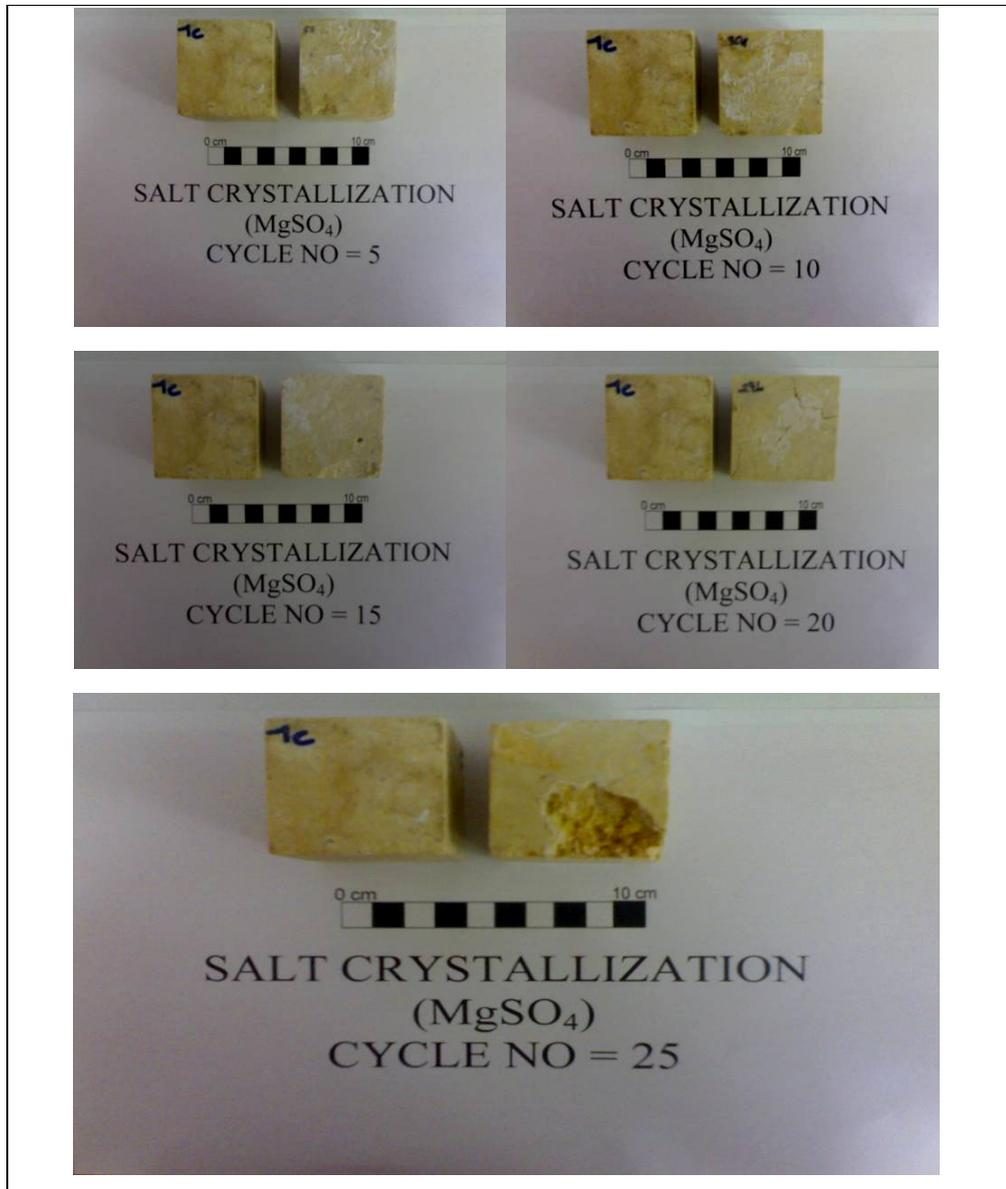
Figure 4.17 Physical appearance of the Değirmençayı limestone subjected to 25 salt crystallization (MgSO<sub>4</sub>) test cycles. The sample at the left side of the photograph is a fresh reference sample.
