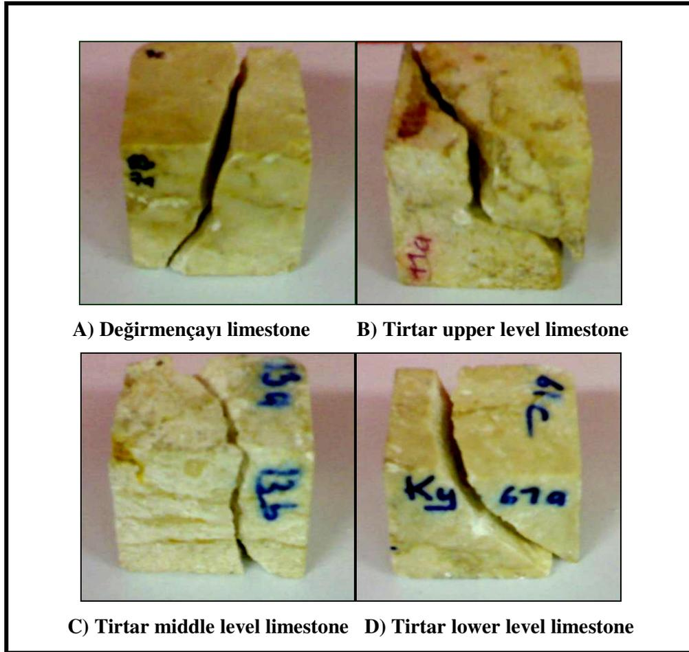
Figure 4.3 The limestones after the point load tests.
