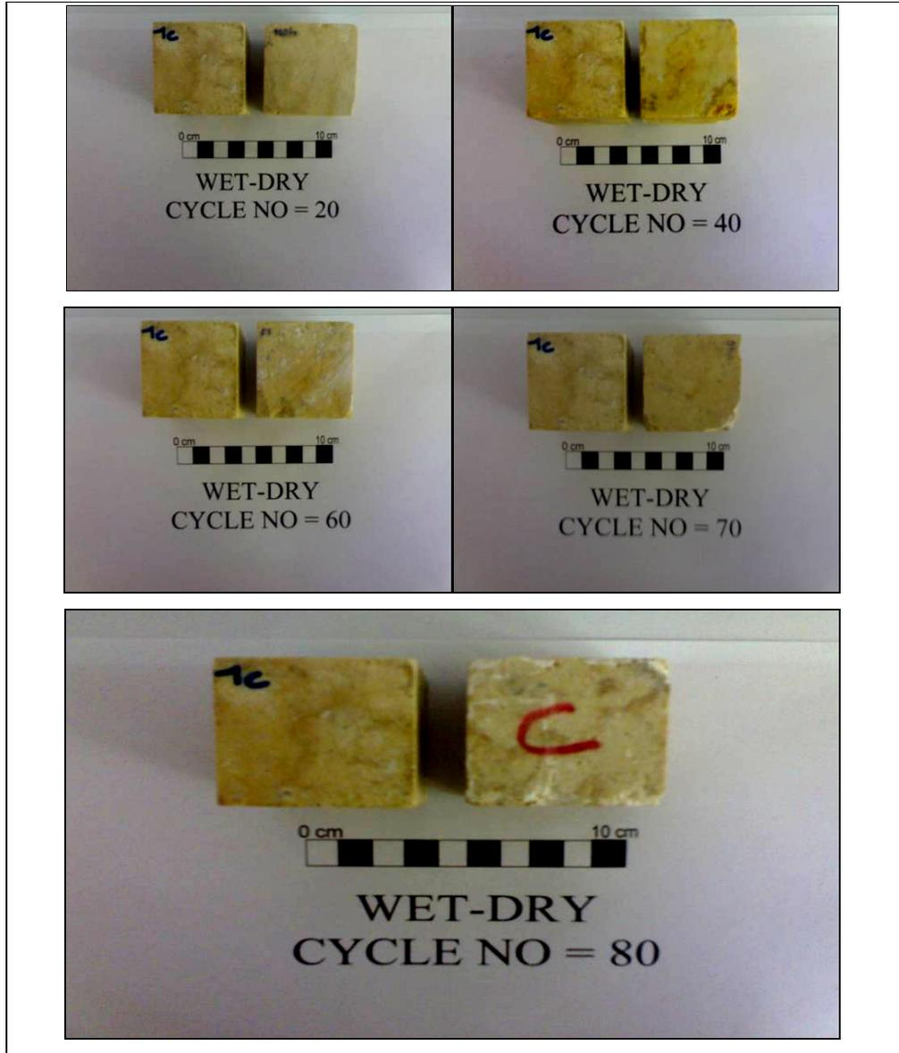
Figure 4.7 Physical appearance of the Değirmençayı limestone subjected to 80 wetting-drying test cycles. The sample at the left side of the photograph is a fresh reference sample.
