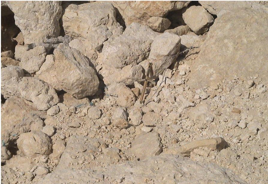
Figure 6.4 Limestone blocks used in Kumkuyu harbour with dissolution effects after 1 year.
