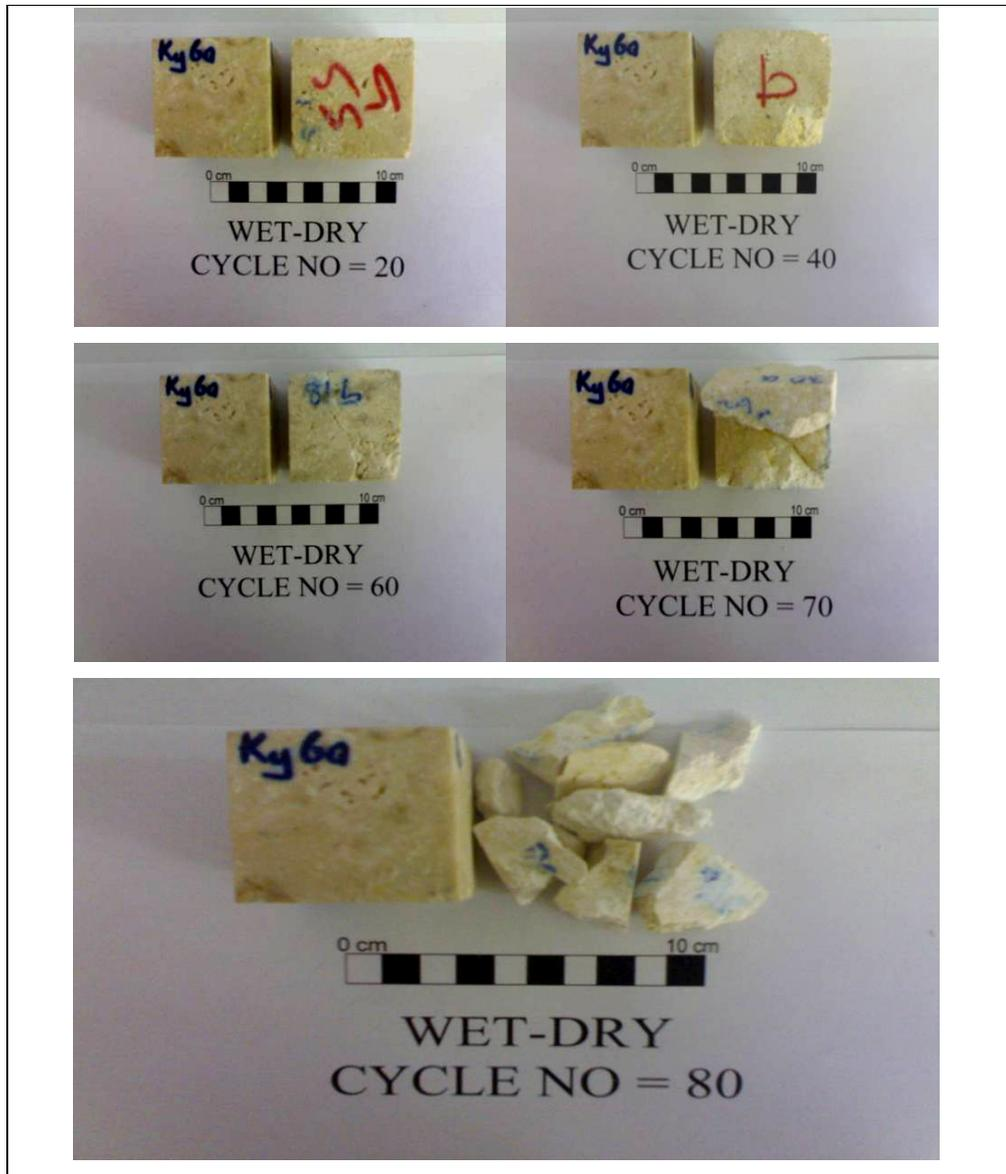
Figure 4.10 Physical appearance of the Tirtar lower level limestone subjected to 80 wetting-drying test cycles. The sample at the left side of the photograph is a fresh reference sample.
