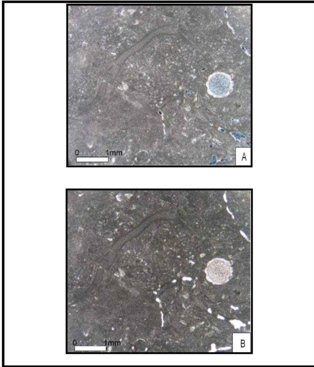
Figure 2.2 Photomicrographs of the Değirmençayı limestone (A) Plaine polarized light (PPL)x5, (B) Cross polarized light (CPL)x5
