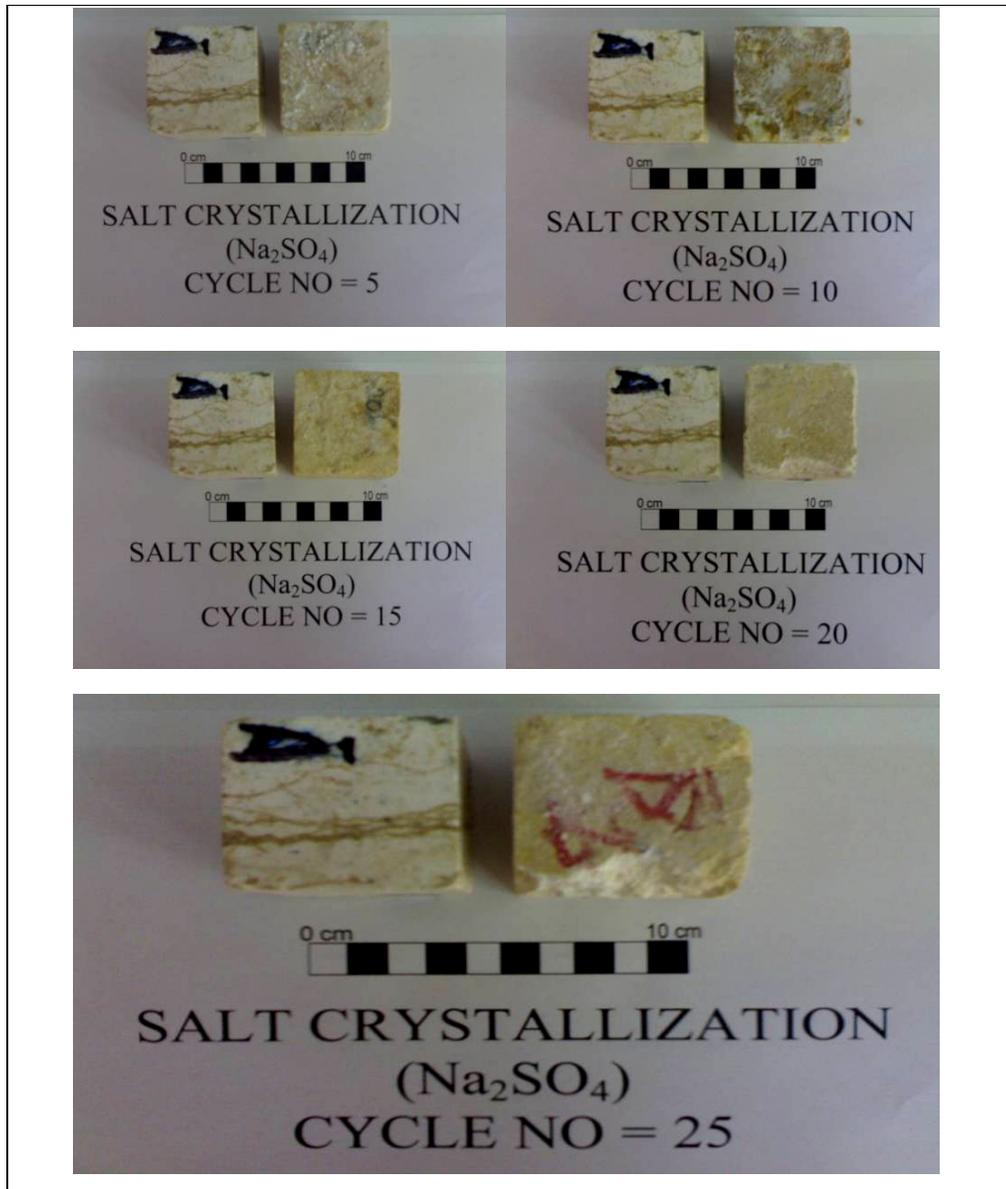
Figure 4.24 Physical appearance of the Tirtar middle level limestone subjected to 25 salt crystallization ( $\text{Na}_2\text{SO}_4$ ) test cycles. The sample at the left side of the photograph is a fresh reference sample.
