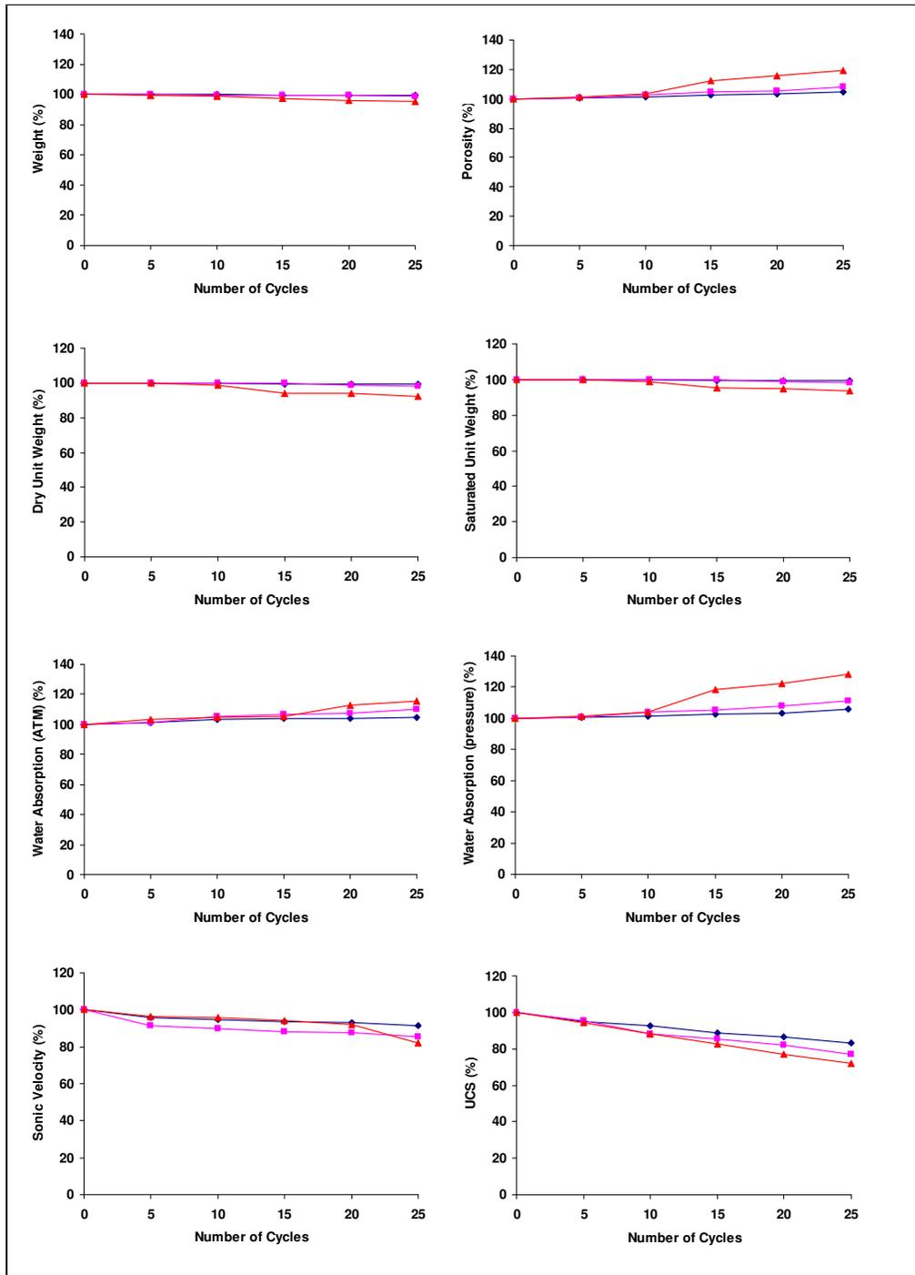
Figure 4.35 Effect of durability tests on the physical and mechanical properties of the Değirmançayı limestone (blue line shows wet-dry; pink line shows freeze-thaw and the red line shows salt crystallization test).
