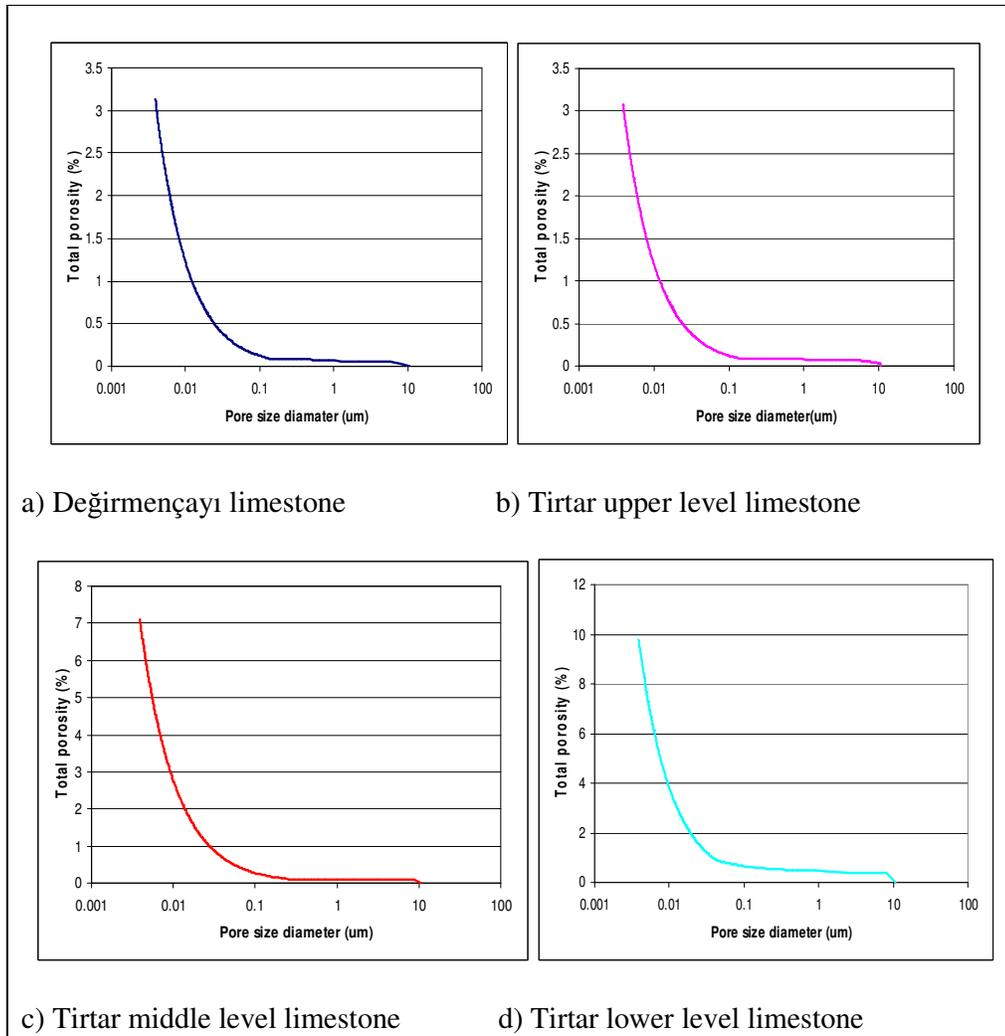
Figure 4.28 Cumulative intrusion curves of the four fresh limestone samples.
