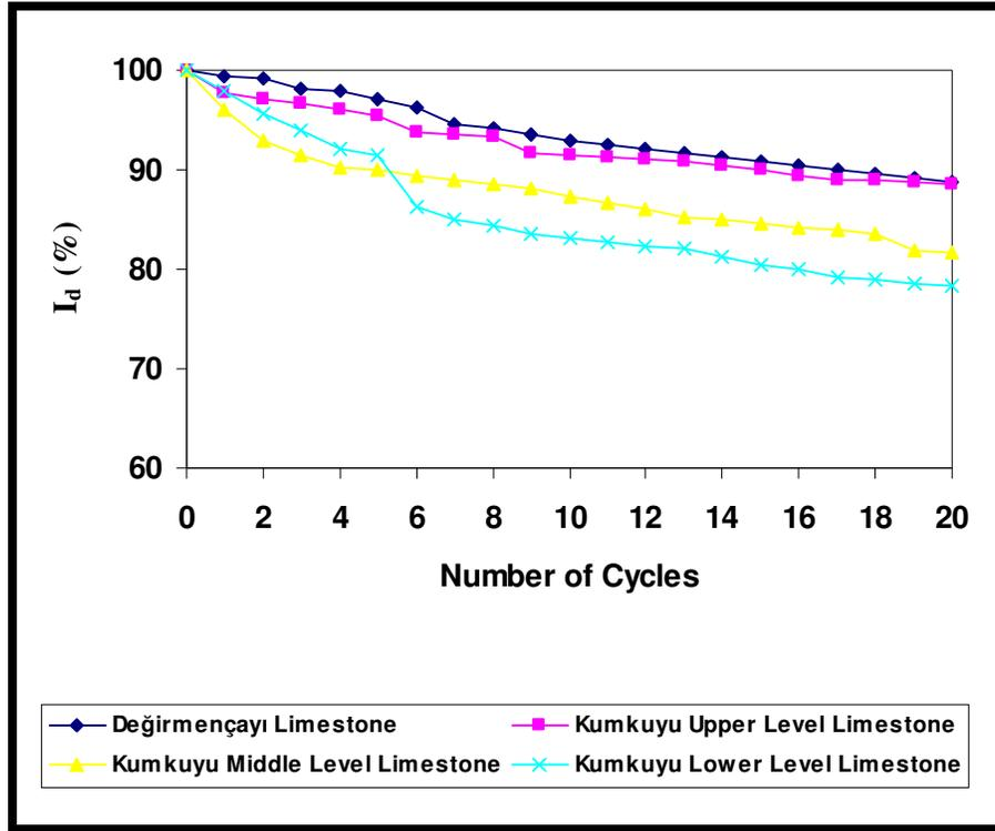
Figure 4.4 The variation of slake durability indexes of the limestones for various test cycles.
