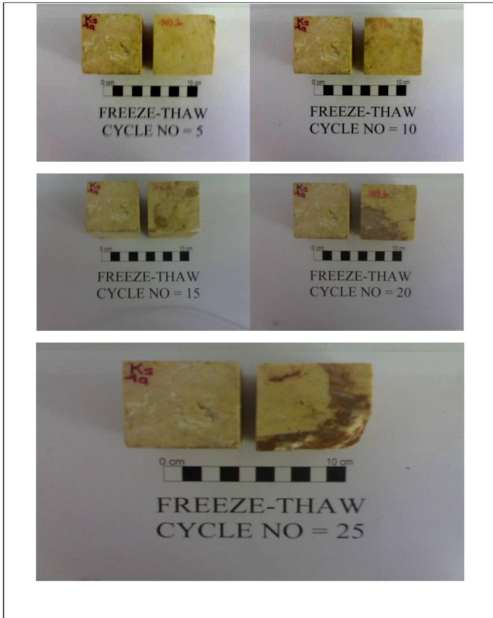
Figure 4.13 Physical appearance of the Tirtar upper level limestone subjected to 25 freezing-thawing test cycles. The sample at the left side of the photograph is a fresh reference sample.
