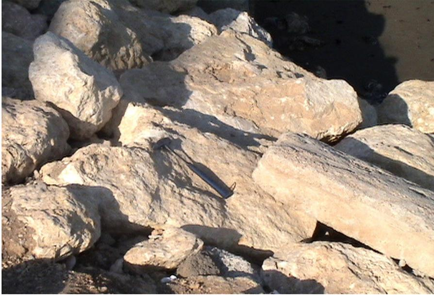
Figure 6.3 A close-up view of the Tirtar upper level limestone used in Kumkuyu harbour.
