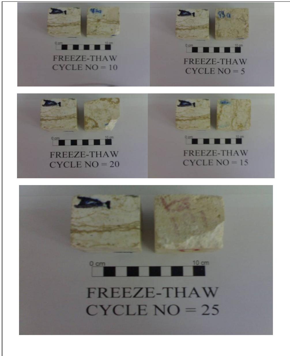
Figure 4.14 Physical appearance of the Tirtar middle level limestone subjected to 25 freezing-thawing test cycles. The sample at the left side of the photograph is a fresh reference sample.
