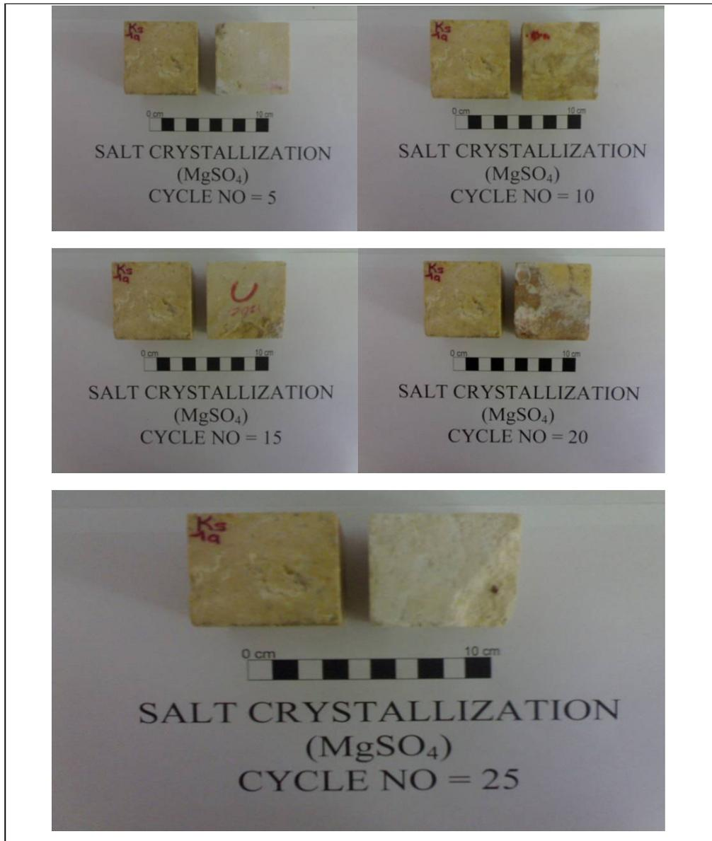
Figure 4.18 Physical appearance of the Tirtar upper level limestone subjected to 25 salt crystallization (MgSO<sub>4</sub>) test cycles. The sample at the left side of the photograph is a fresh reference sample.
