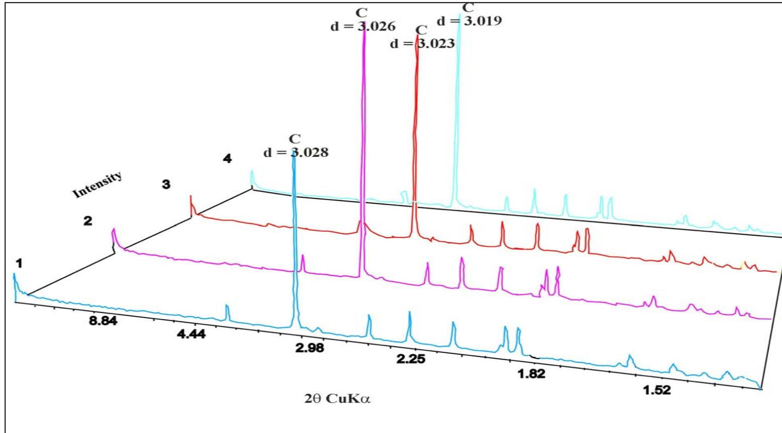
Figure 4.5 The XRD diffractograms of the unoriented samples (C=  $\text{CaCO}_3$  , blue line shows Değirmençayı limestone, pink line shows Tirtar upper level limestone, red line shows Tirtar middle level limestone, turquoise line shows Tirtar lower level limestone.
