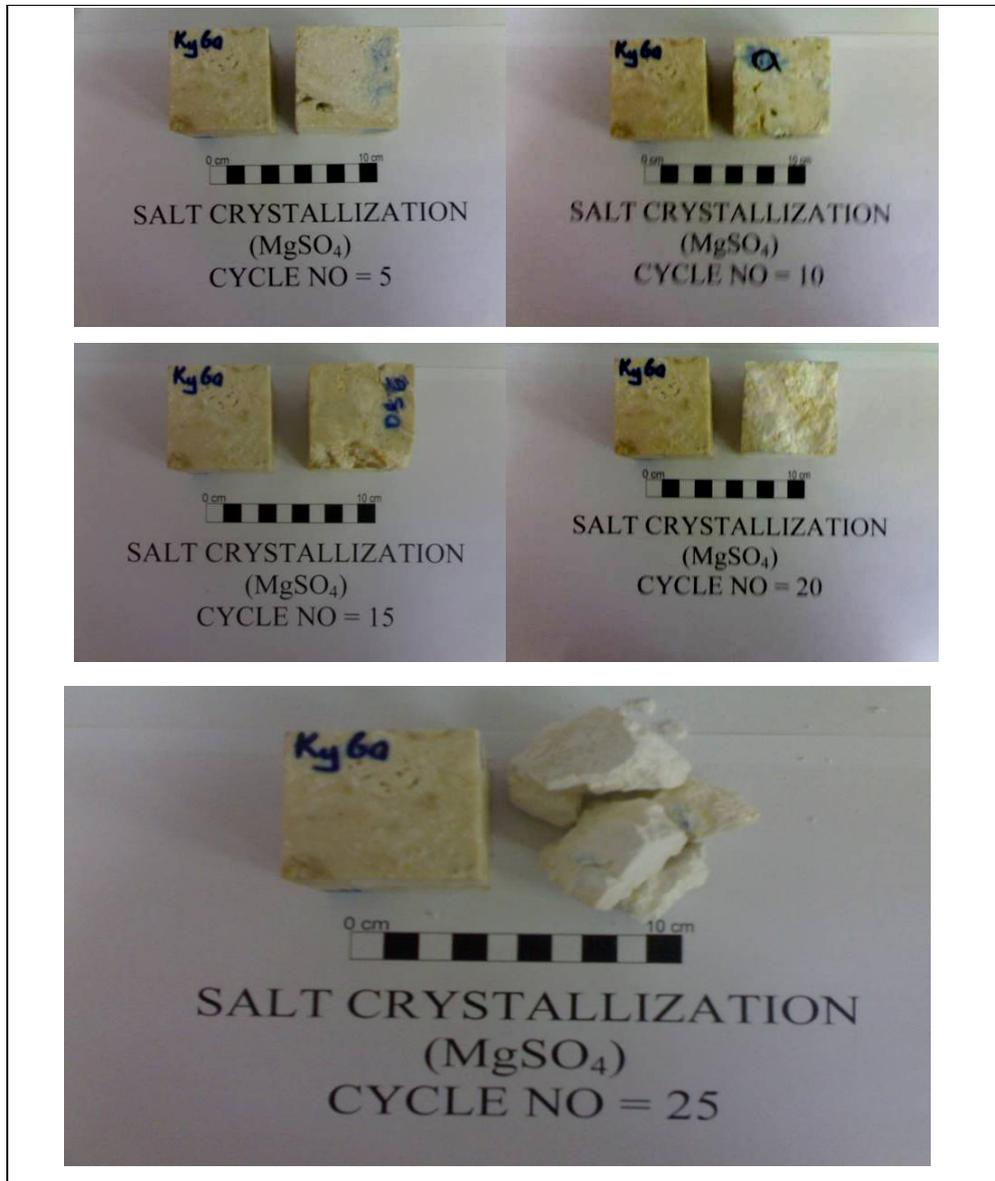
Figure 4.20 Physical appearance of the Tirtar lower level limestone subjected to 25 salt crystallization (MgSO<sub>4</sub>) test cycles. The sample at the left side of the photograph is a fresh reference sample.
