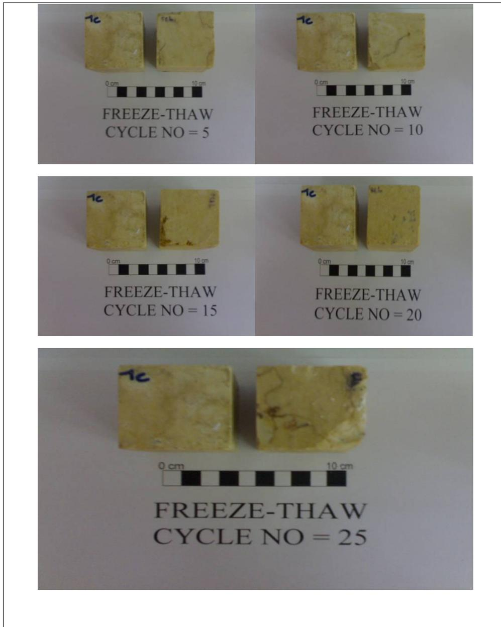
Figure 4.12 Physical appearance of the Değirmençayı limestone subjected to 25 freezing-thawing test cycles. The sample at the left side of the photograph is a fresh reference sample
