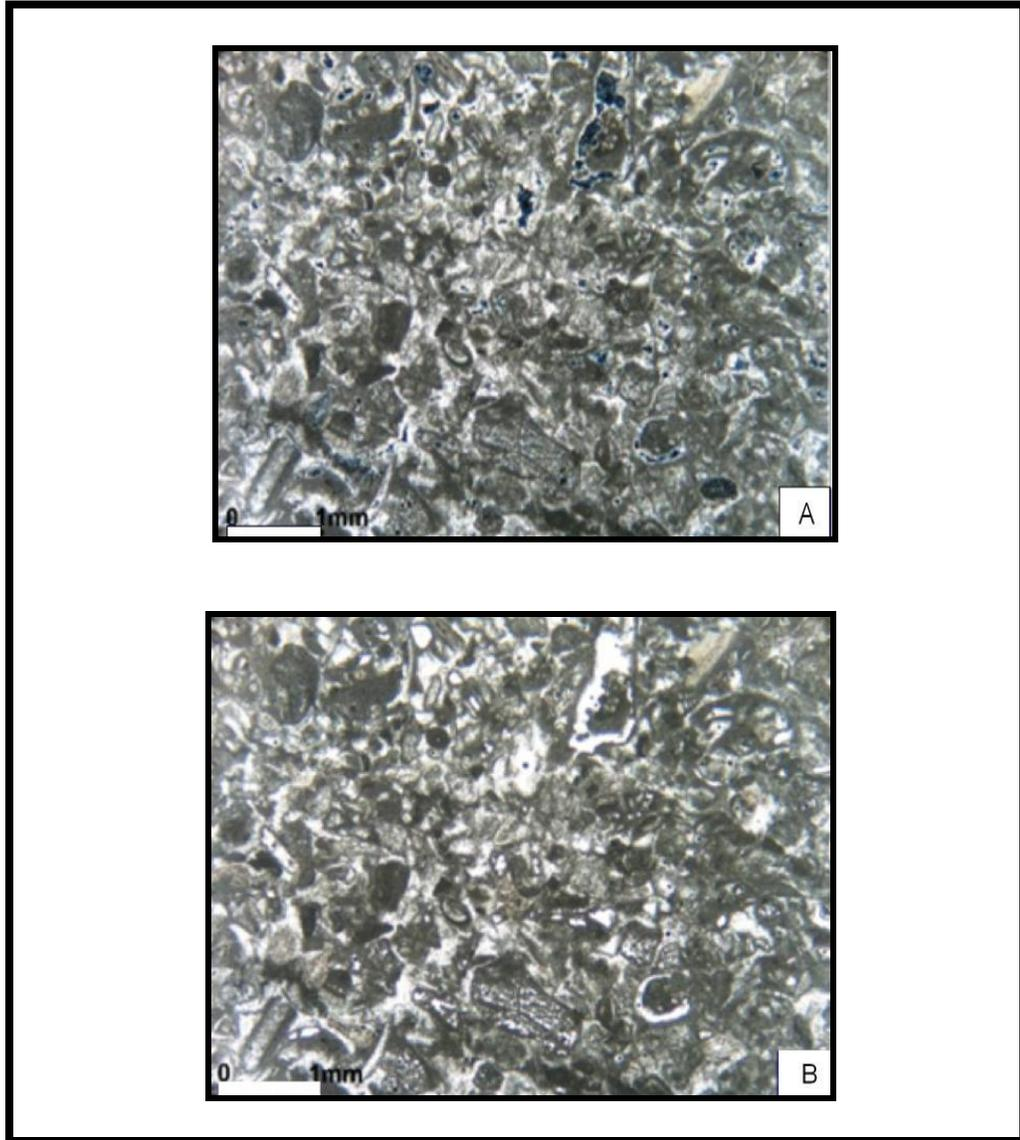
Figure 2.6 Photomicrographs of the Tirtar lower level limestone (A) Plain polarized light (PPL)x5, (B) Cross polarized light (CPL)x5
