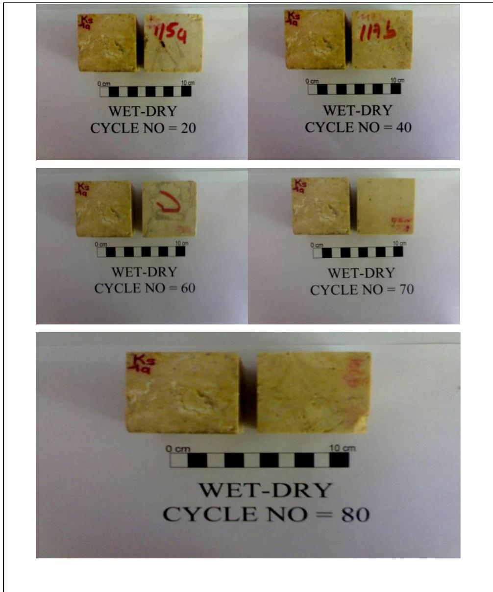
Figure 4.8 Physical appearance of the Tirtar upper level limestone subjected to 80 wetting-drying test cycles. The sample at the left side of the photograph is a fresh reference sample.
