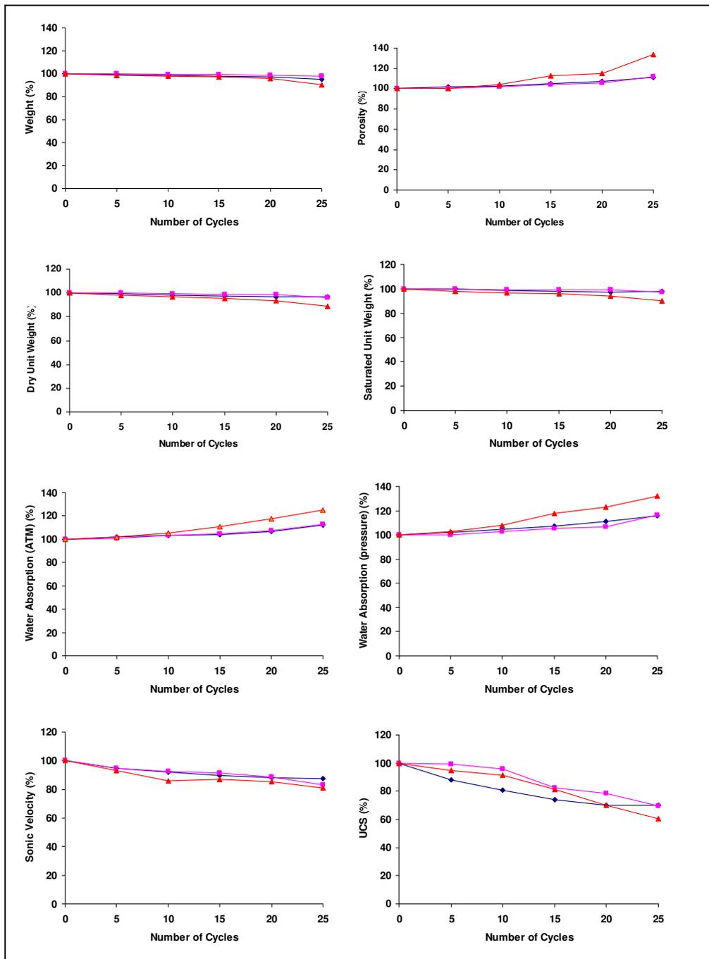
Figure 4.38 Effect of durability tests on the physical and mechanical properties of the Tirtar lower level limestone (blue line shows wet-dry; pink line shows freeze-thaw and the red line shows salt crystallization test).
