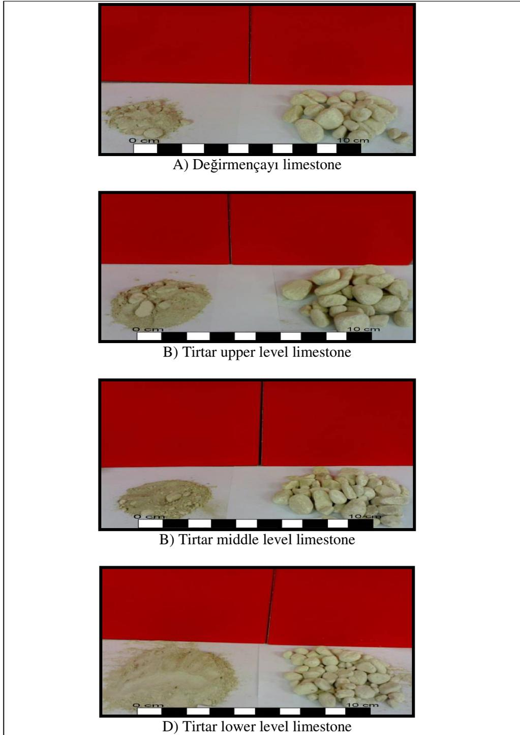
Figure 4.26 The physical changes of limestones after 1000 revolutions Los Angeles test cycles. Figures show materials passing 1.7 mm sieve (left side ) and retained (right side).
