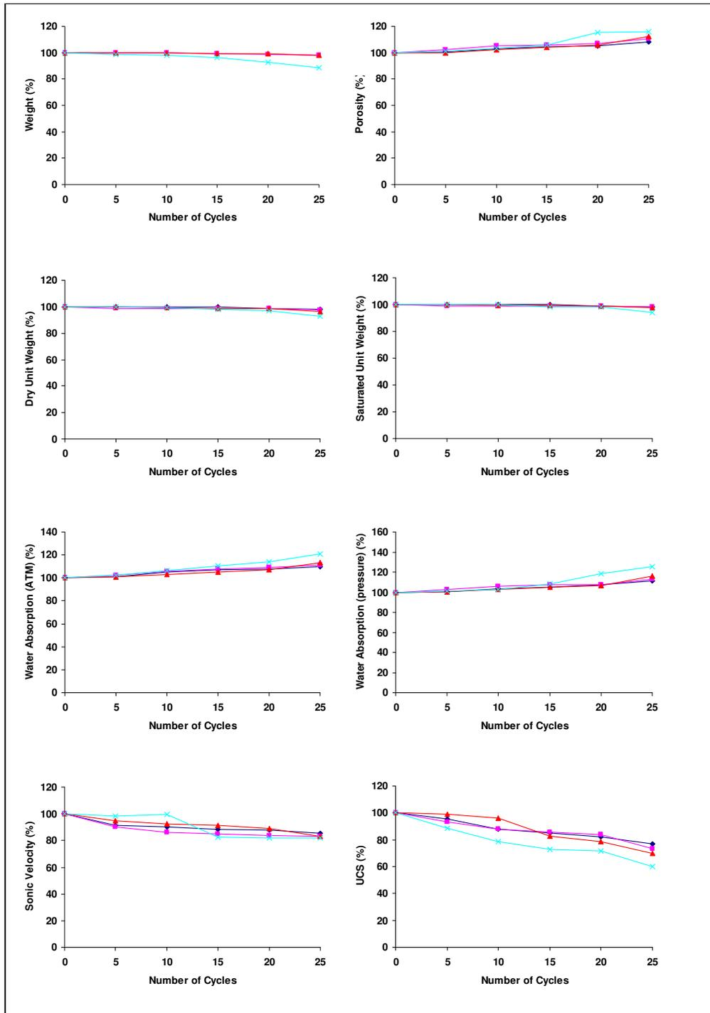
Figure 4.11 Variation of physico-mechanical properties of the limestones after the freezing-thawing tests blue line shows (blue line shows Değirmençayı limestone, pink line shows Tirtar upper level limestone, red line shows Tirtar middle level limestone, turquoise line shows Tirtar lower level limestone).
