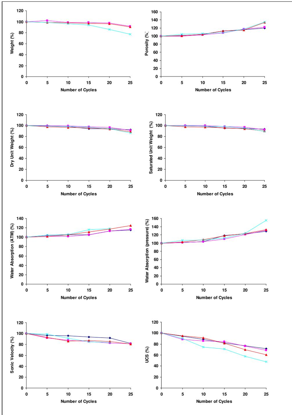
Figure 4.16 Variation of physico-mechanical properties of the limestones after  $MgSO_4$  salt crystallization tests (blue line shows Değirmençayı limestone, pink line shows Tirtar upper level limestone, red line shows Tirtar middle level limestone, turquoise line shows Tirtar lower level limestone).
