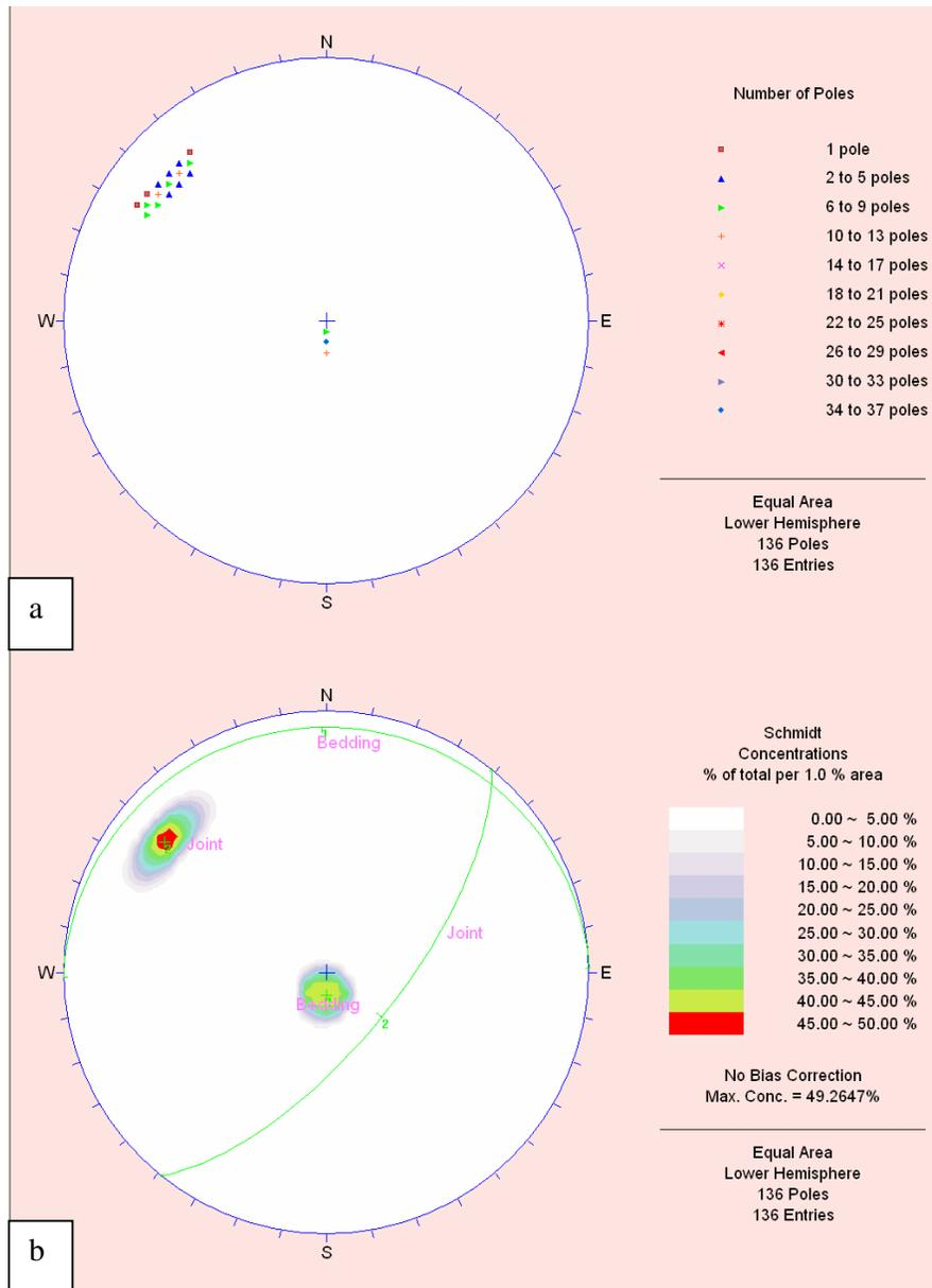
Figure 4.32 Pole plot (a) and contour plot (b) of the discontinuities in the Değirmençayı quarry.
