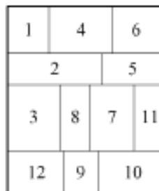
Figure 3.2 – Example of a layout constructed by using flexible bay representation (Chen et al., 2002)
