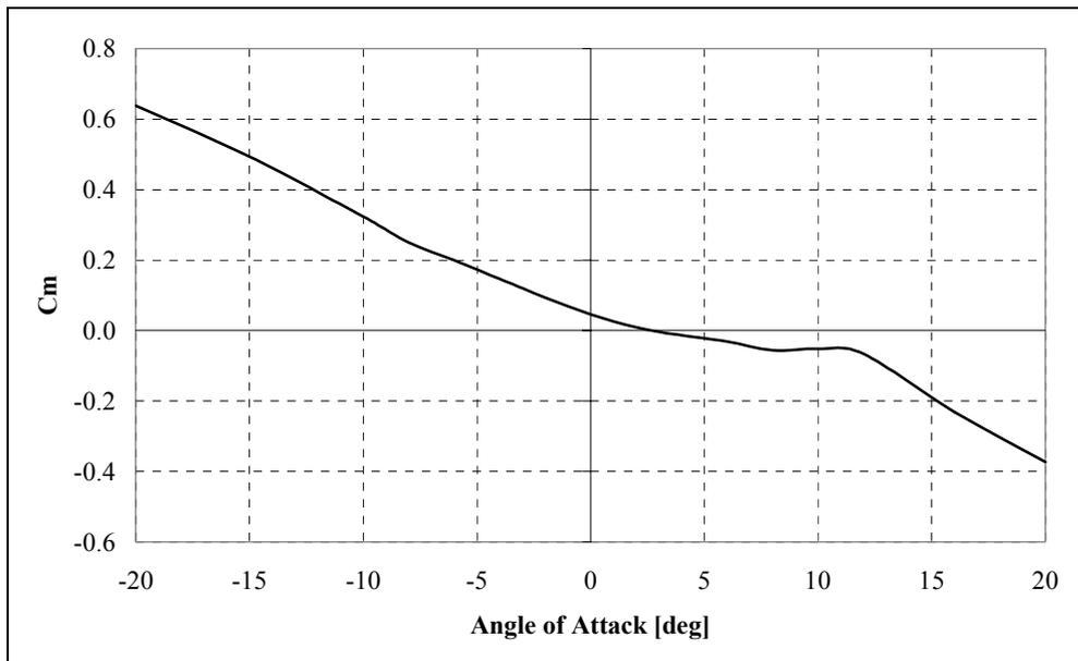
**Figure 15. Variation of  $C_m$  with angle of attack [deg]**
