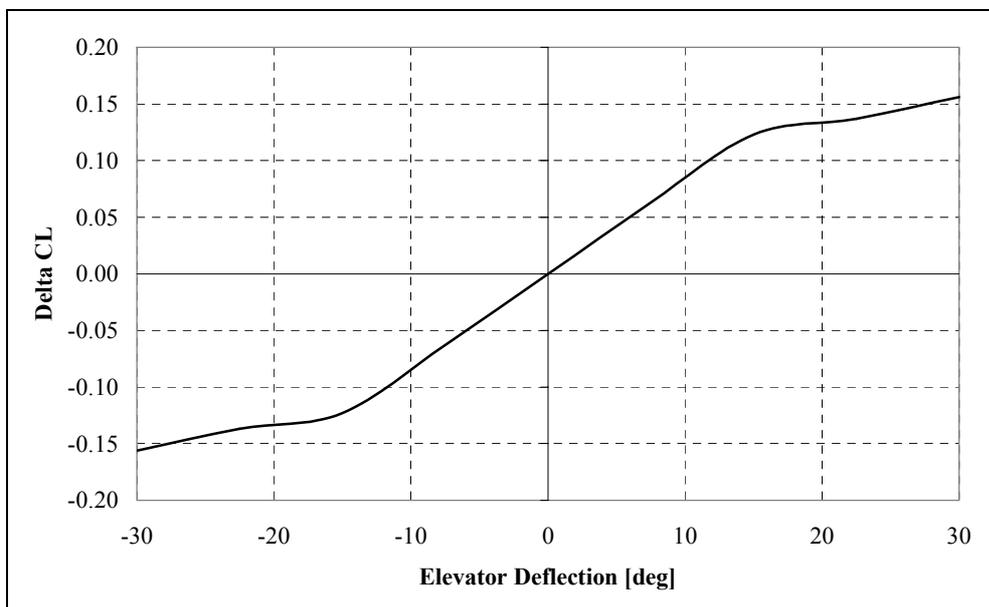
**Figure 16. Increment in  $C_L$  due to elevator deflection [deg]**
