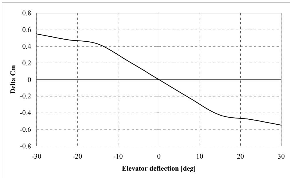
**Figure 17. Increment in  $C_m$  due to elevator deflection [deg]**
