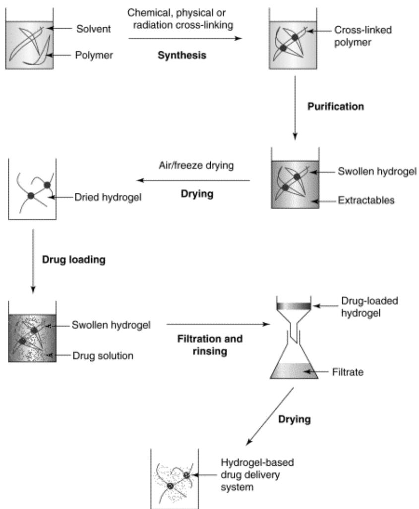
Figure 1.3 Preparation of hydrogel-based drug delivery systems [21]
