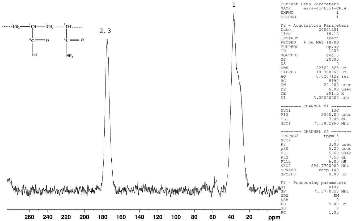
Figure 3.13 Solid state  $^{13}\text{C}$ -NMR of the hydrogel
