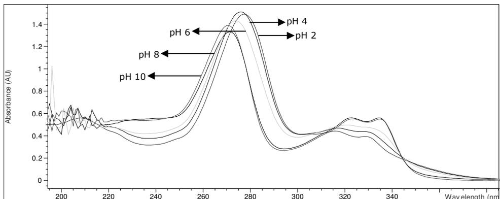
Figure 2.3 UV-Vis spectra of CPFV solution at varying pH values
