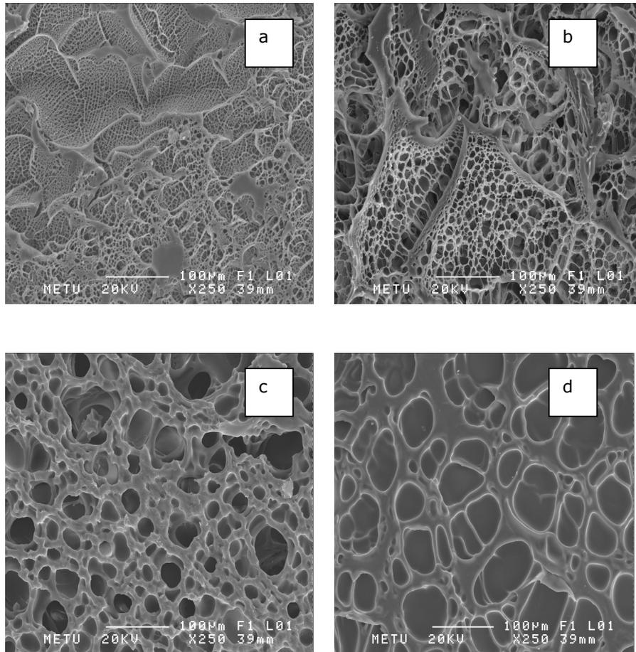
Figure 3.24 SEM images of a) cont; b) pls 20; c) pls 100; d) prs samples swelled in pH 2 buffer
