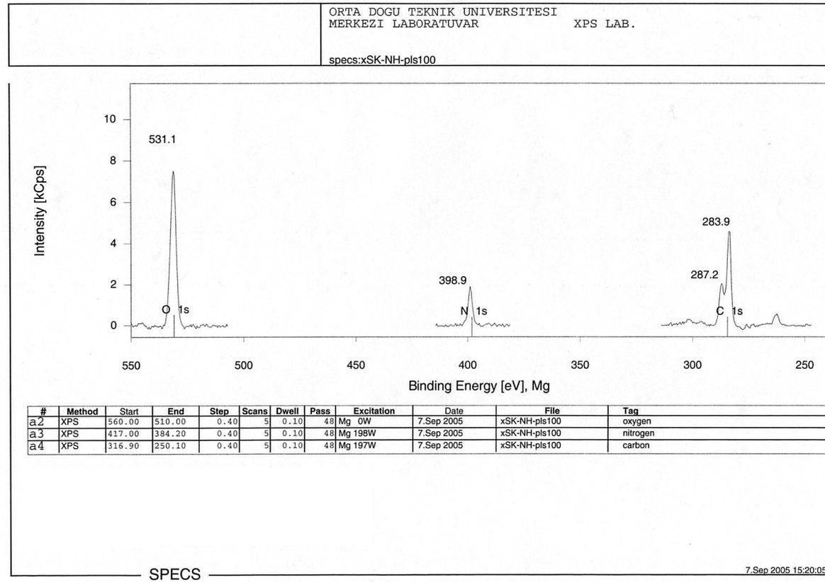
Figure 3.21 XPS survey scan spectrum for pls 100 sample
