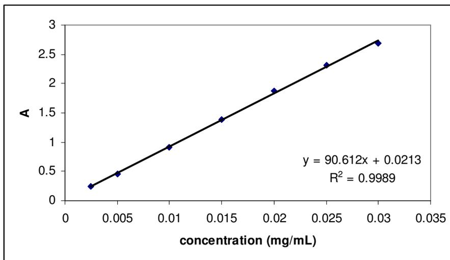
Figure B.4 Calibration curve for CPFY dissolved in pH 8 buffer solution
