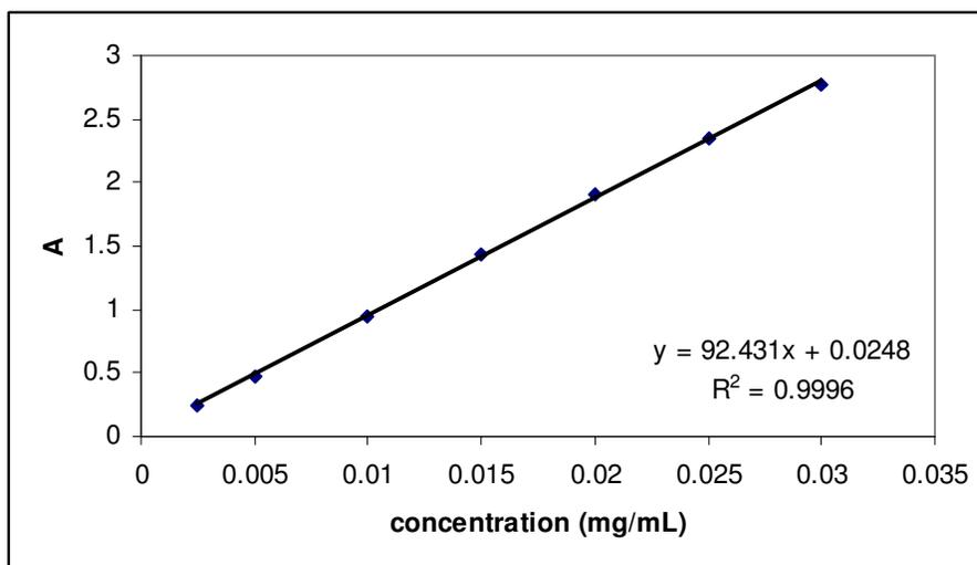
Figure B.3 Calibration curve for CPFY dissolved in pH 6 buffer solution
