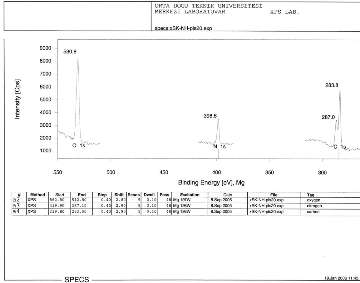
Figure 3.20 XPS survey scan spectrum for pls 20 sample
