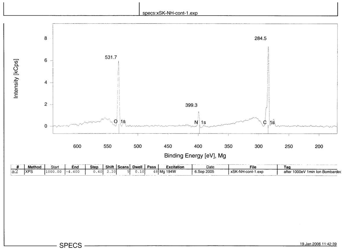
Figure 3.19 XPS survey scan spectrum for control sample
