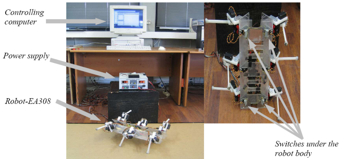
Figure 3.5: Experimental setup for the Robot-EA308 for learning of five-legged walking.
