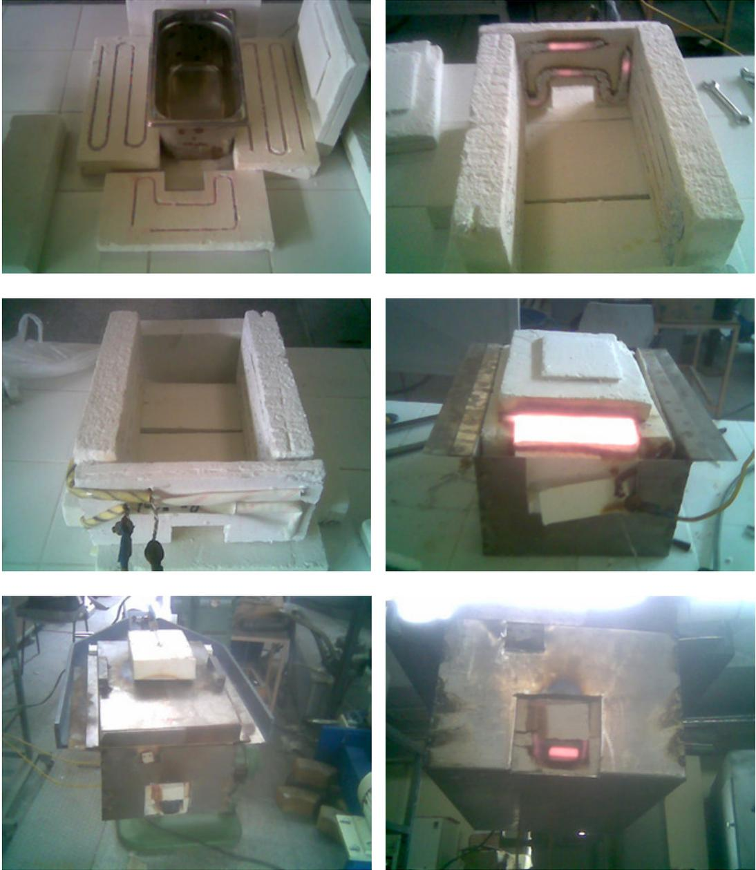
Figure 3.6 Photographs of electrical resistance furnace production.
