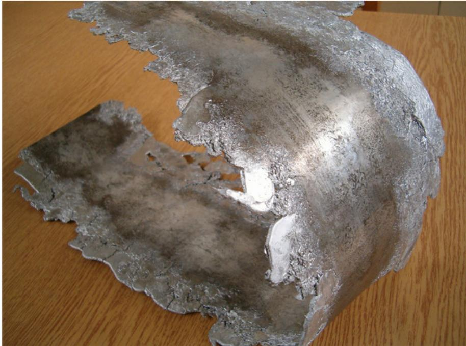
Figure 3. 9 The continuous flat Al-Fe-V-Si alloy product
