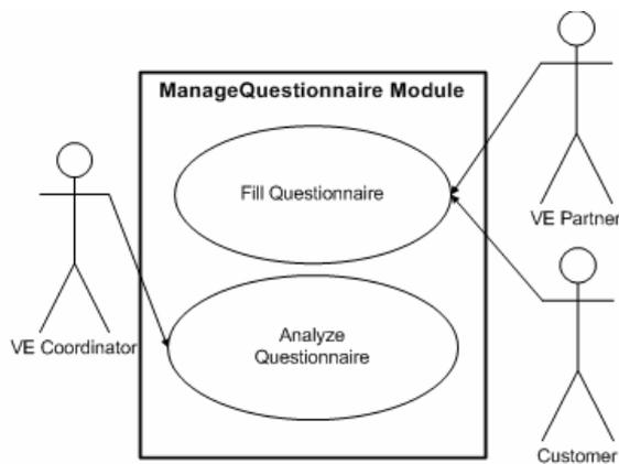
**Figure A35** Use case diagram of “Manage Questionnaire” module
