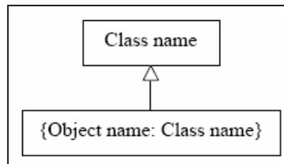
**Figure 2.14** Object instantiated from class (Rational, 1997)
