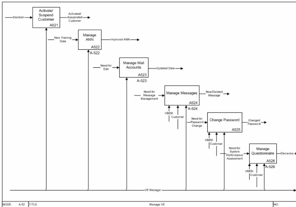
Figure A12 Decomposition of node A52
