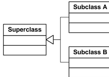
**Figure 5.17** Notation for generalization
