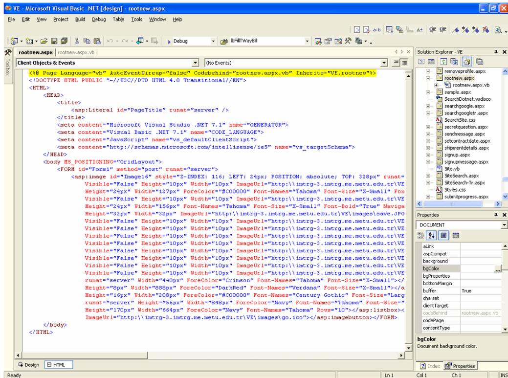
**Figure 5.24** Typical contents of a web form
