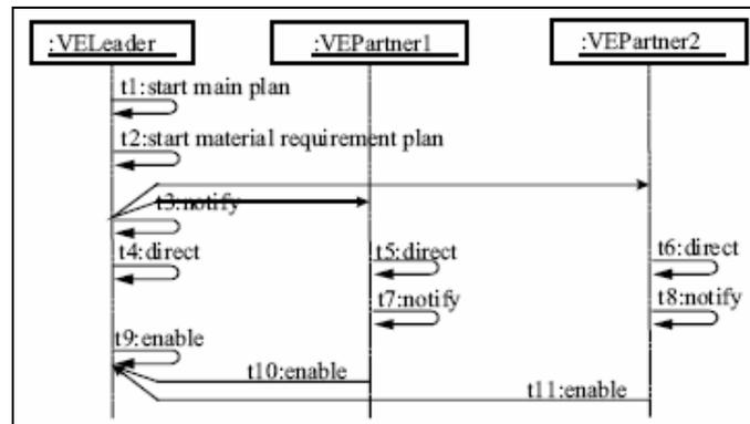
**Figure 2.24** UML sequence diagram for message transfers (Hongmei et al, 2000)
