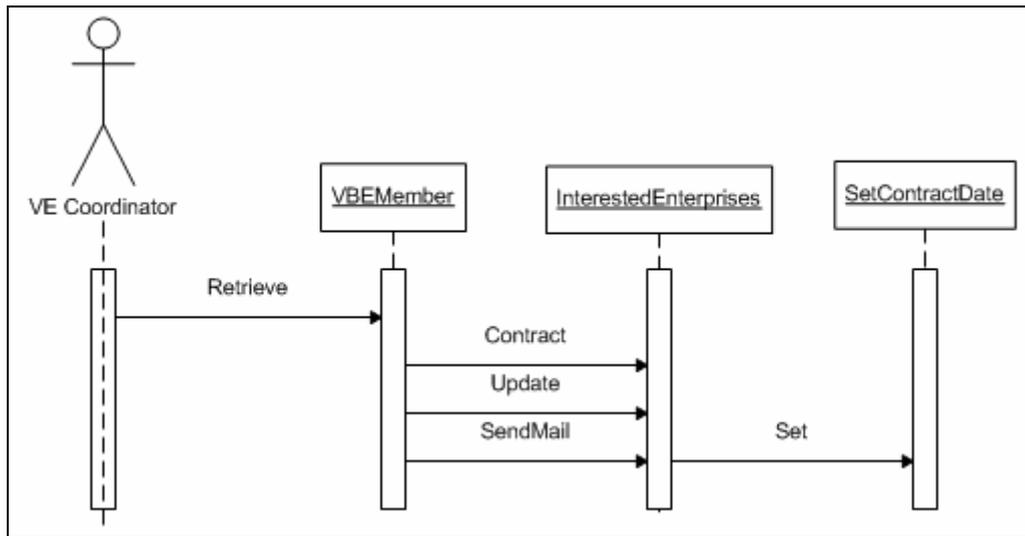
**Figure A44** Sequence diagram for “VBEM Selection”
