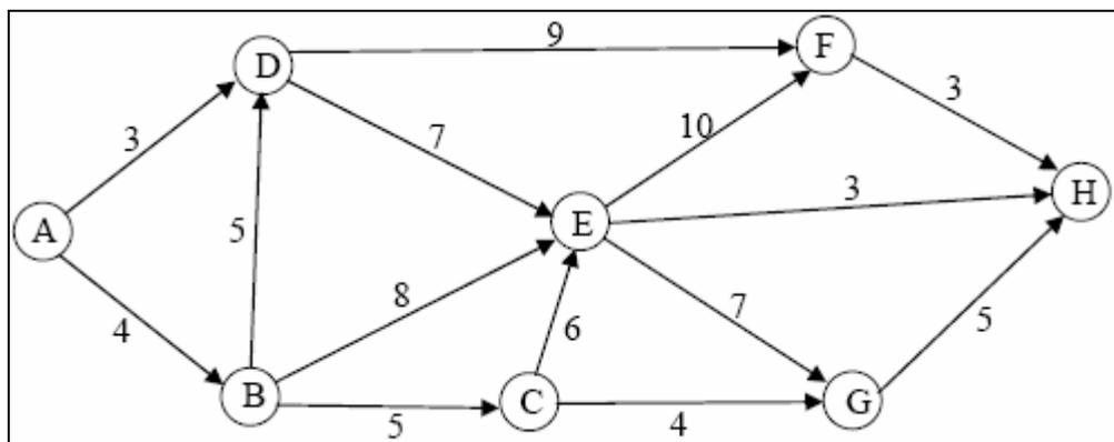
**Figure 3.4** An example of a PERT diagram
