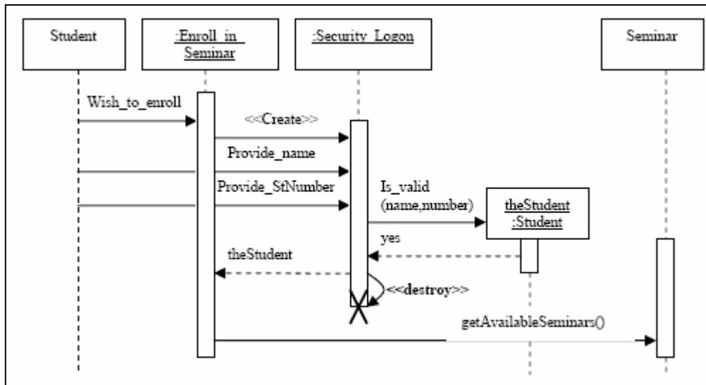
**Figure 2.15** Sequence diagram for enrolling a student (Rational, 1997)
