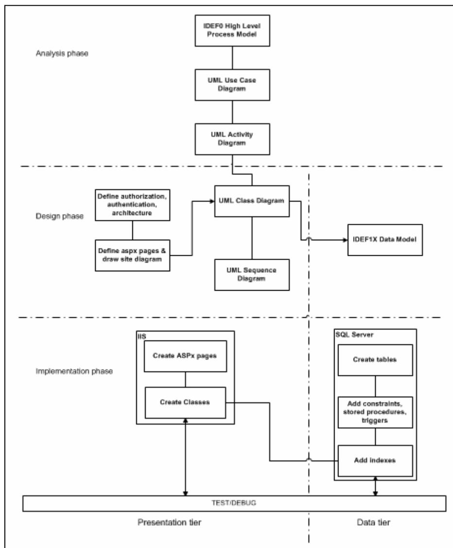
**Figure 5.2** Structured methodology for virtual enterprise systems
