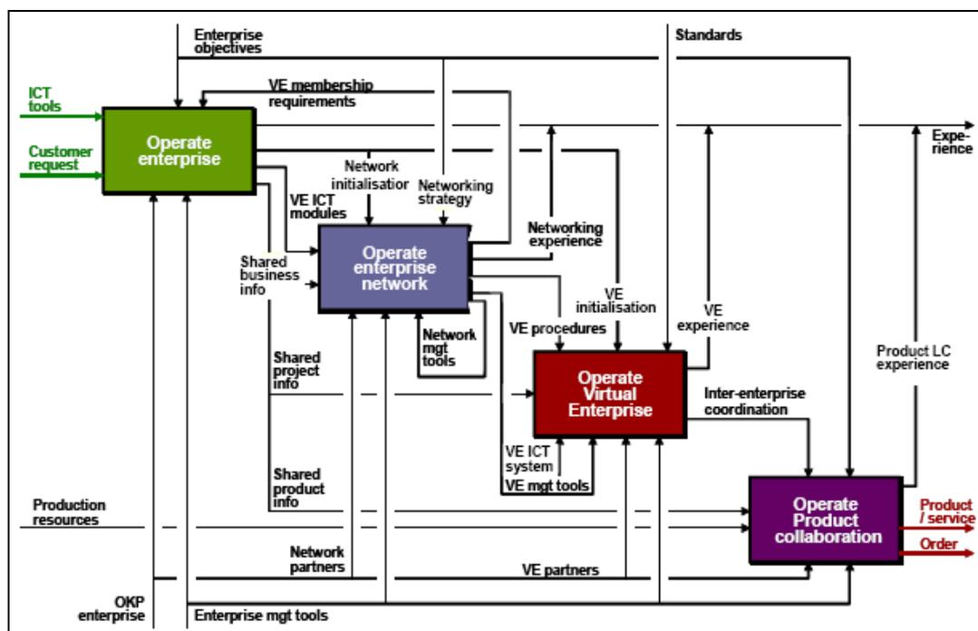
**Figure 2.7** Core functions in IDEF0 format (Globemen, 2002)
