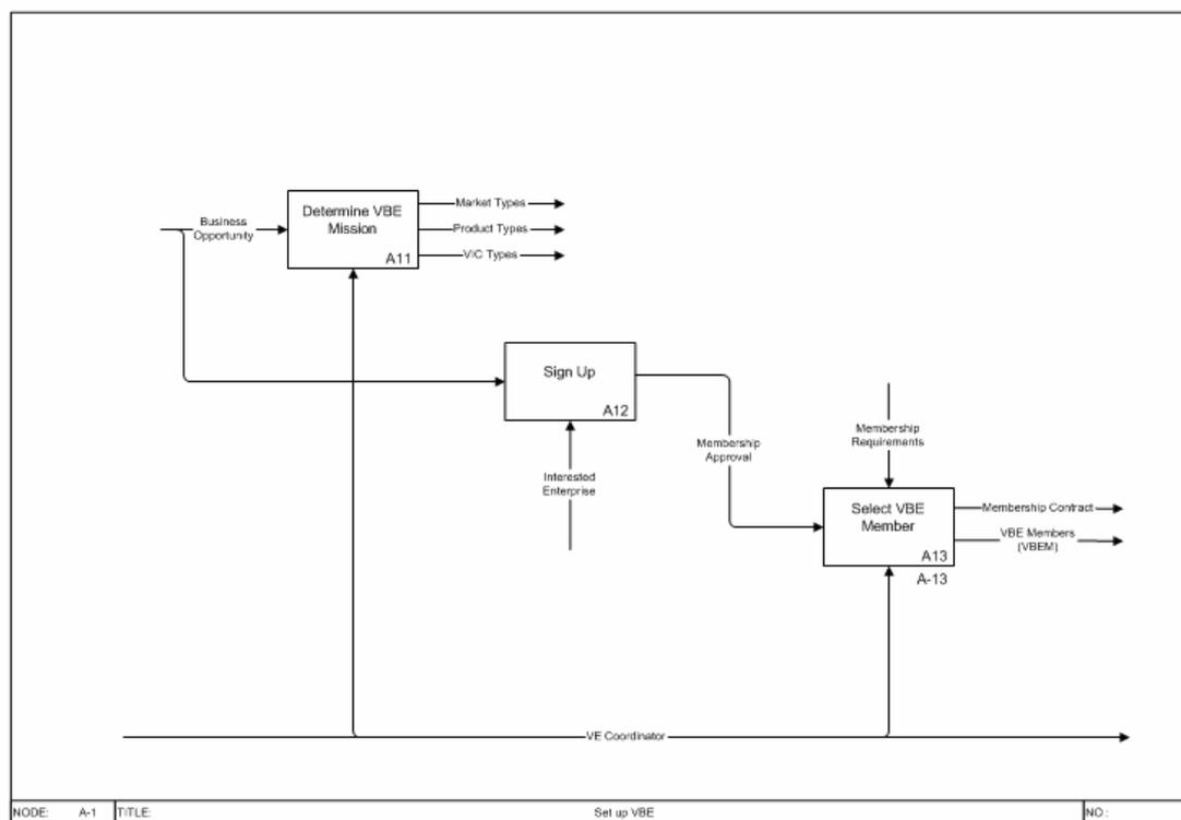
**Figure 6.5** Decomposition of node A1
