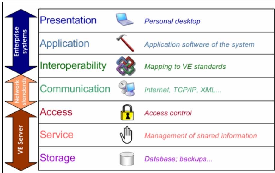
**Figure 5.1** Layered ICT reference architecture
