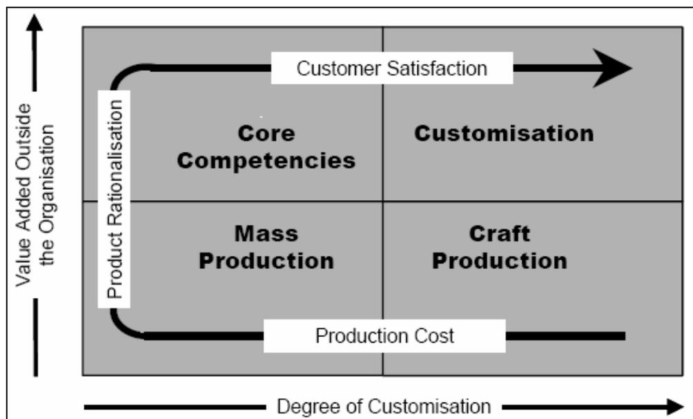
**Figure 3.1** Craft production through mass production to customization
