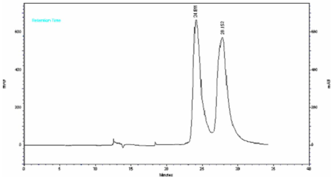
**Figure 15:** Chiral HPLC chromatogram of racemic  $\alpha'$ -acetoxy enone ( $\pm$ )-16
