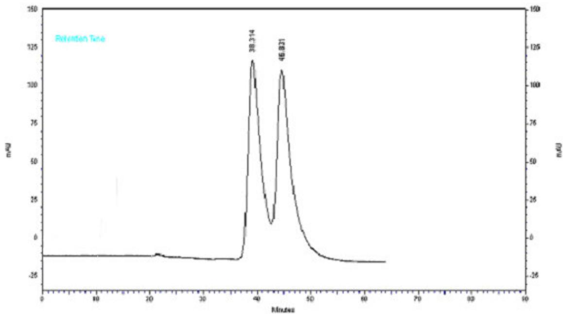
**Figure 14:** Chiral HPLC chromatogram of racemic  $\alpha'$ -acetoxy enone ( $\pm$ )-14
