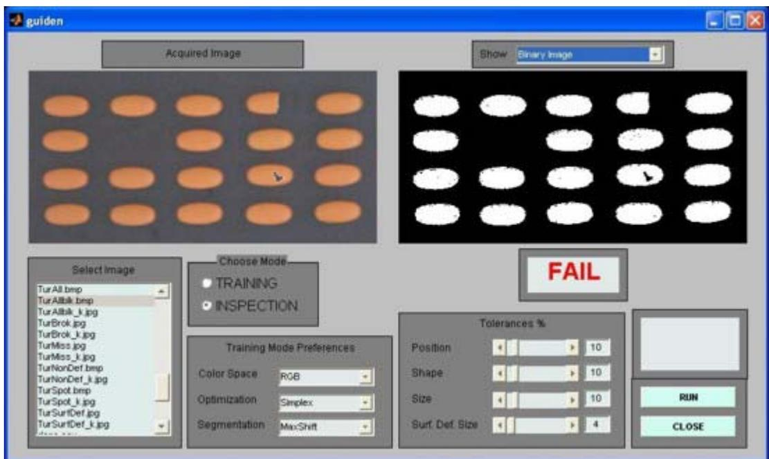
Figure 5.10. Inspection mode result of a blister of defected tablets using MaxShift algorithm in RGB color space
