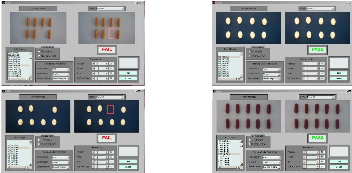
Figure 5.15. Inspection mode results for tablet images
