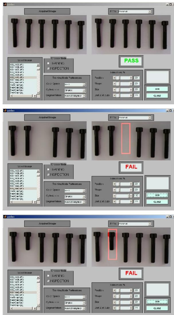
Figure 5.16. Inspection mode results for screw image
