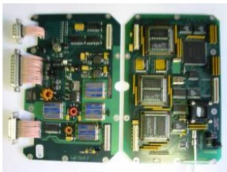
Figure-2.2: Processing unit of star camera
