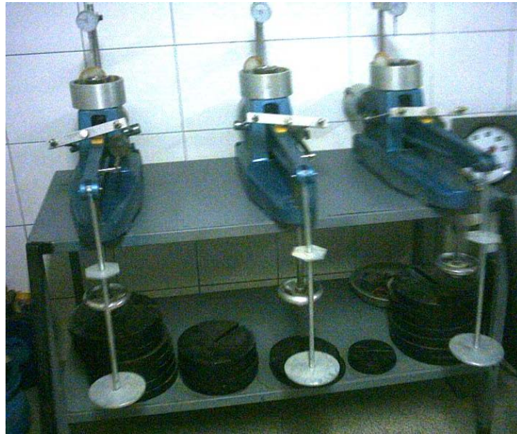
Figure 3.2 Photo image of oedometer device in soil mechanics laboratory of Yüksel Proje
