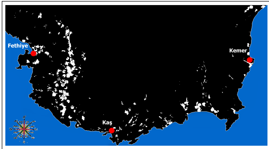
Figure 5.21 Final prediction map generated by adding layers of seven parameters. White pixels show suitable areas other unsuitable.
