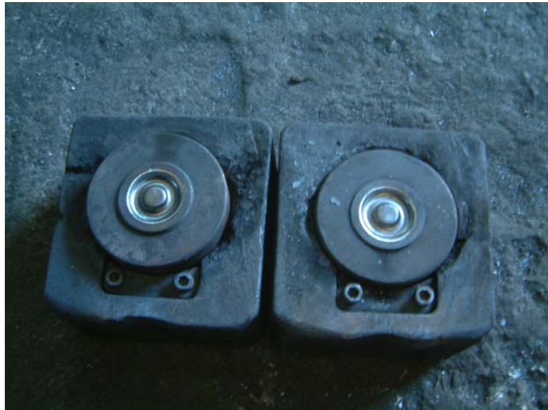
Figure 3.25 Lower and Upper Finish Dies Used in Experiment
