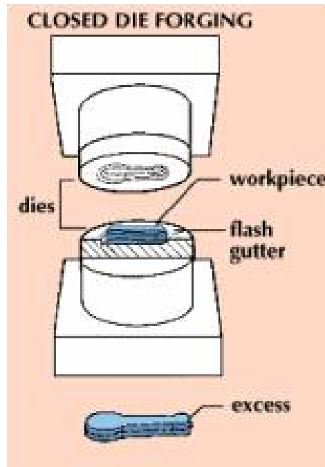
Figure 1.3 Schematic Drawing of Closed Die Forging
