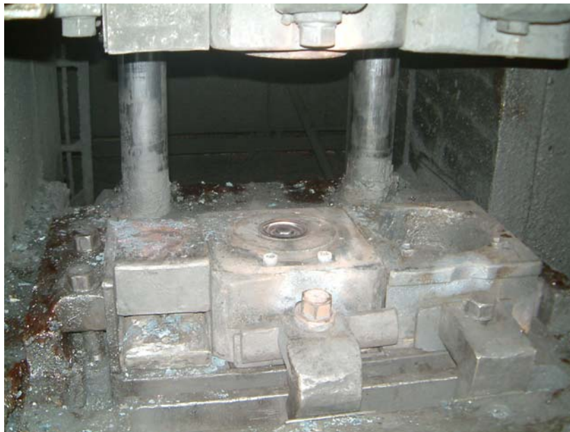
Figure 3.24 Preform and Finish Dies Fastened to the Press
