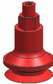
Figure 6.6 3-D cad view of the selected suction cup
