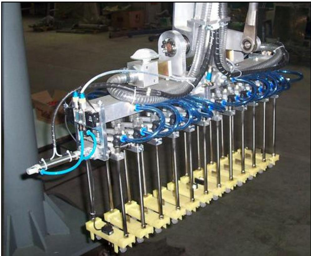
Figure 6.4 Actual gripper integrated with the robotic arm
