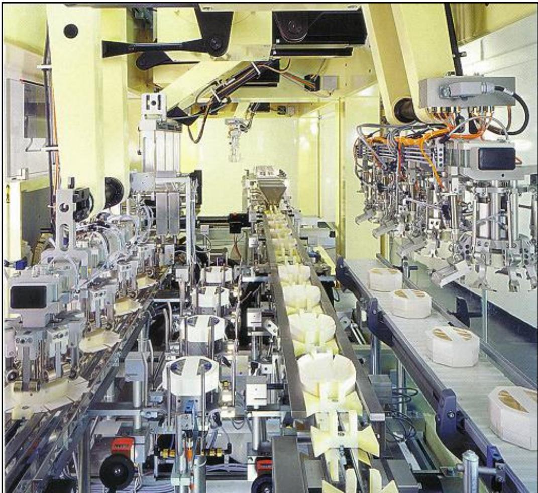
Figure 2.4 Schubert's secondary packaging automation solution
