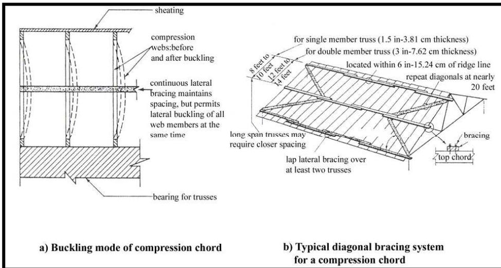
**Figure III. 14** a) Buckling mode of a compression chord when lateral bracing is not tied to a braced system. b) Typical diagonal bracing for a compression chord (Faherty, 1989: 6.93, 6.94).
