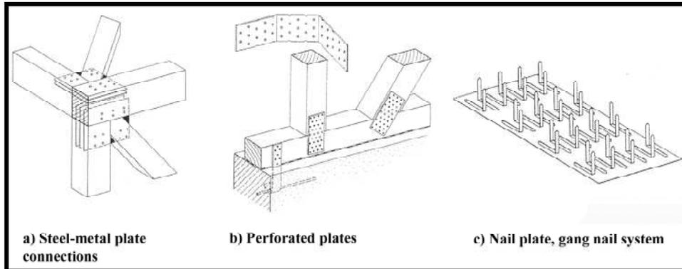
**Figure III. 17** Various connections are used for jointing timber members (Götz *et al.*, 1989:52).
