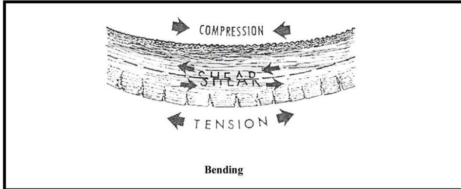
**Figure III. 9** Bending a length of wood sets up multi-stresses: compression, shear and tension (Oberg, 1963:83).
