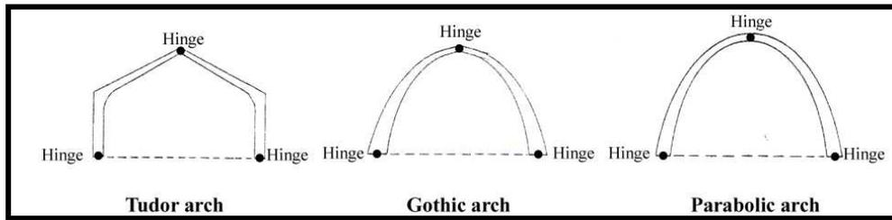
**Figure II. 34** Three hinged arches have three general forms (Hornbostel and Hornung, 1982:183).
