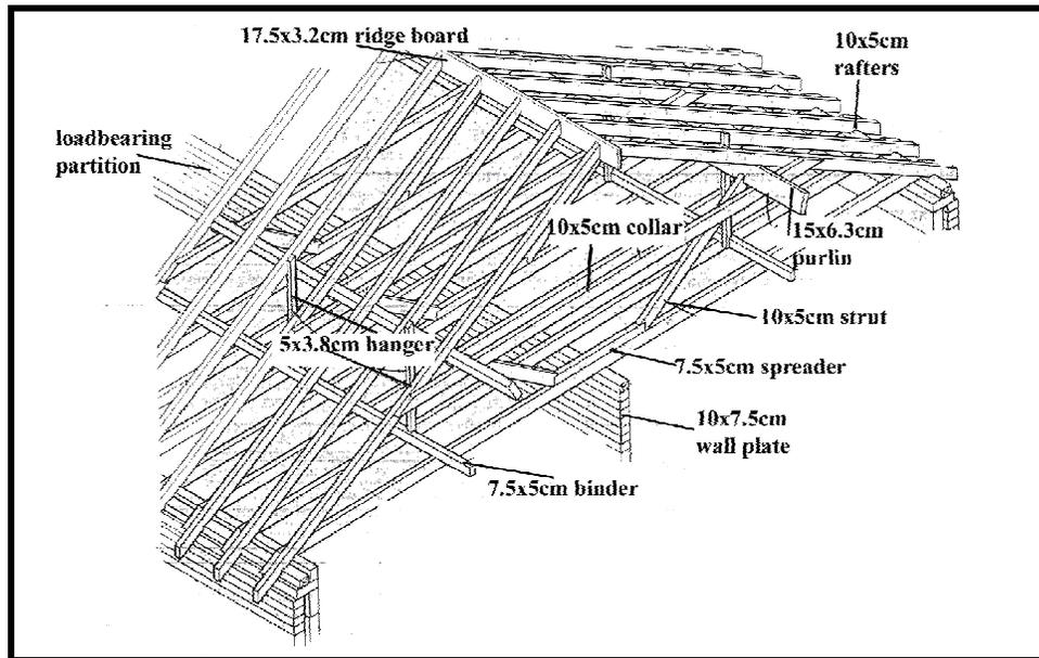
**Figure II. 16** Purlin roof construction (Foster, 1983:180).
