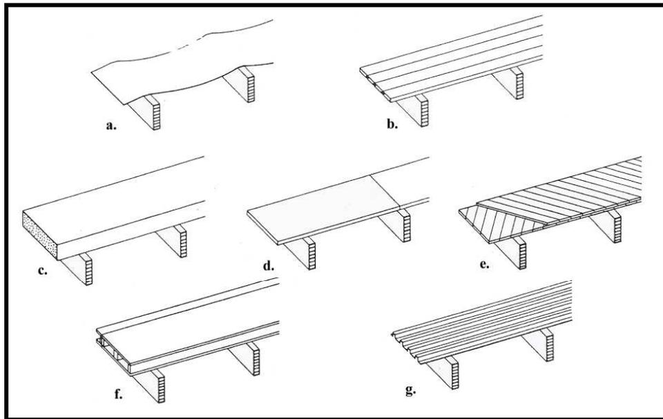
**Figure II. 10** Roof decking arrangements are: a) Fabric or plastic roof on braced beams, b) Tongue or groove planking or splined boards, c) Composite materials, d) Wood chipboards, plywood or furniture panels, e) Diagonal planking, f) Panel elements of timber slats or sheathing, g) Trapezoidal sheet metal (Götz *et al.*, 1989:127).
