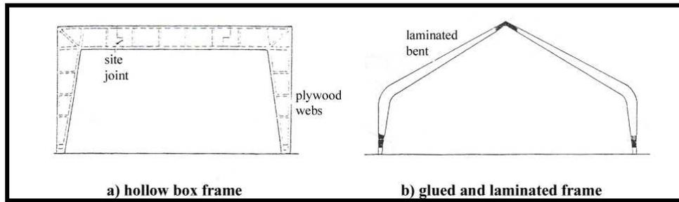
**Figure II. 36** Frame structures are arranged two different ways (Foster, 1983:350).
