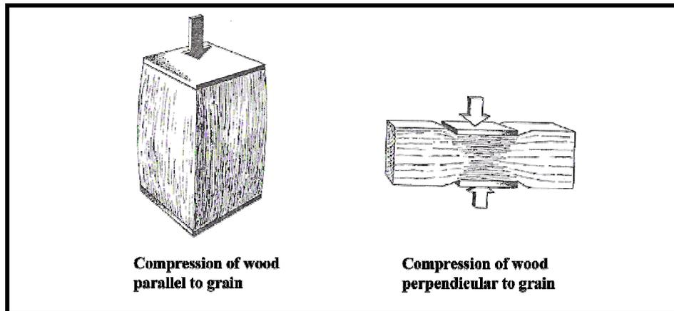
**Figure III. 4** Compression of wood parallel and perpendicular to grain (Oberg, 1963:80).
