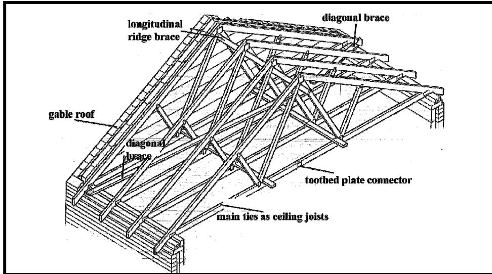
**Figure II. 17** Trussed rafter roof construction (Foster, 1983:191).
