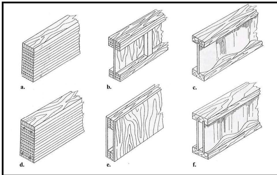
**Figure II. 3** Typical sections of glued laminated structures: a) solid rectangular section, b) ‘I’ section with a plywood web, c) ‘I’ section with a corrugated web, d) reinforced section, e) box shaped section, f) box shaped corrugated section (Karlsen, 1989:377).
