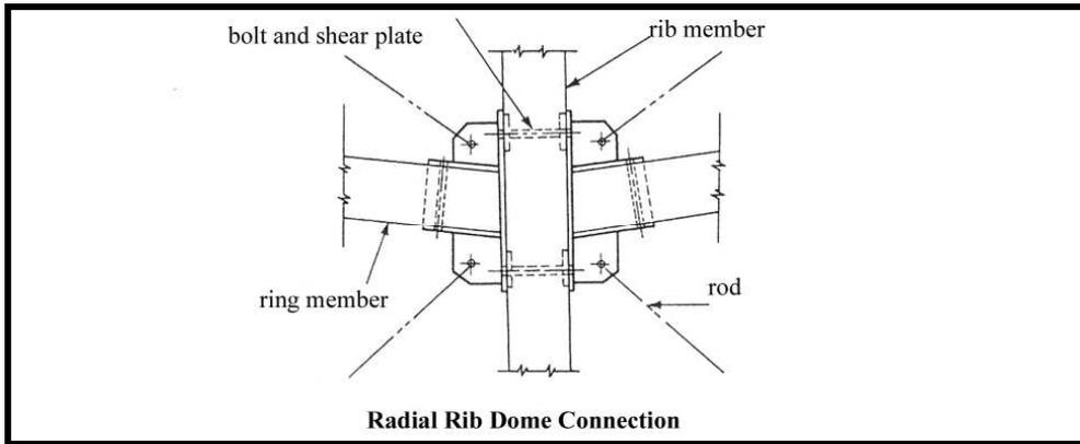
**Figure II. 59** The connections of the rib members are critical. Radial rib dome connection is illustrated in the figure (Faherty, 1989: 9.46).
