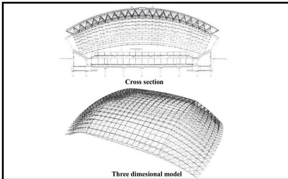
**Figure II. 45** Roof structure of Oguni Dome<sup>7</sup>, Japan (Chilton, 2000:76).
