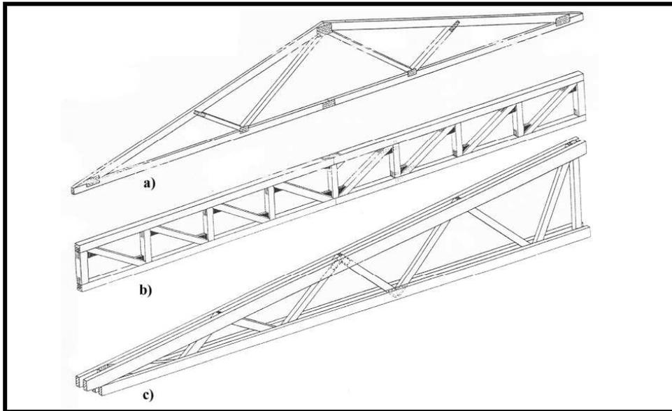
**Figure II. 28** a) Nail plate truss: Node plates consist of galvanized steel plates, they are pressed from both sides into wood. b) Greim truss: Steel plates are placed in sawn mortises and nailed from the outside without predrelling. c) Menig truss: Node plates are placed between struts and are not visible in the finished truss (Götz *et al.*, 1989:58).
