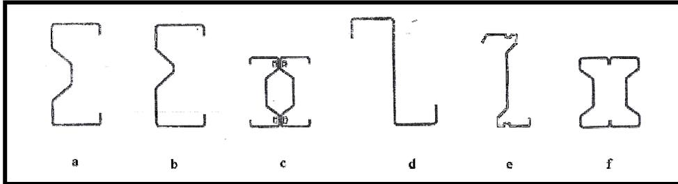
**Figure II. 7** Typical cold rolled steel sections (Owens, 1992:429).
