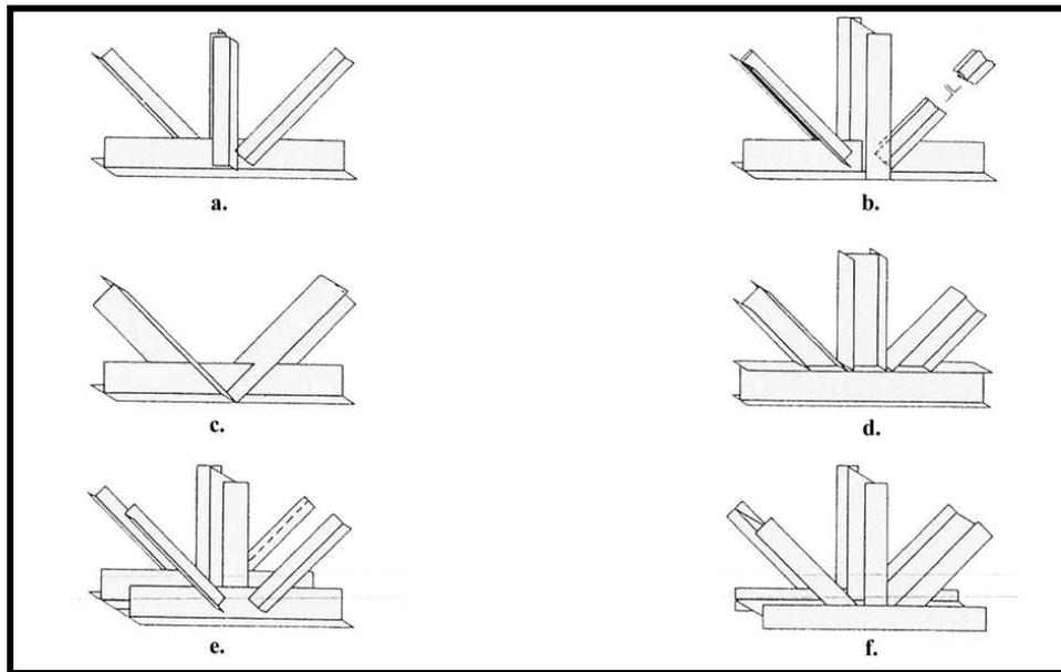
**Figure II. 31** Connections for simple welded trusses (Ellison, 1987:211).
