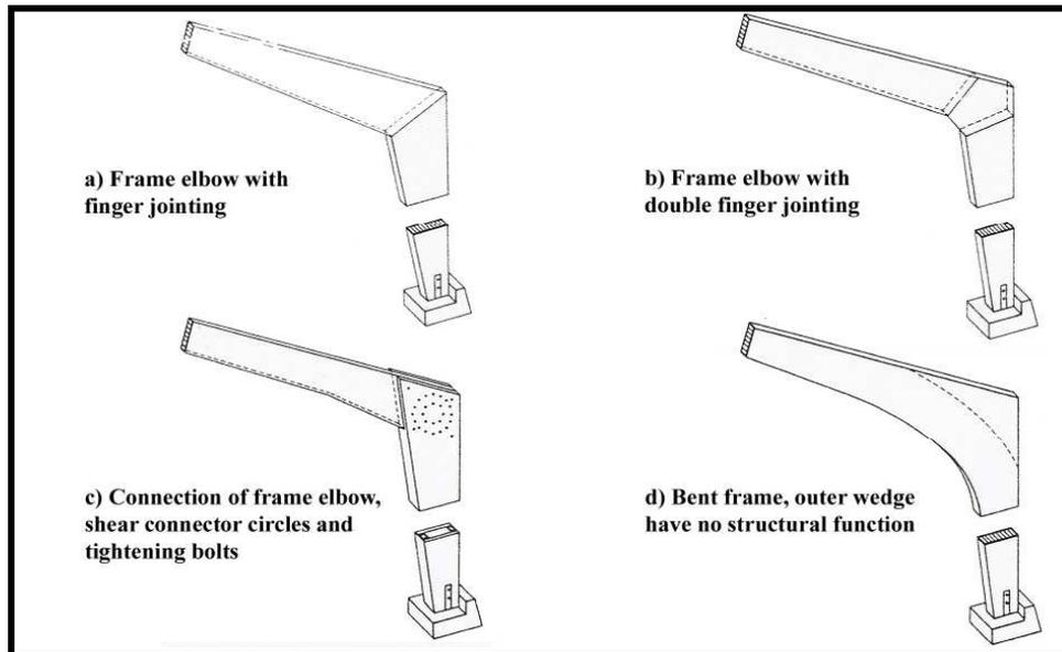
**Figure II. 39** Frame leg details for three hinged frames (Götz *et al.*, 1989:133).
