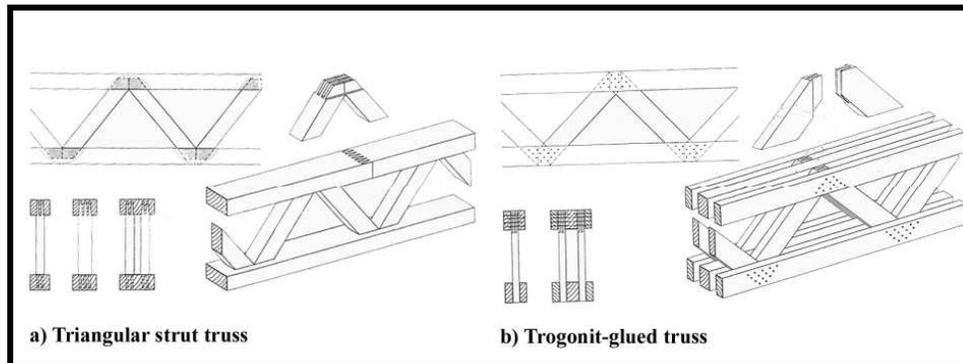
**Figure II. 27** Triangular struts are glued by finger joints, in trigonit girder truss diagonals are joined by finger joints, double or triple flanges are nailed together with each nail loaded in double shear (Götz *et al.*, 1989:55-56).
