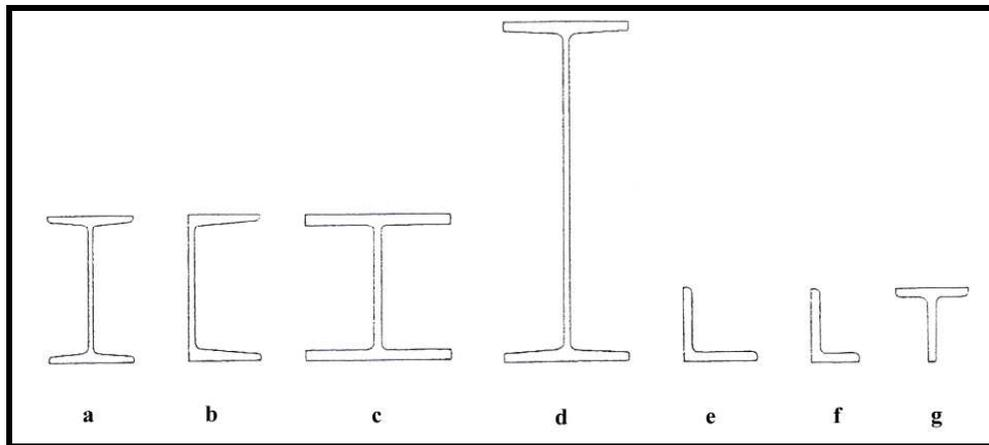
**Figure II. 6** Typical hot rolled steel sections (Foster, 1983:143).
