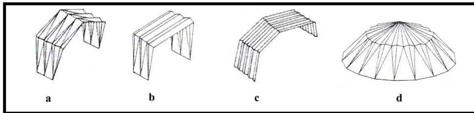
**Figure II. 48** Folded plate types: a) three pin folded plate portal frame, b) two pin folded plate portal frame, c) folded plate arch, d) folded plate dome (Benjamin, 1984:326).
