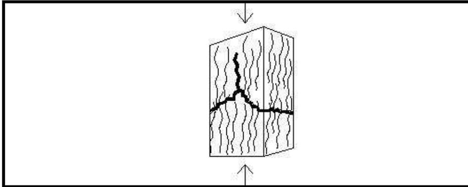
**Figure III. 5** Breakdown of a test specimen under a compressive load applied parallel to the grain (Karlsen, 1989: 22).
