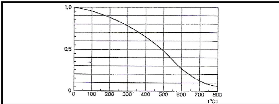
**Figure III. 30** Reduction factor for steel's stiffness at high temperatures (Eggen *et al.*, 1995:36).
