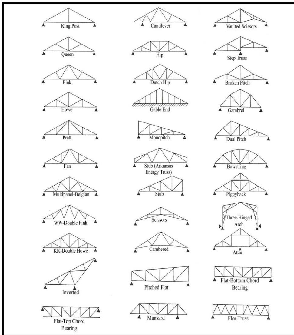
**Figure II. 26** Typical truss types have various names in different cultures (Faherty, 1989: 6.7-6.8).
