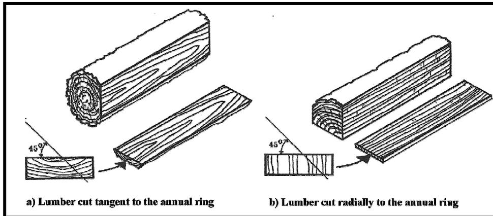
**Figure II. 2** Lumber is cut tangent or radially to the annual ring (Olin, 1990:201.22).
