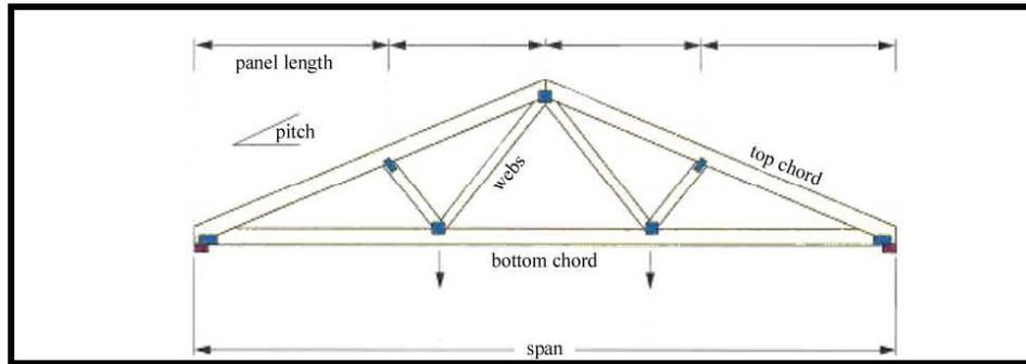
**Figure II. 25** Typical truss members and definitions in truss design (MiTek Solutions, document online).
