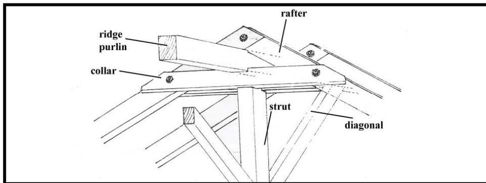
**Figure II. 13** Ridge connection in a three purlin hip roof is composed of rafters, purlins, collars, struts and diagonals (Binan, 1990:82).
