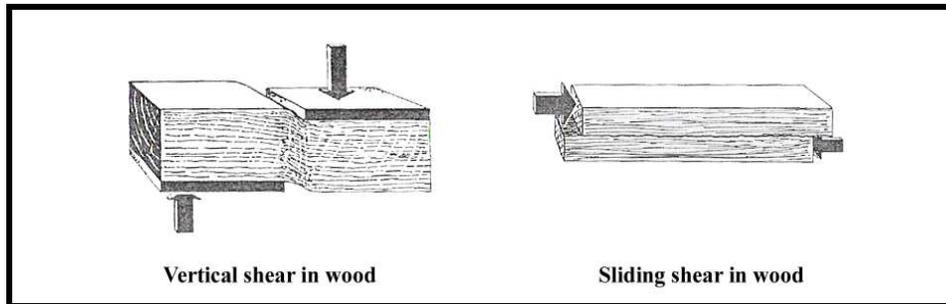
**Figure III. 7** Vertical shear in wood is a shearing that is perpendicular to the grain. Sliding shear in wood is a shearing stress that is parallel to the grain (Oberg, 1963:82).
