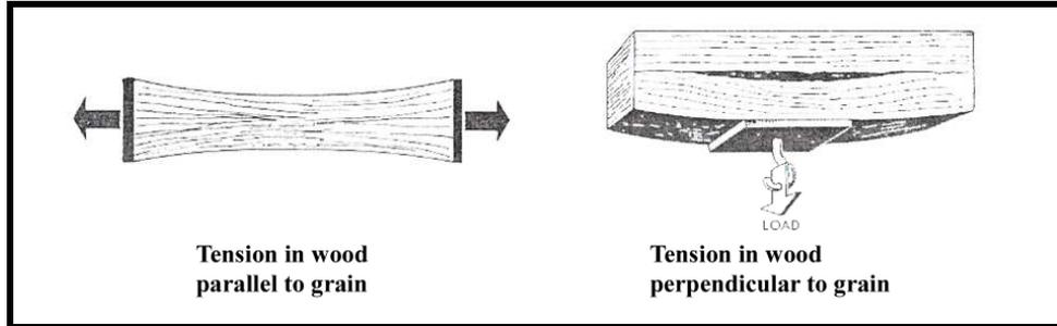
**Figure III. 6** Tension in wood parallel and perpendicular to grain (Oberg, 1963:81).
