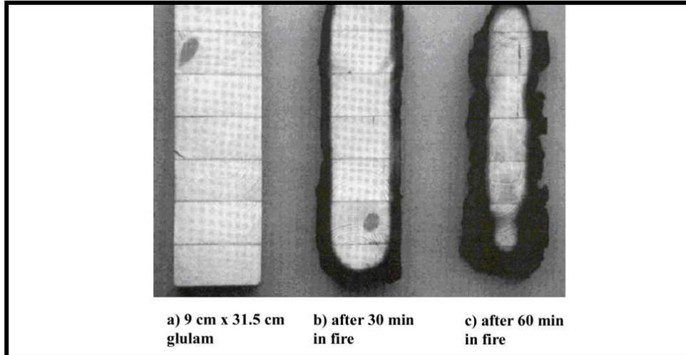
**Figure III. 28** The effect of fire at 30 and 60 minutes on a glulam piece, dimensions of the beam is 9 cm by 31.5 cm before fire (Glued Laminated Timber Association, Technical Data Sheet, document on-line).
