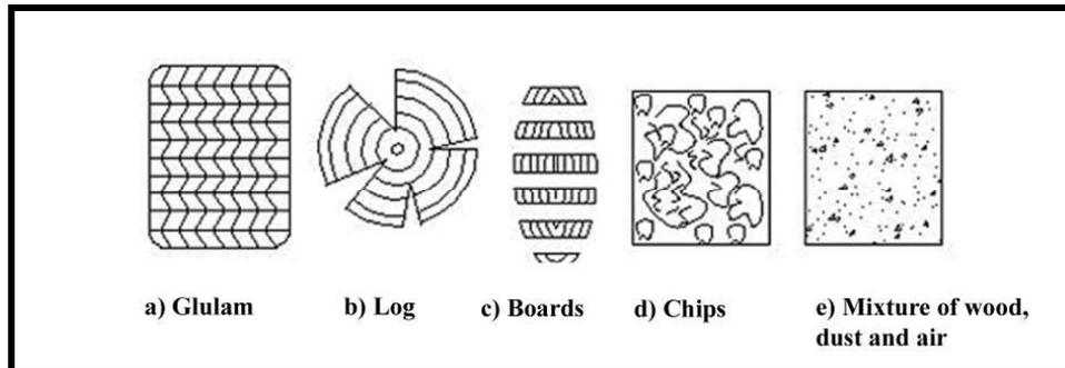
**Figure III. 27** Fire resistance of various wood members and materials. Glulam and log are the most fire resistant, in boards and chips fire resistance decrease, the mixture of wood dust and air is regarded as explosive (Karlsen, 1989:51).
