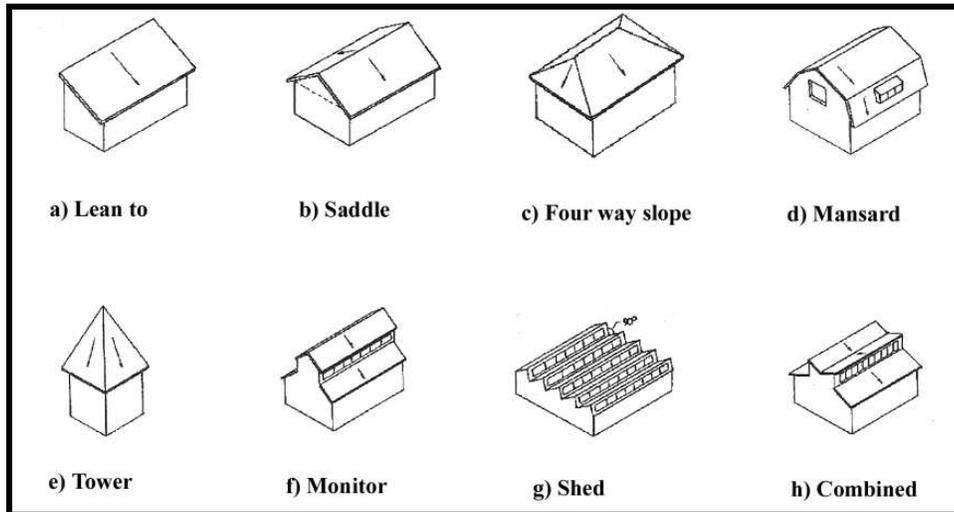
**Figure II. 11** Classification of roof forms (Özdemir, 2003:90-91).
