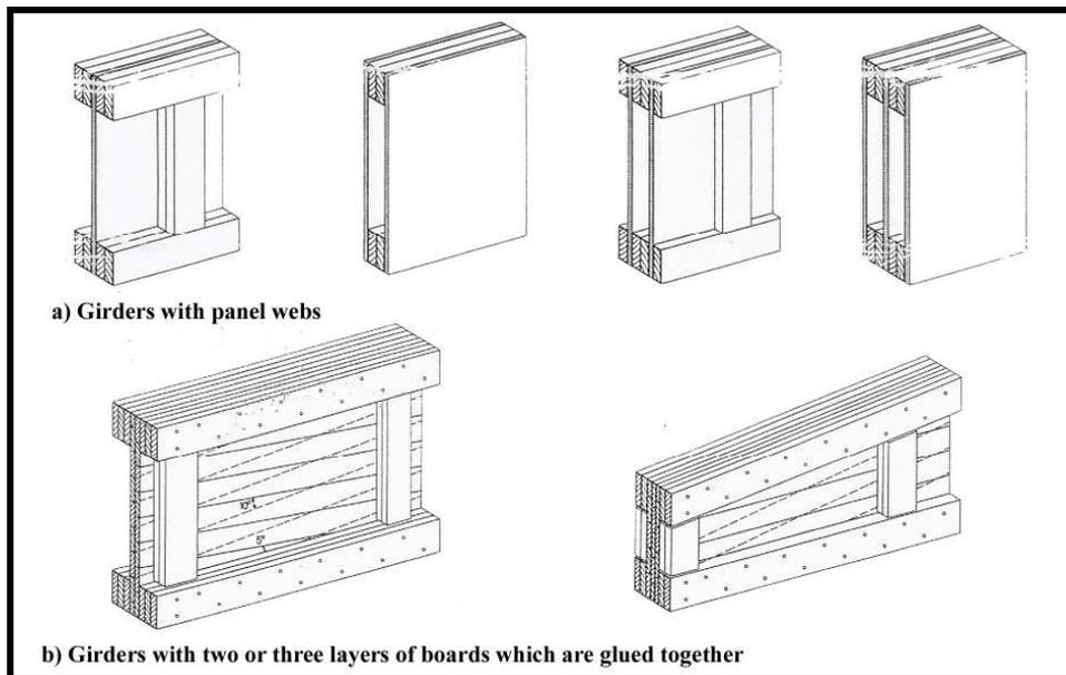
**Figure II. 18** Girders are composed of 'I' or box sections with panels or with glued boards (Götz *et al.*, 1989:57).
