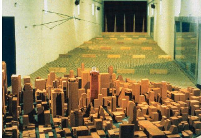
**Fig.4.1. Wind Tunnel Test** (The 1:500 Model of the Four Times Square Tower in the Center of New York )
