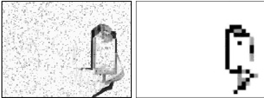
Figure 3.1: 10x10 blocks in frame difference detection provide a noiseless result
