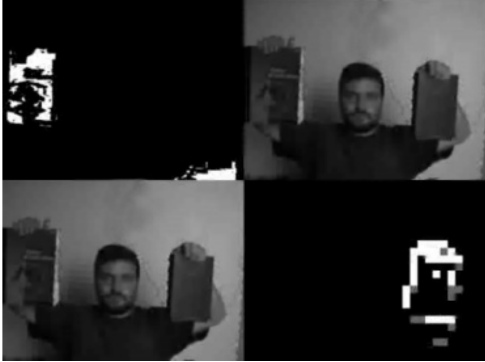
Figure 5.1: A snapshot of motion and color channels where the black book is under motion and orange one is stationary
