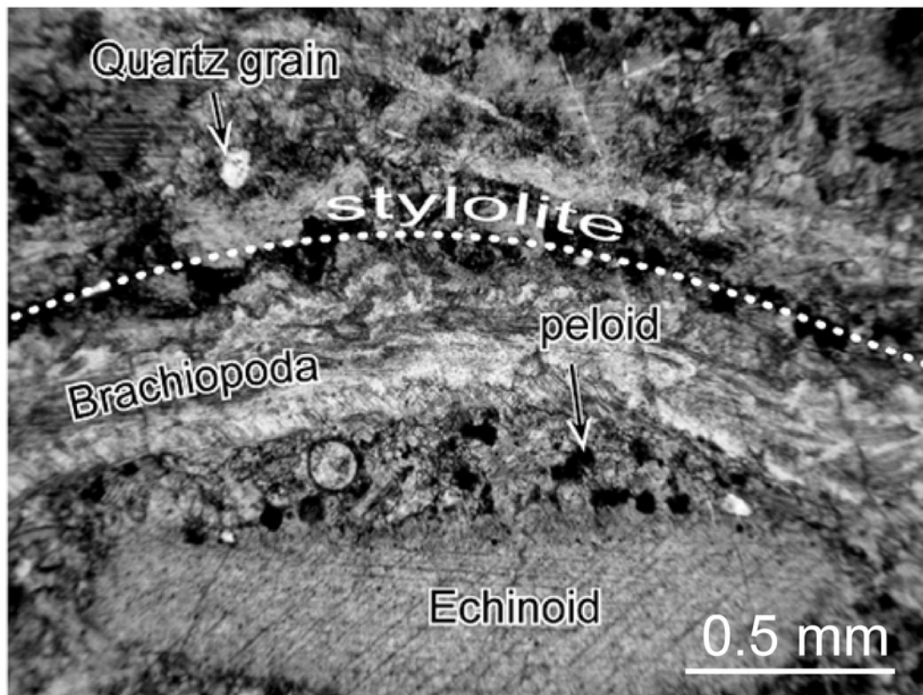
Figure 2.14: Photomicrograph of crinodal wackestone – packstone facies with stylolite Section AP, Sample AP-36.
