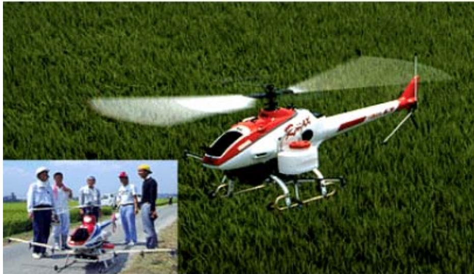
Figure 1.7. Yamaha industrial – use unmanned helicopter at work [8]
