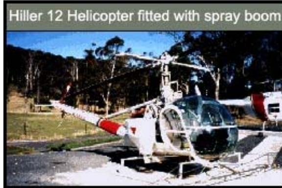
**Figure 1.5.** Hiller 12 Helicopter fitted with spray boom [7]
