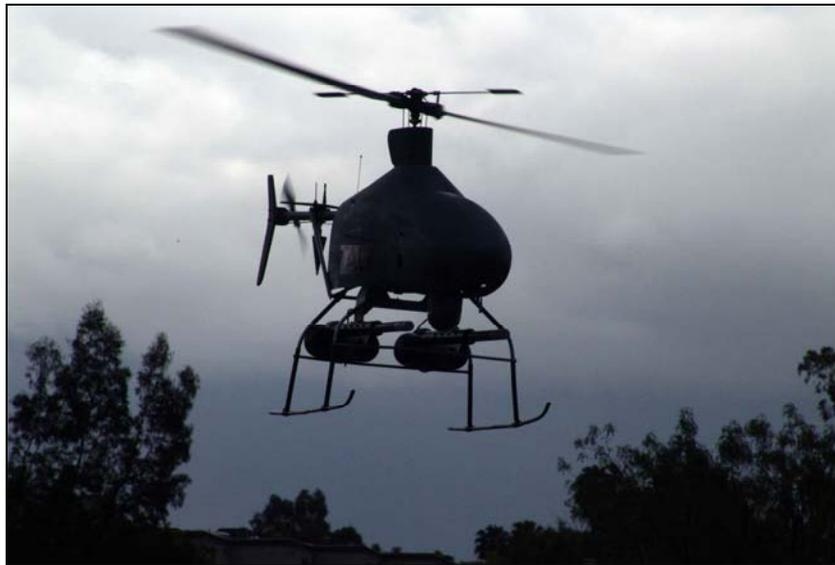
**Figure 1.8.** TAG UAV performing the role of ‘Crop Duster’ [9]
