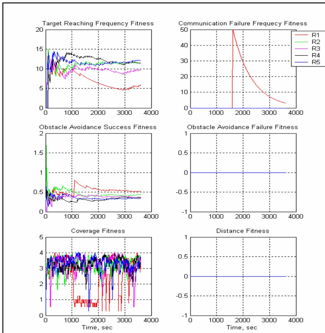
**Figure 95 Fitness functions for all robots. Red line is belonging to defective robot making physical errors.**
