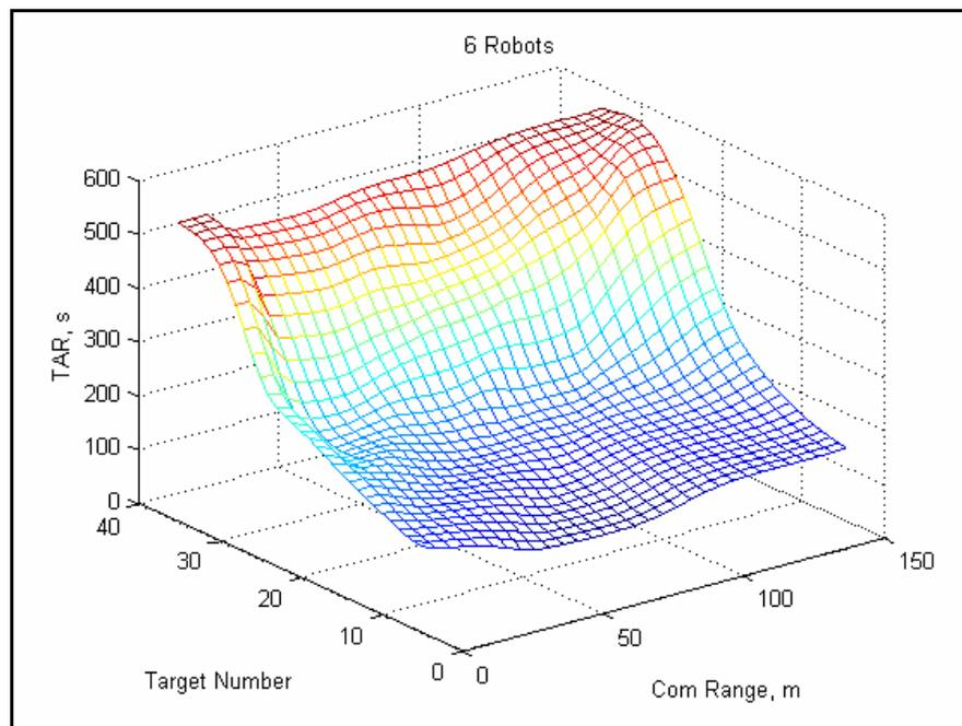
**Figure 80 Neural network TRT estimates for 6 robots for different target numbers and communication ranges**
