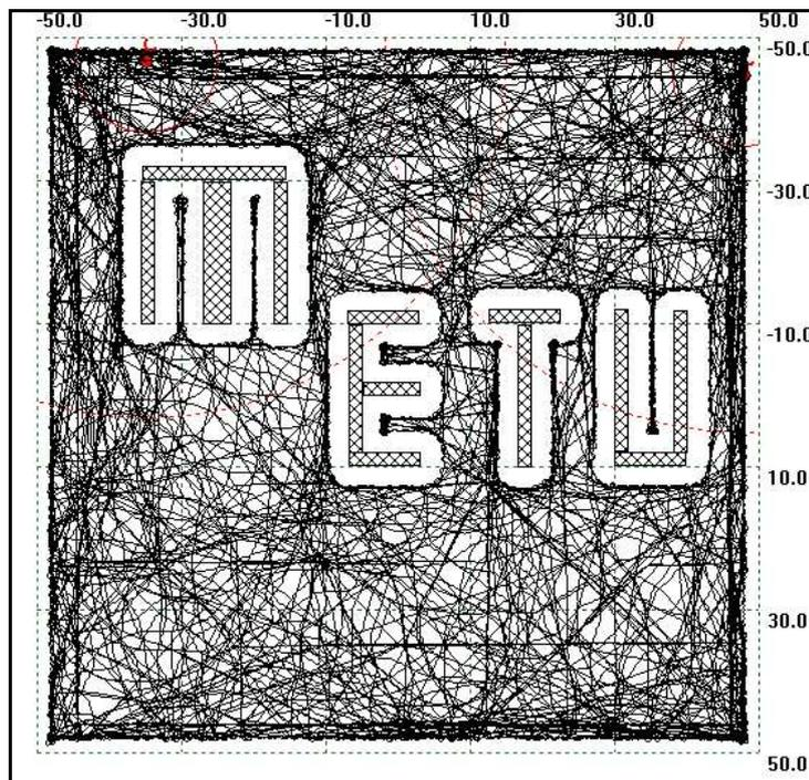
Figure 59, Final situation of two robots mapping. Black curves are the path of the robots.
