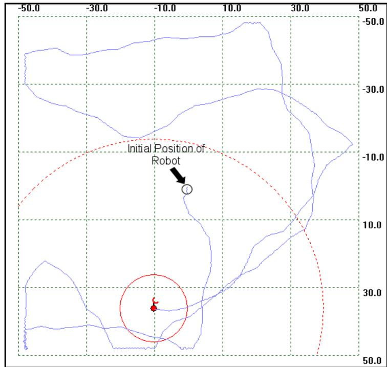
**Figure 54, Robot path after 200 seconds. Coverage is 56 percent.**
