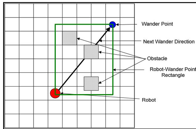
Figure 29, Robot-Wander Point rectangle for obstacle crash check
