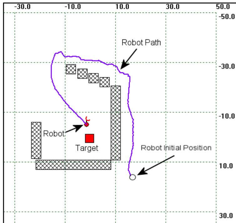
**Figure 49, Final position of obstacle avoidance from a concave obstacle. Robot avoided obstacle successfully by following shown path.**
