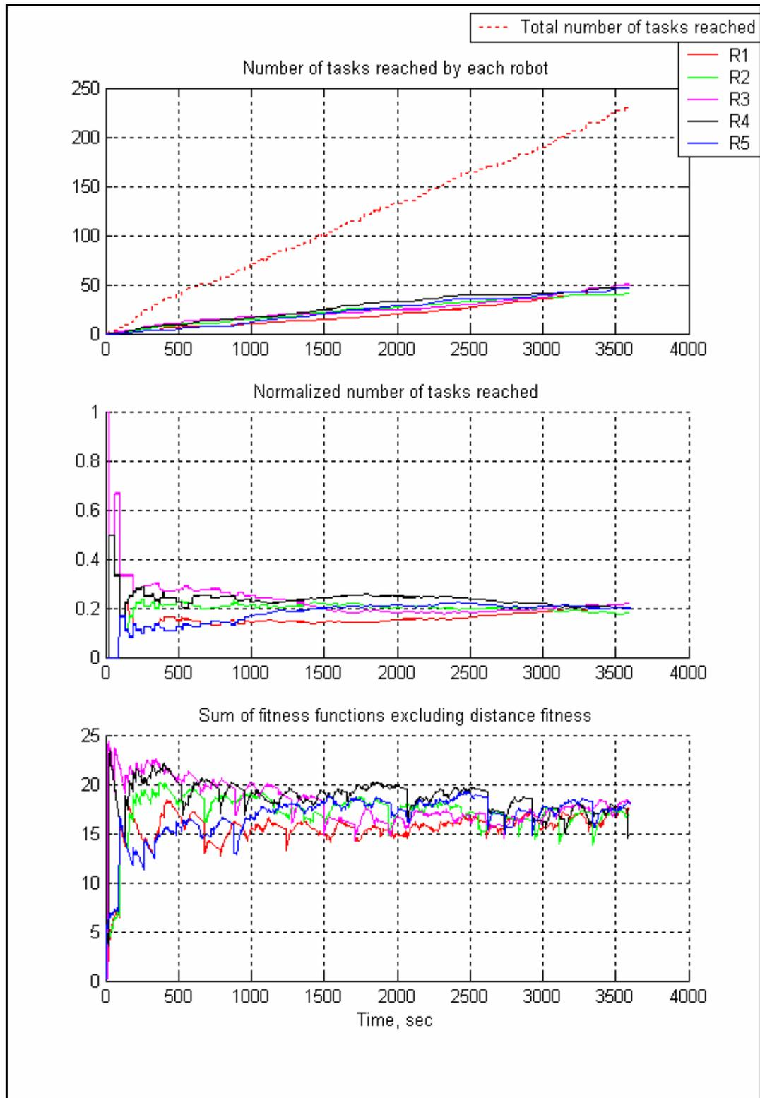
**Figure 85** Number of tasks reached statistics, and sum of fitness function excluding distance of 5 robots in obstacle-dense region for  $5/(100 \times 100)$  task/m<sup>2</sup> task density.
