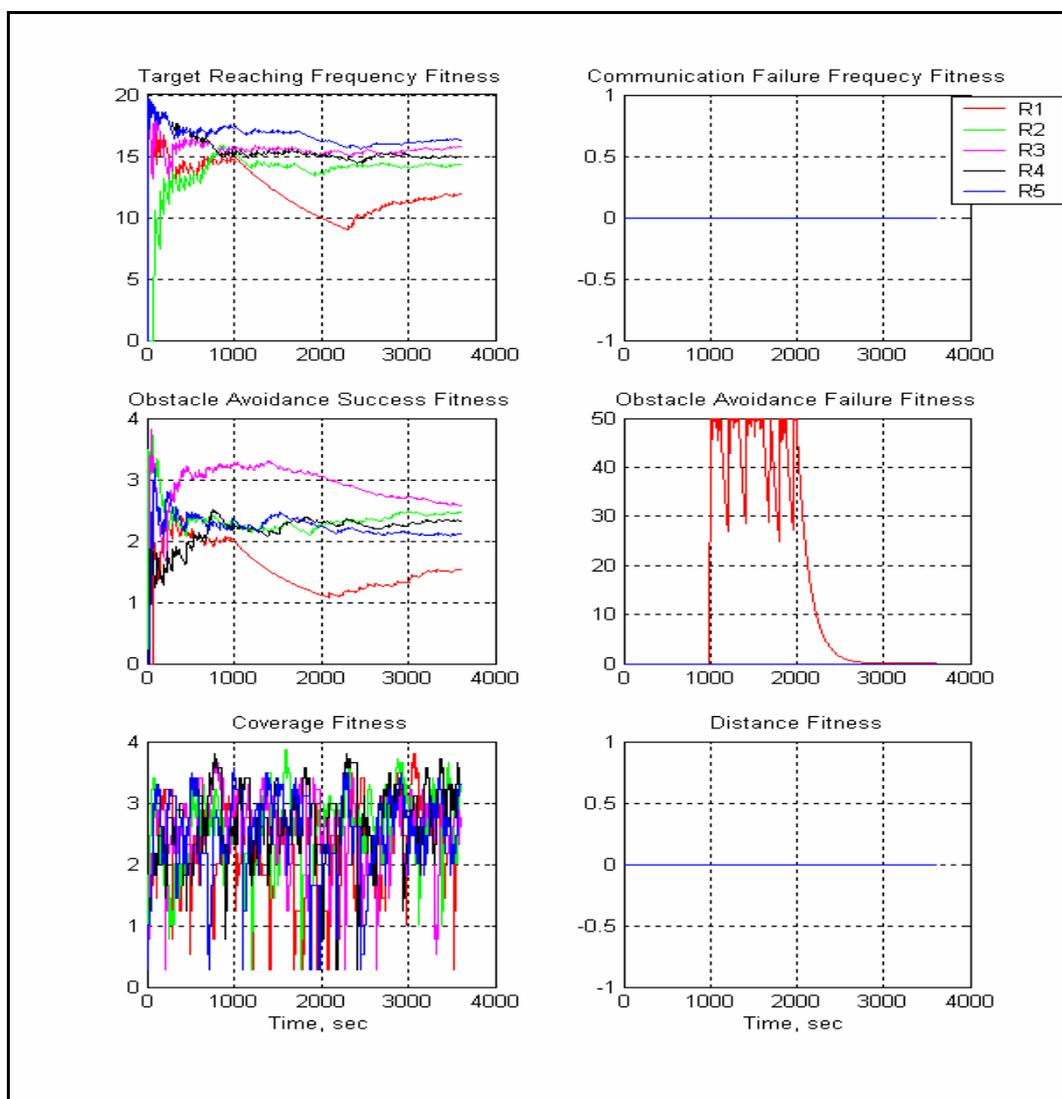
**Figure 93, Fitness functions for all robots. Red line is belonging to defective robot making obstacle avoidance errors.**
