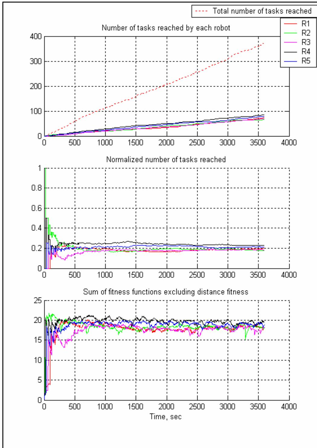
**Figure 83** Number of tasks reached statistics, and sum of fitness function excluding distance of 5 robots in obstacle-free region for 5/(100x100) task/m<sup>2</sup> task density.
