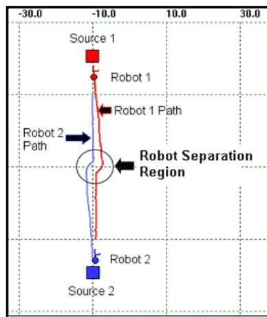
**Figure 52, Robots having initial positions shown in Figure 51 avoided collision each other in robot separation region successfully.**
