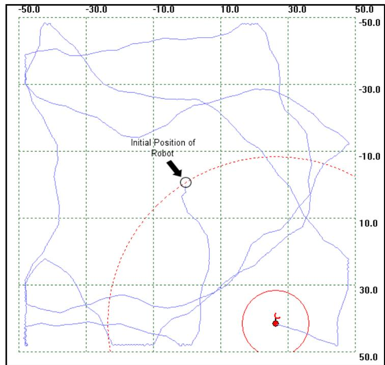
**Figure 55, Robot path after 300 seconds. Coverage is 77 percent.**
