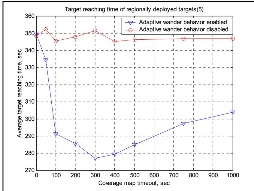
**Figure 72, Target reaching time of a single robot with respect to  $TO_{cov}$ . If Adaptive wander is enabled target reaching time decreases considerably in case of regionally deployed targets. There is a local minima optimizing dynamic response to regionally target deployments.**
