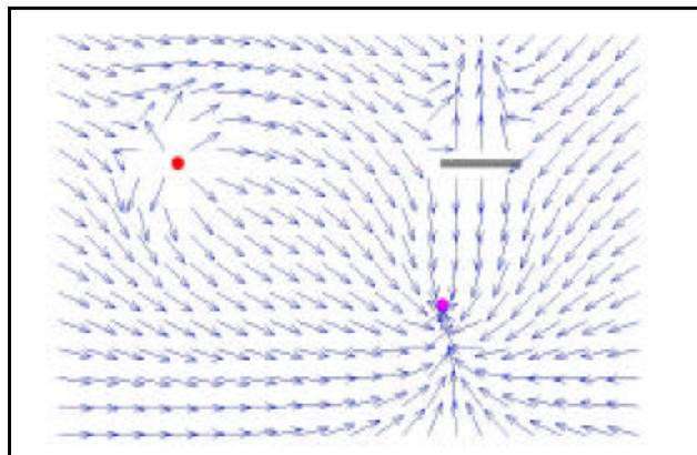
**Figure 7, Potential field forces generated by one attractive point, one repulsive point and one obstacle.**
