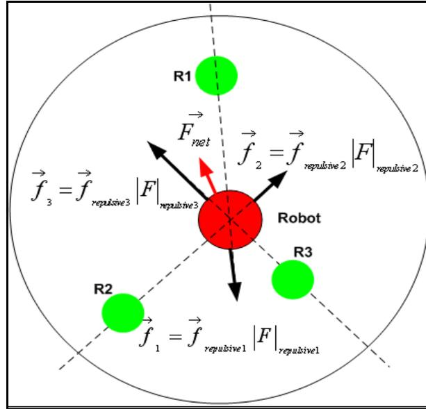
Figure 19, Robot Separation Forces
