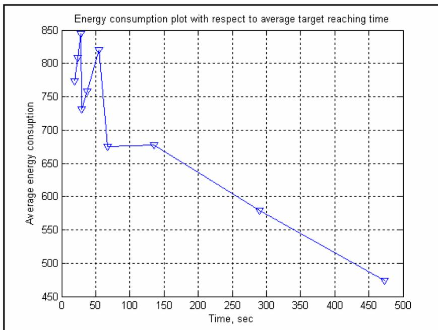
**Figure 71, Average energy consumption of different number of robots with respect to time. Each triangle corresponds to an energy-time-number of robots triplet.**
