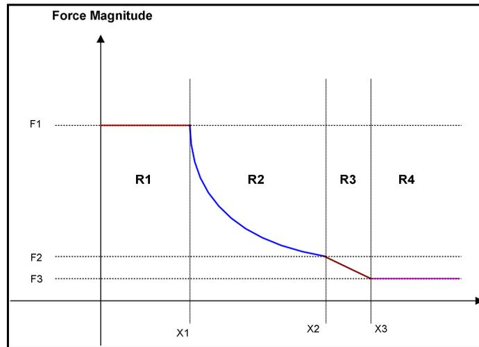
**Figure 15, Potential field force magnitude with respect to distance**
