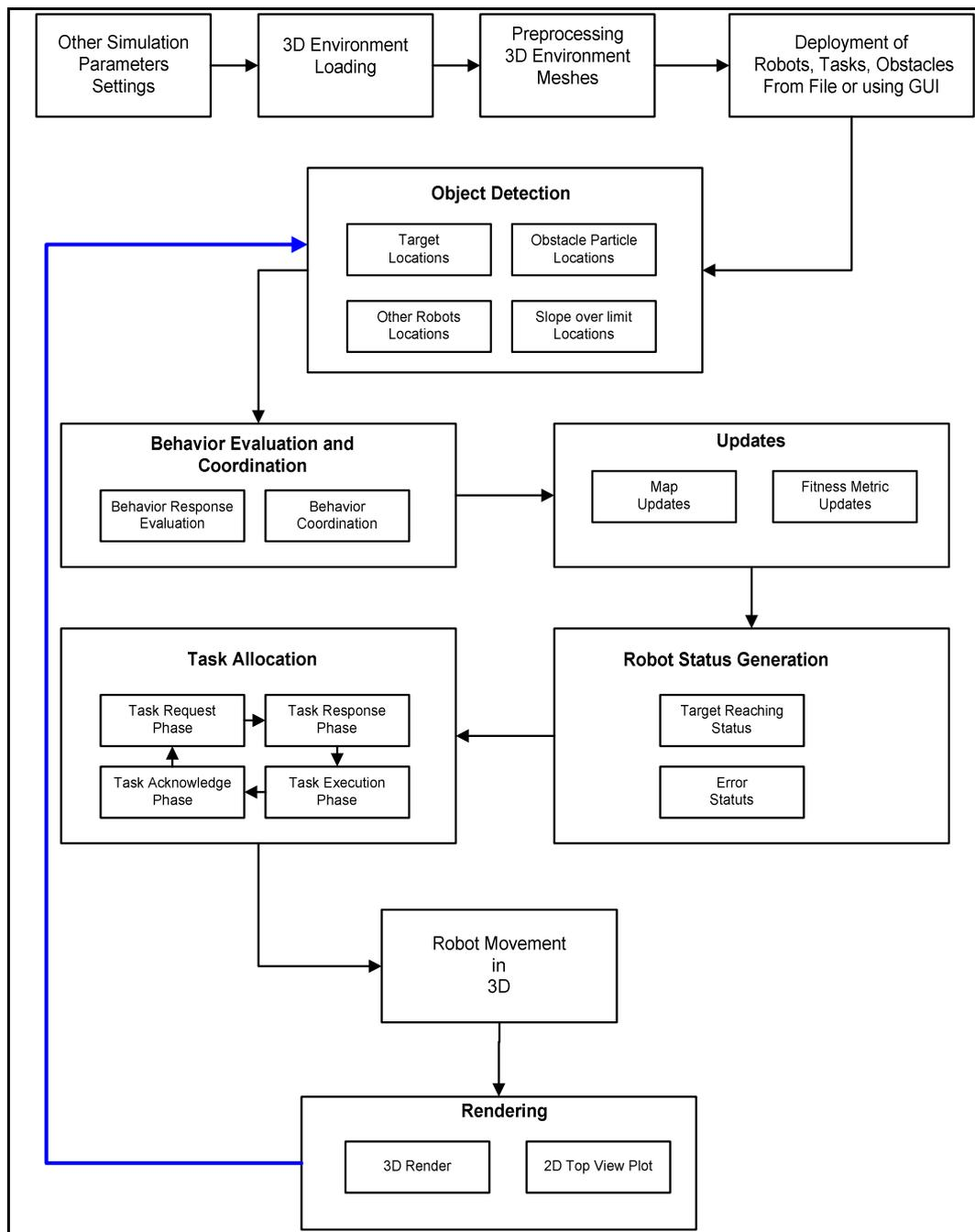
Figure 45 Flow of simulation for each robot
