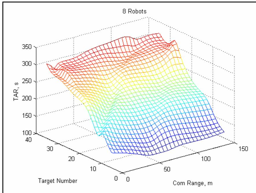
**Figure 81 Neural network TRT estimates for 8 robots for different target numbers and communication ranges**
