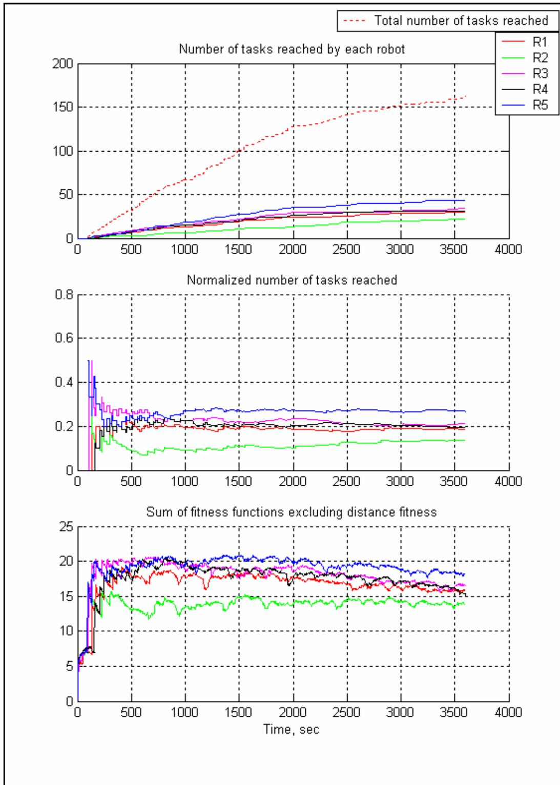
**Figure 88 Only target reaching frequency fitness function is activated. Number of tasks reached statistics, and sum of fitness function excluding distance of 5 robots in obstacle-dense region for 5/(100x100) task/m<sup>2</sup> task density.**
