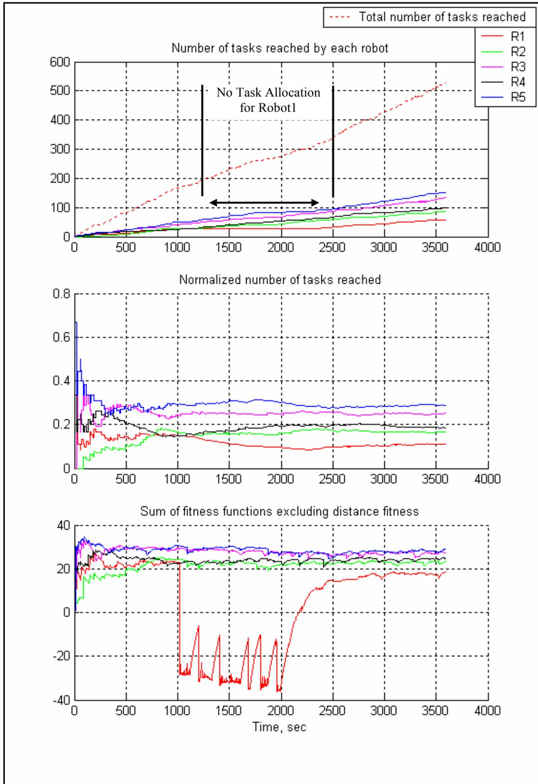
**Figure 94** Number of tasks allocated, and sum of fitness functions for all robots. Red line is belonging to defective robot making obstacle avoidance errors.
