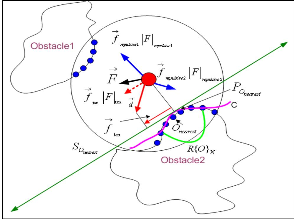
Figure 18, Tangential and repulsive force diagram.
