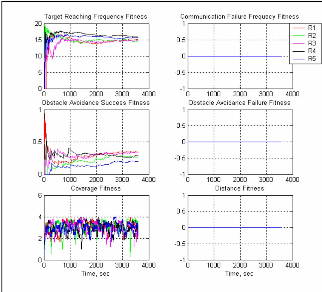
**Figure 82 Fitness functions of 5 robots in obstacle-free region for  $5/(100 \times 100)$  task/ $m^2$  task density.**
