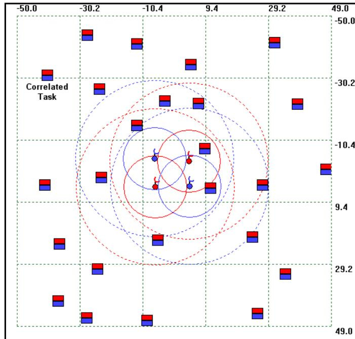
**Figure 73** A screen shot from simulation environment for 6 robots and 25 correlated tasks. Communication range is 25 for each robot.
