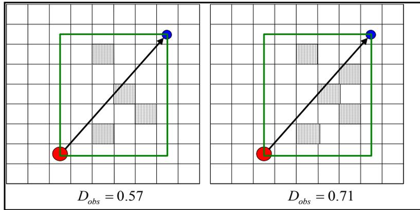
Figure 30, Obstacle Density for two situations. Image at the left hand side has obstacle density 0.57 whereas right hand side situation has 0.71 obstacle density.
