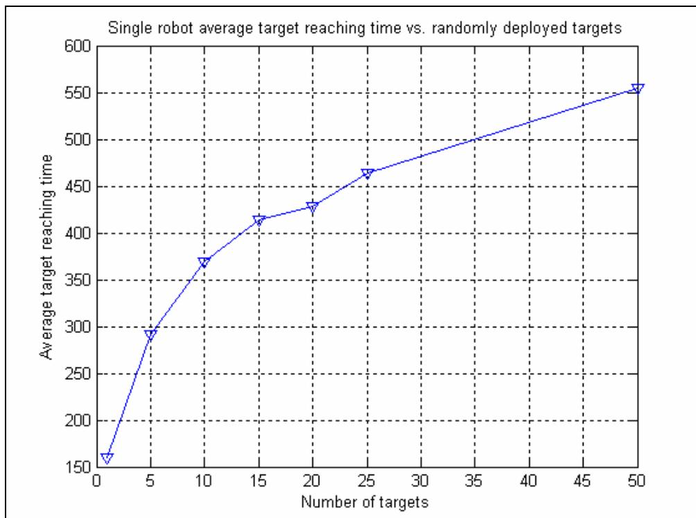
**Figure 68, Average target reaching time of single robot with respect to different number of randomly deployed targets.**
