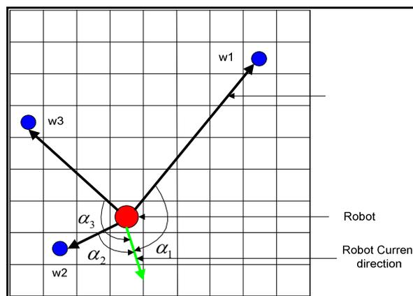
Figure 31, Wander point angle with respect to robot current direction
