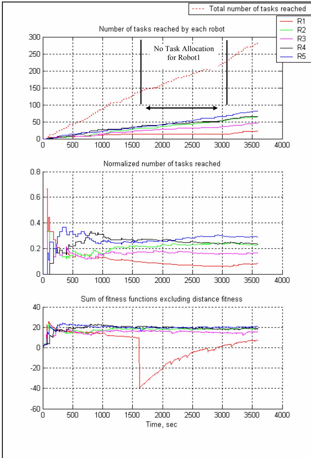
**Figure 96 Number of tasks allocated, and sum of fitness functions for all robots. Red line is belonging to defective robot making physical integrity errors.**
