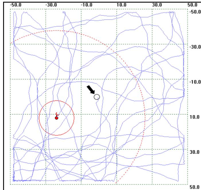
**Figure 57, Robot path after 900 seconds. Robot has covered the entire region.**
