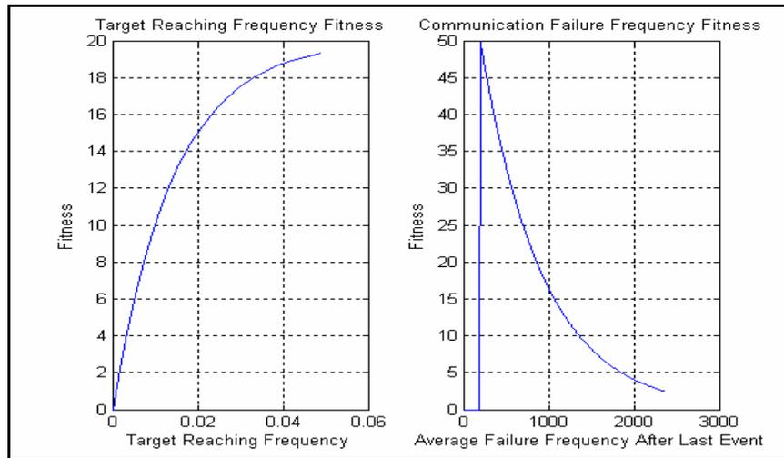
**Figure 39, Target reaching frequency, and communication failure frequency fitness plot with parameters in Table 6. At  $t_0 = 200$  seconds a communication failure is occurred.**
