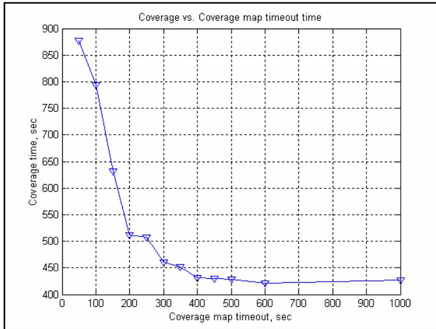
Figure 62, 95% Coverage for different coverage map timeouts,  $TO_{cov}$ . There is an inverse proportionality between coverage time and  $TO_{cov}$ .
