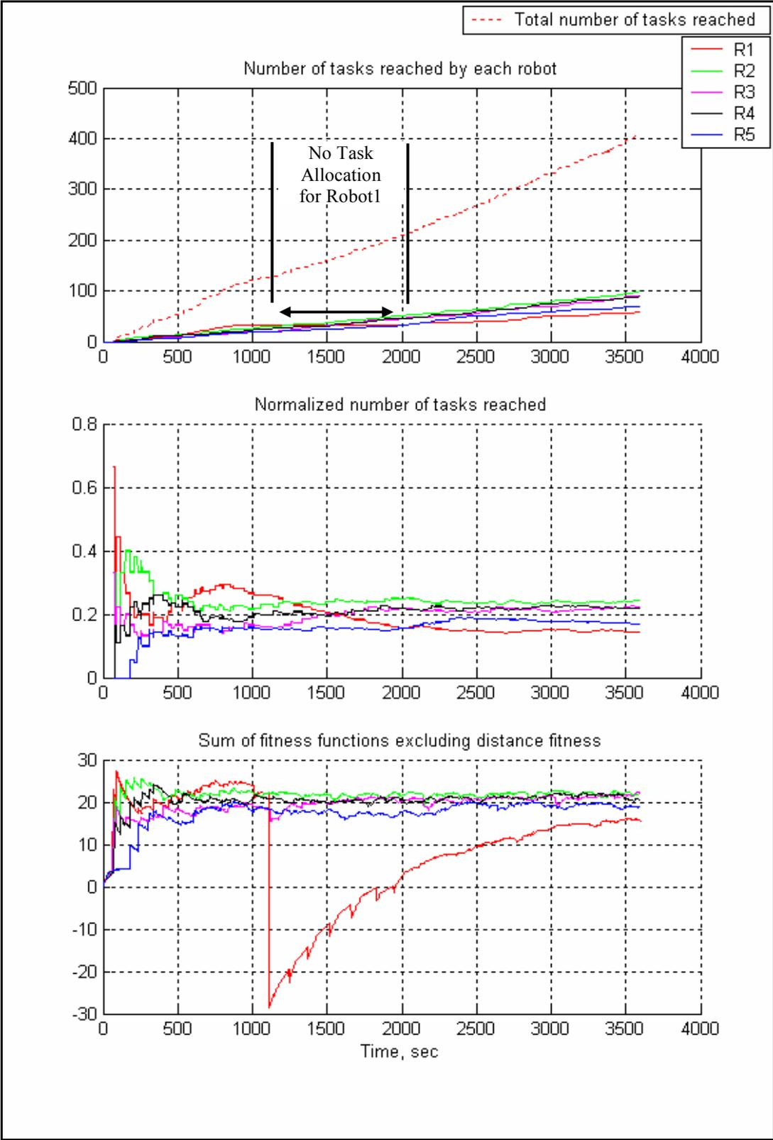
**Figure 92** Number of tasks allocated, and sum of fitness functions for all robots. Red line is belonging to defective robot making target reaching errors.
