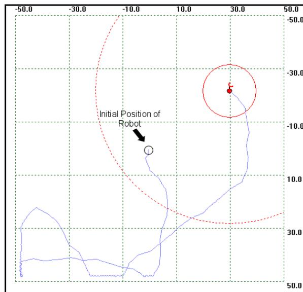
**Figure 53, Robot path generated by heuristic wander behavior after 100 seconds from startup.
