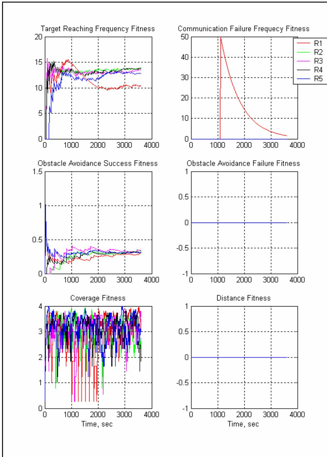
**Figure 91 Fitness functions for all robots. Red line is belonging to defective robot making target reaching errors.**
