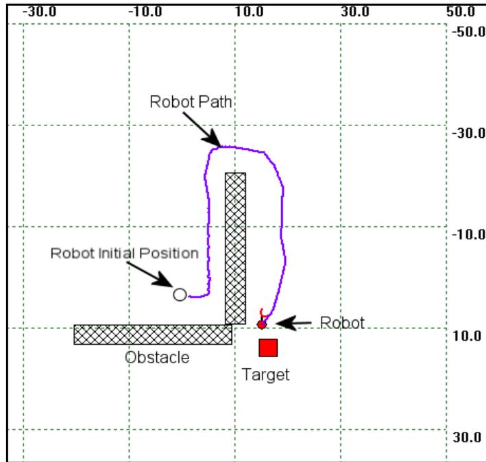
**Figure 48, Final position of obstacle avoidance from a partially concave obstacle. Robot avoided obstacle successfully by following shown path.**
