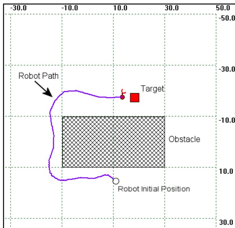
**Figure 47, Final position of obstacle avoidance from rectangular shaped, convex obstacle. Robot avoided obstacle successfully by following shown path.**
