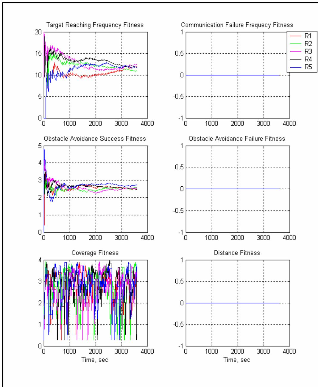
**Figure 84, Fitness functions of 5 robots in obstacle-dense region for 5/(100x100) task/m<sup>2</sup> task density**
