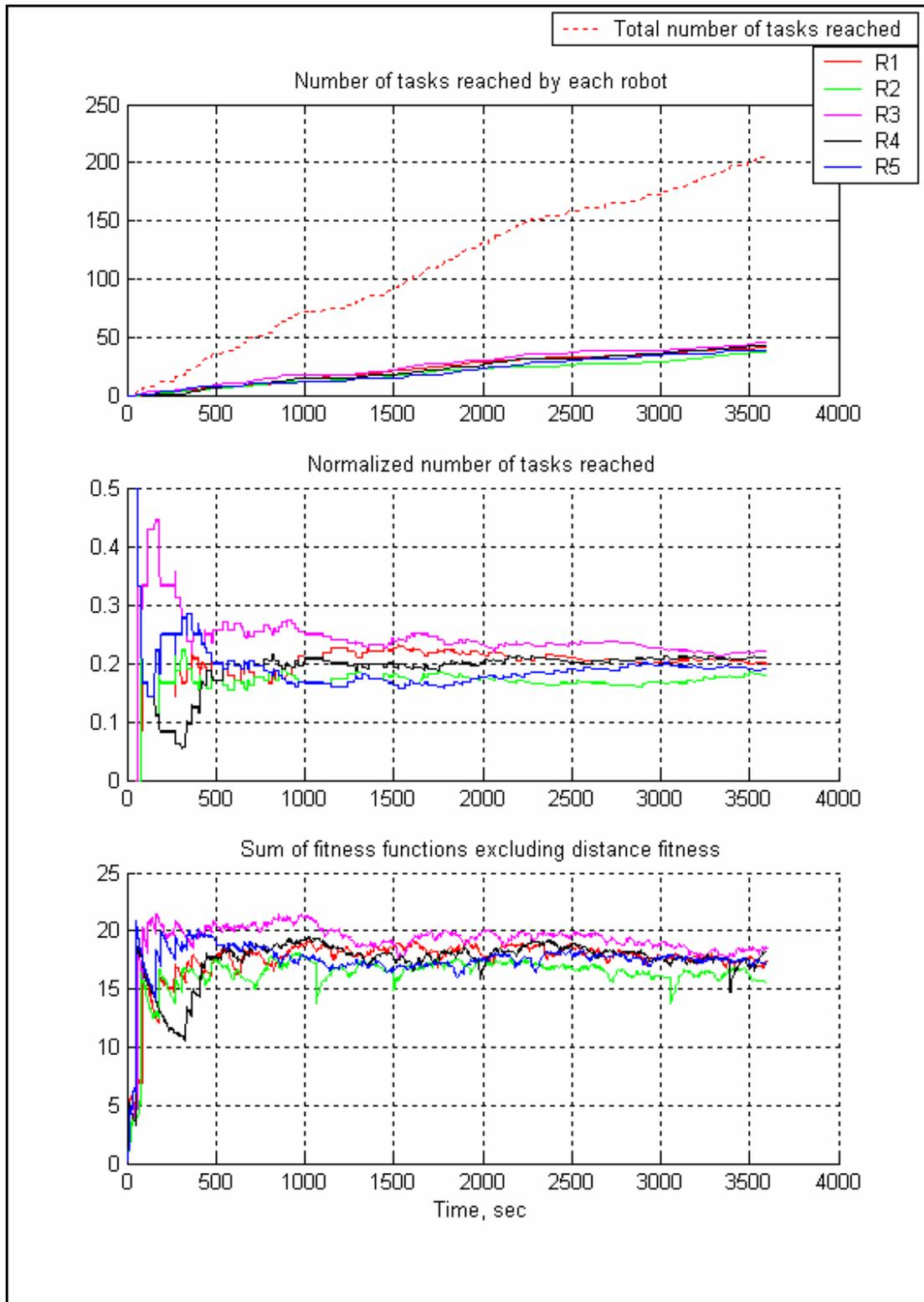
**Figure 89 Only Coverage fitness function is activated. Number of tasks reached statistics, and sum of fitness function excluding distance of 5 robots in obstacle-dense region for  $5/(100 \times 100)$  task/m<sup>2</sup> task density**
