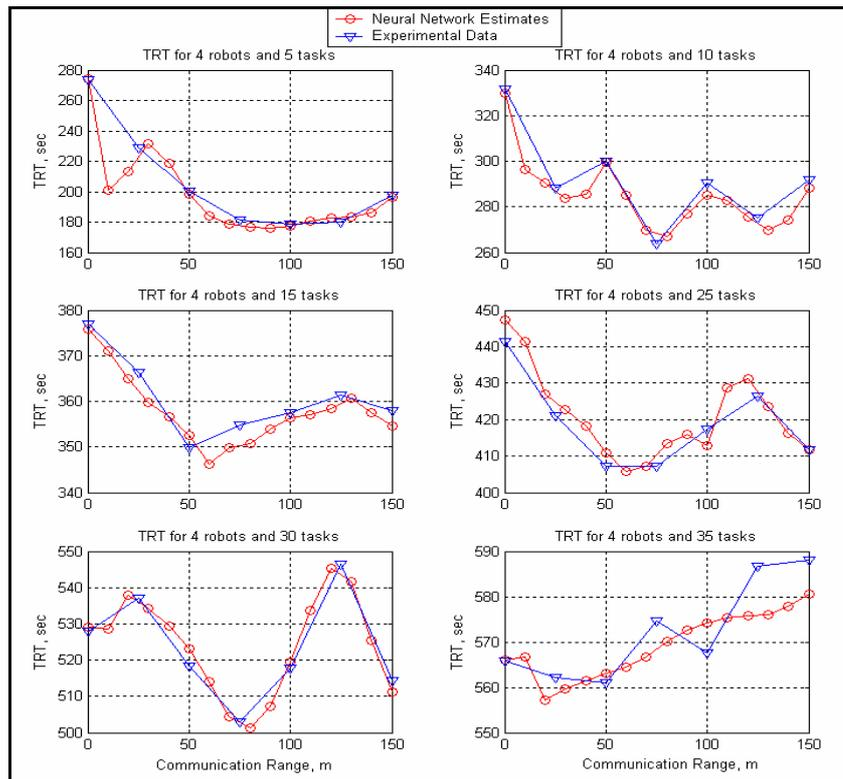
**Figure 74, Target reaching time (TRT) for 4 robots and different number of task and communication ranges. Neural network estimates are also shown as red lines with more resolution.**
