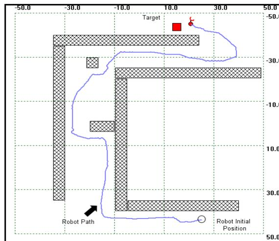
Figure 64, Target reaching in an environment filled by long and small rectangular obstacles.
