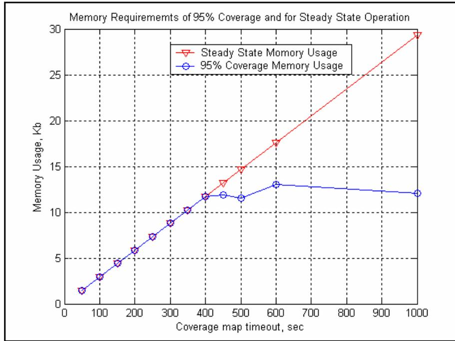
**Figure 63, Memory usage at steady state and memory usage for 95% coverage. After  $TO_{cov} = 400$  seconds, difference between memory usage increases considerably. Appropriate  $TO_{cov}$  value should be selected by considering this observation.**
