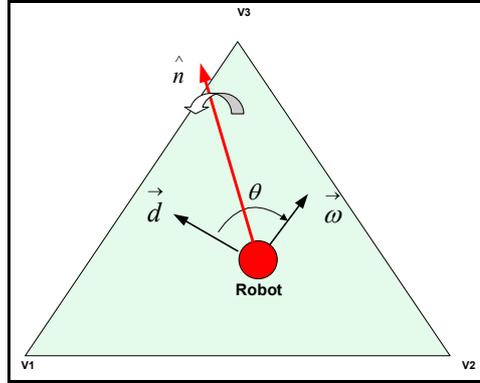
**Figure 20, robot generated a direction randomly by rotating it direction around normal vector of current grid that robot resides.**
