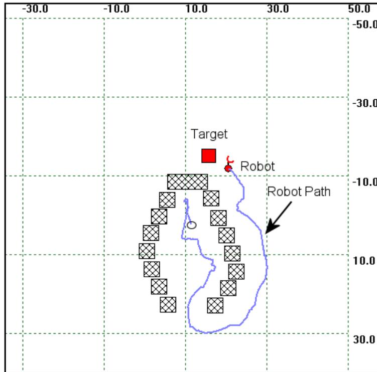
**Figure 50, Final position of obstacle avoidance from a strongly concave obstacle. Robot avoided obstacle successfully by following shown path.**
