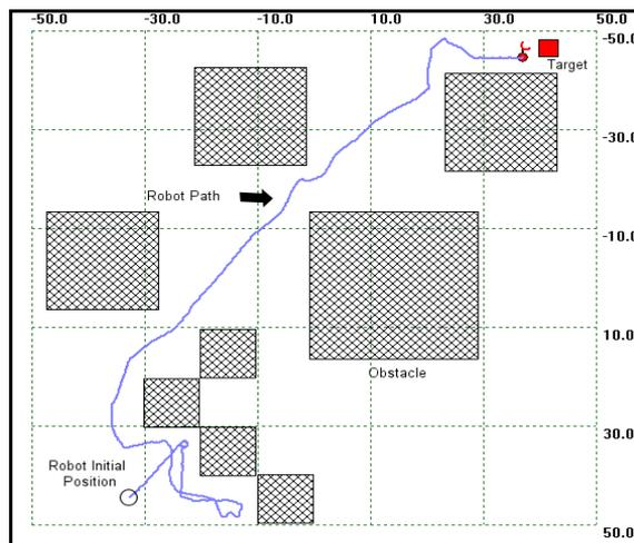
Figure 65, Target reaching in an environment filled by dense concave and convex shaped obstacles.
