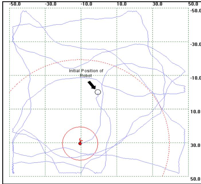
**Figure 56, Robot path after 400 seconds. Coverage is 83 percent.**
