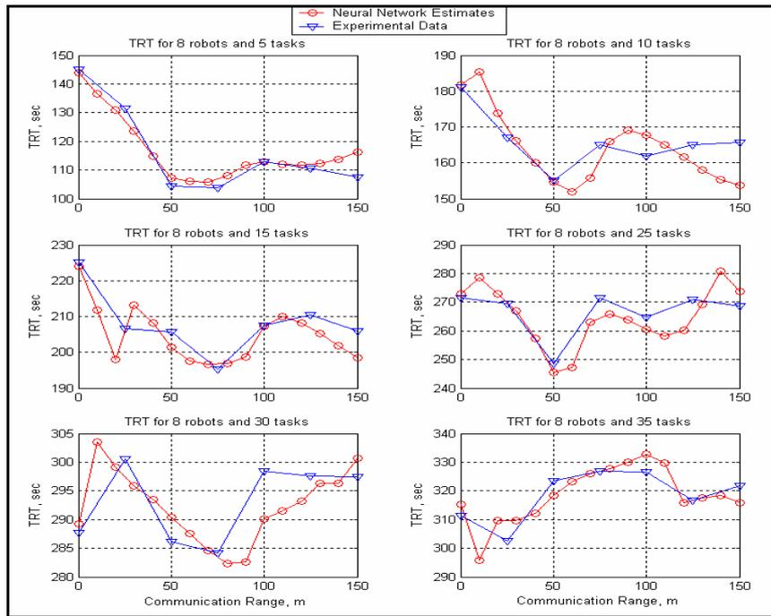
Figure 75, Target reaching time (TRT) for 8 robots and different number of task and communication ranges.
