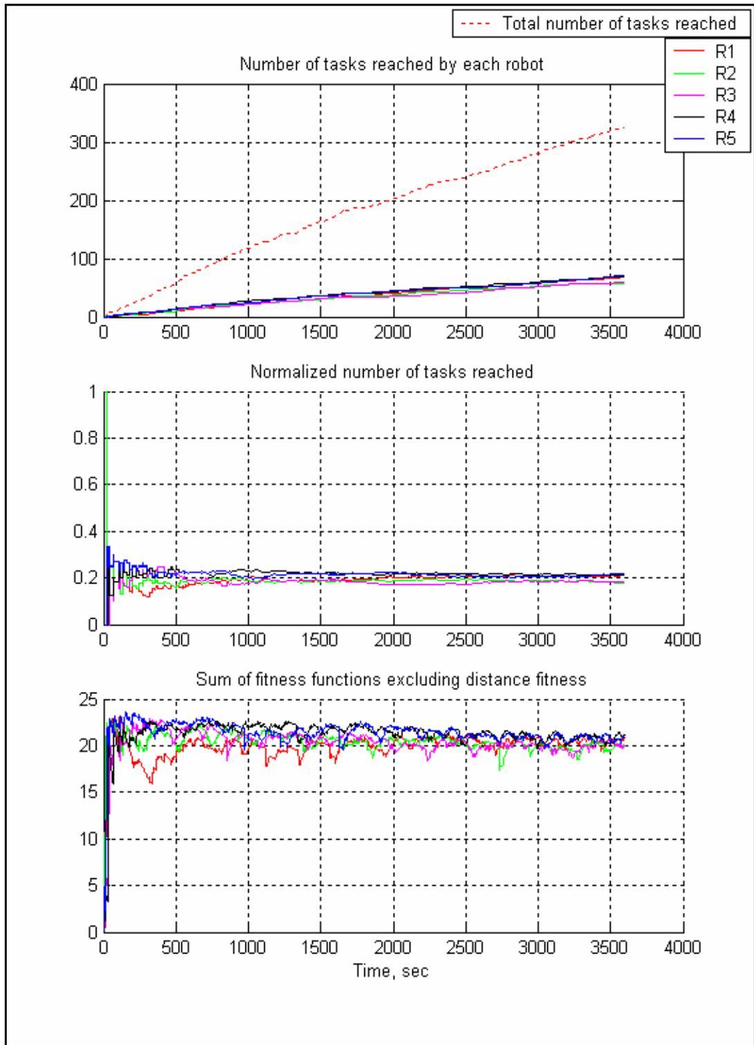
**Figure 87** Number of tasks reached statistics, and sum of fitness function excluding distance of 5 robots in obstacle-dense region for  $10/(100 \times 100)$  task/m<sup>2</sup> task density.
