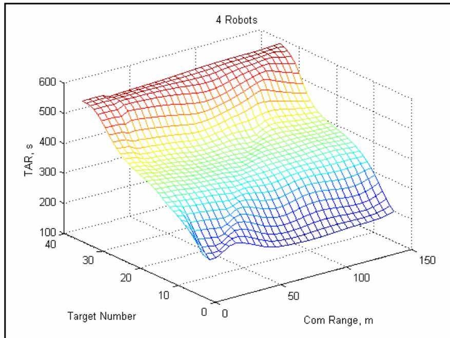
**Figure 79 Neural network TRT estimates for 4 robots for different target numbers and communication ranges**
