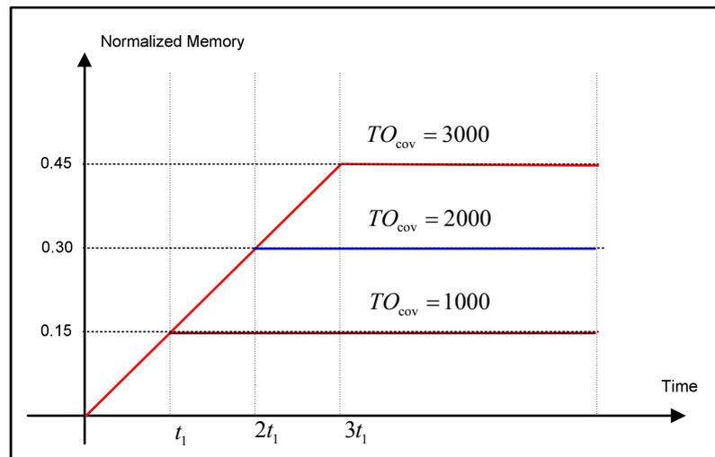
Figure 25, Normalized memory requirement versus time for coverage map. Each line corresponds to different timeout time.
