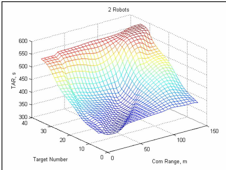
Figure 78, Neural network TRT estimates for 2 robots for different target numbers and communication ranges
