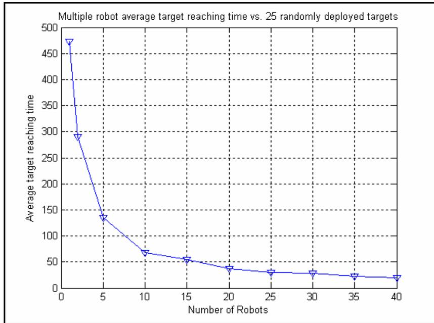
**Figure 69, Average target reaching time of different number of randomly deployed robots to randomly deployed 25 targets.**
