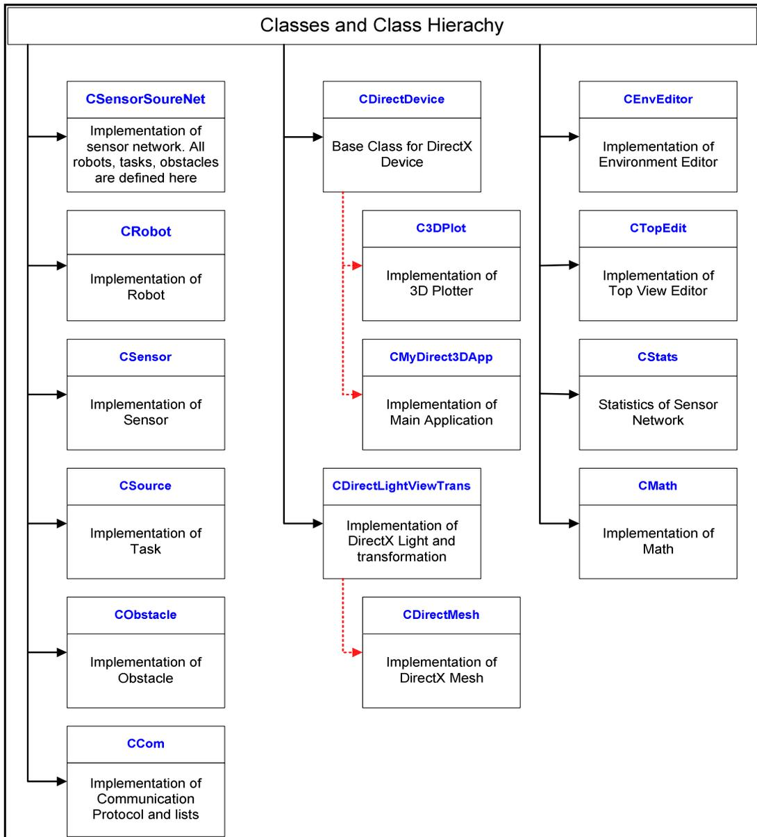
Figure 44, Classes, and class hierarchy used in simulator
