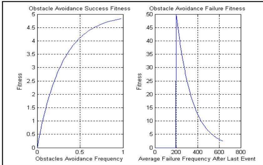
**Figure 40** Obstacle avoidance success, and failure frequency fitness plot with parameters in Table 6. At  $t_0 = 200$  seconds a obstacle avoidance failure is occurred.
