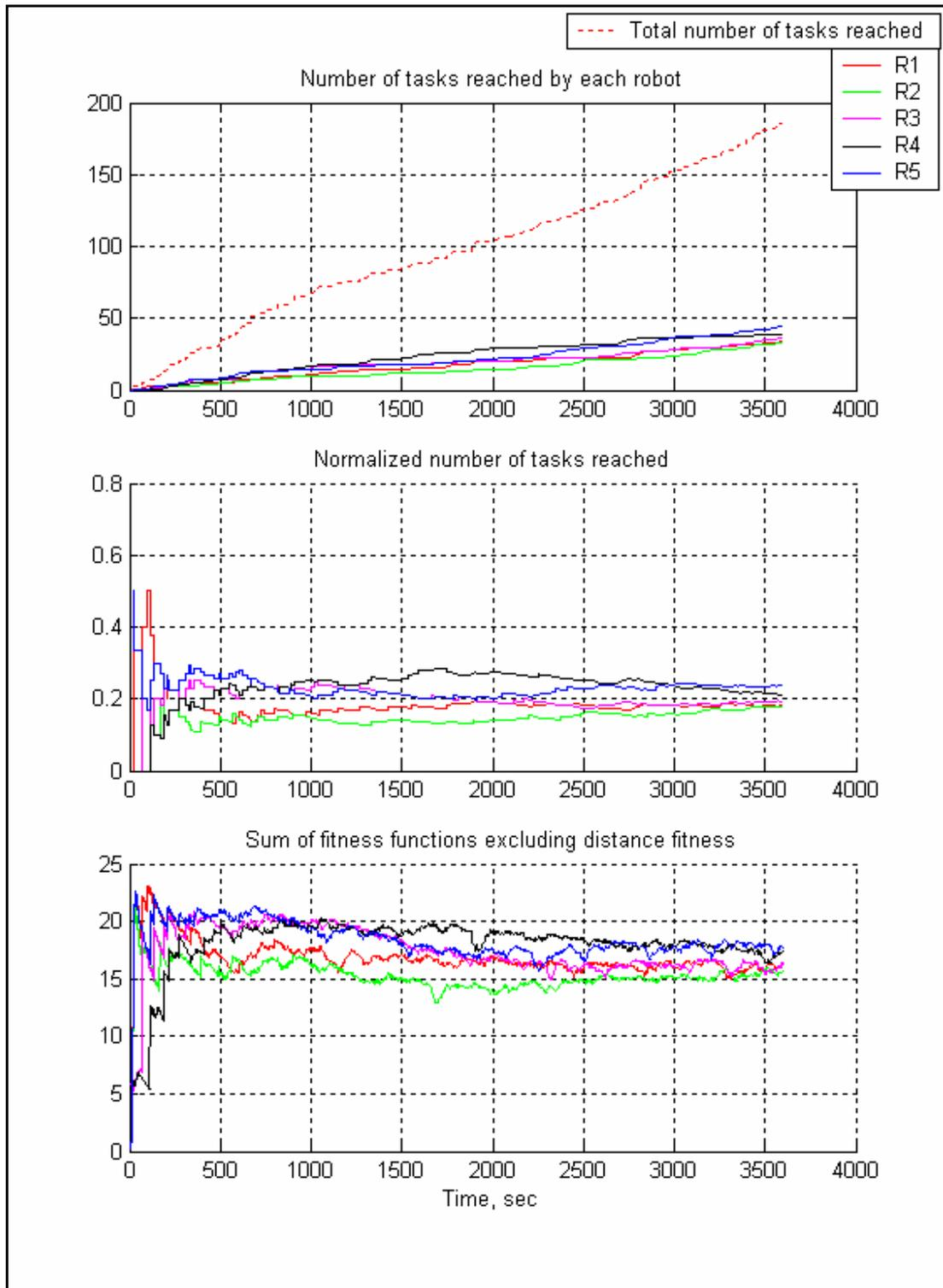
**Figure 90 Only Distance fitness function is activated. Number of tasks reached statistics, and sum of fitness function excluding distance of 5 robots in obstacle-dense region for  $5/(100 \times 100)$  task/m<sup>2</sup> task density**
