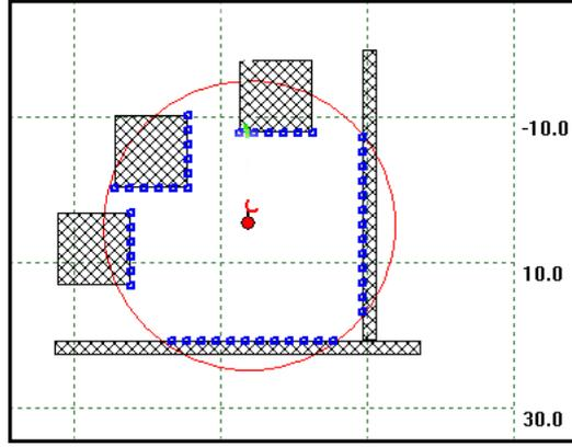
Figure 17, Obstacle particles detected by robot
