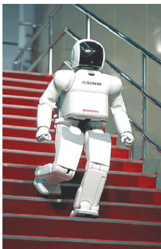
Figure 1.5 ASIMO stepping down the stairs
