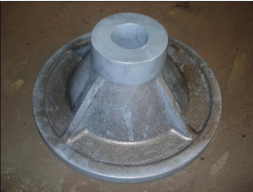
Figure A.8 – Photograph of oil case cover pattern
