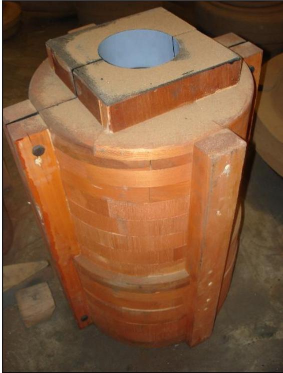
Figure A.5 – Photograph of motor core box
