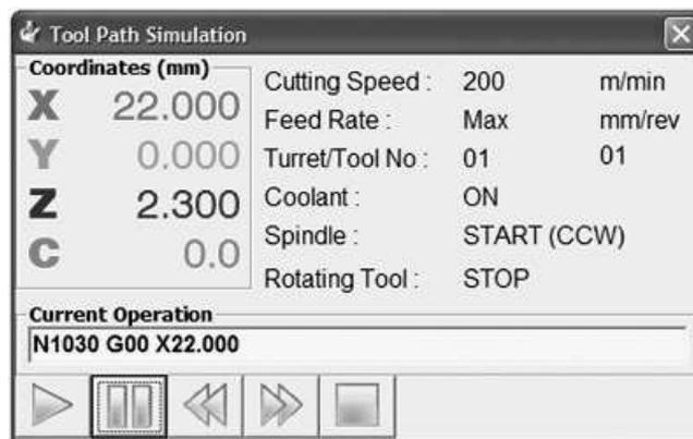
Figure A.27: Part program simulation status window.
