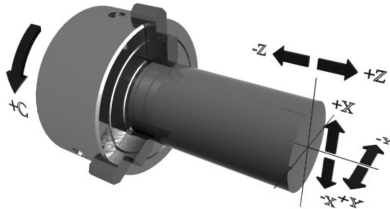
Figure 2.1: Axes of a turning center.
