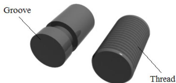
Figure 3.10: Features used to define part turning geometry.
