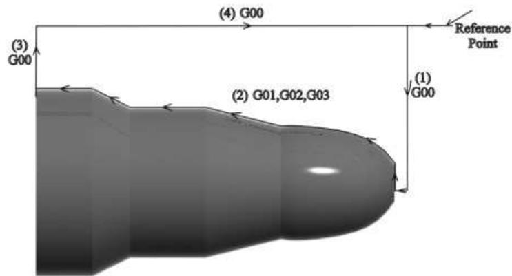
Figure 3.46: Tool path layout for external finishing.
