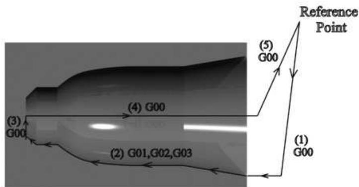
Figure 3.51: Tool path layout for internal finishing.
