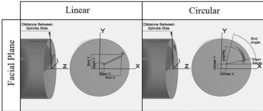
Figure 3.27: Linear and circular path on facial plane.
