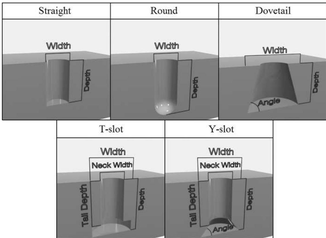
Figure 3.26: Visualization of path cross-sections.
