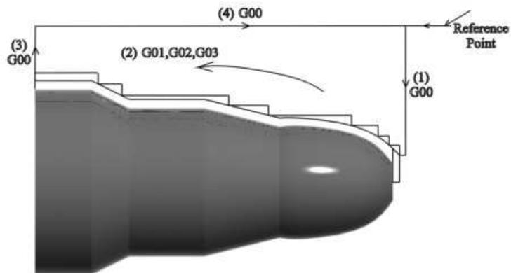
Figure 3.45: Final cut for external roughing.
