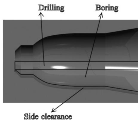
Figure 3.47: Rough inner turning representation.
