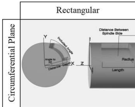
Figure 3.24: Rectangular pocket feature on circumferential plane.
