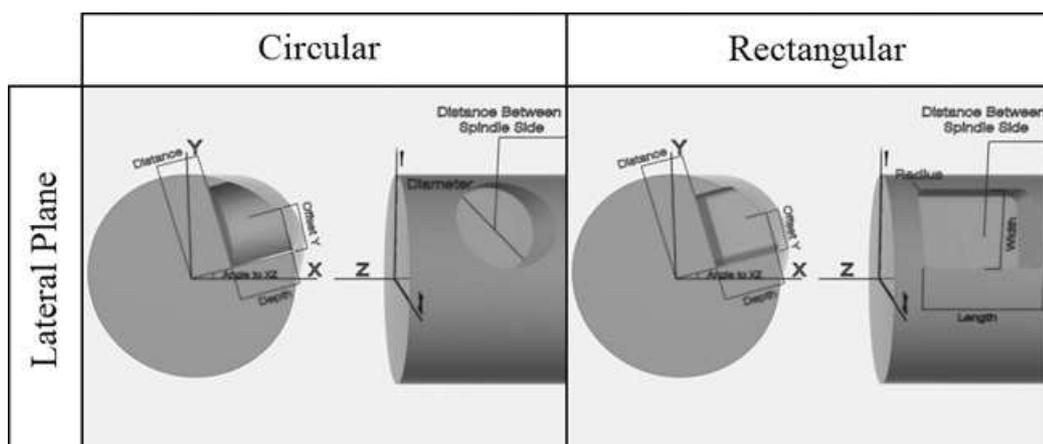
Figure 3.23: Circular and rectangular pocket feature on lateral plane.
