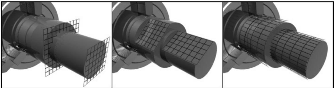
Figure 3.16: Visualization of facial, lateral and circumferential planes.
