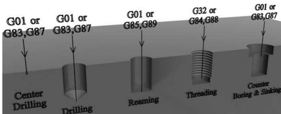
Figure 3.63: Tool path layout for hole milling.
