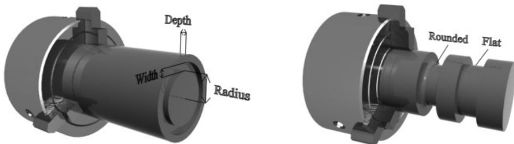
Figure 3.13: Facial groove feature and groove types.
