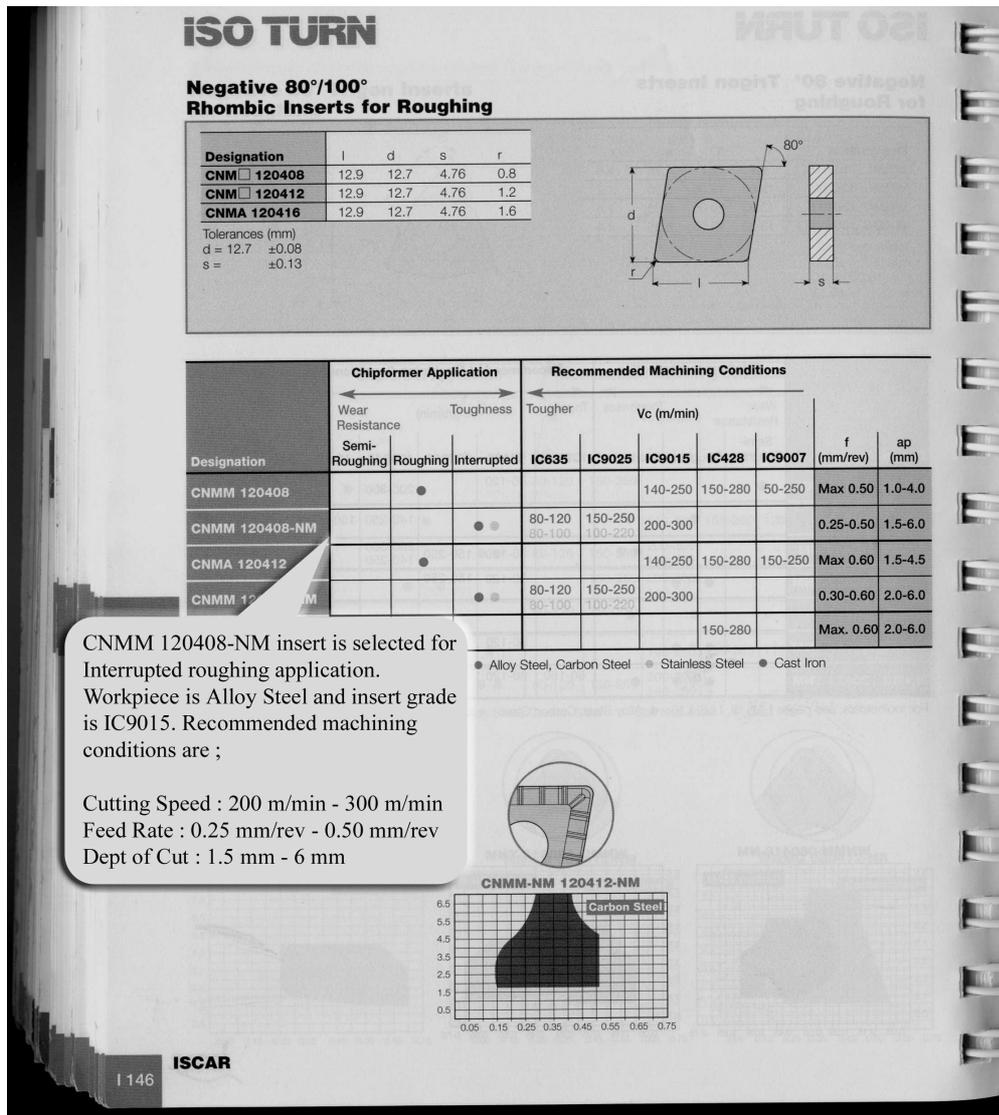
Figure A.23: Insert selection & machining parameters definition.
