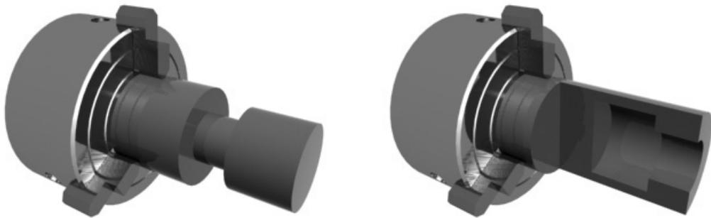
Figure 3.6: Wrong cylinder definitions creating undefined grooves.
