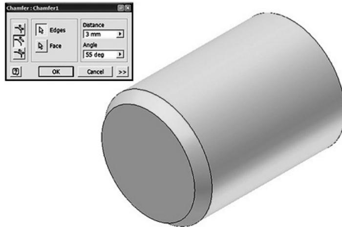
Figure 3.33: Chamfer feature representation.
