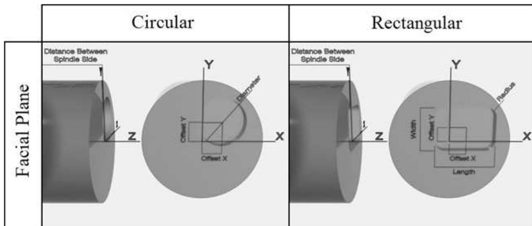
Figure 3.22: Circular and rectangular pocket feature on facial plane.
