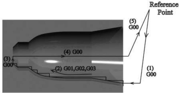
Figure 3.50: Final cut for external roughing.
