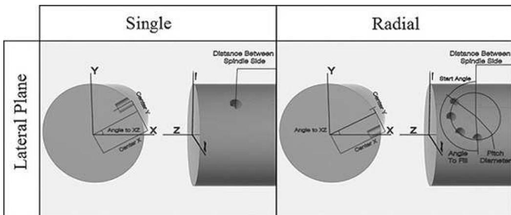
Figure 3.19: Single and radial patterned hole feature on lateral plane.
