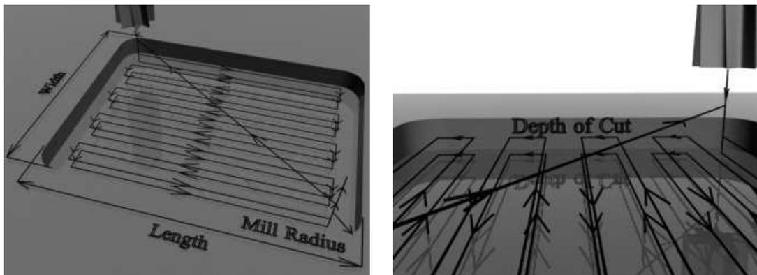
Figure 3.60: Tool path layout for rectangular pocket milling.
