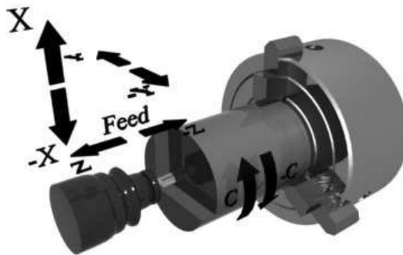
Figure 3.55: NC coordinate system for machining on facial plane.
