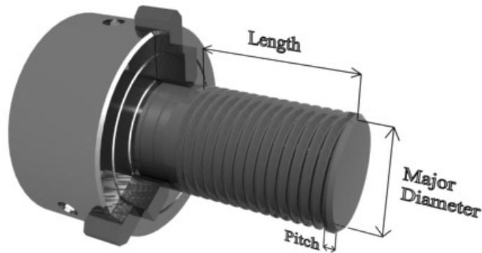
Figure 3.11: Thread feature parameters.
