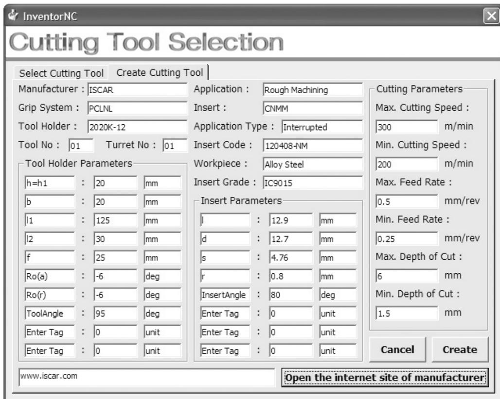
Figure A.24: Cutting tool creation window (Filled).
