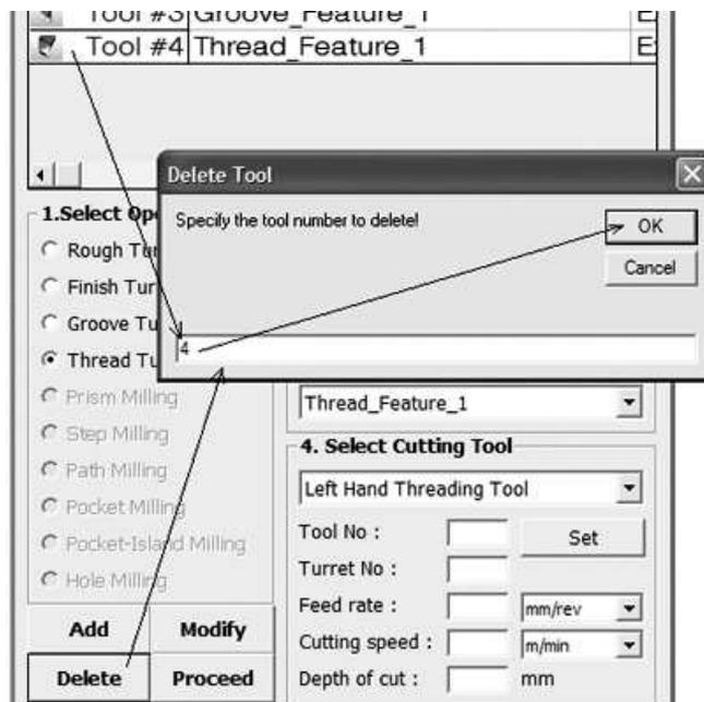
Figure A.19: Delete cutting tool.
