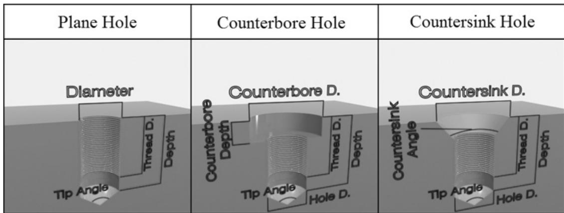
Figure 3.17: Hole feature types and parameters.
