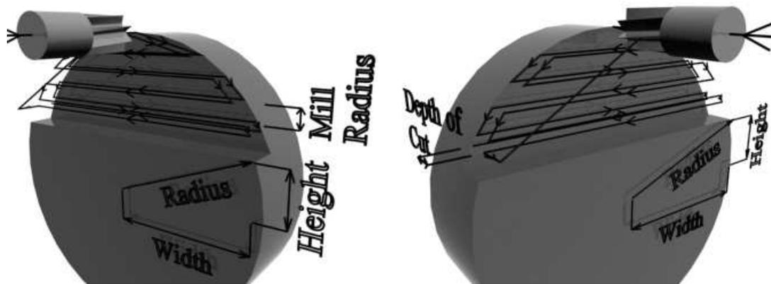
Figure 3.58: Tool path layout for facial step milling.
