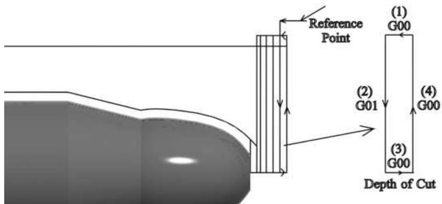
Figure 3.43: Tool path layout for facing.
