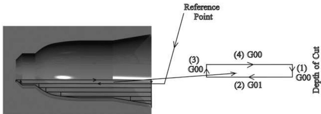
Figure 3.49: Tool path layout for internal roughing.
