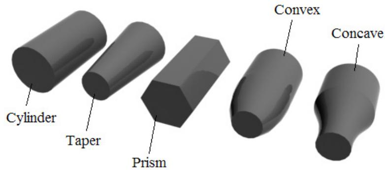
Figure 3.1: Features used to define blank geometry.
