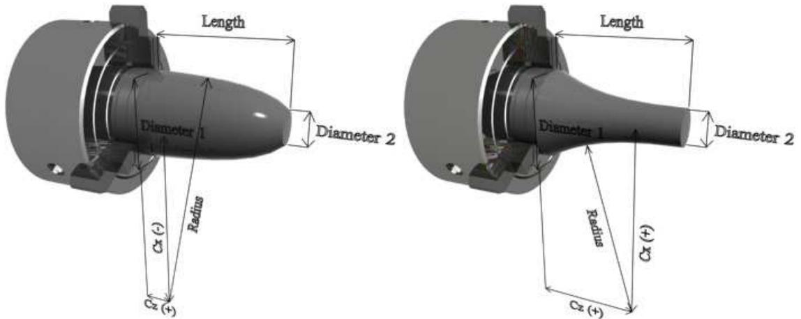
Figure 3.8: Convex and concave feature parameters.
