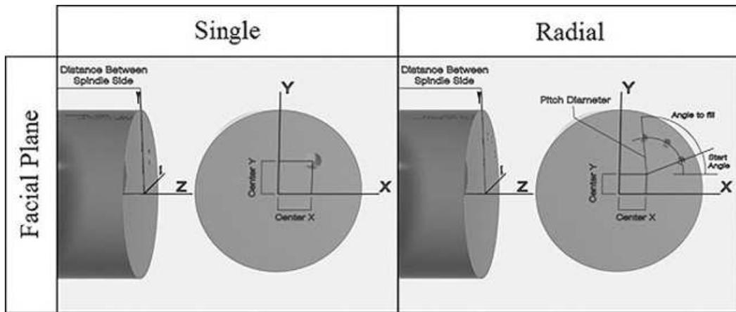
Figure 3.18: Single and radial patterned hole feature on facial plane.
