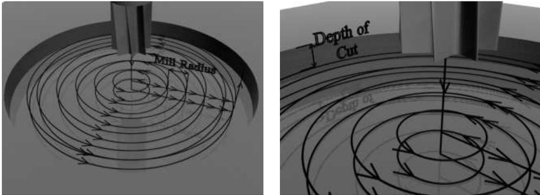
Figure 3.61: Tool path layout for circular pocket milling.
