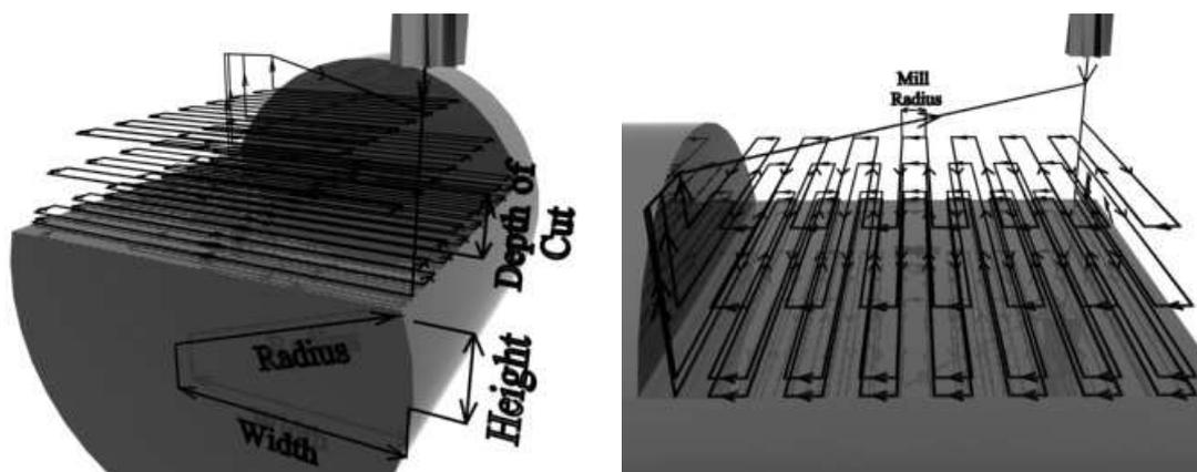
Figure 3.59: Tool path layout for prism and lateral step milling.
