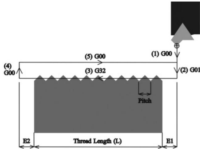
Figure 3.54: Tool path layout for external threading.
