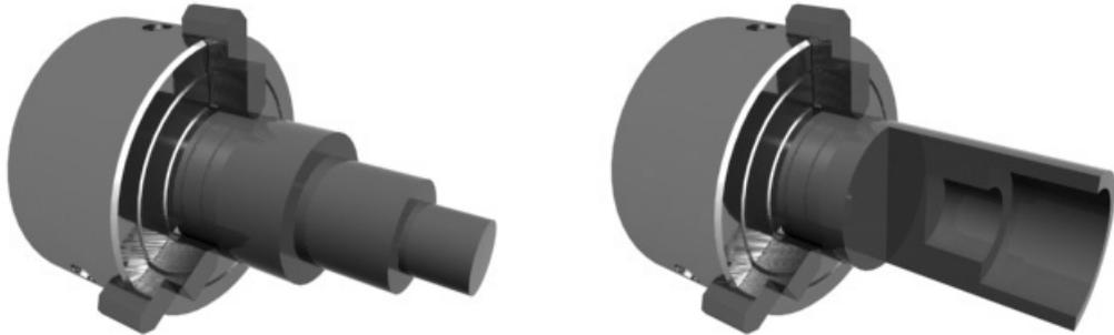
Figure 3.5: Simultaneous cylinder definitions for inner and outer profile.
