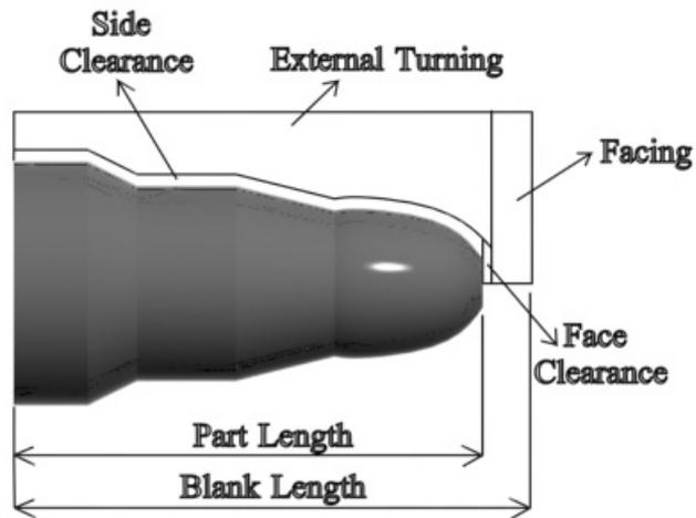
Figure 3.42: Rough outer turning representation.
