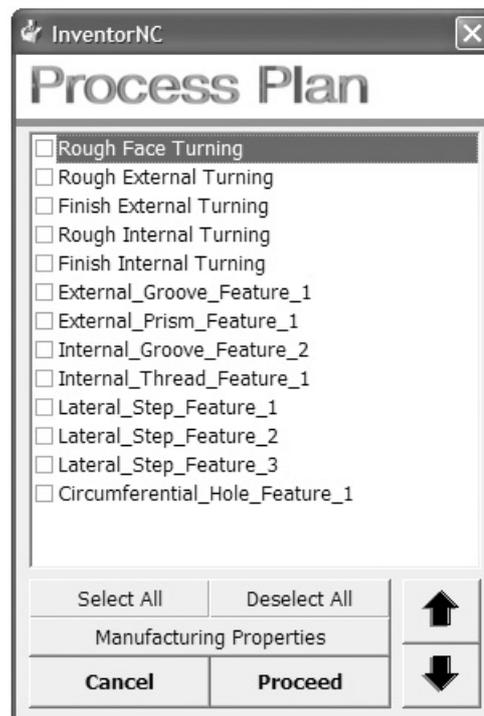
Figure A.15: Process plan window.
