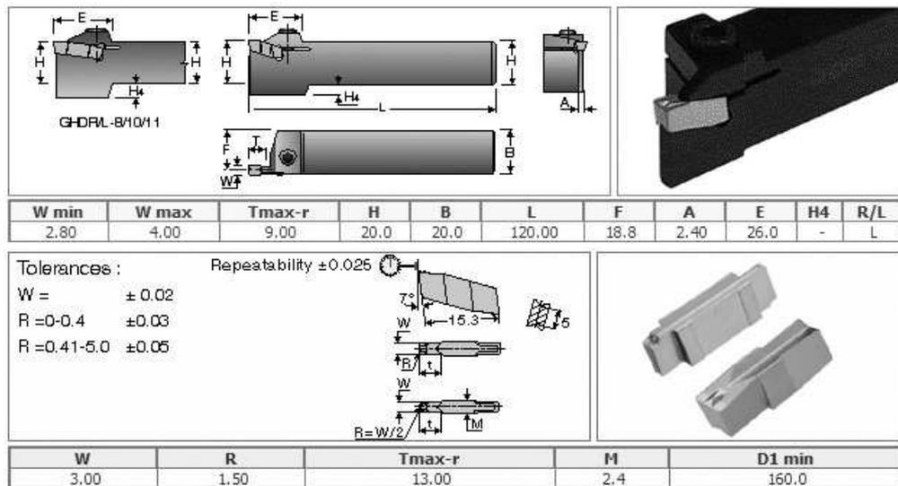
Figure 4.15: Holder and insert dimensions of Tool#3.
