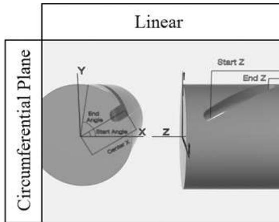
Figure 3.29: Linear path on circumferential plane.
