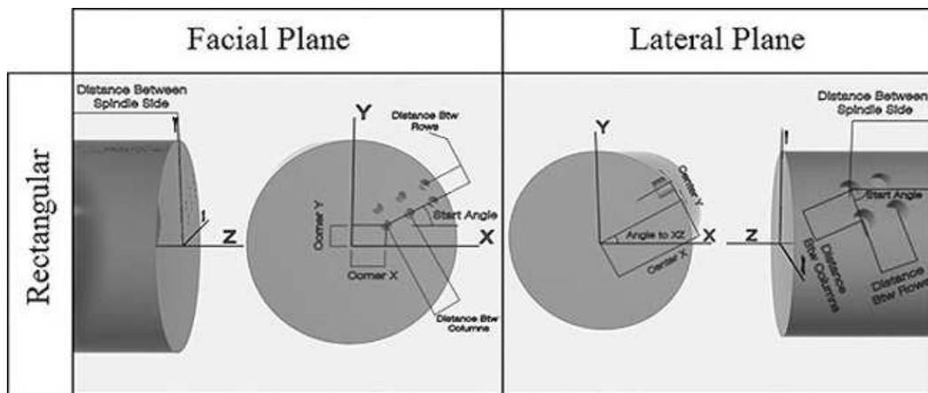
Figure 3.20: Rectangular patterned hole feature on facial and lateral plane.
