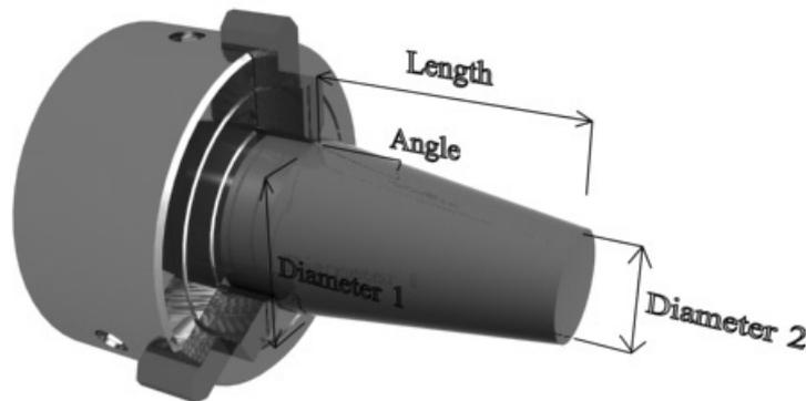
Figure 3.7: Taper feature parameters.
