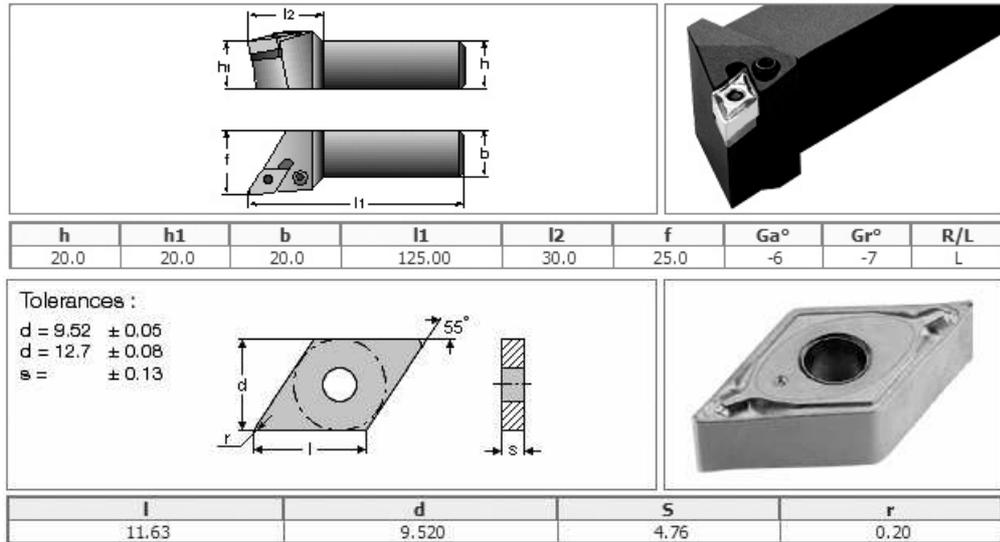
Figure 4.14: Holder and insert dimensions of Tool#2.
