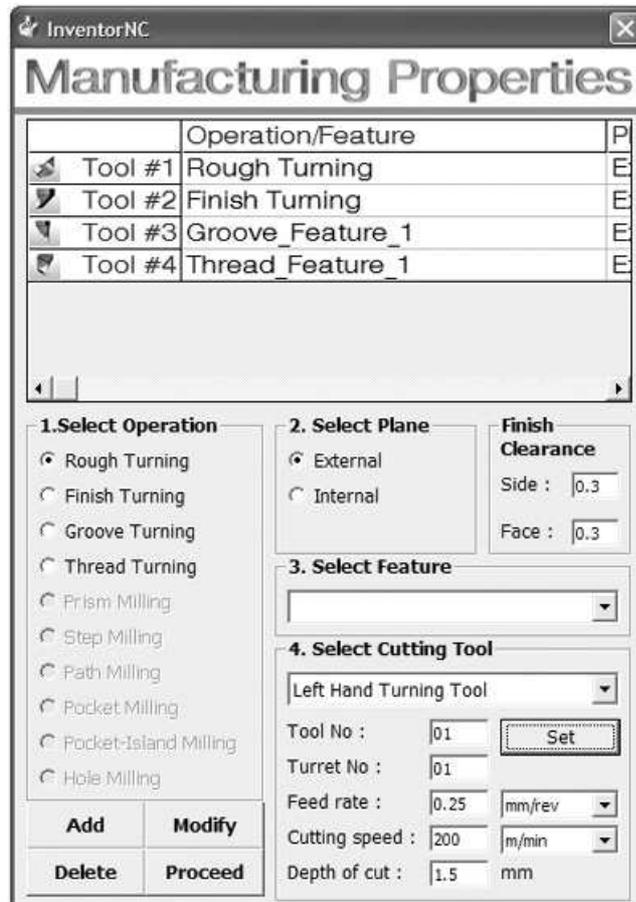
Figure A.16: Process plan window.
