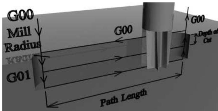
Figure 3.62: Tool path layout for path milling.
