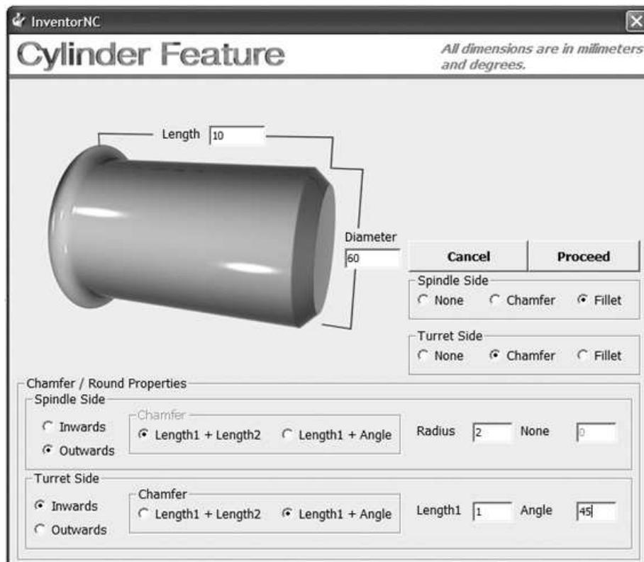
Figure A.11: Cylindrical feature information entry window.
