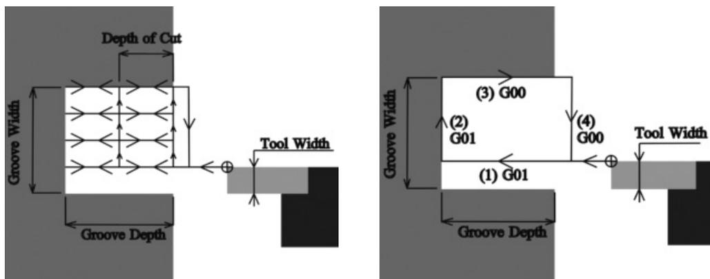
Figure 3.53: Tool path layout for facial grooving.
