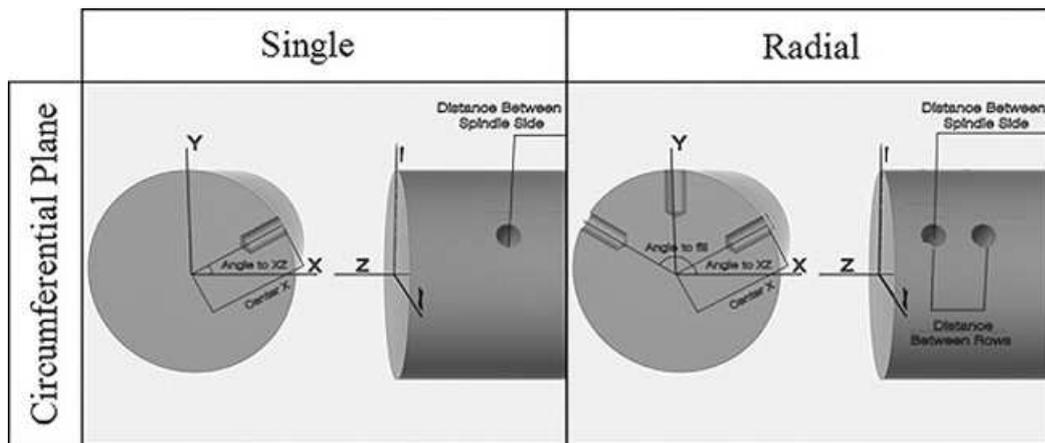
Figure 3.21: Single and radial patterned hole feature on circumferential plane.
