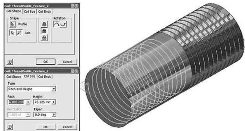
Figure 3.35: Coil feature representation for creating threads.
