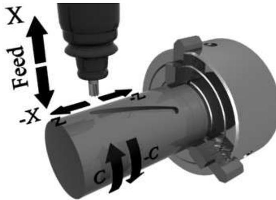
Figure 3.57: NC coordinate system for machining on circumferential plane.
