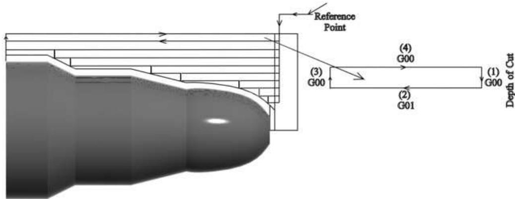
Figure 3.44: Tool path layout for external roughing.
