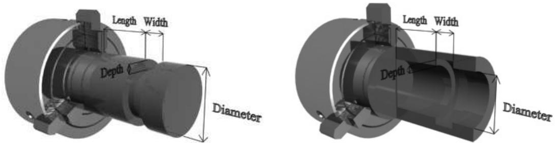
Figure 3.12: Groove feature parameters.
