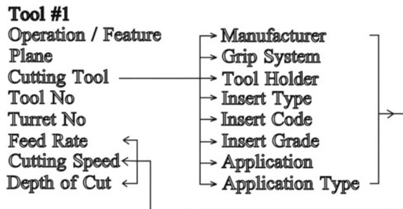
Figure 3.39: Classification of tool definition algorithm.
