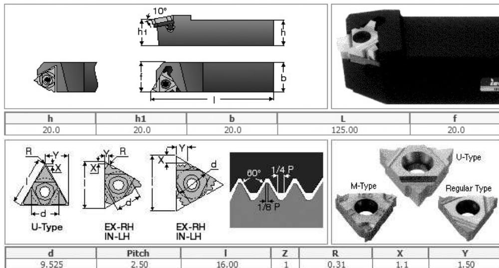
Figure 4.16: Holder and insert dimensions of Tool#4.
