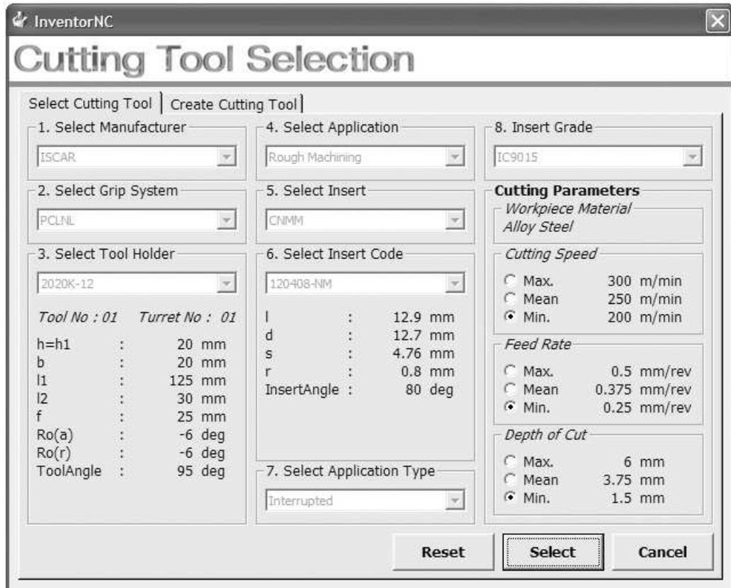
Figure A.17: Cutting tool selection window.
