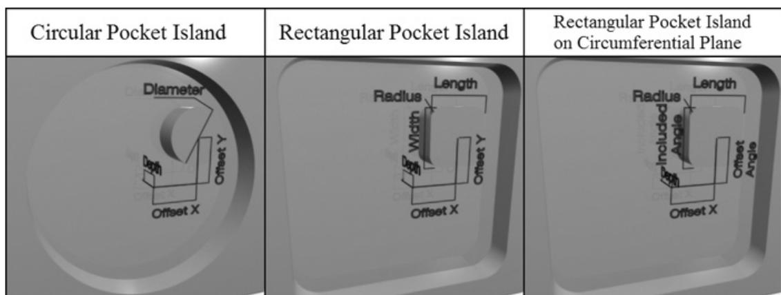
Figure 3.25: Circular and rectangular pocket-island feature on each milling plane.
