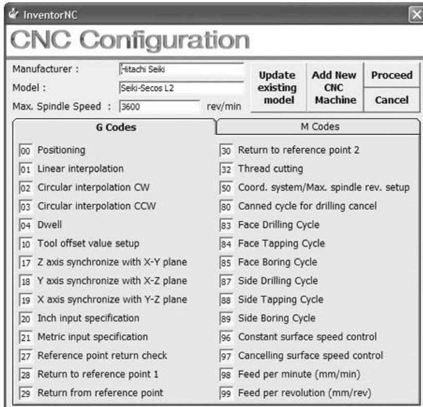
Figure A.6: CNC configuration window.
