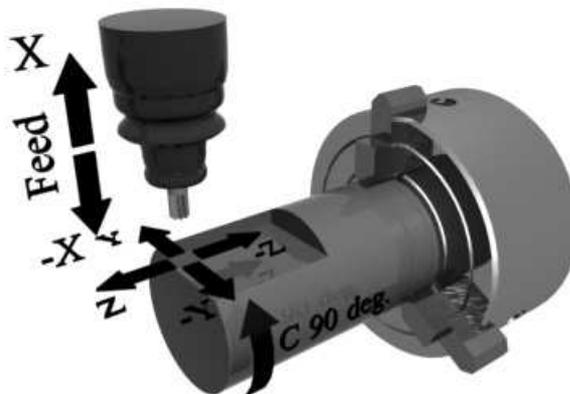
Figure 3.56: NC coordinate system for machining on lateral plane.
