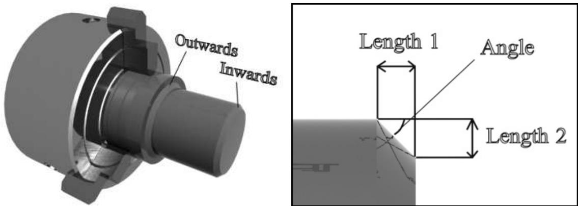
Figure 3.14: Chamfer feature parameters.
