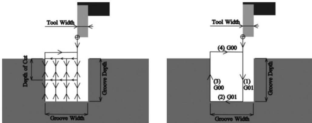
Figure 3.52: Tool path layout for external grooving.
