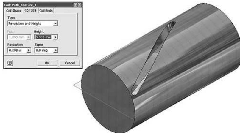
Figure 3.36: Coil feature representation for circumferential path.
