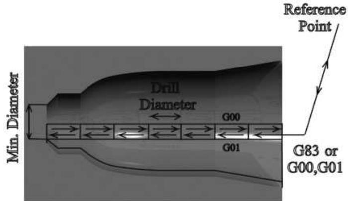
Figure 3.48: Tool path layout for drilling.
