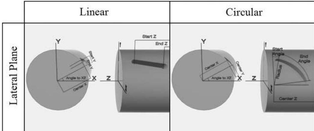
Figure 3.28: Linear and circular path on lateral plane.
