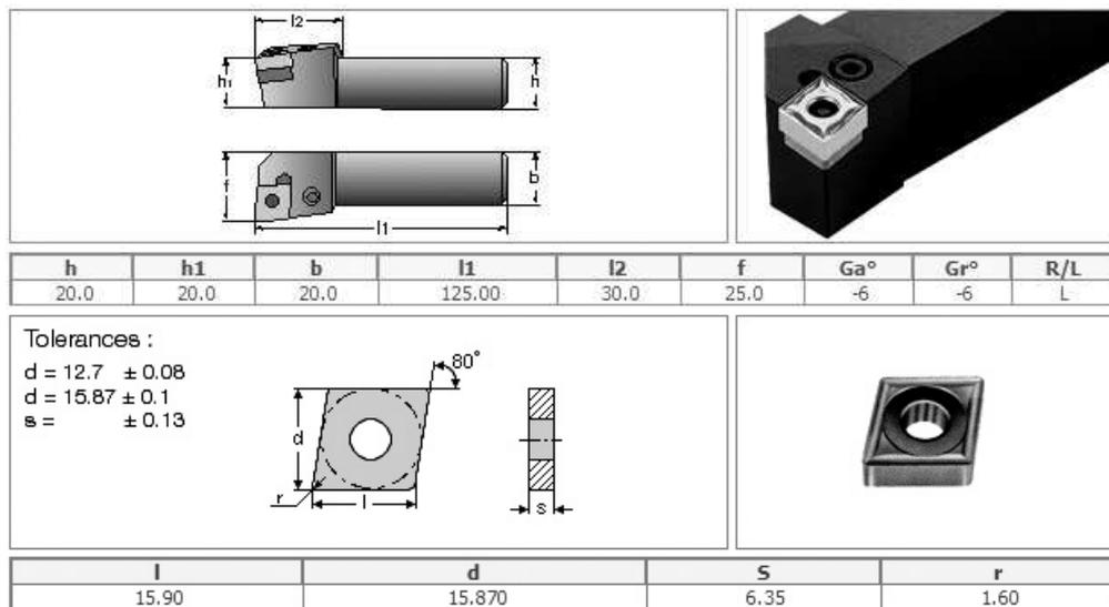
Figure 4.13: Holder and insert dimensions of Tool#1.
