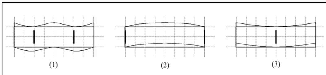
**Figure 4.33:** Behaviour of the diaphragm according to the locations of shear walls
