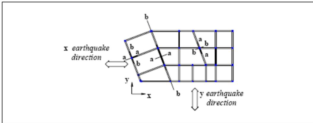
**Figure 4.35:** Nonparallel Axes of Structural Elements
