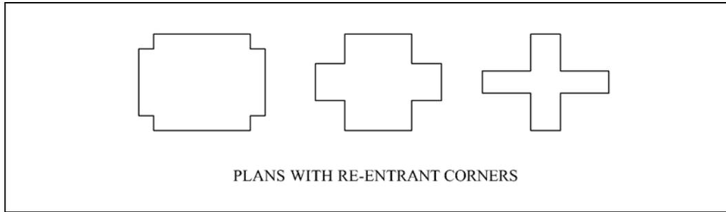
**Figure 4.8:** Re-entrant corners in plan
