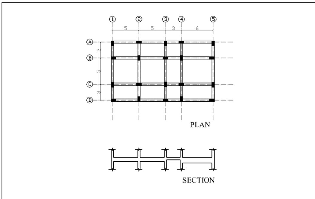
**Figure 4.26:** The depth of the beams due to spans
