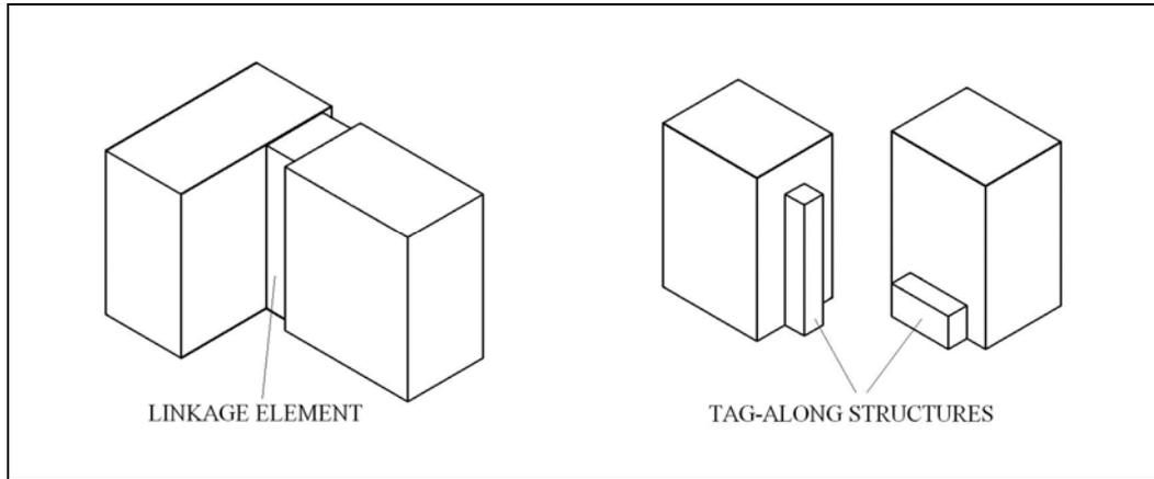
**Figure 4.14:** Buildings with linkage element and tag-along structures
