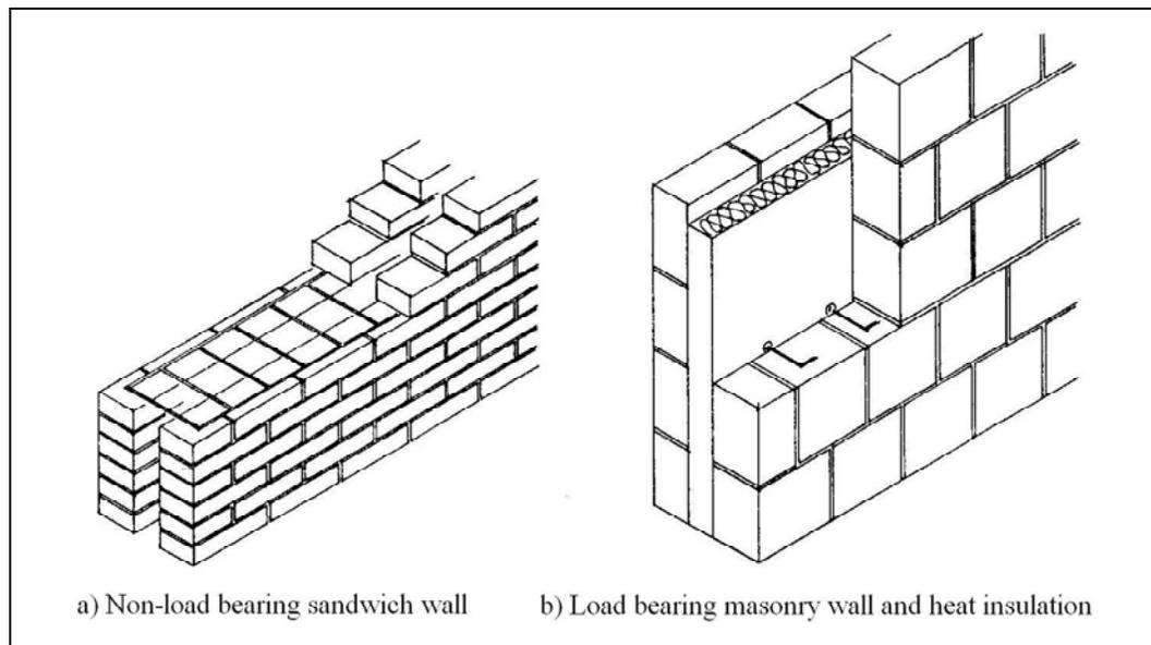
**Figure 4.53:** Details for sandwich wall (Erman, 2002, p.83)
