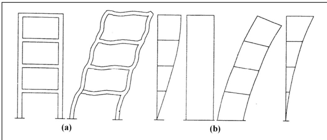
**Figure 4.39:** The deformations of frame system (a) and the shear wall system (b) (Bayülke, 2001, p.138)
