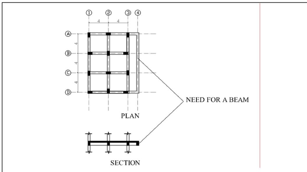
**Figure 4.28:** Beam for cantilever
