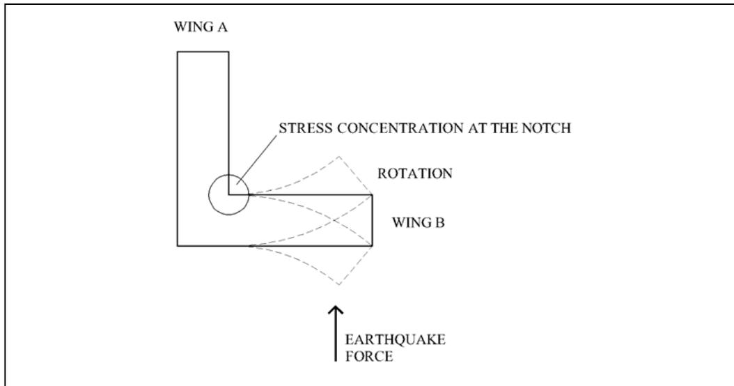
**Figure 4.10:** L-shaped building behaviour under earthquake force
