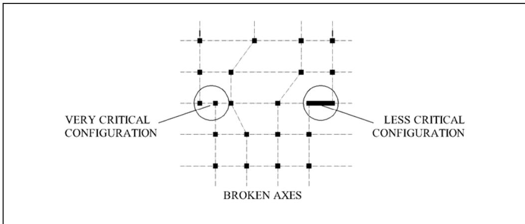
**Figure 4.22:** Frames with broken axes
