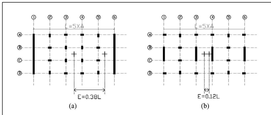
**Figure 4.23:** Eccentricity due to shear walls arrangement
