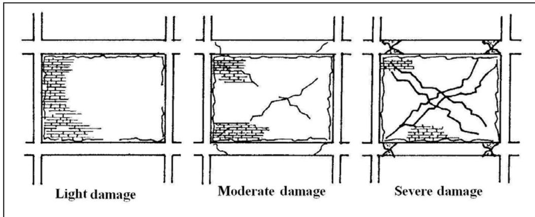
**Figure 4.48:** Level of damages of infill walls inserted in a frame (Erman, 2002, p.78)
