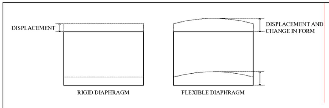
**Figure 4.31:** Behaviour of the diaphragm under earthquake loading
