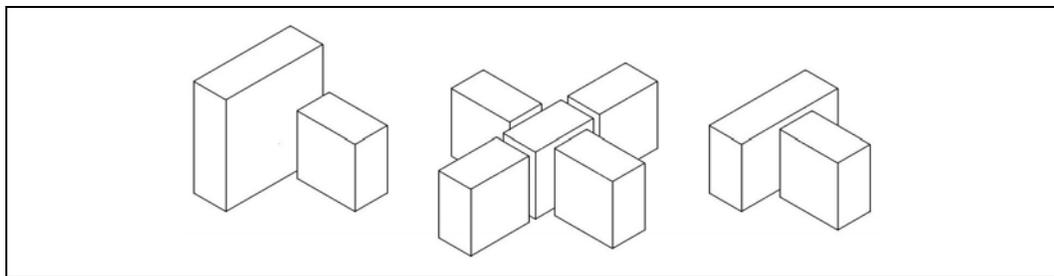
**Figure 4.11:** Separation of buildings into portions
