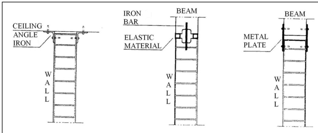
**Figure 4.49:** Details for an infill wall in order to prevent overturning out of its plane (Bayülke, 2001, p.90)
