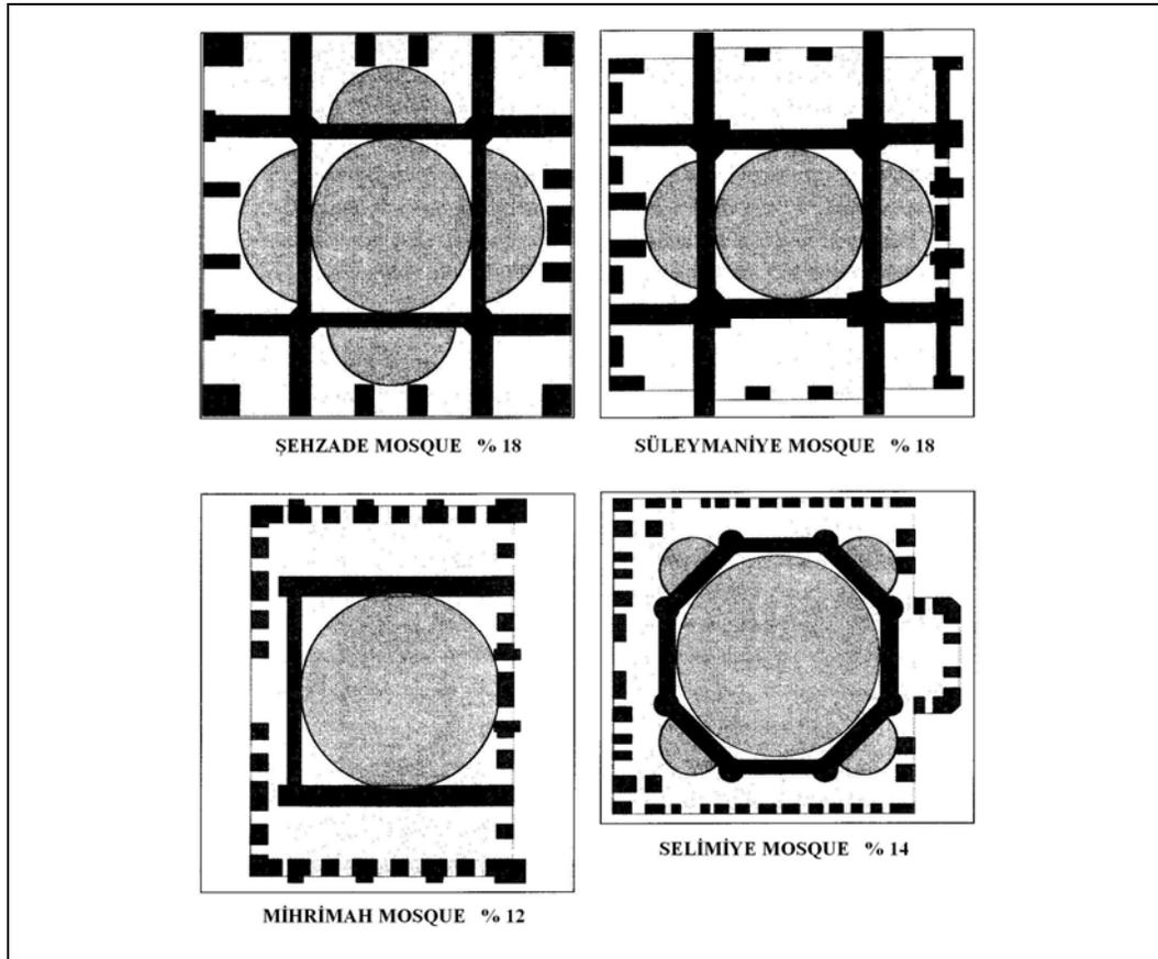
**Figure 4.37:** The structural plan density of historical buildings (Ünay, 2002, p.73)
