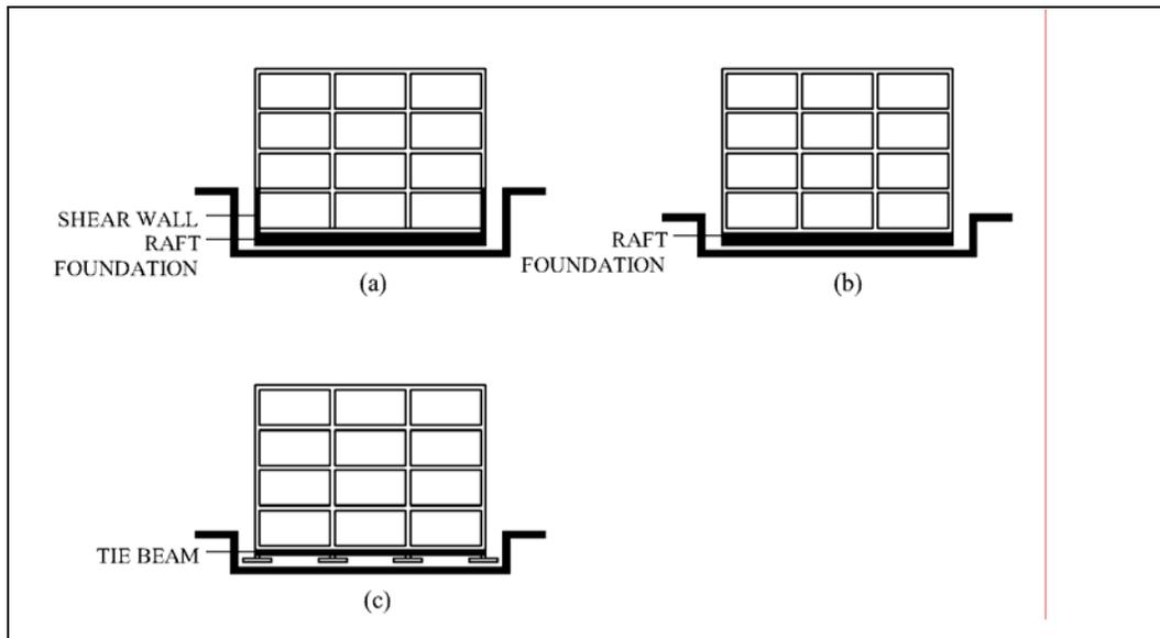
**Figure 4.47:** Type of foundations for seismic zones
