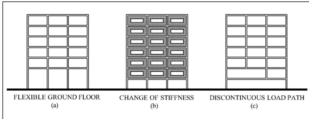
**Figure 4.41:** The causes of soft storey formation
