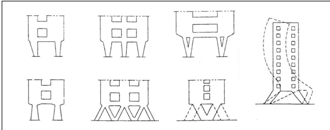
**Figure 4.38:** The inclined base of the shear walls and its behaviour due to earthquake forces (Bayülke, 2001, p.137)
