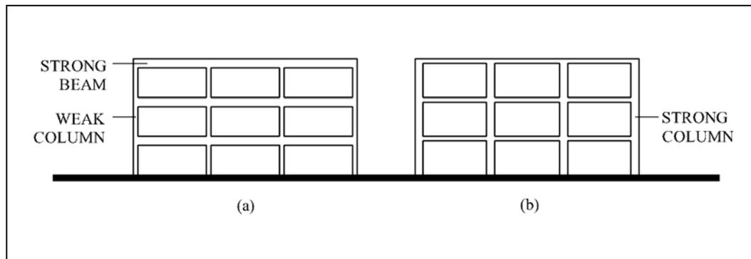
**Figure 4.44:** The weak-column, strong-beam formation
