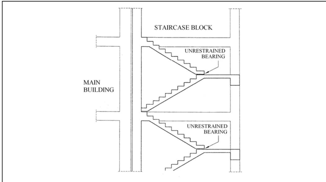
**Figure 4.54:** Details in order to prevent damage of staircases (Bayülke, 2001, p.96)
