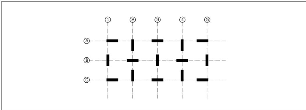
**Figure 4.24:** Distribution of the shear walls within the building
