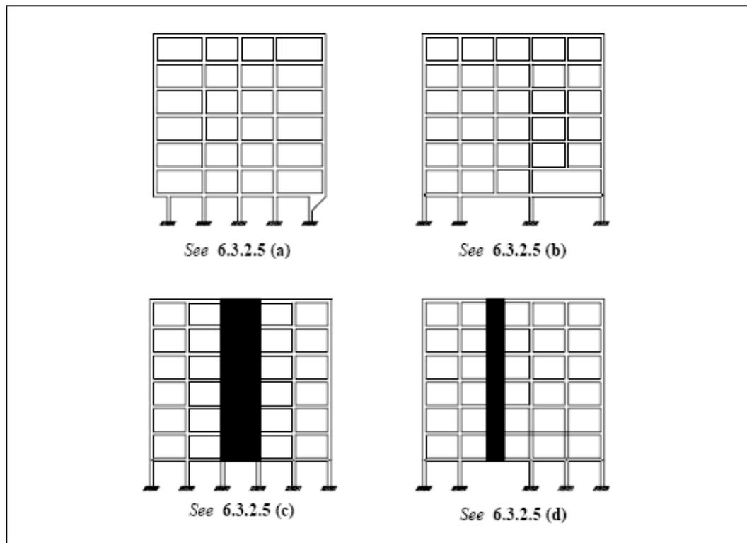
**Figure 4.43:** Discontinuity of vertical structural elements
