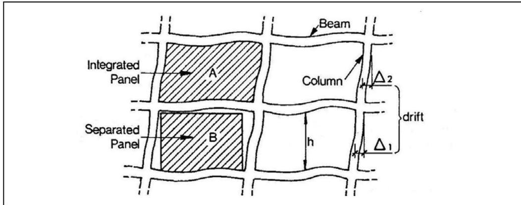
**Figure 4.50:** Two opposite approaches for frame and non-structural infill wall
