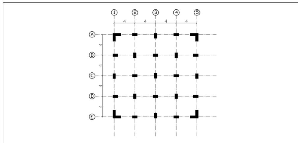
**Figure 4.20:** L-shaped columns and shear walls on the corners
