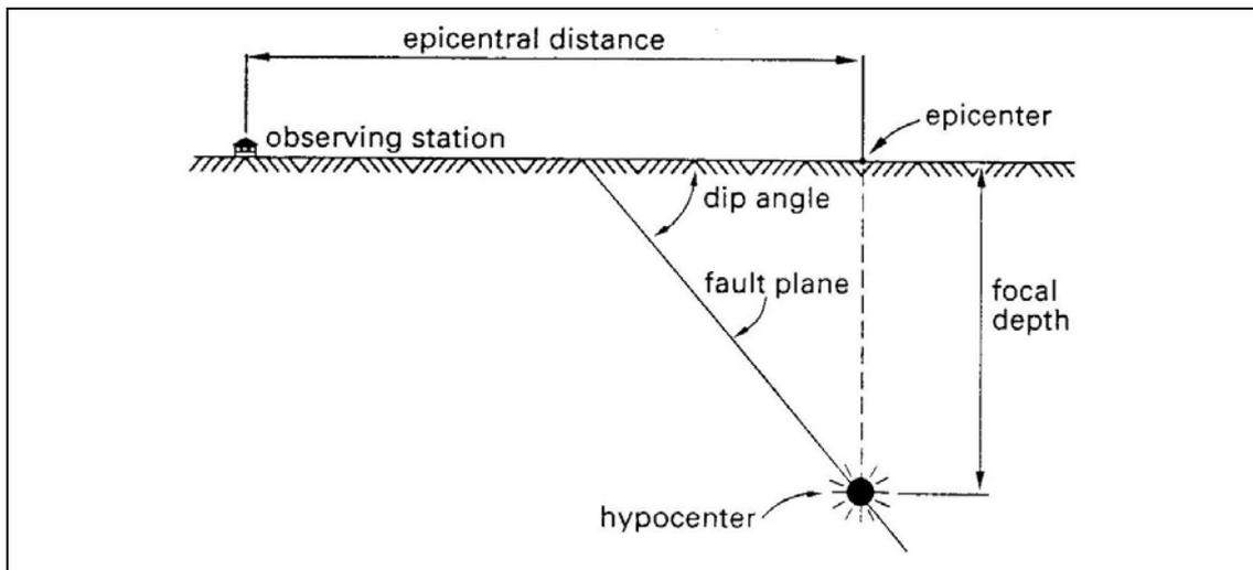
**Figure 2.3:** Earthquake terminology (Lindeburg and Baradar, 2001, p.2)
