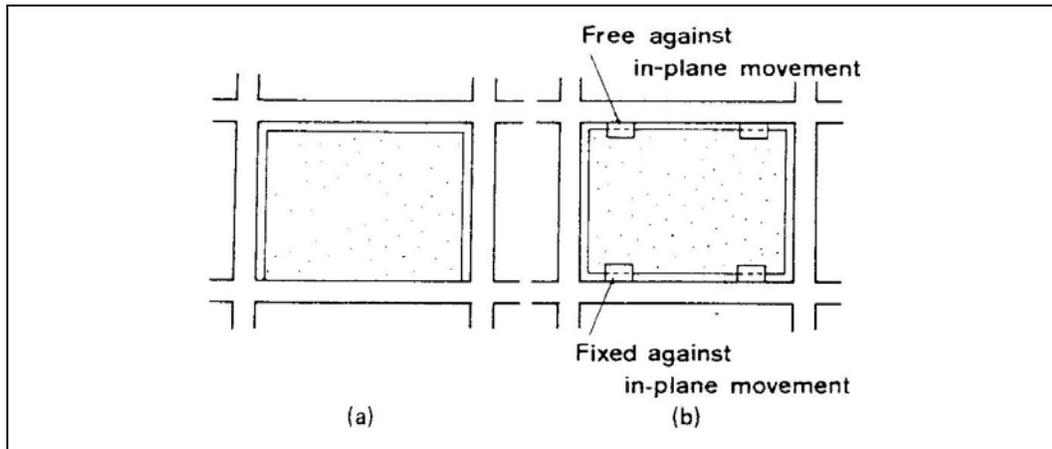
**Figure 4.51:** Separating the infill wall from the structure (Wakabayashi, 1986, p.269)
