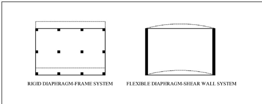
**Figure 4.32:** Behaviour of the diaphragm according to the structural system
