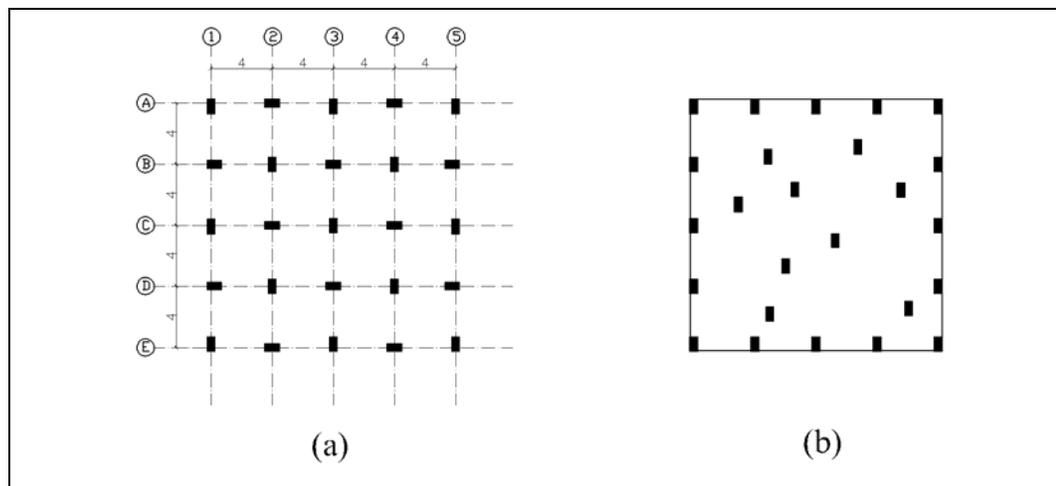
**Figure 4.19:** Regular and irregular vertical structural system configuration in plan
