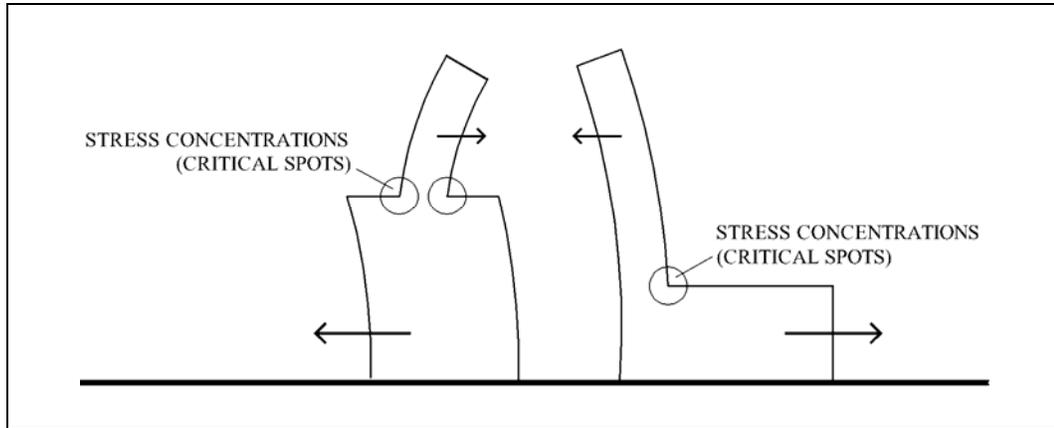
**Figure 4.15:** Stress concentrations due to setbacks
