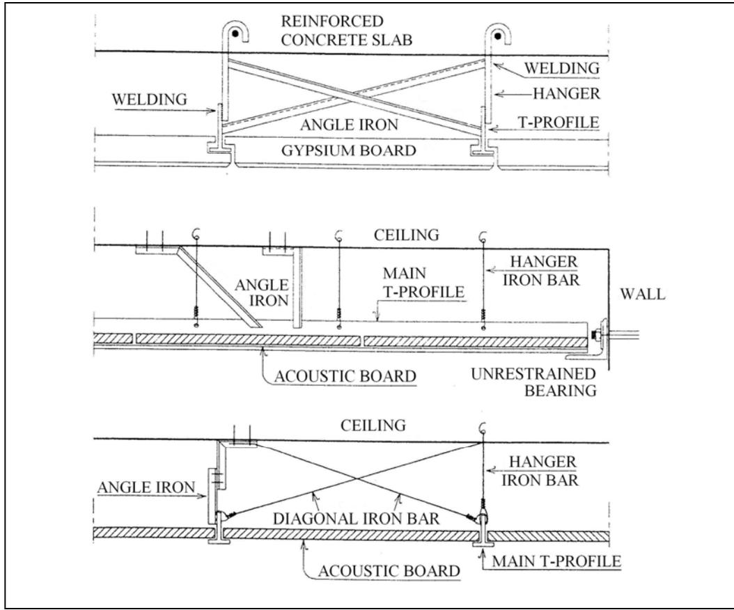
**Figure 4.57:** Details of suspended ceiling construction (Bayülke, 2001, p.100)
