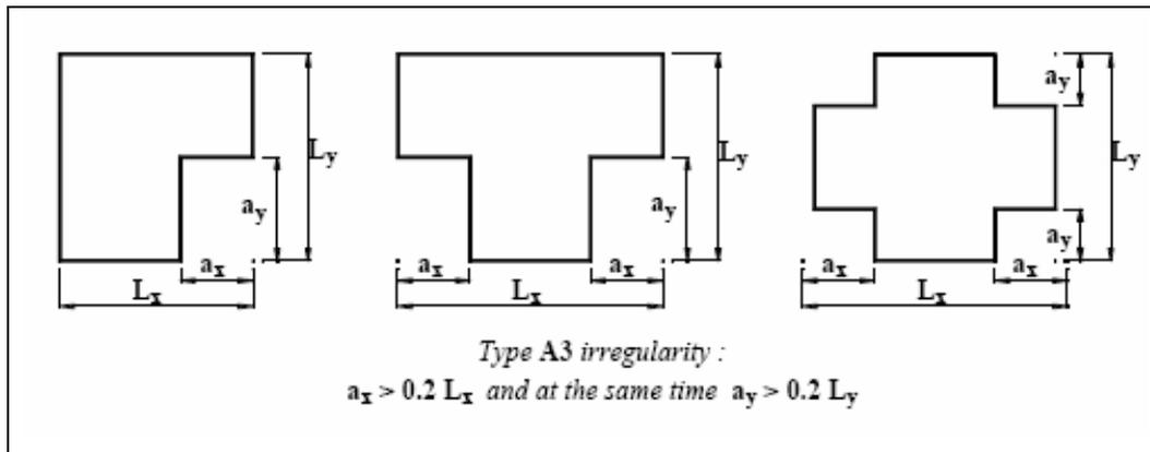
**Figure 4.9:** Projections in Plan (Turkish Earthquake Code, 1998, p.9)
