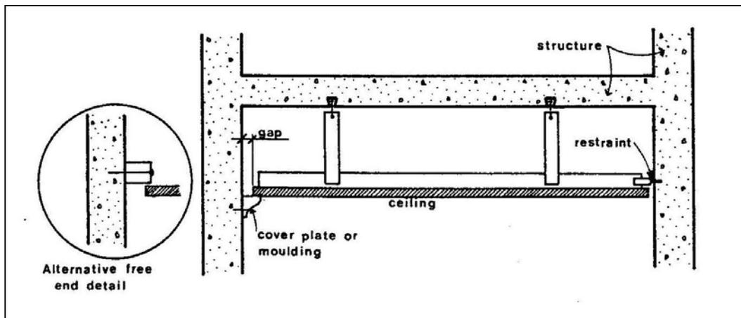
**Figure 4.56:** Details of suspended ceiling to prevent hammering and excessive movement (Dowrick, 1987, p.451)
