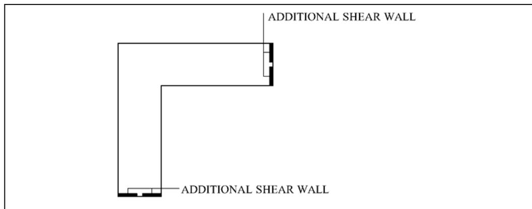
**Figure 4.12:** Additional shear wall to free end of wings
