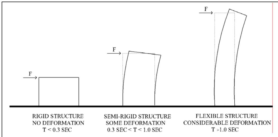
**Figure 4.4:** Seismic response of buildings with different heights
