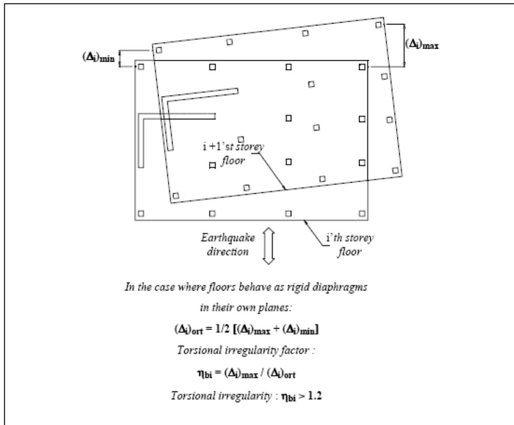
**Figure 4.30:** Torsional Irregularity (Turkish Earthquake Code, 1998, p.8)
