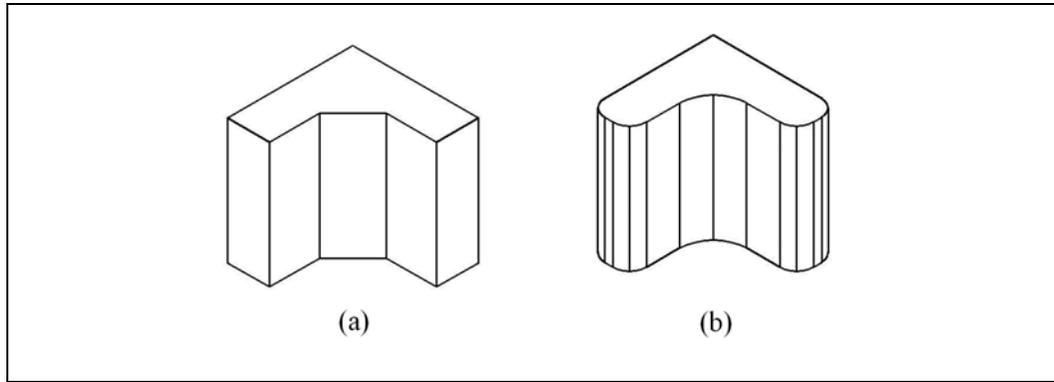
**Figure 4.13:** Softening the right-angle re-entrant corner
