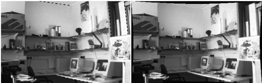
**Figure 2.6:** Radial distortion example [1]: Notice the distortion in the linear lines in the left image. Right image is the corrected one; lines are straight in this image.
