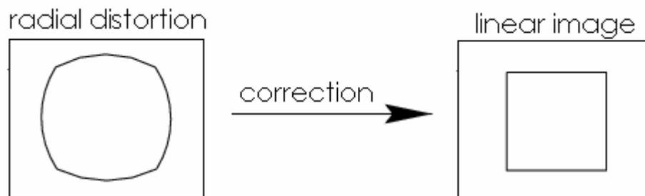
**Figure 2.5** Radial distortion [1]: Left image represents the image before correction and right image is the corrected linear image.
