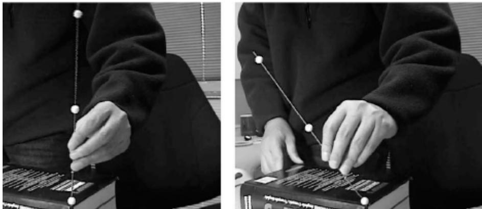
**Figure 2.9:** 1D calibration pattern [8]
