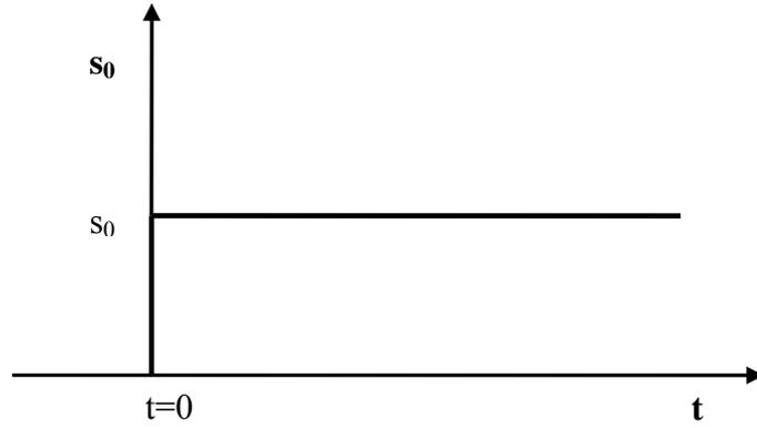
**Figure 2.9:** Stage hydrograph for a sudden rise in the stream level.
