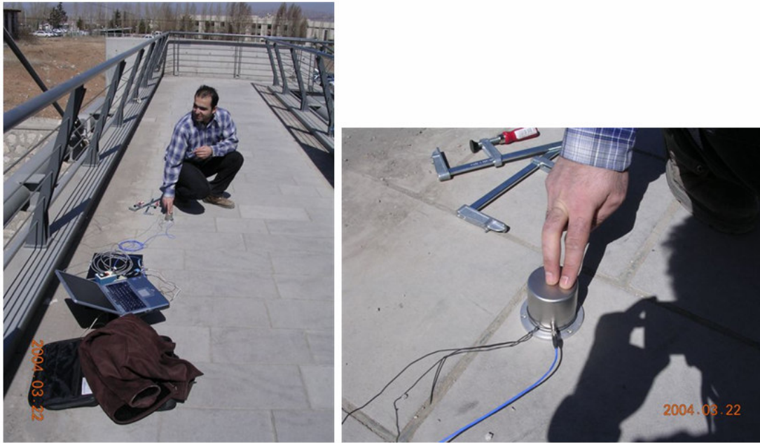
Figure 4-8: Dynamic test views on the deck
