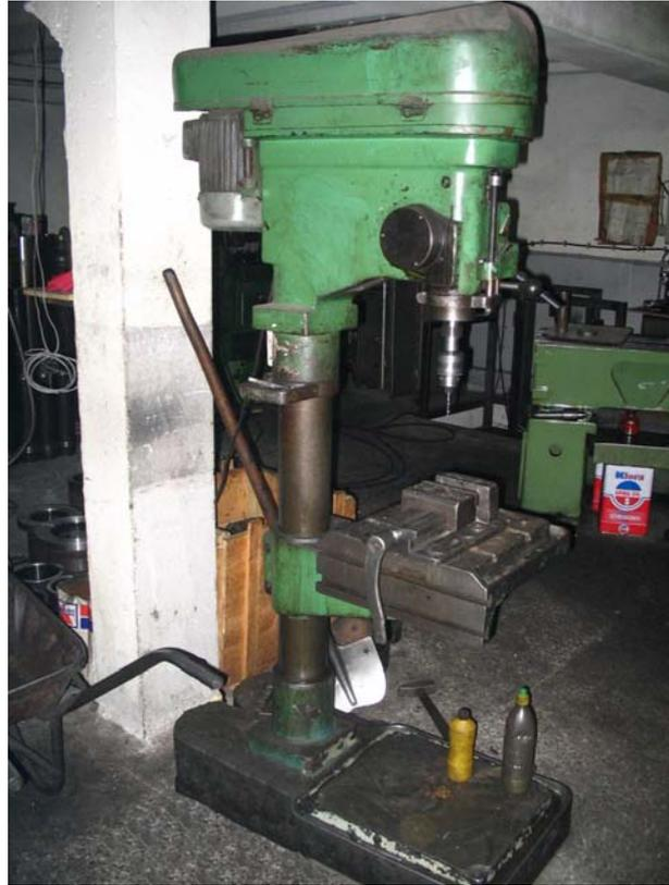
Figure A.10 A View of Vertical Drilling Machine
